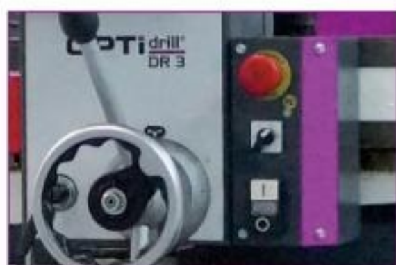
Controls with 24 V DC electrical system
