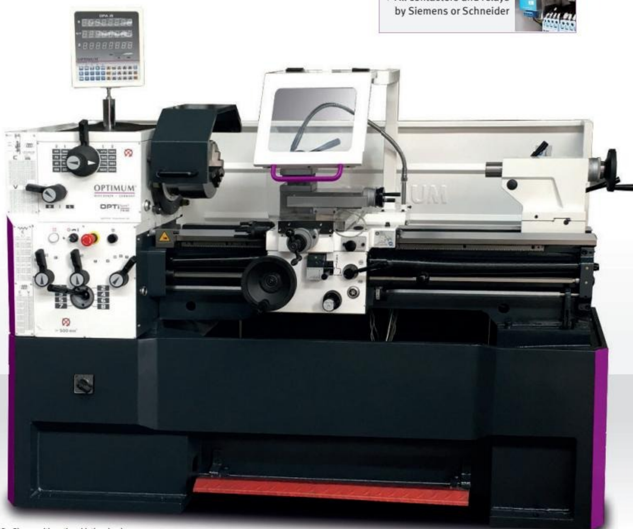
Fig.: TH 4210D - Shown with optional lathe chuck
