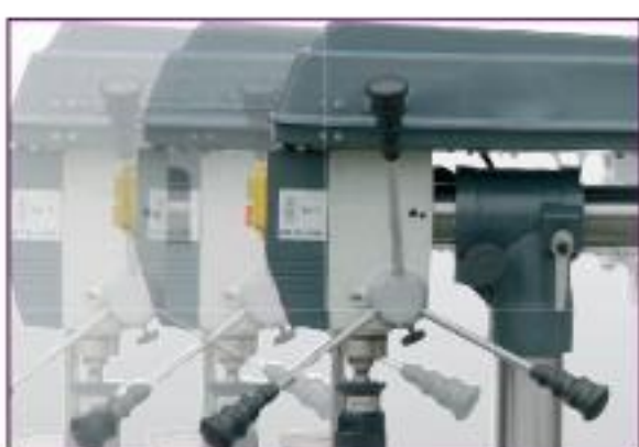
› Variable outreach by displacing the drilling head
