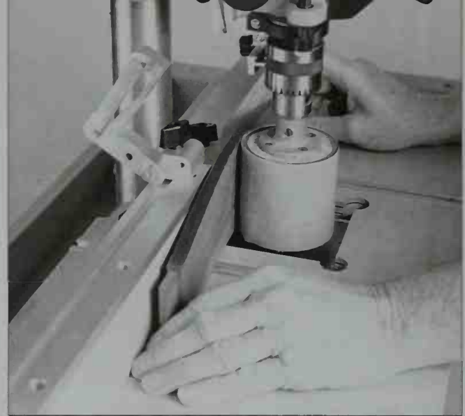
6-40. The sanding drum on the drill press is used to finish the concave side. A micro-adjuster on this drill press allows multiple passes to be adjusted in small increments
