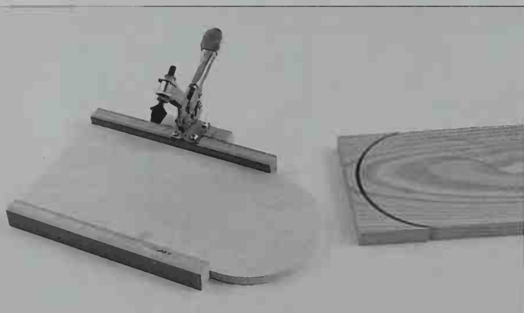
6-21. The half-circle jig consists of a piece of plywood with strips of plywood nailed to its sides. An adjustable clamp is used to hold the workpiece during the saw cut.
