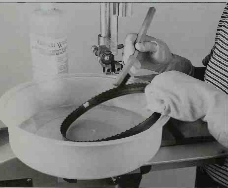
2-34. Use a stiff bristle or fine wire brush to clean coarse-tooth blades.
