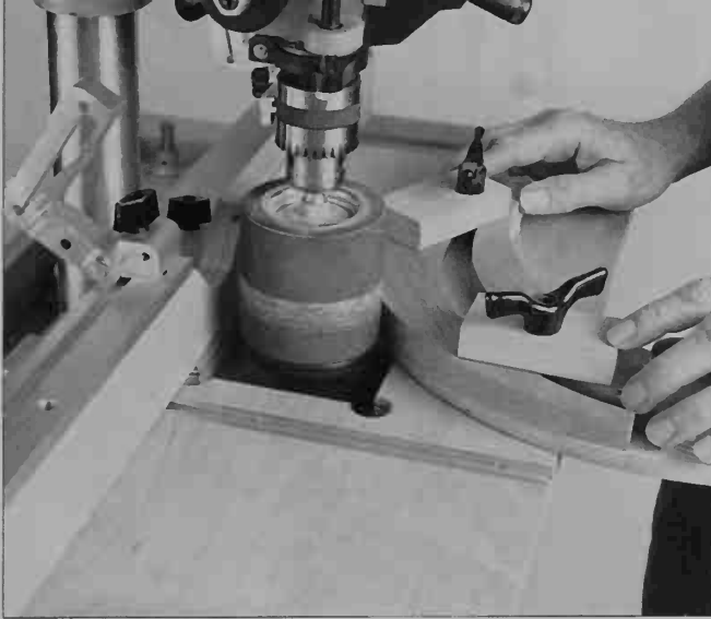
6-36. Using the sander in a drill press.
