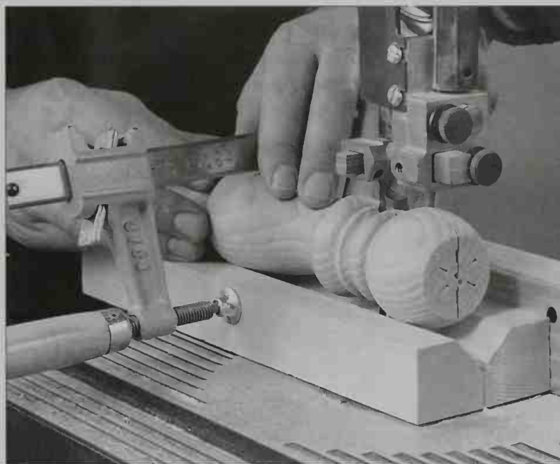
6-1. A V-block is a simple fixture that can be used for a variety of purposes, including cutting round stock.
