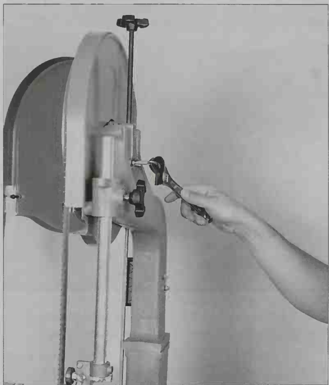
4-1. One way to make it easier to back a blade out of a cut is to tilt the top wheel backward slightly. Turn the saw off before doing this.
