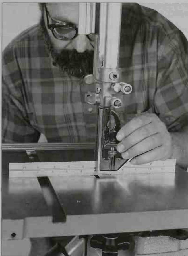
3-27. Use a square to ensure that the blade and table are at 90 degrees to each other.
