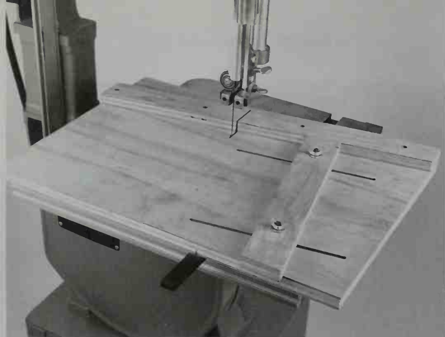
4-77. The tails are first cut with a plywood jig that holds the workpiece at a 10-degree angle.
