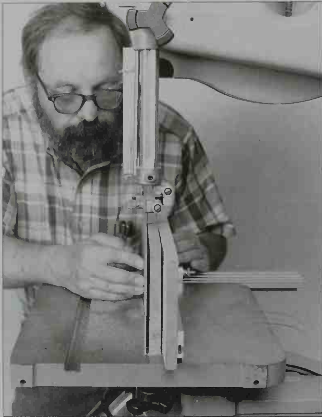
4-57. When resawing, feed the workpiece slowly, applying pressure against the fence just behind the blade. For safety reasons, never apply pressure next to the blade.
