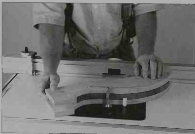
6-46. A sandwich jig permits the woodworker to cut with the grain by flipping the assembly when the wood grain changes directions. The white plastic peg is a starting pin, which helps in starting and stopping the cut.
