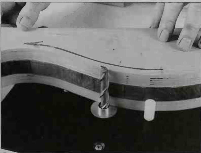
6-50. The router cutting the sandwiched workpiece. The bottom pattern contacts the guide bushing in the router-table plate.
