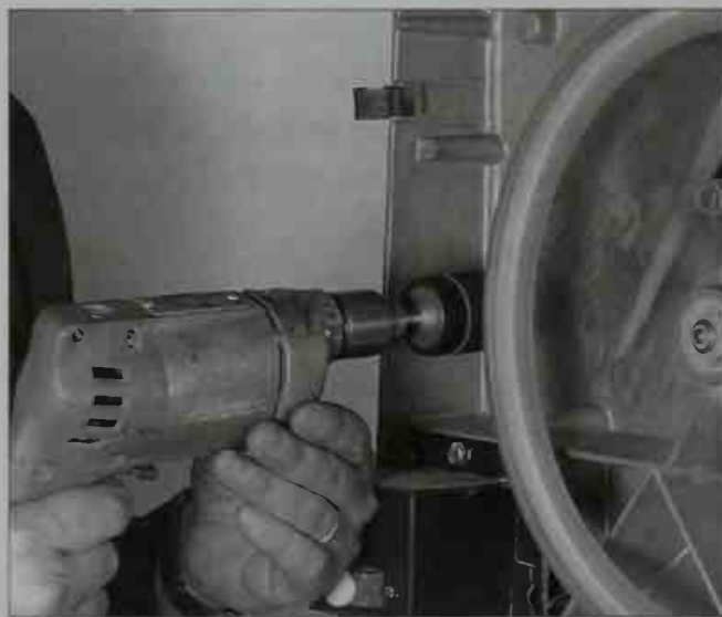
1-15. The top wheel does not have a source of power, so an outside source such as a drill should be used to rotate it. Here a drill is being used with a 1¼-inch sanding drum to rotate the wheel.
