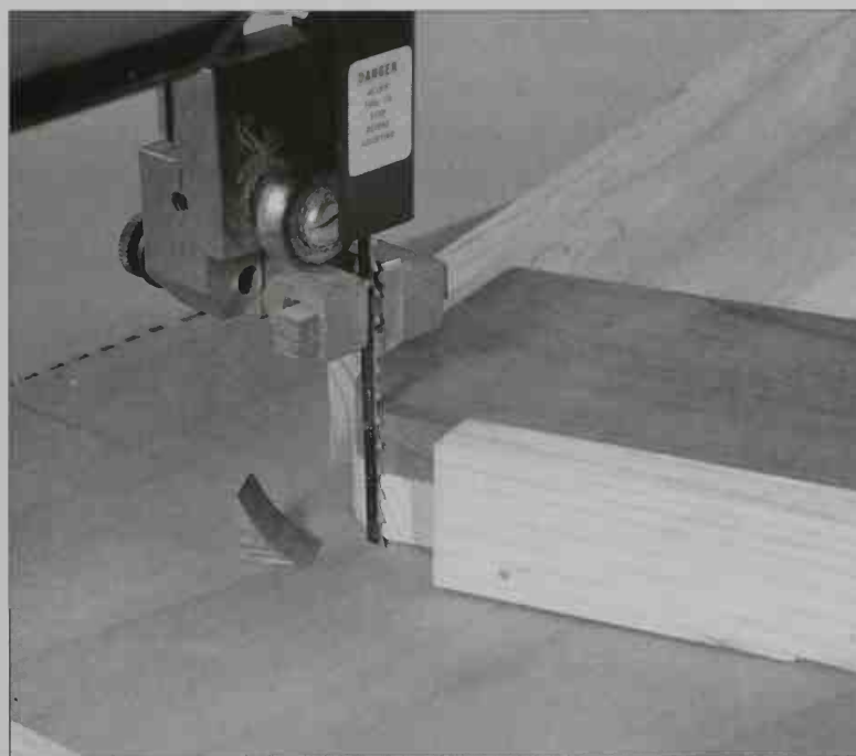
6-27. A quarter-circle jig is made by adding a wood strip to each side. The workpiece is held in the corner of the jig and the cut is made. The cut can be made without the need to measure, mark, or make a hole.
