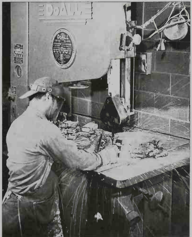
2-14. In friction-sawing, a high blade speed is used to produce heat. This softens the metal and makes it easier to remove with the saw teeth.
