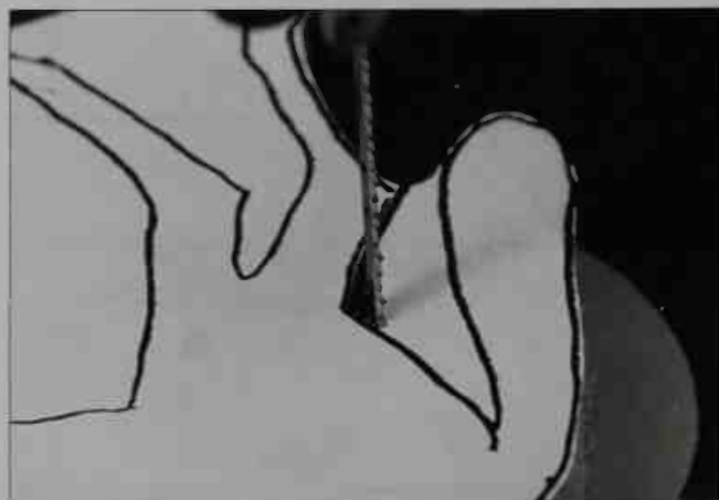
4-18. Next, the workpiece is rotated so that the blade is in line with the pencil line.
