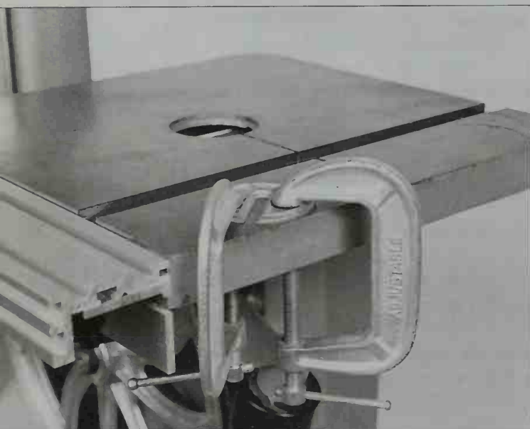
1-29. Straightening a bent table insert. Notice the miter-gauge slot, a feature on most band saws.
