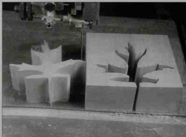
4-28. A \frac{1}{16} -inch band-saw blade cuts much faster than a scroll-saw blade, particularly in thick, hard wood such as the 2-inch-thick hard maple shown here.
