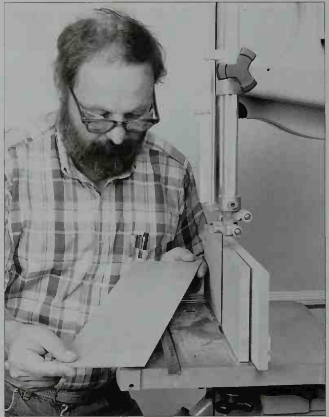
4-58. Proper band-saw alignment, a sharp \frac{1}{2} inch-wide 3 TPI blade, and a slow, steady feed rate yield a uniform piece of veneer.
