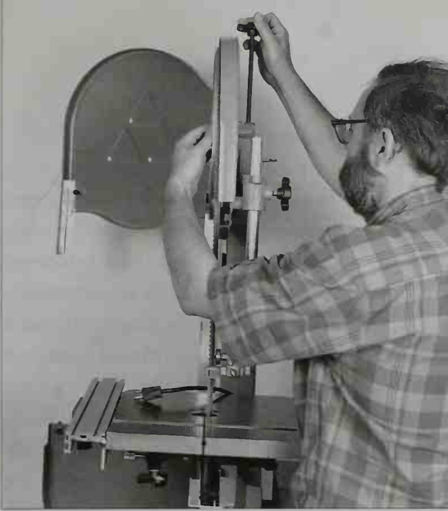
2-22. To apply tension to the blade, adjust the upper wheel assembly upward by turning the knob or hand wheel while simultaneously measuring the tension on the blade.
