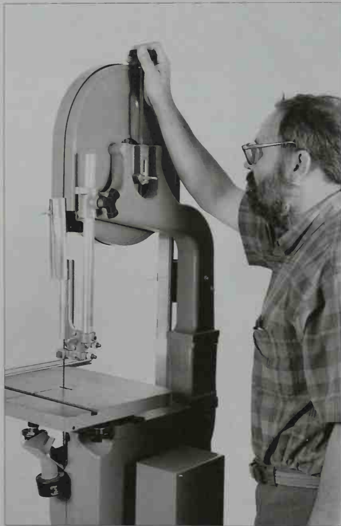
3-15. The top wheel is lowered to release the blade tension.
