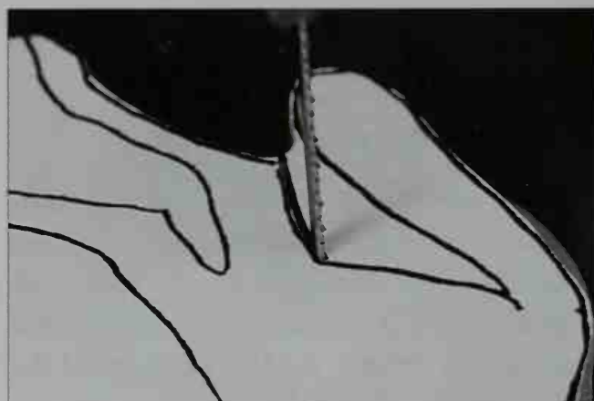
4-17. The corner is too square to allow the blade to rotate, so the first step is to make a straight cut into the corner. Then the workpiece is backed up and multiple cuts the width of the blade are made, as shown here.
