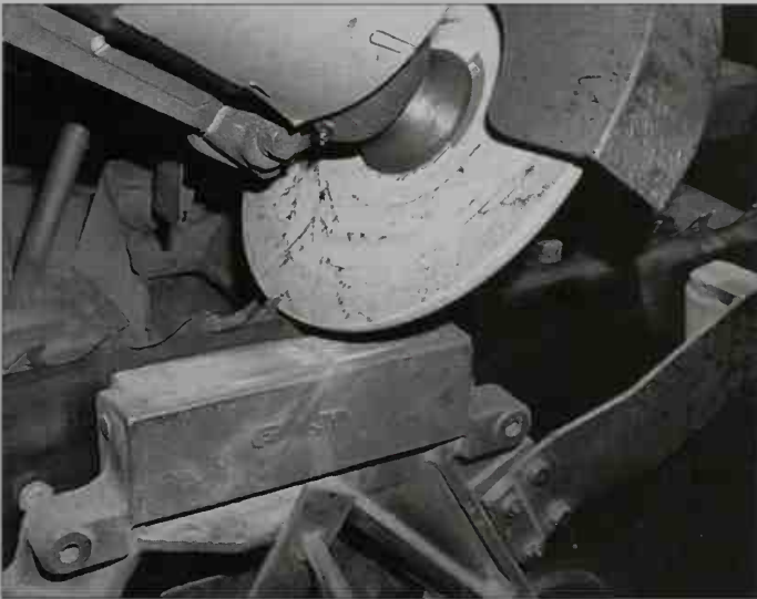
2-48. A 14-inch grinding wheel is being used to sharpen a band-saw-mill blade at Johnson Lumber Company in Charlotte, Michigan. The grinding wheel and the blade movement are coordinated so that the back and the face of the blade are ground.
