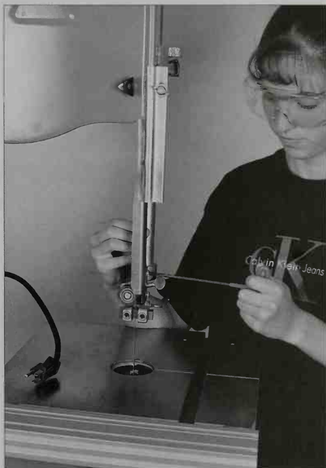
3-13. The blade guard is unscrewed.
