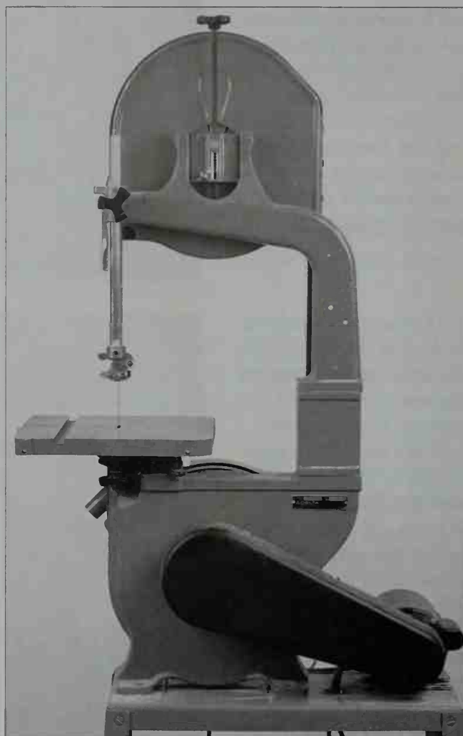
1-21. This Delta 14-inch (14-inch throat capacity) band saw has a skeletal framework, which is either cast or welded to the band saw, and wheel covers.
