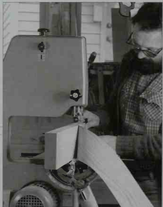
I-5. Resawing oak into veneer with a 3-TPI (teeth per inch) hook-tooth blade. Blades are discussed in Chapter 2.
