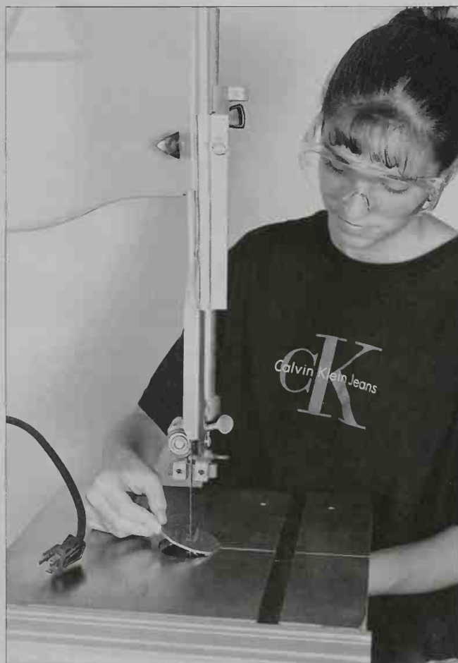
3-14. Next, the throat plate is removed.
