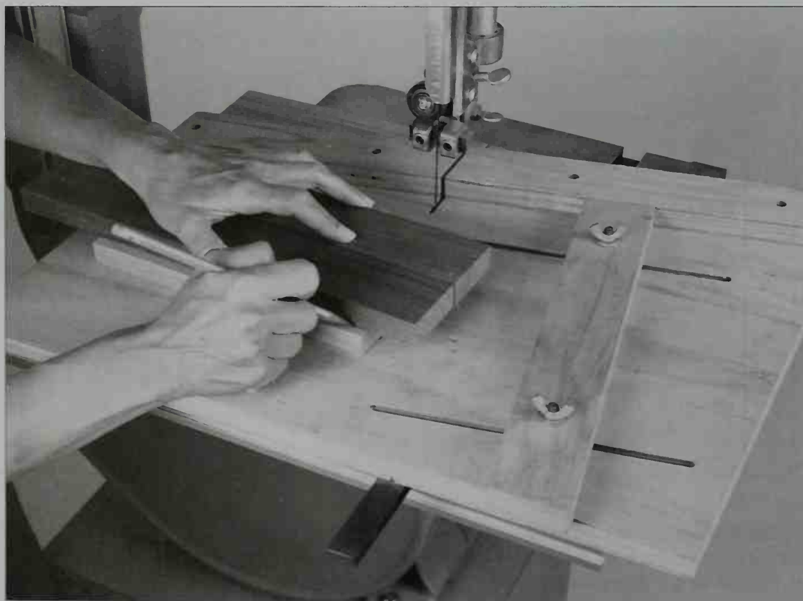
4-81. The blocks are placed on top of the workpiece and a pencil mark is made. This mark represents the difference between the workpiece and the total width of the blocks.
