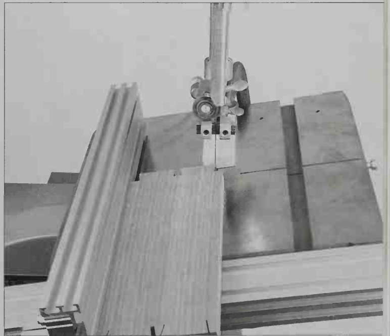
4-93. The second series of cuts are made with the table angled in the opposite direction. The corner of the tail is lined up with the blade.
