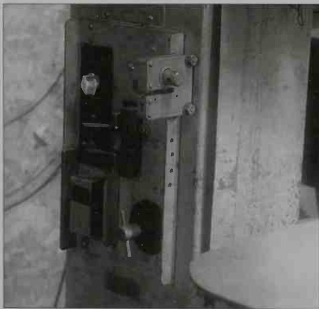
2-38. A close-up of a resistance welder on a metal-cutting band saw. These are the most commonly used welders in industrial and professional shops. They expedite interior-cutting.
