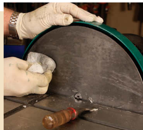
The PSA-backed sanding disks often require a fair amount of scraping to get the paper off, and leave a bit of residue behind. You can remove any adhesive residue with a solvent, such as naphtha.
