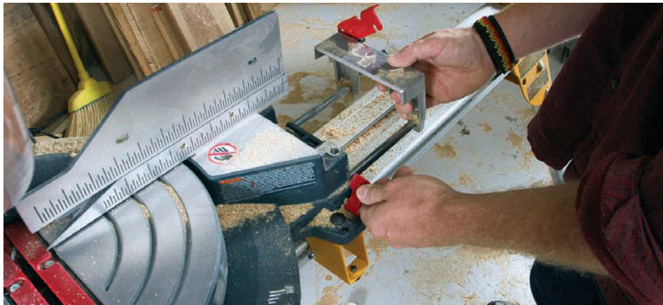
Some saws have slide-out extension wings to help support longer boards. The wings should operate smoothly and be in perfect alignment with the table. Misalignment of extension wings and the fence is a common problem with inexpensive saws.
