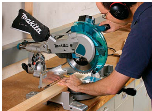
Dual slides. Pairs of top and bottom slides give the 10-in. Makita LS1016L nearly the capacity of a 12-in. sliding model. The maker says the design also improves rigidity for more accurate cuts.
