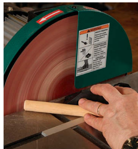
Different approach. With the miter gauge angled, you can chamfer dowels and through-tenons. Just use a light touch.
