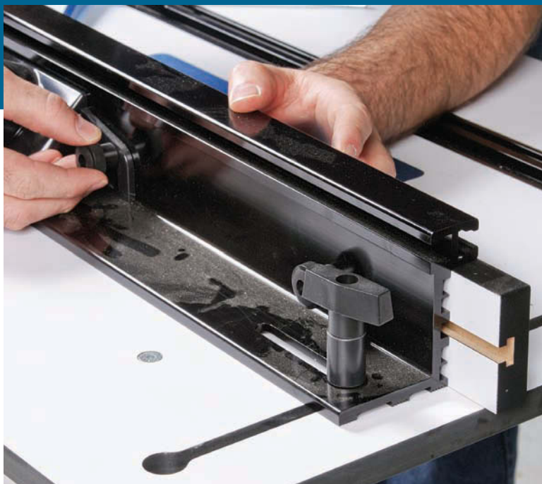
Adjustable fence faces. The opening between fence faces gets changed often to accommodate different-size bits. Look for a fence, like this one on the Rockler table, that lets you make the adjustments without tools.
