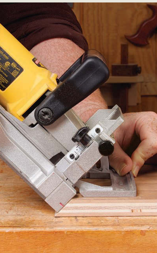
Two ways to slot a miter. The DeWalt fence doesn't adjust past 90^\circ , so to biscuit a standing miter, you angle the fence to 45^\circ and cut the slot with the workpiece clamped flat (left). But workpieces can shift, so it makes sense to slot these parts while they're clamped in a vise (right). The material won't move, and there are no clamps to get in the way, but you need a fence that adjusts to 135^\circ , like that on the Porter-Cable (shown at right).
