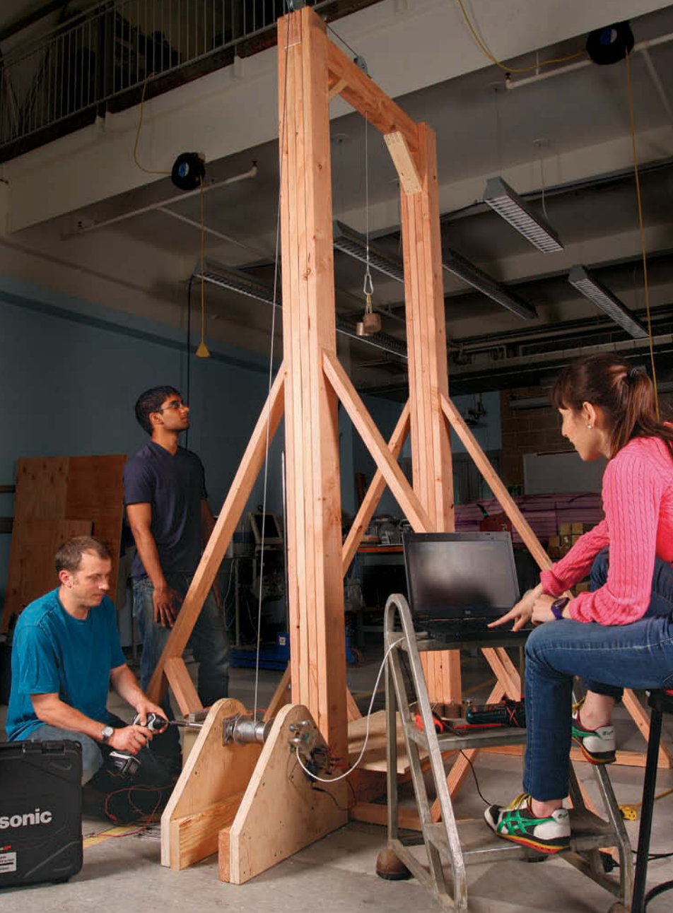
Up she rises. To gauge each drill's sustained torque, Eric Constans and his students built the "guillotine" and used it to see how much weight the tool could lift.
