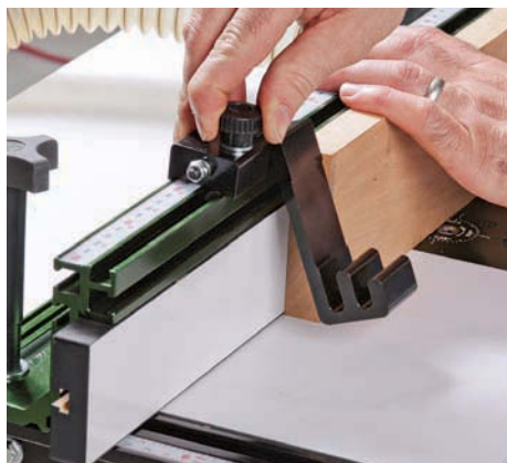
T-tracks make the table more versatile. Use them to attach stops as on the Excalibur (left) and featherboards like on the JessEm (right), which allow you to work more accurately and safely.
