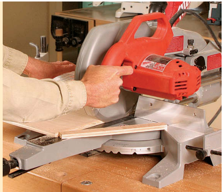
Some saws have slide-out extension wings to help support longer boards. The wings should operate smoothly and be in perfect alignment with the table. Misalignment of extension wings and the fence is a common problem with inexpensive saws.
