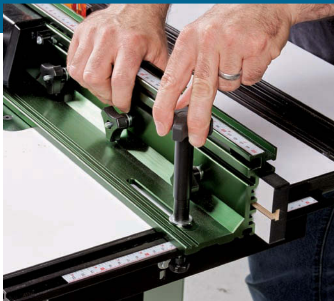
Quick and precise fence adjustments. You shouldn't need tools to move the fence; they only slow things down. A scale on the Excalibur's mounting bracket helps to locate the fence faster.
