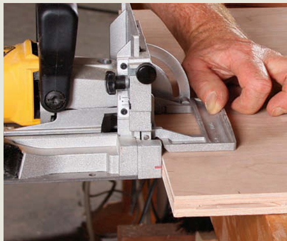
Dial in the height. The DeWalt fence is easy to adjust with a thumbscrew (left), with scales that are easy to read.
