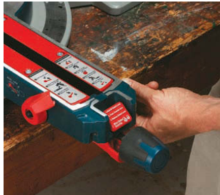
Up-front bevel controls. Rather than a knob or lever at the back of the saw, Bosch's miter saws have the bevel lock at the front. The setup is more convenient and more ergonomic than rear-mounted controls.
