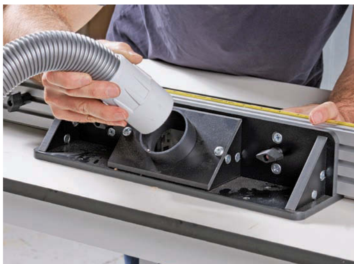
Dust port keeps the table clean. Clearing chips and dust is crucial to a clean, safe cut. All the tables, including this Woodhaven unit, have a port on the fence. Some also have a port on the router enclosure.
