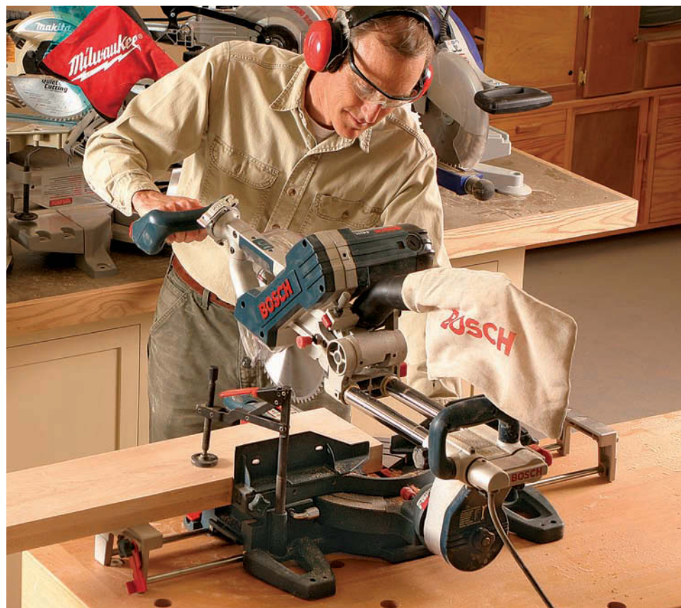
Motor on top. Some saws have the motor mounted above the blade, which allows the saw to bevel through thick stock without the motor getting in the way. It also provides better visibility.
