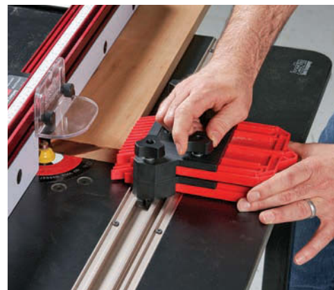
T-tracks make the table more versatile. Use them to attach stops as on the Excalibur (left) and featherboards like on the JessEm (right), which allow you to work more accurately and safely.
