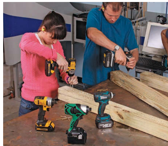
Drive till you drop. To gauge battery life, students measured how many 3-in. screws each driver could sink into pressure-treated pine on a single charge.
