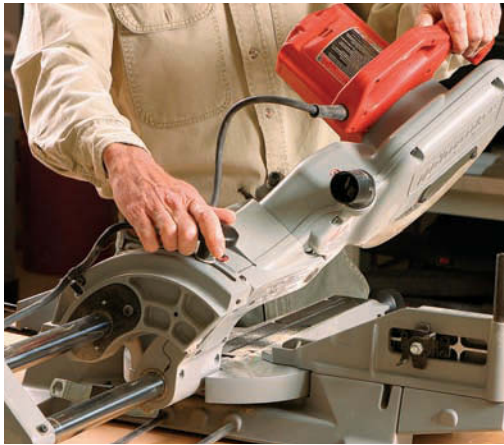
The bevel-angle setting is on the back of most saws. It's a time-tested design, but it can be quite a stretch when making frequent adjustments.
