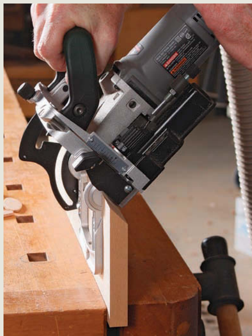
Two ways to slot a miter. The DeWalt fence doesn't adjust past 90^\circ , so to biscuit a standing miter, you angle the fence to 45^\circ and cut the slot with the workpiece clamped flat (left). But workpieces can shift, so it makes sense to slot these parts while they're clamped in a vise (right). The material won't move, and there are no clamps to get in the way, but you need a fence that adjusts to 135^\circ , like that on the Porter-Cable (shown at right).
