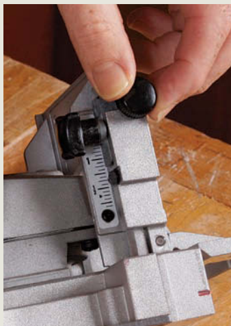
Dial in the height. The DeWalt fence is easy to adjust with a thumbscrew (left), with scales that are easy to read.
