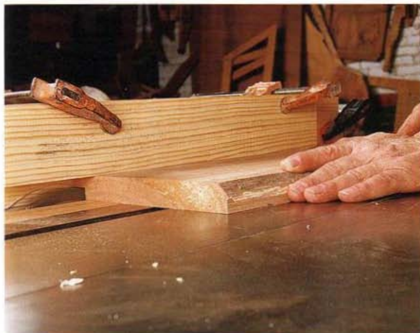
The safest, most accurate way to cut rabbets using a dado head is to clamp a board to the rip fence above the workpiece where it can serve as a hold-down and blade guard.
