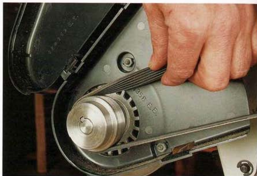
The grooved belt on this Ridgid® saw is more pliable than a typical V-belt and transmits power better.
