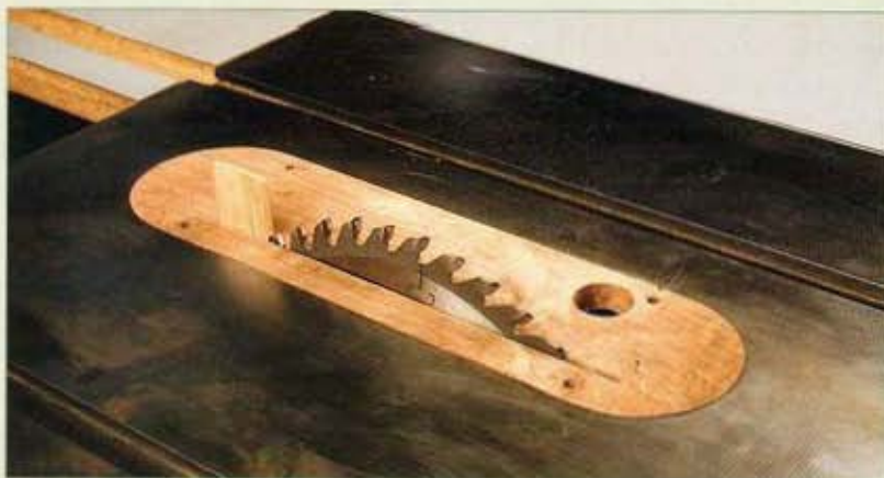
A piece of hardwood glued into the slot in a zero-clearance throat plate serves as a shopmade splitter.
