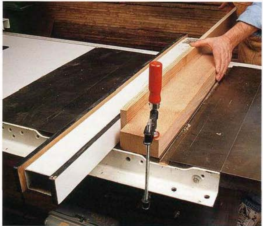
When grooving the edge of a long workpiece for splining, a long board clamped across the saw table will keep the workpiece pressed to the fence for an accurate cut.
