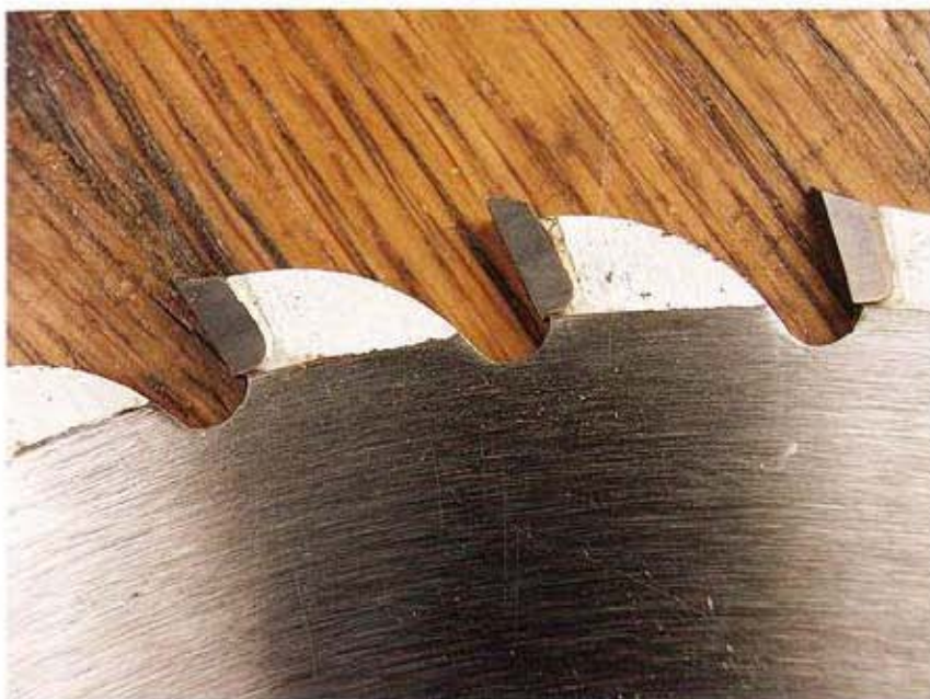
One indication of a premium blade is smooth, nonpitted brazing where the tooth attaches to the plate of the blade.
