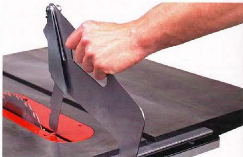
The rear of the Excalibur splitter hooks over a rear-mount assembly, while the front end clicks into a mount inside the saw on the blade carriage.
