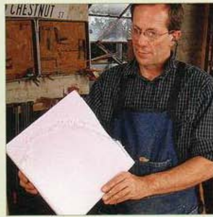
The arched scar on the underside of the workpiece is a result of its travel over the top of the blade.
