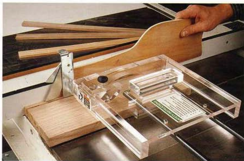
A blade guard and splitter or riving knife are essential table-saw accessories. Using a pusher to feed the wood keeps your hands out of harm's way.
