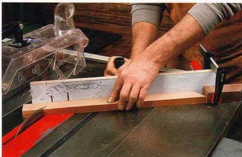
When cutting miters with a miter gauge, use an auxiliary fence and a stop block.
