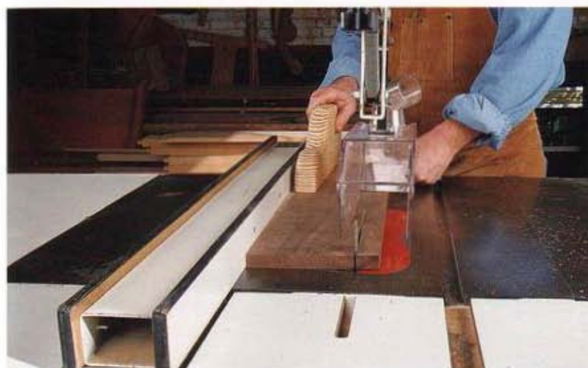
For a typical rip cut, a board's jointed face and edge are pressed against the saw table and fence. The operator stands to the side of the board and finishes the cut using a pusher.
