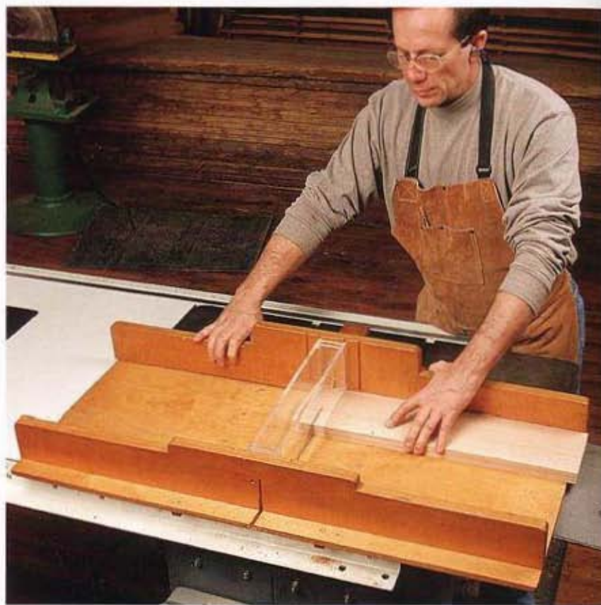
One of the best ways to crosscut a board to length is to use a crosscut sled that slides in your saw's miter-gauge slots. The sled is much more stable and accurate than a stock miter gauge.
