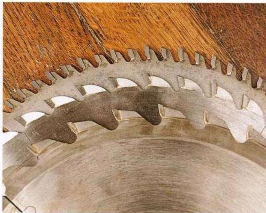
A 24-tooth FTG blade (foreground) serves for fast ripping. A 40-tooth ATB blade (center) does a good job of both ripping and crosscutting. The 80-tooth ATB blade (rear) crosscuts with little or no tearout.
