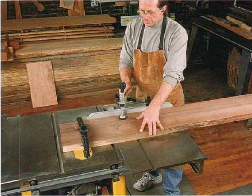
A sliding table—like the one on this DeWalt® 746 saw—allows easy, accurate crosscutting of long, wide, or heavy workpieces.
