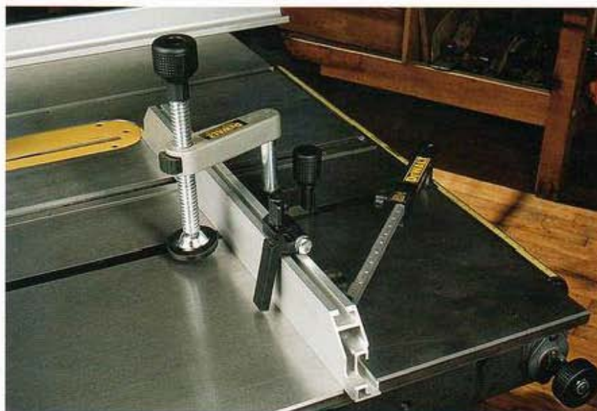
European-style miter gauges include a longer fence for better bearing and integral flip-down stops for repetitive cutting.
