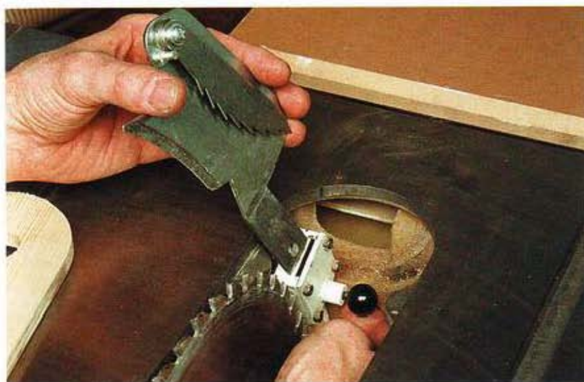
The Biesemeyer splitter snaps easily into its mounting bracket and can be removed by retracting the round knob on the bracket.
