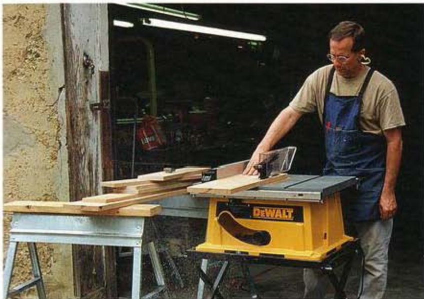
A portable saw can be quickly set up anywhere, making it ideal for job-site work.
