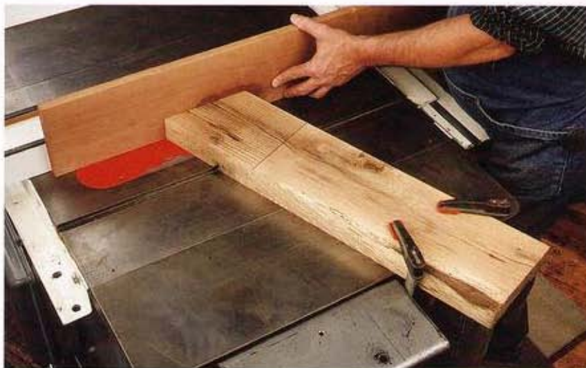
A featherboard applies springlike pressure to hold a workpiece against the fence or table, preventing backward travel at the same time.
