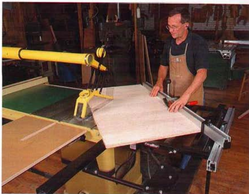
An aftermarket sliding, or rolling, table attaches to the side of a saw, providing increased crosscutting capacity. Although these rolling tables make handling large stock much easier, they are not as accurate as an integral sliding table that comes right up to the sawblade.
