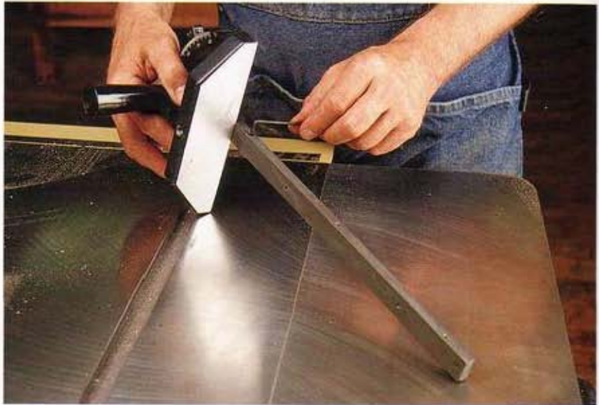
Some miter-gauge bars include Allen screws or other fittings for adjusting the width of the bar to better fit its slot.
