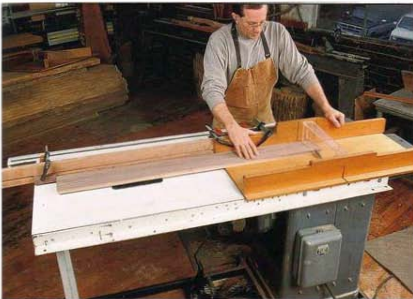
For repetitive cutting of pieces that are longer than the sled fence, clamp an extension board to the fence, then clamp a stop block to the extension board.
