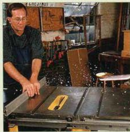
The workpiece is hurled diagonally backward toward the operator.
