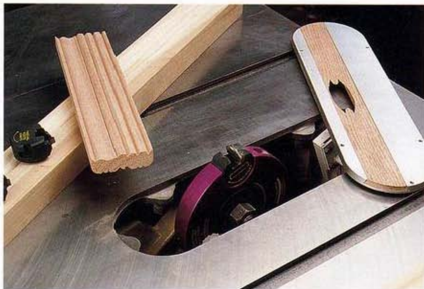
A molding head can be mounted on a saw to shape profiles. The Magic Molder shown here limits the depth of cut to reduce the chance of kickback.
