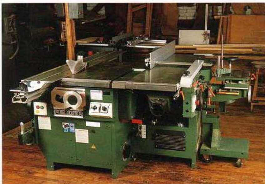
A combination machine offers a table saw, jointer, planer, shaper, and horizontal mortiser all in one relatively compact, high-quality package.
