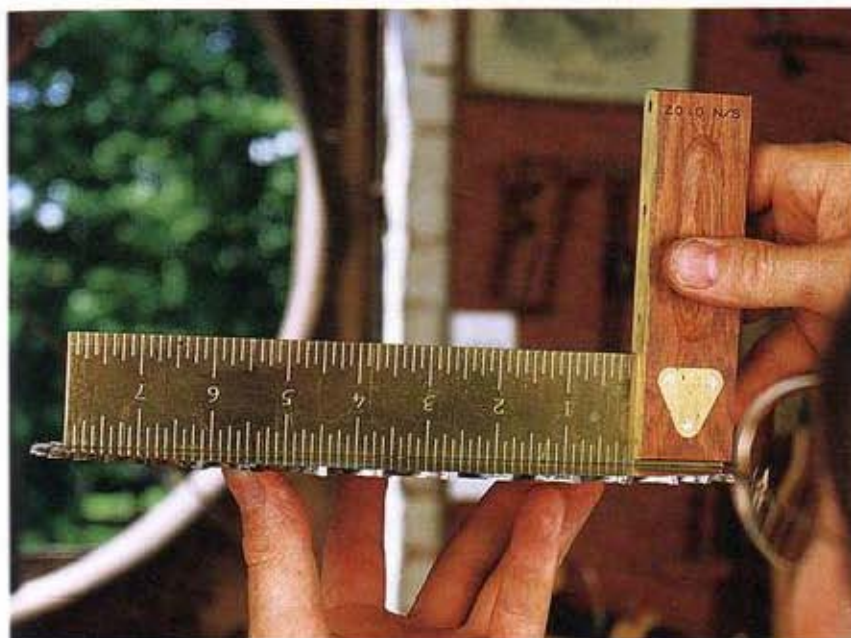
A good straightedge will detect serious warp in a blade.
