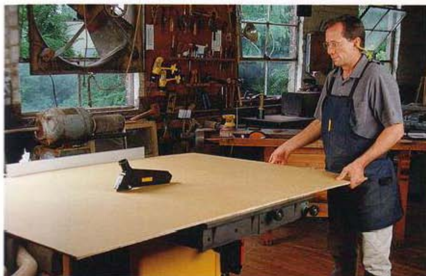
A home-shop saw is well suited to cutting sheet goods as well as most dimensional lumber, although it's underpowered for sawing thick hardwood.
