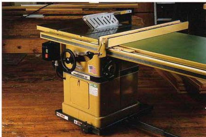
The cabinet saw is the choice of professional woodworkers due to its accuracy, stability, and power.
