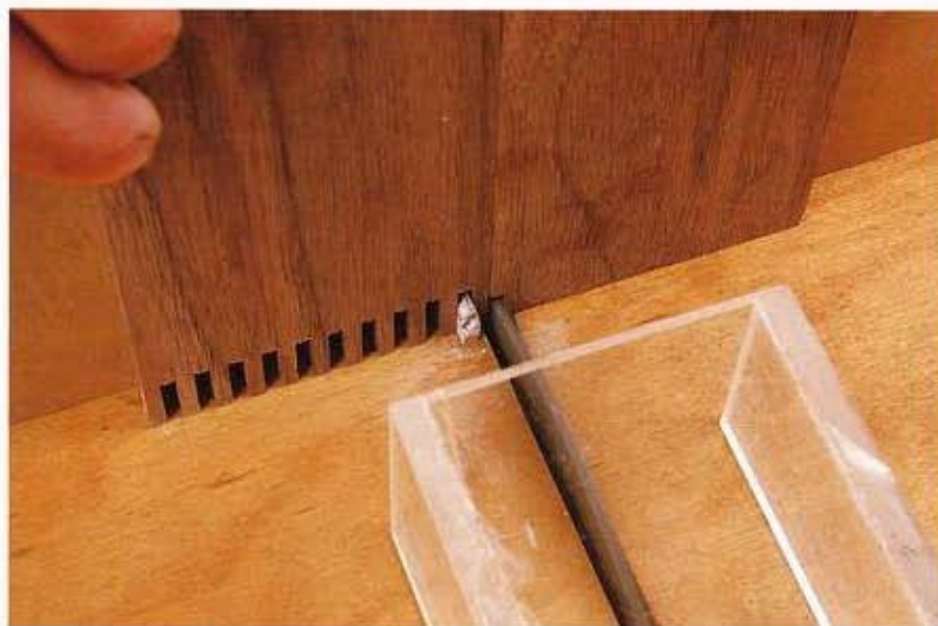
To establish the location of the first slot in the mating board, place the last-cut slot on the first piece over the key, then place the workpiece edges together.
