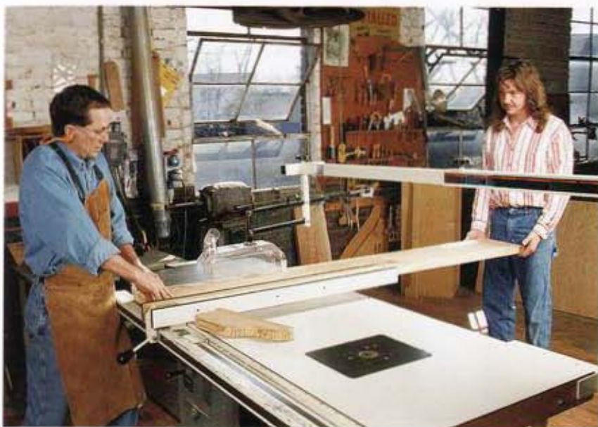
When you are ripping a lot of long stock, using a helper to accept the boards can be very efficient. The helper should never pull or guide a board, but simply support it with palms upraised.
