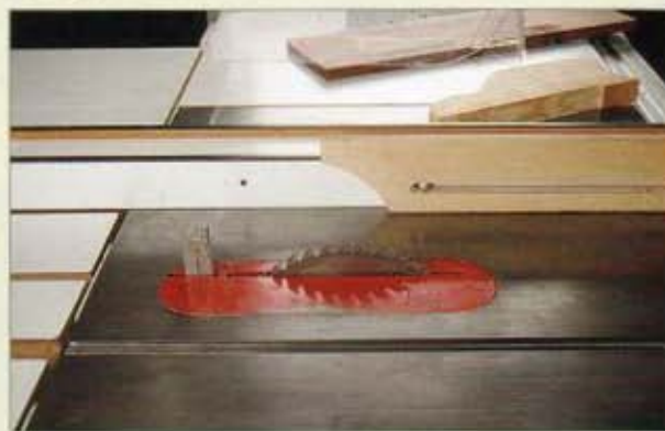
A half-fence, which extends just beyond the cutting edge of the sawblade, allows the workpiece to spread apart after being cut, reducing the risk of kickback.
