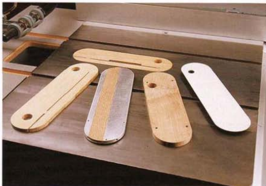
Shopmade or commercial throat inserts provide zero clearance around the blade, making for safer, cleaner cutting.
