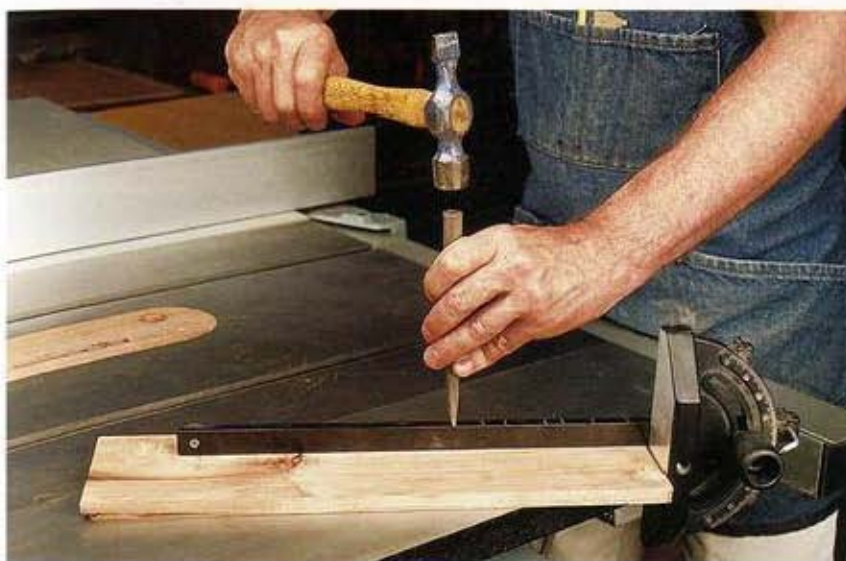
To effectively widen a miter-gauge bar that fits sloppily in its grooves, pound a series of chisel grooves across the edge of the bar.
