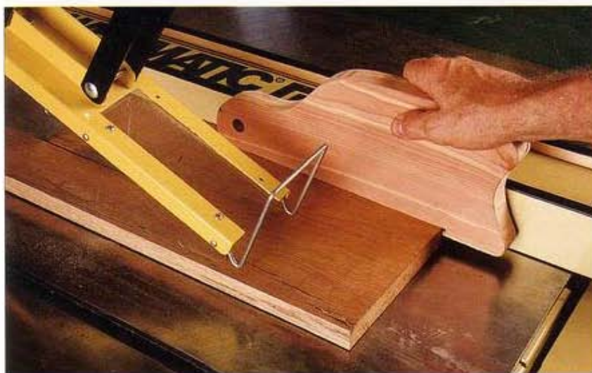
The long sole on a shoe-type pusher provides great bearing and control when ripping.
