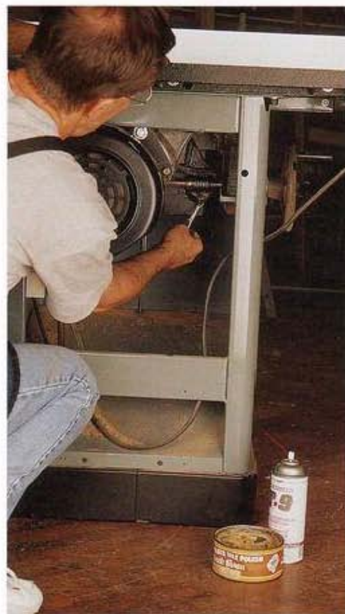
Apply wax to the sector gear teeth using a toothbrush. There's no need to buff it off.
