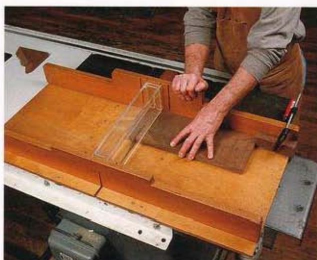
Next, slide the workpiece over against the stop block to crosscut it squarely to final length.
