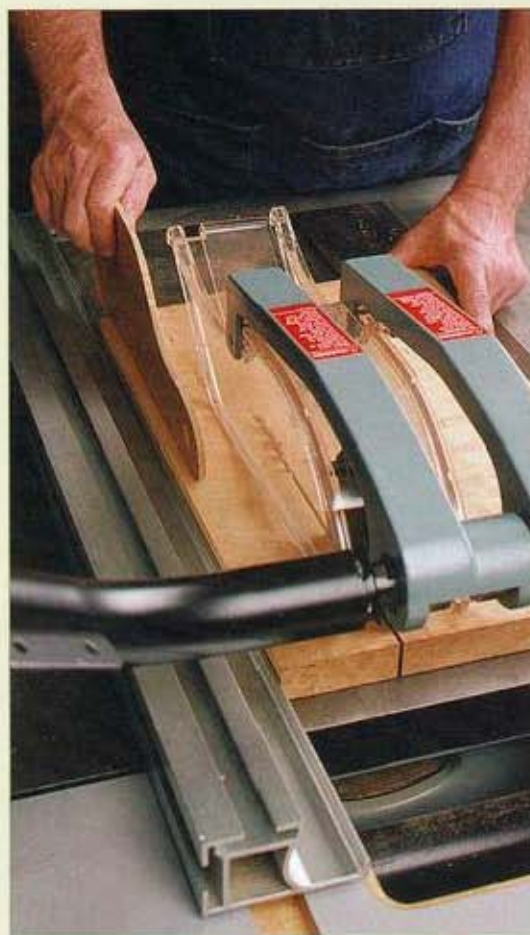
The Delta Unifence, as well as most European-style fences, can be mounted in low position for ripping narrow stock. This provides room to better maneuver your hands and push stick.
