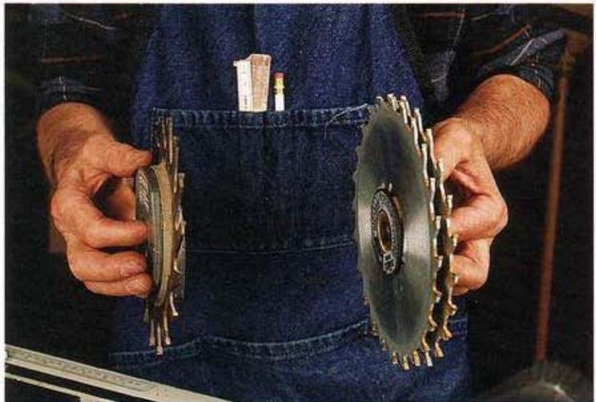
Wobble dadoes that adjust on a hub provide an inexpensive alternative to stack dadoes. The V-dado on the right employs two blades.
