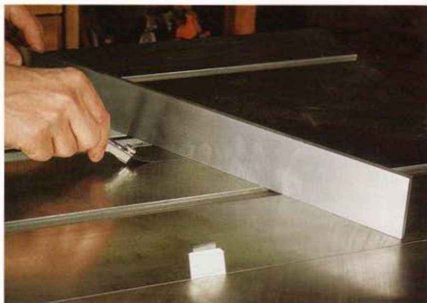
An accurate straightedge placed diagonally across the main table will reveal twist. The low spot between the table's two high corners can be measured with a feeler gauge.
