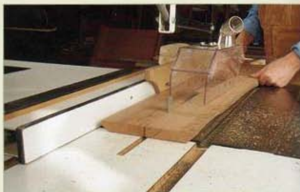
A half-fence, which extends just beyond the cutting edge of the sawblade, allows the workpiece to spread apart after being cut, reducing the risk of kickback.
