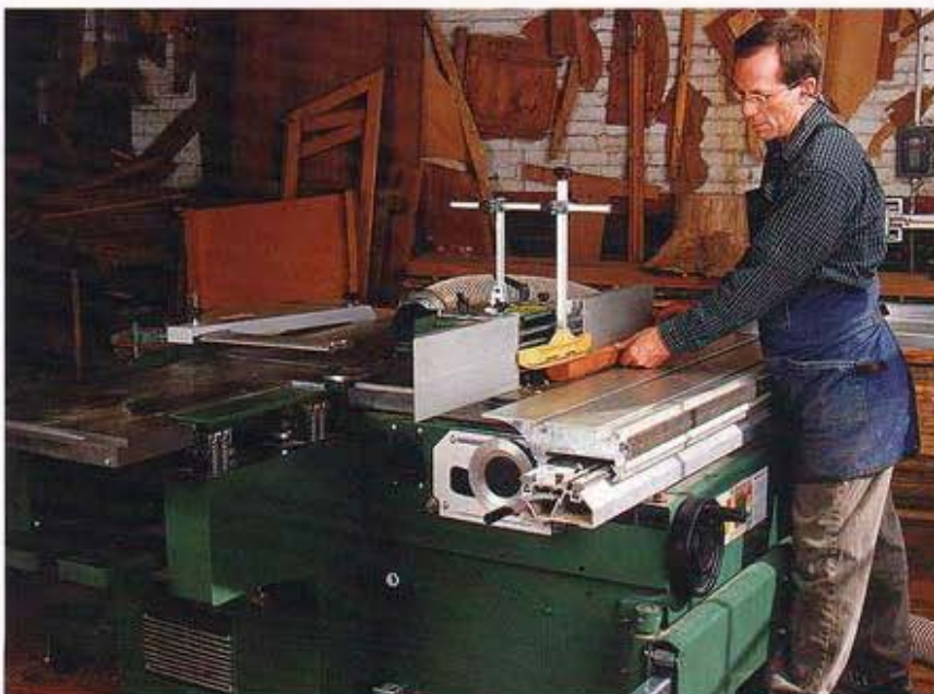
A fully outfitted combination machine combines a table saw, a shaper, and a jointer/planer all in one space-saving package.
