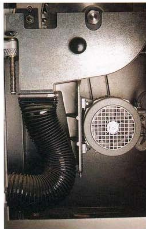
Dust collection on European saws, such as the Inca saw shown here, incorporates a ported blade shroud that connects to a dust collector via a hose.
