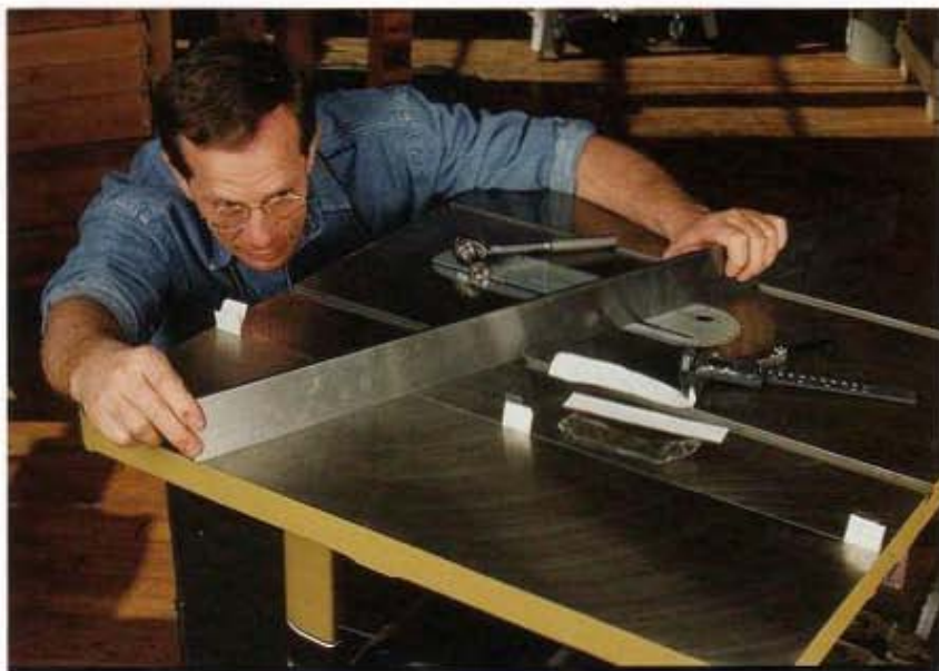
Use a long straightedge and shims to set the extension wings level and flush to the main table.
