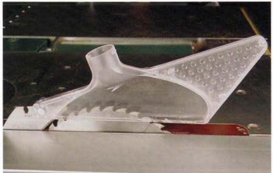
The typical European blade cover removes easily for blade changes and includes a dust port. The riving knife maintains its relationship to the blade regardless of blade angle or height.
