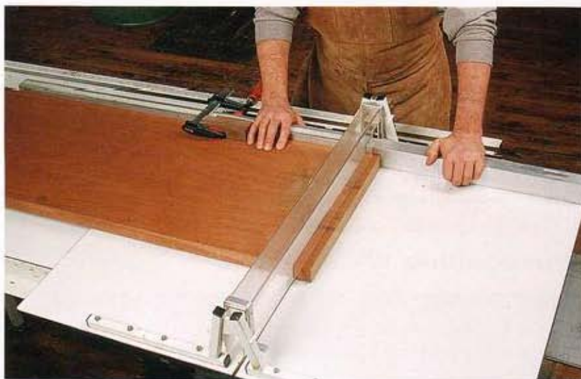
You can crosscut wide panels using a large sled. A wood block clamped to the fence holds long boards down against the base of the sled.
