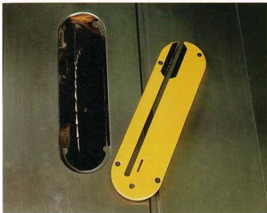
The leveling screws in a throat plate allow for adjusting its height level to the tabletop.
