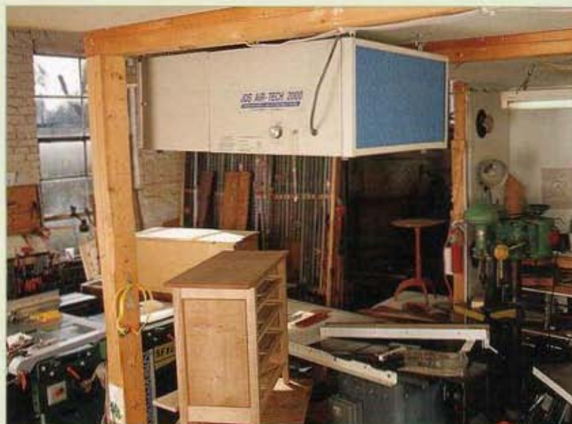
An ambient air cleaner filters from the shop air the very fine dust that is most harmful to the lungs.
