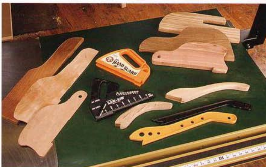
Pushers can be bought or made in various shapes to suit particular ripping tasks.
