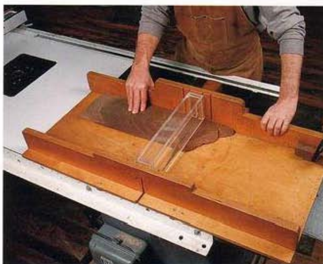
For repetitive crosscutting using a crosscut sled, first square one end of the workpiece from the right side of the sled.
