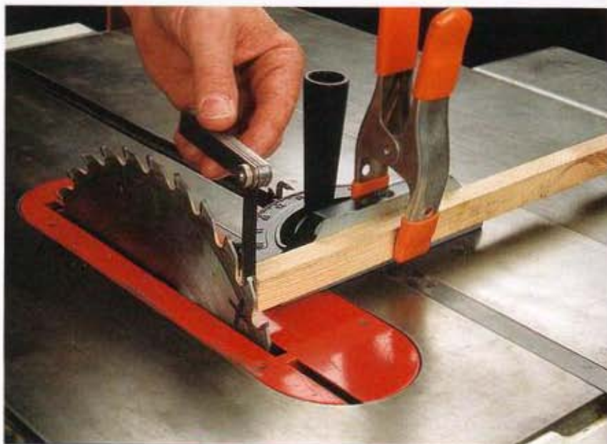
If you don't have a dial indicator, you can use a feeler gauge to measure the distance between the blade and a piece of wood clamped to a miter gauge.
