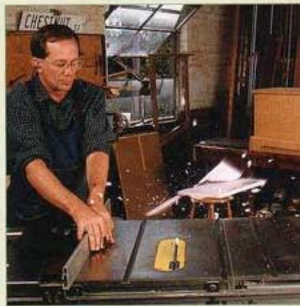
As the workpiece is lifted by the rising rear teeth of the blade, it climbs over the top of the blade, traveling backward.
