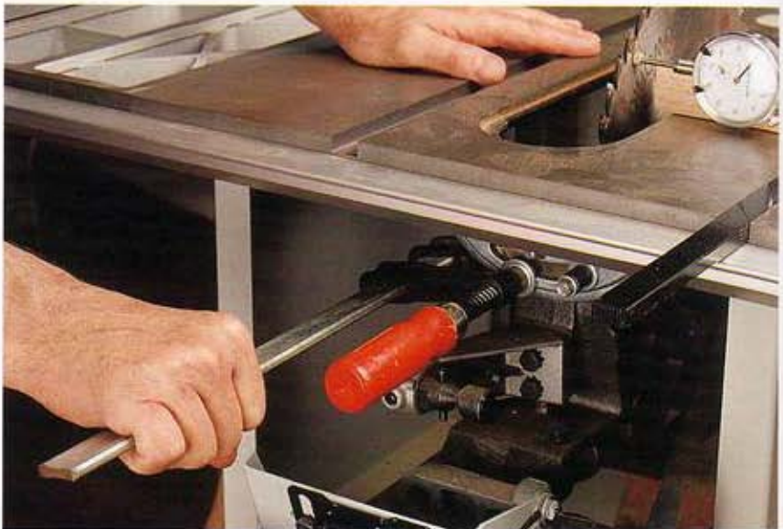
A dial indicator provides an immediate readout for adjusting the blade parallel to the miter groove. A bar clamp locked onto the rear trunnions provides a lever for easy adjustment of the trunnion position.
