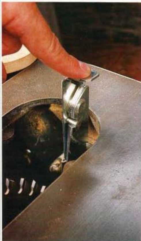
The Delta Disappearing Splitter can be pushed down under the throat plate for non-through-cutting operations such as grooving and rabbeting.
