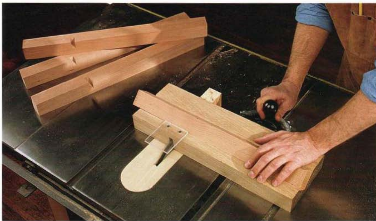
A V-block jig holds the workpiece for cutting a corner dado.
