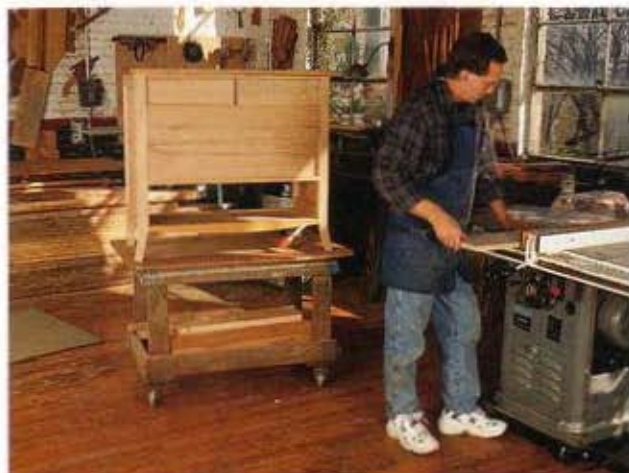
Wheeled carts can conveniently ferry workpieces and work in process from machine to machine. A cart can also serve as an extension table when needed.
