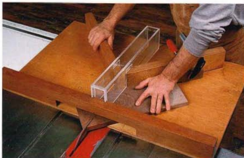
The best way to cut 45-degree miters is to use a crosscut sled with two fences that are perpendicular to each other and angled at 45 degrees to the blade. A cutout in the sled's rear rail allows you to miter wide workpieces.
