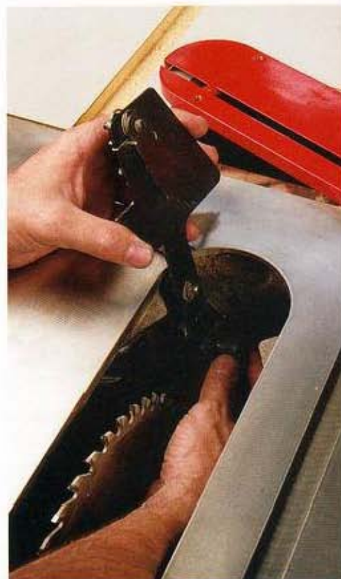
The Delta Deluxe UniGuard Splitter is clamped in place with a threaded knob, which also allows you to remove it for non-through-cutting operations.
