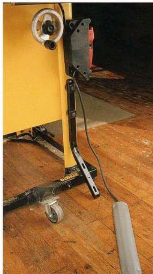
A cord cover prevents tripping over cords snaking across the floor to the table saw.
