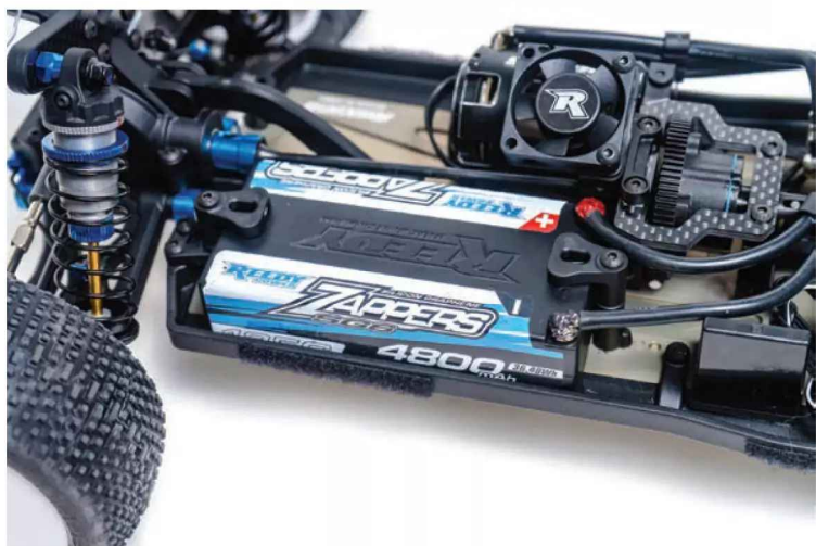
Just like the rest of the car, the battery bay is fully adjustable, allowing you to move the battery fore/aft to change the weight distribution.
