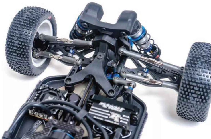
The front plastic upper chassis brace helps to keep the front end stiff. Note the durable 3.5mm turnbuckle and ballcaps.
