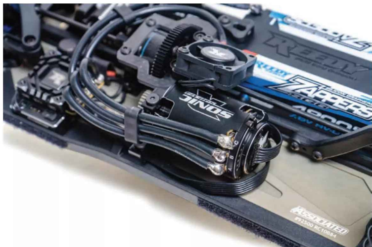
The aluminum motor mount makes it easy to change motors and adjust the gear mesh quickly and accurately.
