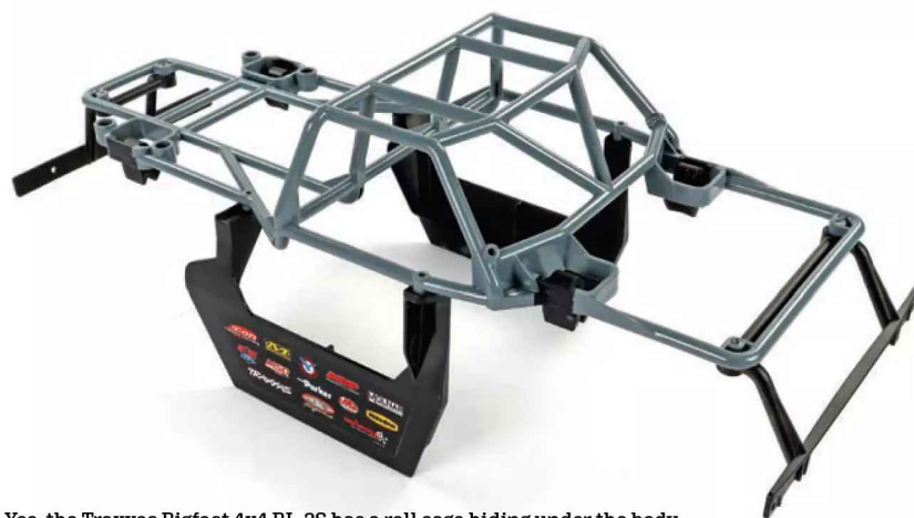
Yes, the Traxxas Bigfoot 4x4 BL-2S has a roll cage hiding under the body. I painted the top portion gray to make it easier to see.
