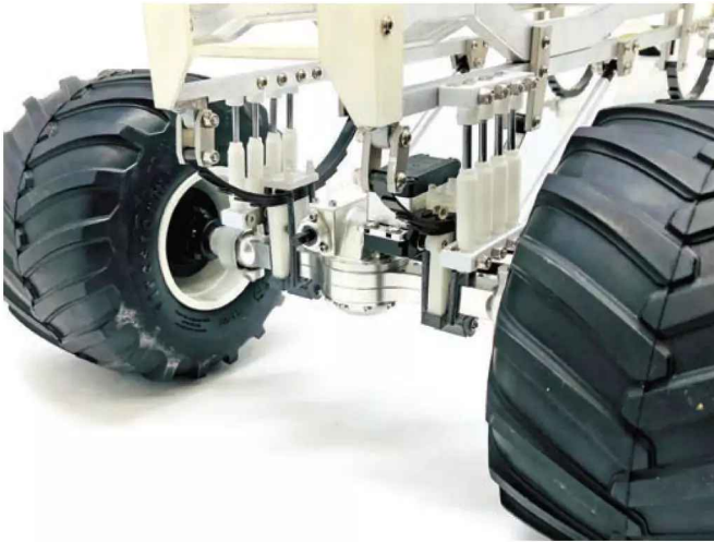
If the suspension doesn't move, there's no need for a functioning shock. I designed some 3D-printed units that look the part.
