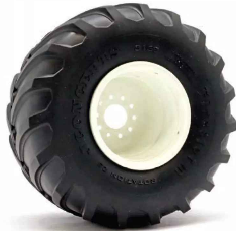
Tamiya Clod Buster wheels were modified to work with the scale drum brakes that I have on the axles, and the bolt pattern was drilled using a 3D-printed guide. JConcepts Firestorm tires complete the look.
