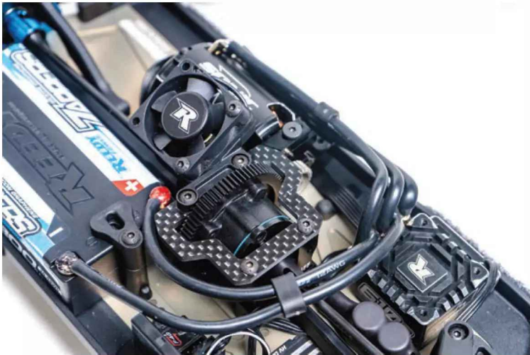
The center differential is housed between two aluminum bulkheads with a carbon fiber top plate.
