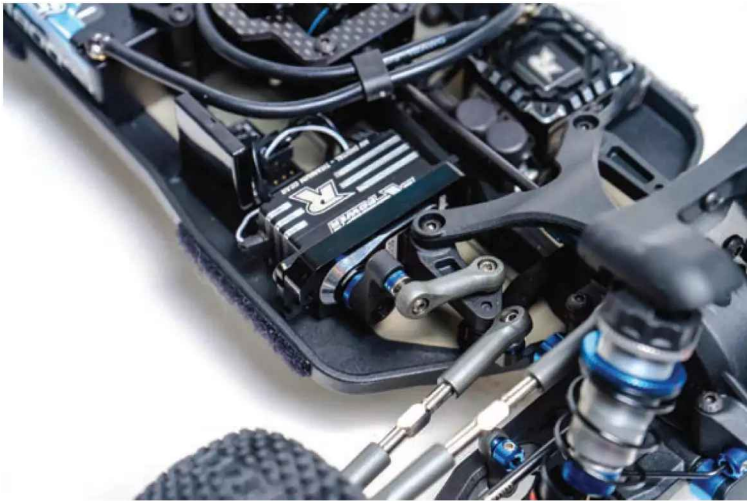
The steering servo bolts onto an aluminum floating mount that incorporates into the front chassis brace.
