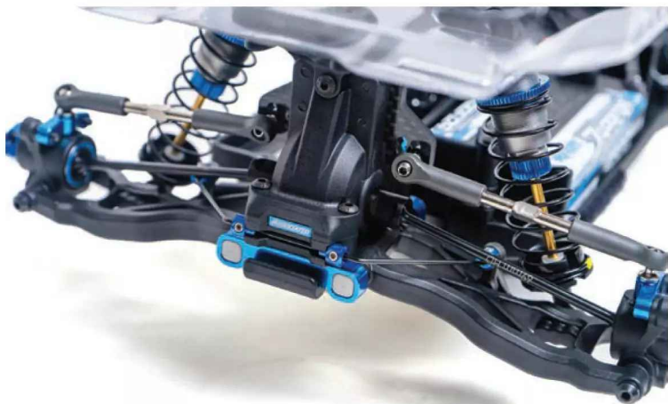
The all-new sway bar system helps to keep chassis roll to a minimum on the track while allowing quick changes in the pits.
