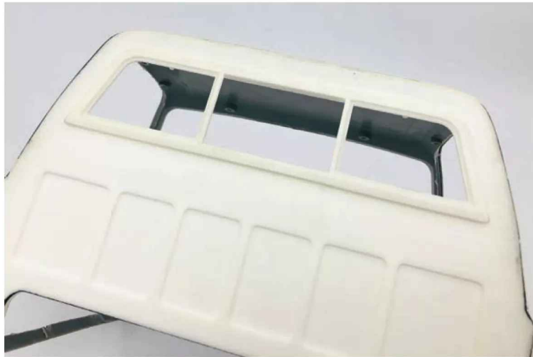
I designed the back cover for the cab and had it 3D printed. A functional sliding rear window was incorporated to add more realism.
