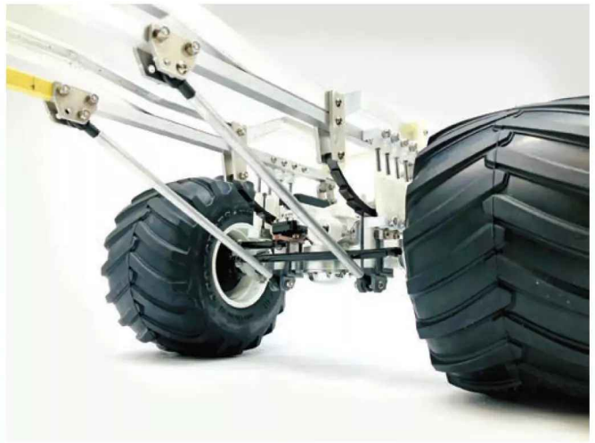
I designed and made the front and rear axle supports to look like the ones on the full-size truck.
