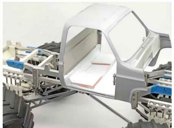
The entire floor/firewall was built by cutting up sheets of polystyrene and gluing it all together. Some adjustments will have to be made once the engine finds its final resting place.
