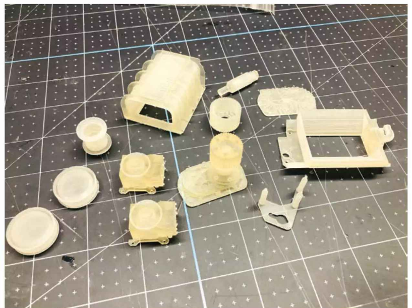
I modified the RC4WD engine to make it look more like a blown monster truck engine by designing some 3D-printed parts and painting the block orange, which looks more realistic than orange anodizing.
