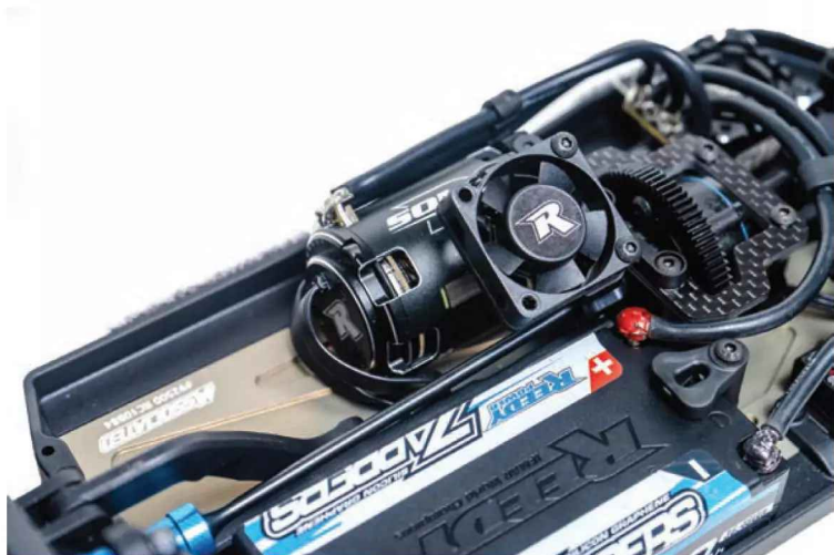
Two mounts are included with the B84D that allow you to mount a 30mm fan above or behind the motor to help cool it effectively.
