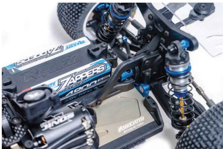
The rear chassis brace has multiple screw mounting points, giving you the option to add or remove screws to alter the rear chassis flex.
