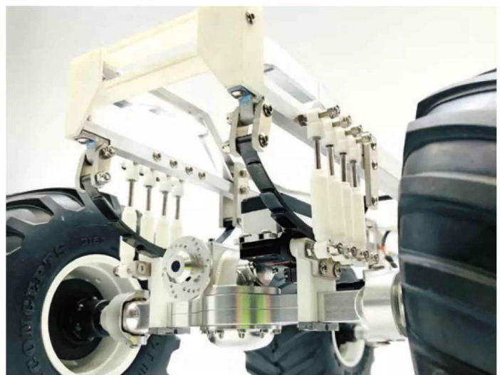
The steering servos are tucked into the axle assembly and mounted using custom mounts. This will hopefully make them less visually distracting once the truck is complete.
