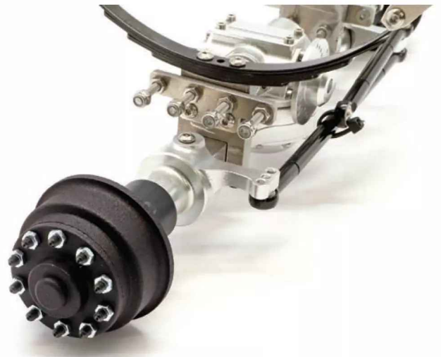
3D-printed brake drums add to the look of the axle assembly, and the scale lugs are used to attach the wheel to it.
