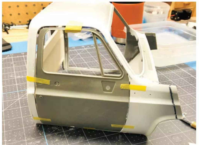
The edges of the doors and the openings are a little rough after the cut, but some sanding sticks and strips of polystyrene make quick work of cleaning them up like factory-issue.
