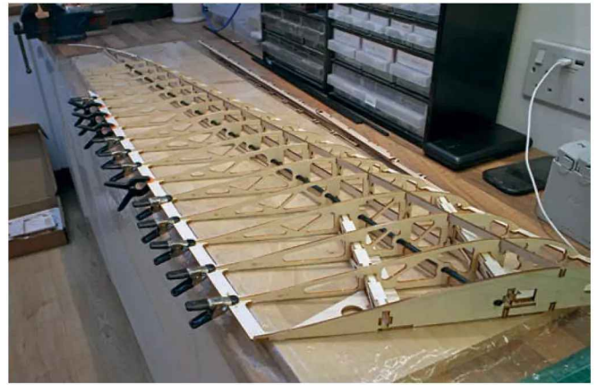
First wing well under way, with the trailing edge being added.
