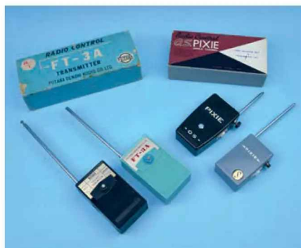
With the advent of transistors, OS and Futaba produced some very small, almost palm sized transmitters. They set the standard for what could be achieved.
