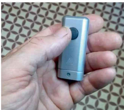
Phil Green's own designed 'Lock Down' micro two channel, full range proportional transmitter.
