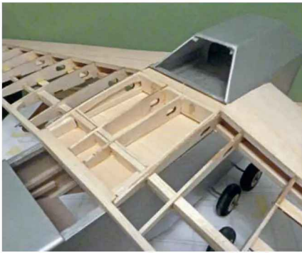
Ensuring correct fit of the wing dowels and clearance around the fuselage.
