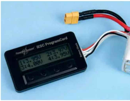
The programming box can also be used as a battery checker.
