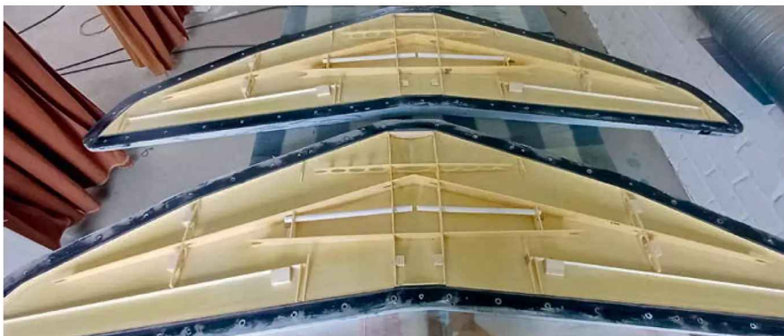
Equinox wing construction. It's a bit scary seeing how little there is inside modern composite wings!
