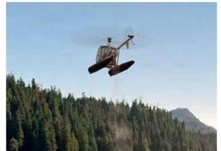
This takes me back! My first helicopter used floats as a training undercarriage.
