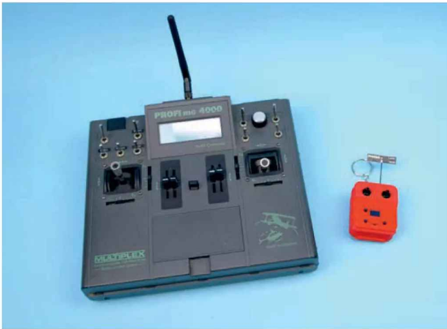
It's hard to believe when sitting next to this Multiplex set but Tobe's latest micro-Tx is full range, fully featured and has eight model memories.
