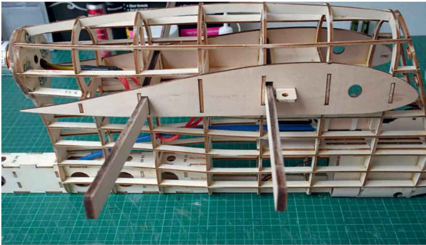
Fuselage almost complete with stringers added.
