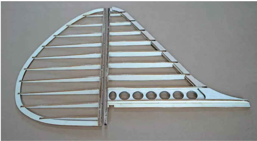
Completed fin and rudder assembly.
