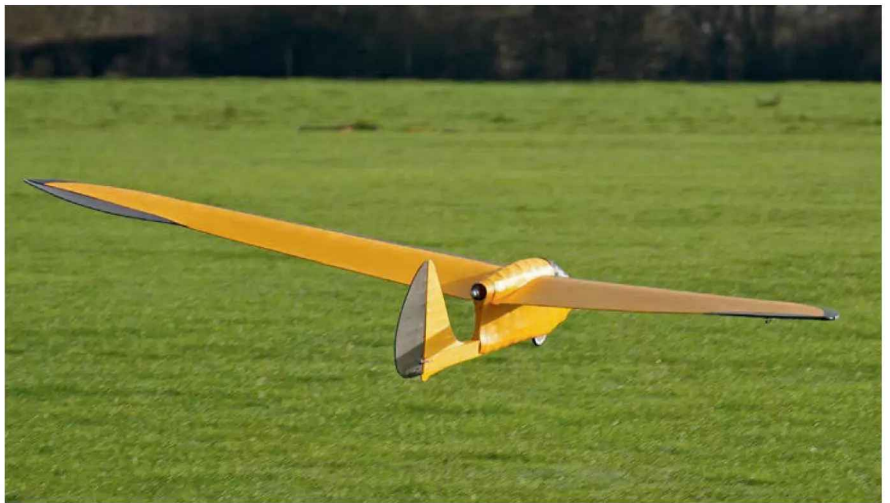
She will rise off ground if assisted during take-off by supporting the rear of the model and keeping the wings level.
