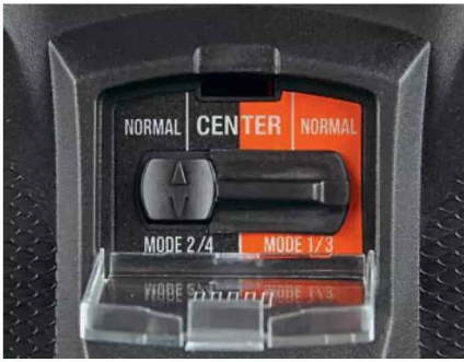
Under a cover on the back of the Interlink's case is a stick mode changing switch.
