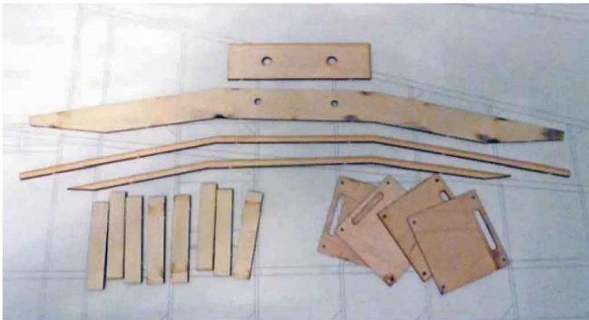
Main wing spars and servo hatch plates.
