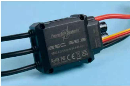
Note the data port. A lead supplied uses this to connect to the Futaba receiver's S.Busz socket.
