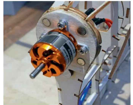
Motor installed on former F1.
