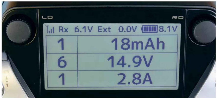
The top screen on my T26SZ transmitter. From the top: consumed current, LiPo pack voltage and real time current draw.
