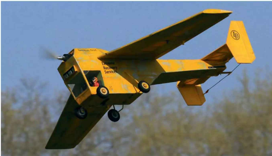
The use of anhedral increases roll sensitivity so be aware until you get a feel for it.
