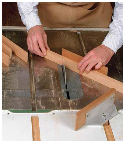
SEPARATE THE SPINNER STOCK. Becksvoort cuts the spinners using a 45° crosscut sled.
