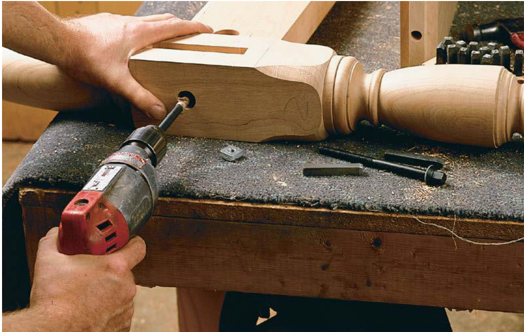
BORING BED-BOLT HOLES. Steve Latta drills through a post into the end of a rail. The post hole is counter-bored for the bed-bolt head.
