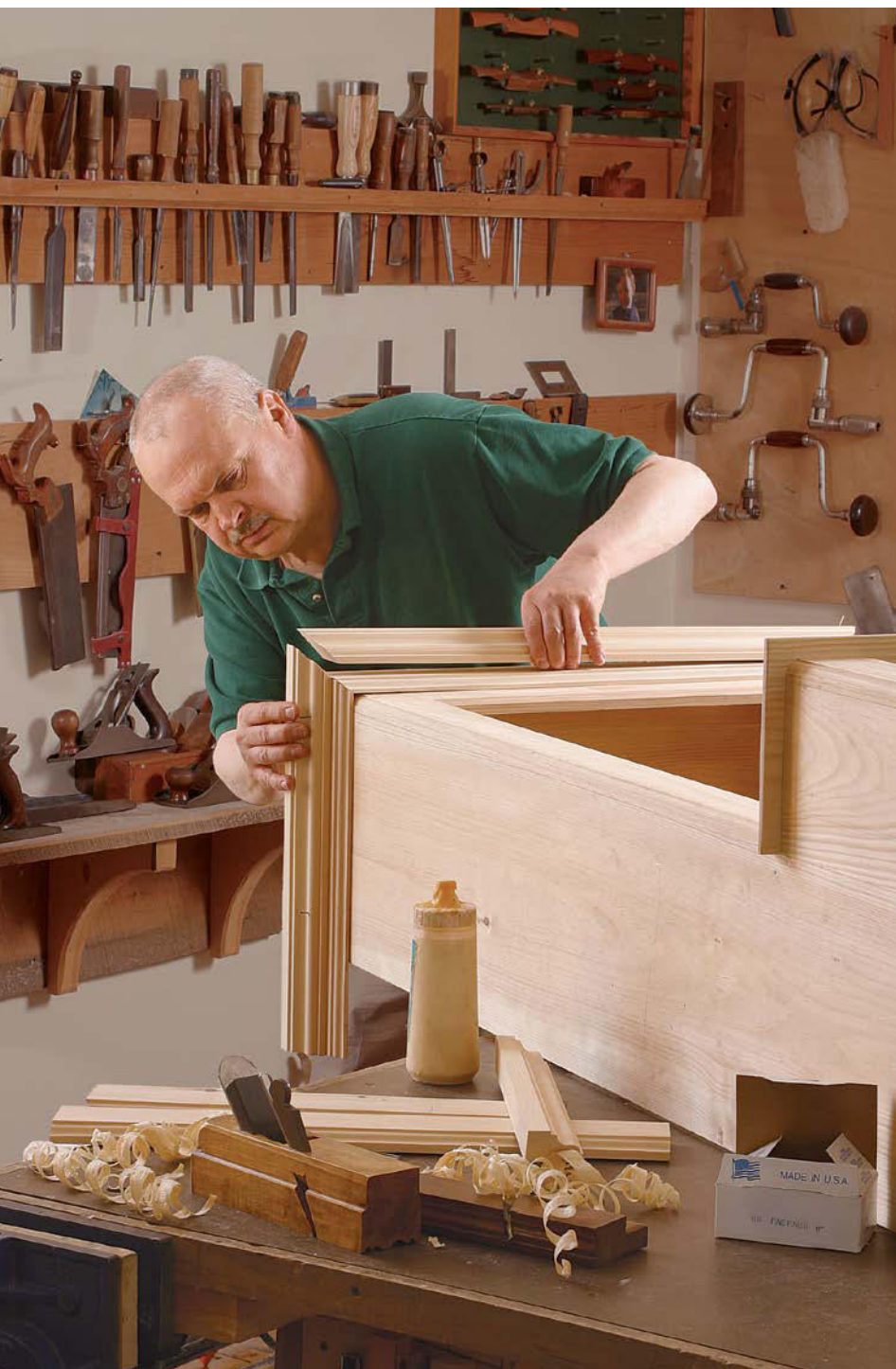
ADD A CORNICE TO THE TOP. The cornice, shaped with a molding plane, is built up from two layers to achieve its pronounced profile.
