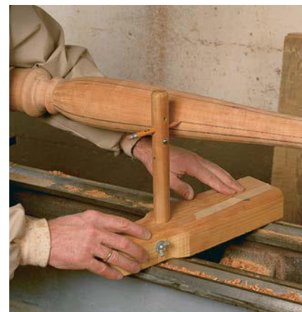
A SCRIBE LAYS OUT EVENLY SPACED REEDS. With a pencil set to the center of the lathe and its base riding on the lathe bed, a scribe accurately draws layout lines for reeds on the top of the bedposts.
