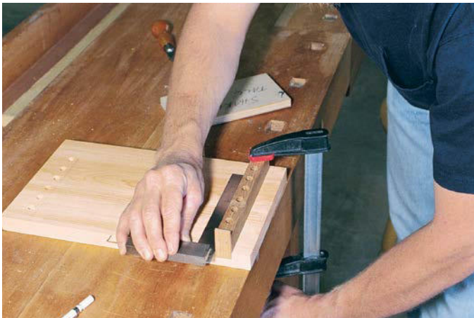
FLIP JIG AND DRILL BOTTOM. The jig, with its fence removed, is flipped over and aligned with layout lines on the case bottom to drill matching holes.
