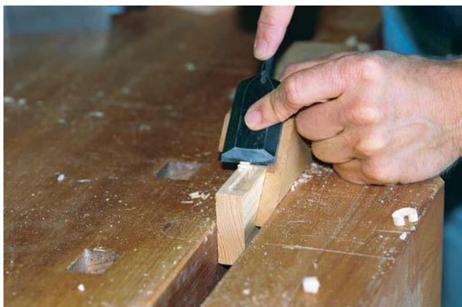
CLAMP AND PARE. With the rabbet cut away at the end of the door stile, the author pares the miter with a sharp chisel. The mitering template is clamped to the stile along the layout line.
