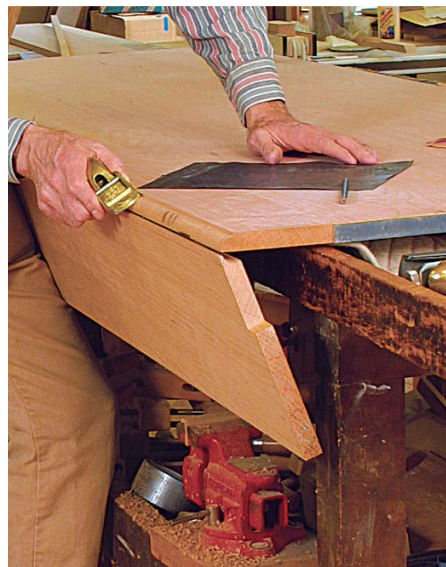
CARBON PAPER STILL HAS A USE. Becksvoort holds carbon paper between the joint as he opens and closes the leaf. Black marks are left where the joint is too tight. Those spots are trimmed with sandpaper or a block plane.
