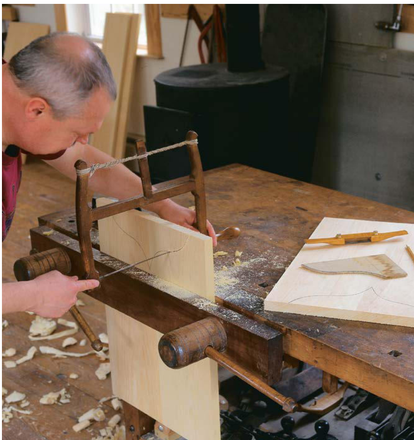
BOWSAWED BOOT JACK. A plywood half pattern, seen on the uncut panel, is used to trace the boot-jack end that forms the blanket chest's feet. If the bowsaw jams in the cut, pop out the waste piece with a chisel blow to the panel's end grain.
