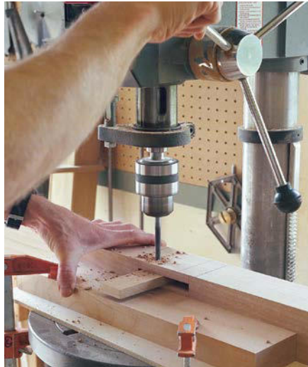
TEMPORARY TENON. A scrap the same thickness as the tenon fills the mortise to prevent tearout as the holes for the pegs are drilled.
