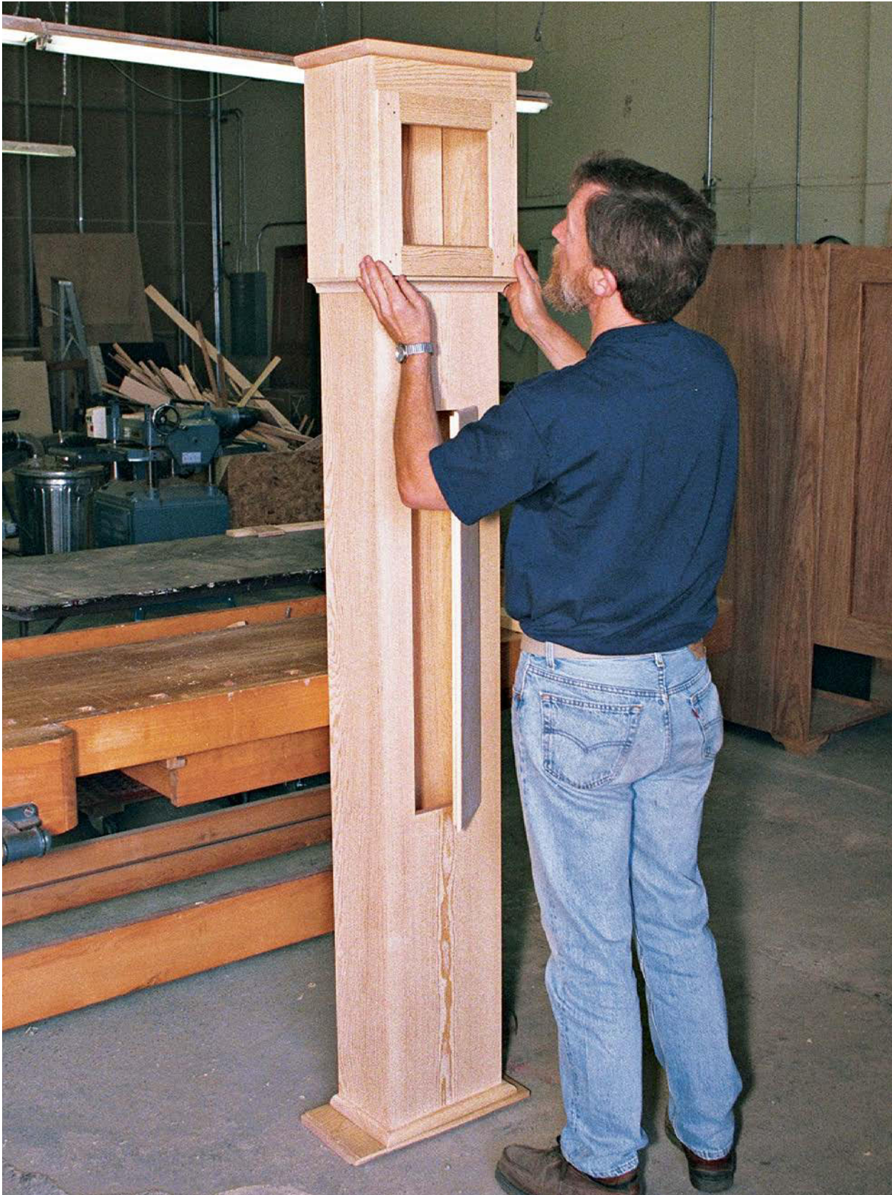
SLIDE-ON BONNET. The bonnet for this Shaker tall clock rests on transitional molding at the top of the case. It slides on and off to provide access to the clock's movement.
