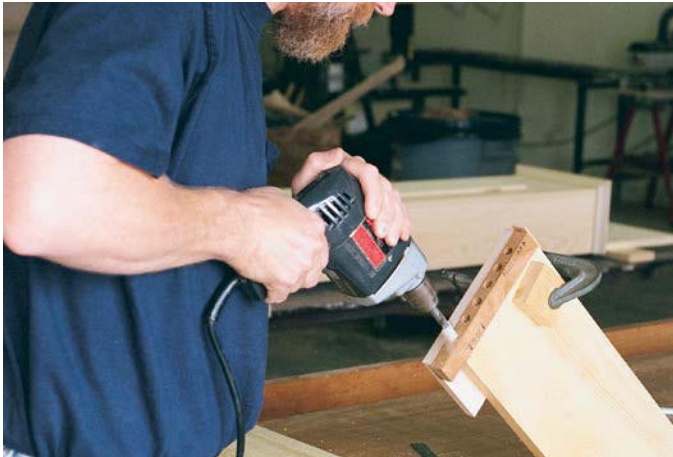
DOWELING JIG. Holes bored in a hardwood scrap guide the bit as the author drills out a case side for glue dowels.
