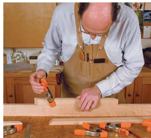
POSITION THE SPINNERS. Starting at the center of the apron, clamp the first spinner in place.
