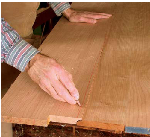
MARK THE CONTACT SPOTS. Set the leaf in place and mark spots where the joint makes contact.
