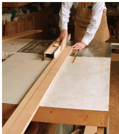
CUT APART THE APRON. At the table-saw, rip the spinner stock from the top edge of the apron.
