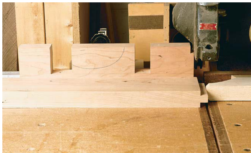
SAWING BED-RAIL TENONS. A 10-in. dado set in the radial-arm saw makes quick work of tenons. To ensure proper registration on bowed rail stock, the authors screwed a spacer block to the left fence (with clearance for the guard), and they shaped the right stop so that it contacts the center of the tenon end.
