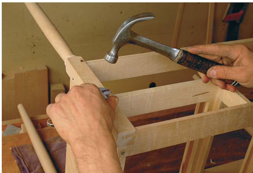
ROSEWOOD PEGS STRENGTHEN THE JOINT, and they add a distinctive touch to the author's table. The adjust- able wrench keeps the pegs properly oriented, parallel to the case's top and sides.
