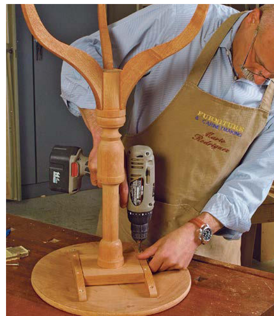
SCREW THE CLEATS TO THE TABLETOP. Slide the cleats onto the round tenons of the pivot block and center the base assembly along the long axis of the tabletop. Attach the catch after the finish has been applied.
