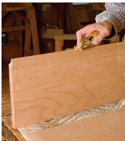
TRIM THE LEAF, not the tabletop. A few passes with a handplane helps achieve an even reveal. Once the joint closes up, rerout the profile on the leaf and try another test fit.
