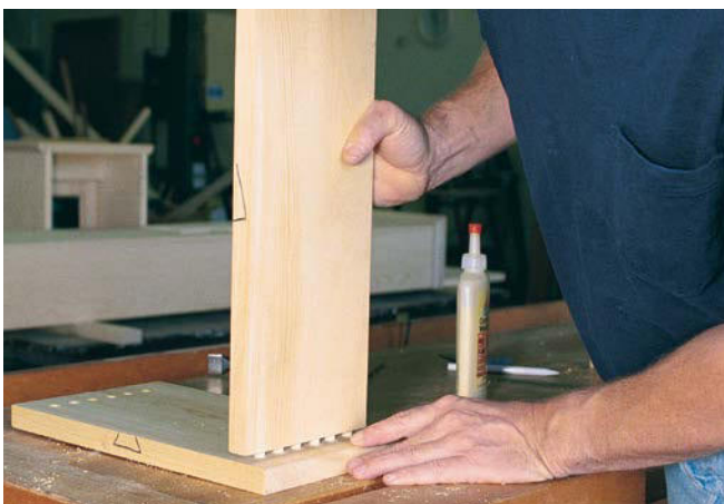
TEST-FIT. The jig ensures that dowels line up correctly, even if guide holes are not perfectly spaced or centered.
