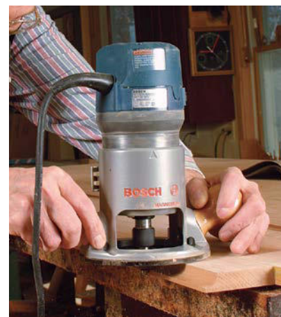
TRIM THE LEAF, not the tabletop. A few passes with a handplane helps achieve an even reveal. Once the joint closes up, rerout the profile on the leaf and try another test fit.
