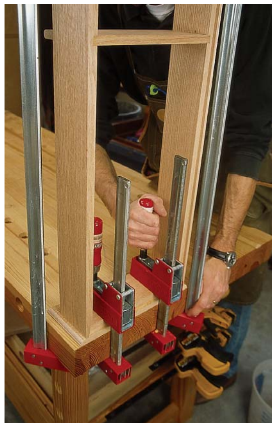
Above, you can see how a couple of well-placed nails keep everything in line as I apply the clamps. Whenever you can, use your bench to assist your clamping (right). It helps spread clamping pressure over a wider area.
