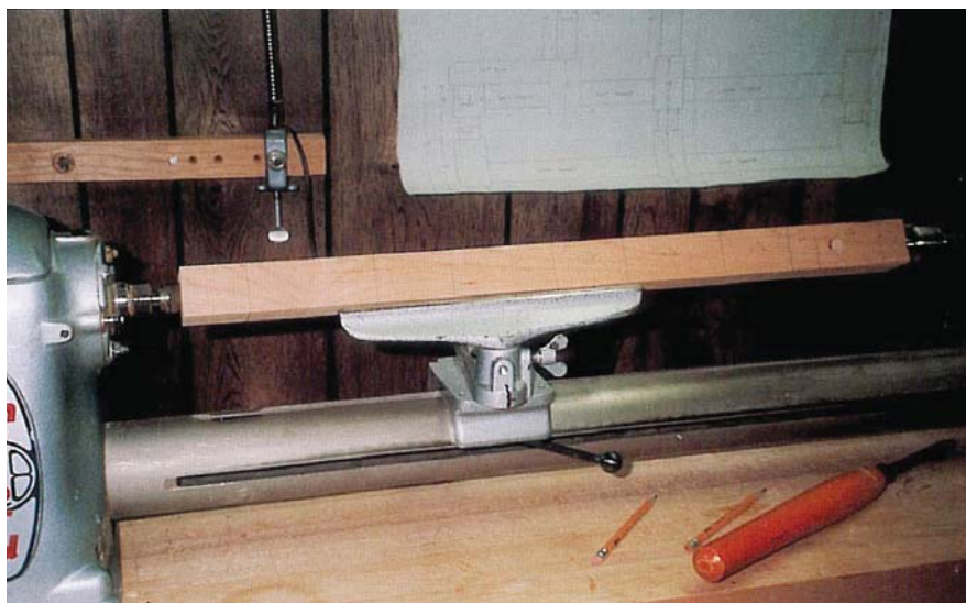
1 Mount the upper post blank on your lathe with all the dimensions marked.
