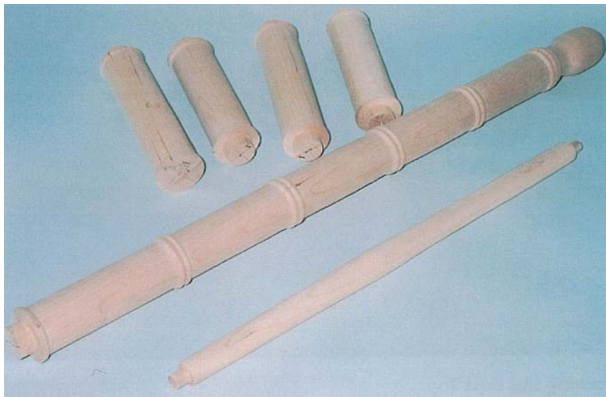
6 The completed rear post with mounted end ball, spacers and stretcher.
