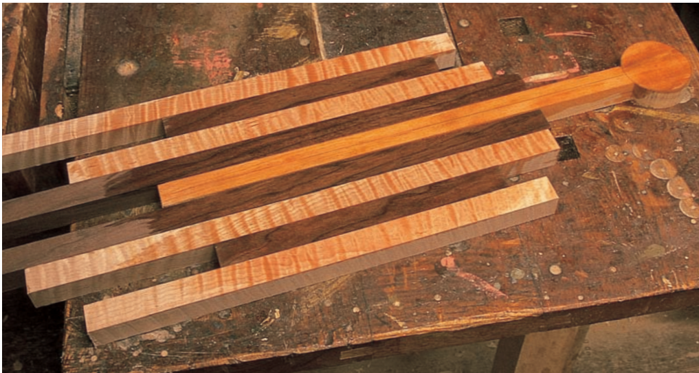
step 7 Because of the eye, the center strip can't be edge-jointed on a jointer like the other rips. Create the glue joints with a block plane, working as close to the eye as possible. Then finish the last couple of inches with a scraper or rasp.
