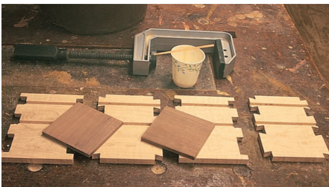
step 20 Before beginning any gluing operation, do a practice run to help you avoid panic situations. Above you can see my preparations for a dry run: all the parts, glue in a paper cup, a glue-spreading stick, the C-clamp to bring the sides together and a bucket of water for cleanup of glue squeeze-out.
