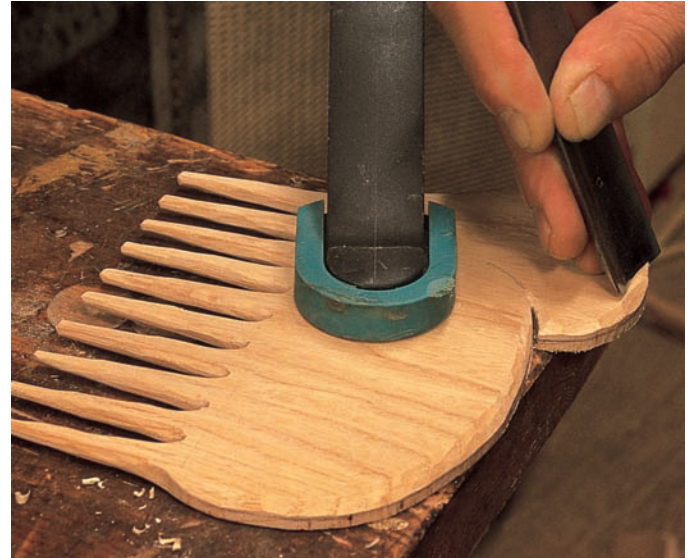
step 8 Cut a rounded bevel on the edges of the comb's spine with a wide sweep carving gouge. Finish with rasps and sandpaper.
