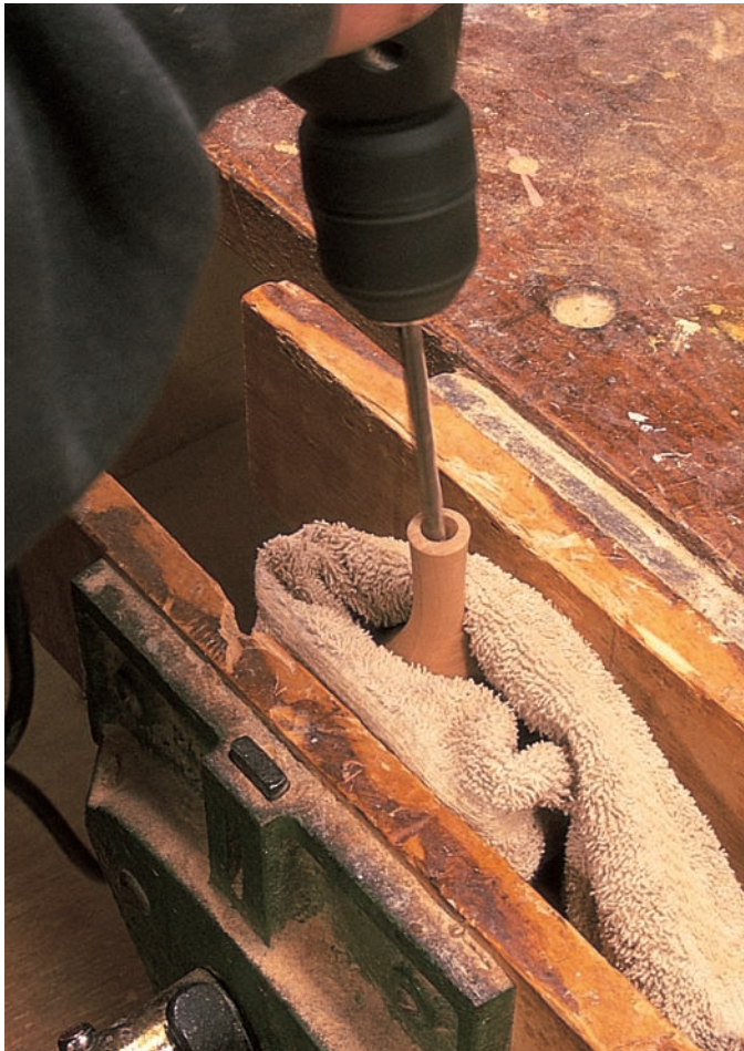
step 13 With a \frac{3}{16} " drill bit, first bore a shallow hole — \frac{3}{4} " to 1" — into the end grain of the neck. Although you need to be careful not to penetrate the sidewalls of the neck, it isn't essential to hit dead center. Once that starter hole has been drilled, use the drill bit as if it were a Dremel tool to abrade away the neck's interior. The object here is to create a graceful, tapered opening with sidewalls of a consistent thickness.
