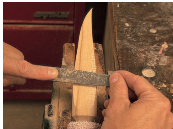
step 19 Clean up the band saw marks and complete the blade shaping with a rasp, followed by sandpaper.
