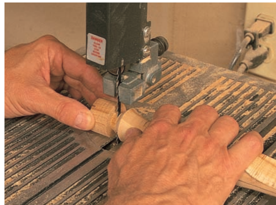
step 18 Remove the waste at the top of the handle. Finish the end with a rasp and sandpaper.
