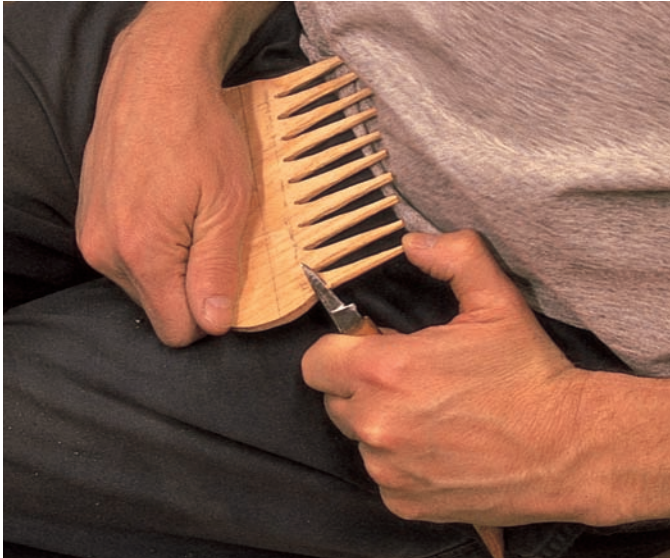
step 7 Some cuts will be easier with the knife cutting toward you.
