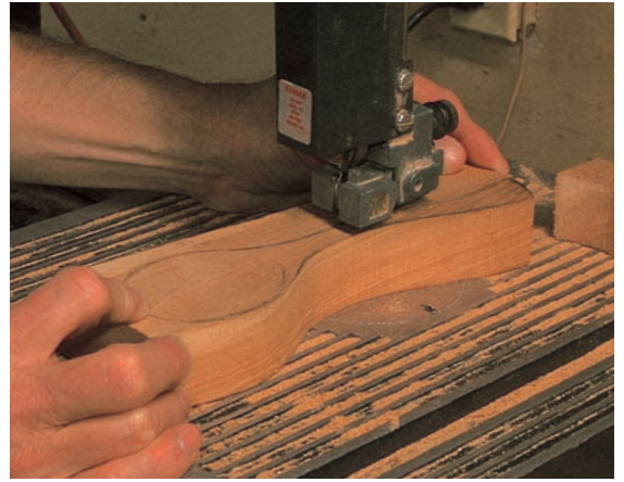
step 2 Cut out that profile on your band saw.
