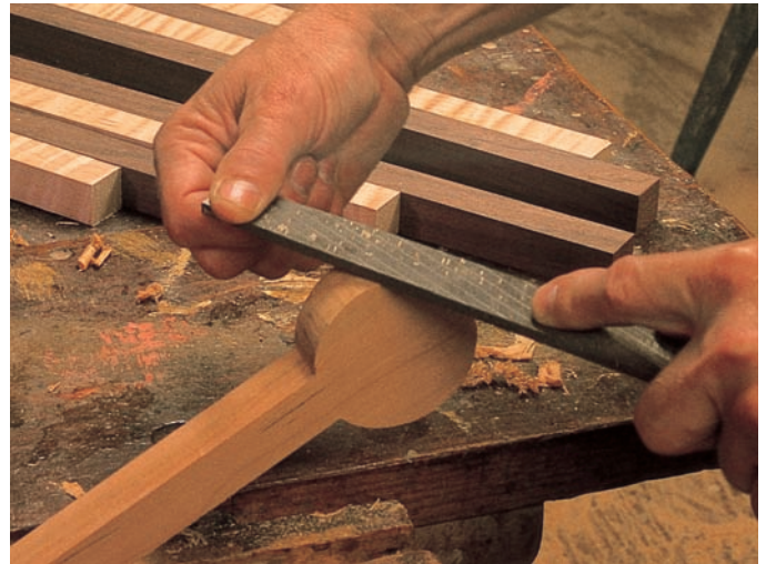
step 8 Remove band saw marks from the eye with a rasp and sandpaper.
