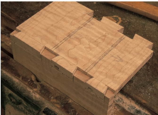
step 18 Test fit the tails and pins without fully seating the joint. If you seat the joint fully, you may not be able to get it apart again. Here, the pins and tails fit together without any fine-tuning, but in many cases a little fitting is necessary. Tweak the joint by paring very fine shavings from the sides of the tight pins until a successful fit is accomplished.
