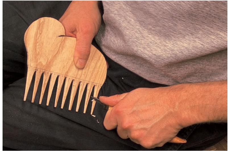
step 6 Sit down in a comfortable chair and begin refining the shape of each tooth with a knife. Some cuts will be most easily made with the knife cutting away from you.
