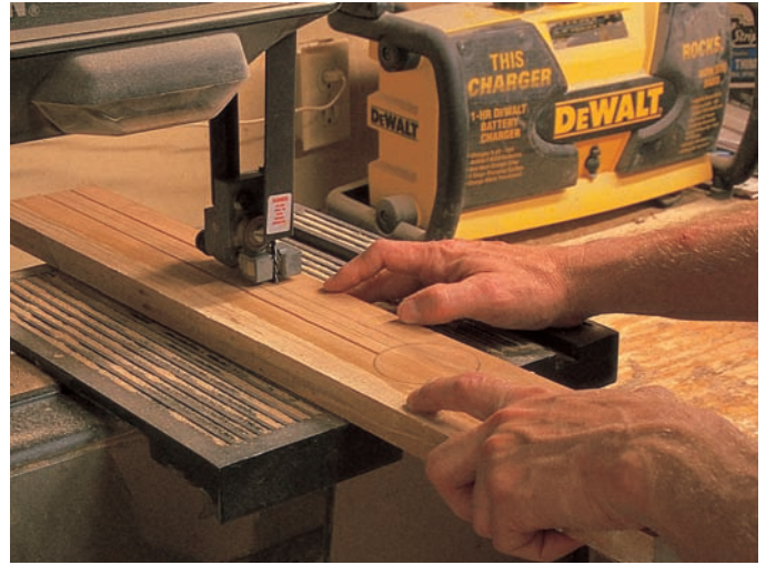
step 6 Cut out this center strip on the band saw.
