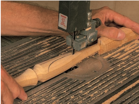
step 15 Cut the blade thickness on the band saw. I began the cut in the waste area beyond the blade tip. Notice that I stayed well outside the line in order to give myself material to rasp away later when I remove the saw marks. This operation requires a steady hand. Although the cut is made freehand, the faces of the blade must remain perpendicular to the band saw table.
