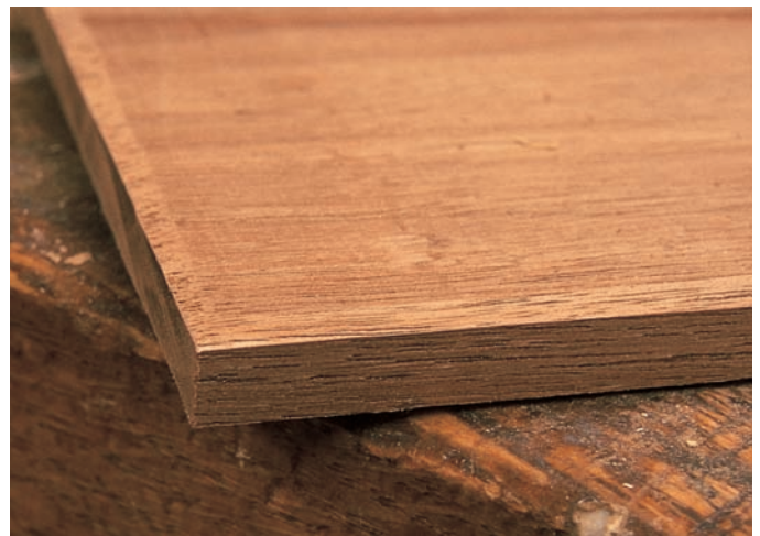
step 19 Before gluing up the case, use your block plane to put a slight bevel on all four sides of the tier bottoms to help ease the bottoms into their grooves during assembly.
