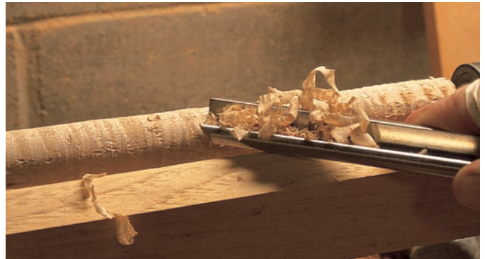
step 12 Because the two smaller frames are made from thinner stock, they need some additional support. That support will be provided by short cylinders of curly maple that will be screwed to the outside diameter of the frames. If you're turning these cylinders from a figured wood like curly maple, a fair amount of tear-out can occur even when the tool is sharp and the technique good. This can be corrected by planing with a skew — if you are experienced with that technique. If you're not, a few light passes with a fingernail gouge will remove most of the tear-out. The rest can be eliminated with sanding.
