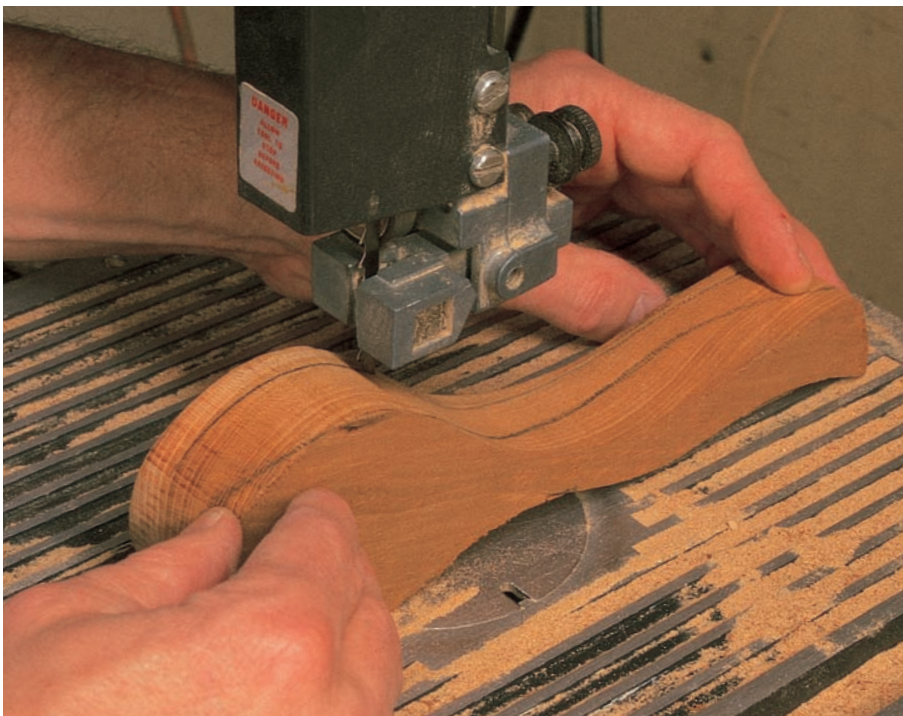
step 4 Cut out that side profile on your band saw.
