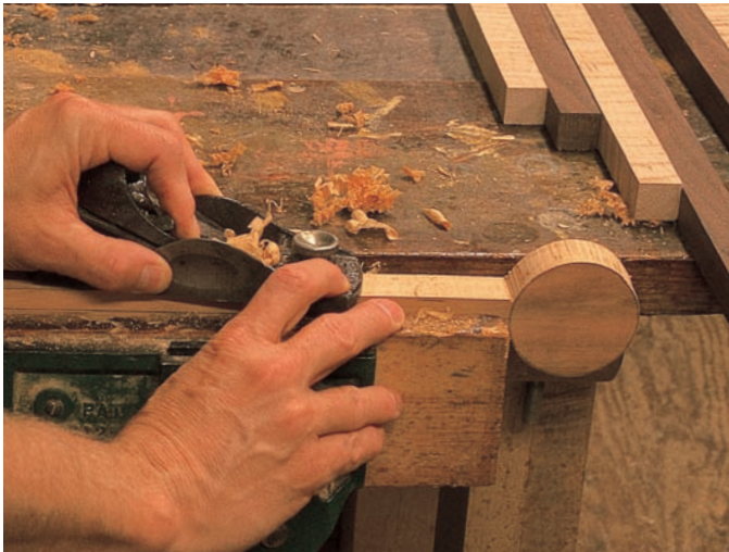
step 7 Because of the eye, the center strip can't be edge-jointed on a jointer like the other rips. Create the glue joints with a block plane, working as close to the eye as possible. Then finish the last couple of inches with a scraper or rasp.
