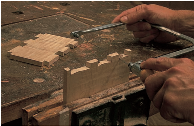
step 16 Use a coping saw to hog out the waste between pins.
