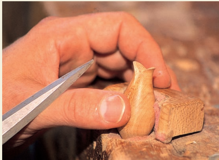
The lips are finished using a file.
