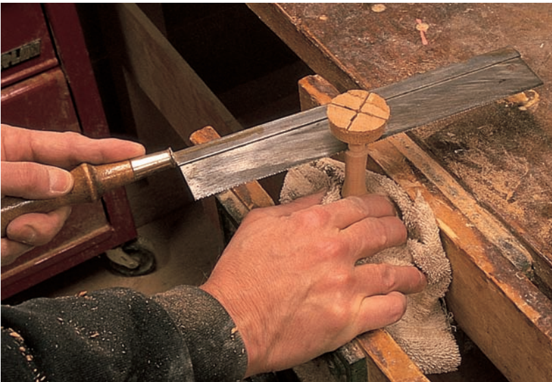
step 11 Wrap the vase in an old towel and gently clamp it in your vise. Then cut away the waste with a fine-toothed backsaw.
