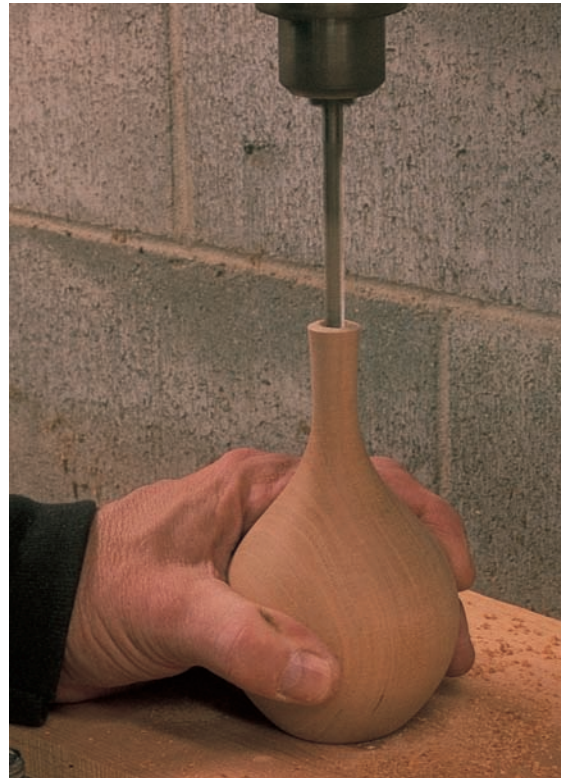
step 14 Using a \frac{1}{4} " bit, bore a deep — 2\frac{1}{2} " to 3\frac{1}{2} " — hole in the center of the opening you created earlier.
