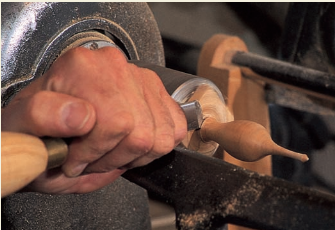
When the turning is complete, it's cut from the spigot with the skew's knife edge.
