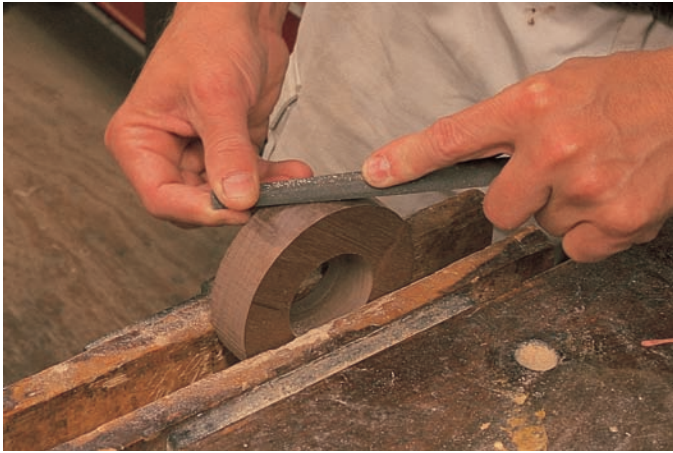
step 9 Remove the band saw marks on the outside profile with a rasp.
