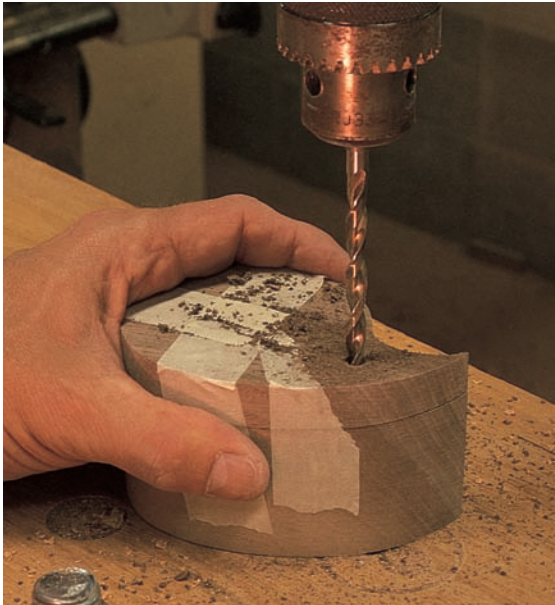
step 9 After hollowing out the box's interior, tape the box and the lid together and drill the hole for your pivot pin.
