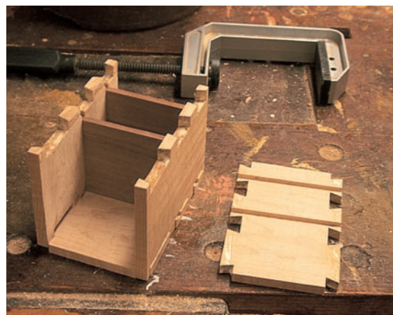
step 21 Apply glue to all the areas that will abut in the finished dovetail joint. Then assemble the case around the two bottom panels, which will fit unglued into their grooves.
