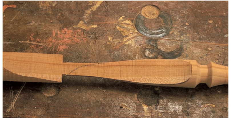
step 16 Mark the tip of the blade on one of the faces created in the previous step.
