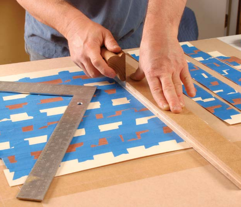
Crosscut the strips. Use the guide again, setting up the first cut with a framing square.
