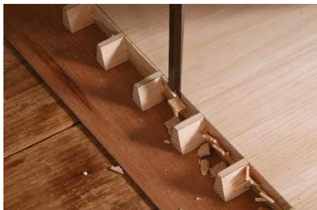
Chop and pare. Chop away the waste between the pins with heavy blows, leaving \frac{1}{16} in. or so along the baseline (top). Follow with paring cuts, starting with the tip of the chisel in the score line. Work from each face of the workpiece toward the middle to avoid blowout (bottom).
