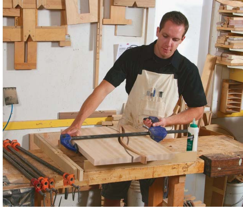
Thin strips make sweet curves. Lewis uses sandwiches of 1/8-in.-thick strips to create the S-curved stripes that pass through the entire board.
