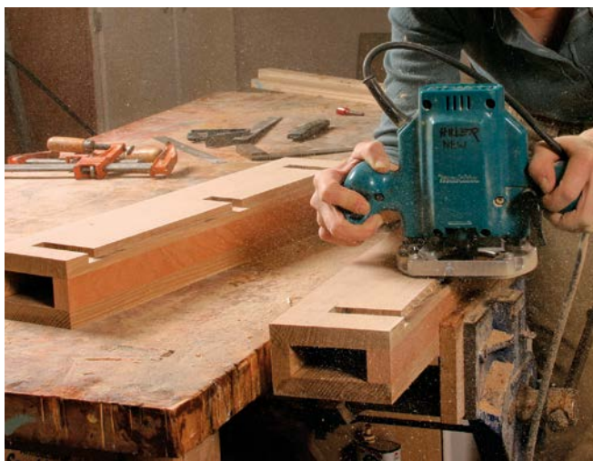
Rout a rabbet for the back boards. A rabbeting bit works well, with the guide bearing running against the side of the column. Stop the rabbet in the shelf dados.
