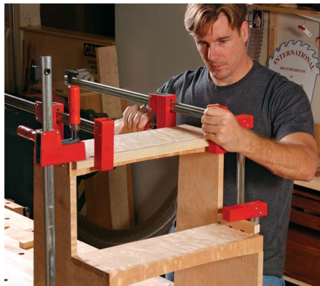
One stretcher at a time. Use two clamps to hold the stretcher against the step and another two to pull it down into its socket.
