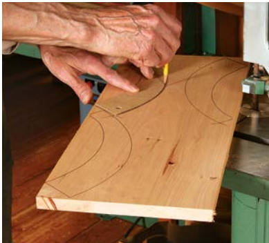
Leg layout. Trace the shape using a cardboard template, orienting the grain so it runs straight from tip to tip (see “Leg Profile” on p. 152).
