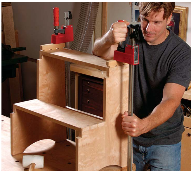
One step at a time. Clamping is easier if you do each step in turn. Dry-fit the rear stretcher to keep things square as the glue dries.
