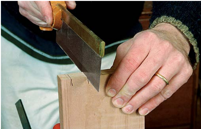
Cut the tails. A fine-tooth backsaw makes a clean and narrow kerf and offers good control over the cut.
