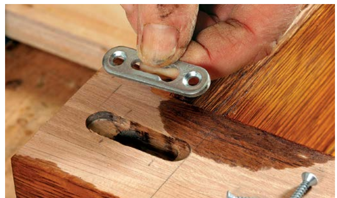
Rout two depths for hanging hardware. The first step will hold the hardware, while the deeper step allows the hanging screw to be inserted.
