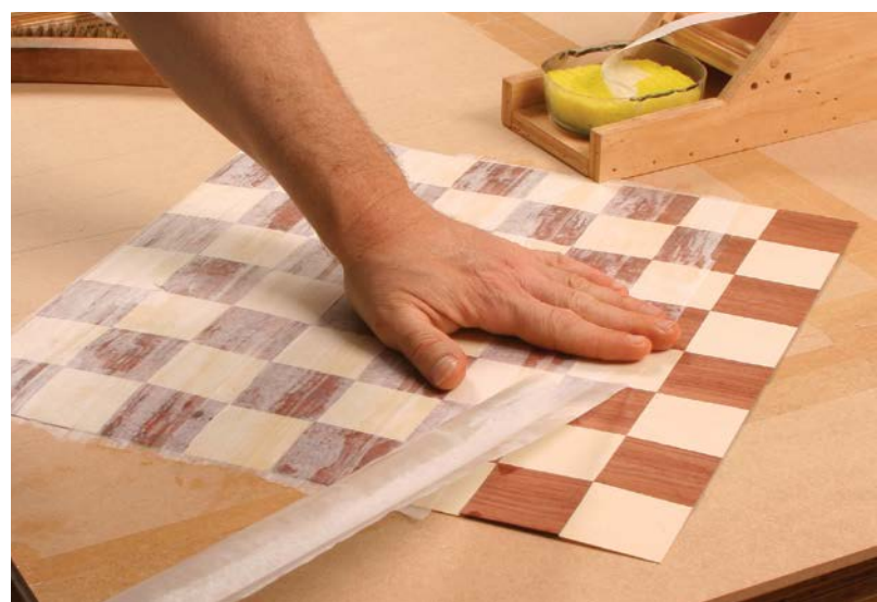
Veneer tape locks in the pattern. Peel off the small pieces of blue tape from the show face. Then use veneer tape on the entire surface (above), overlapping the pieces slightly and trimming away the excess. Draw the tape across a wet sponge to dampen it. After the veneer tape has dried, remove the blue tape from the opposite face (left).
