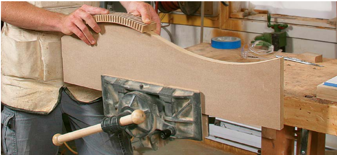
Make it smooth. Fairing the template's curves is vital because any bumps could be visible in the inlay gluelines. Lewis used the tablesaw to cut slots in a piece of MDF, creating a pliable sanding block that conforms to convex and concave curves.
