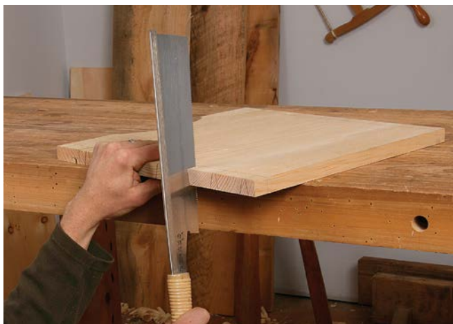
Rip the pins. Hunter saws just shy of his layout line, then pares right to it, leaving the line for reference.
