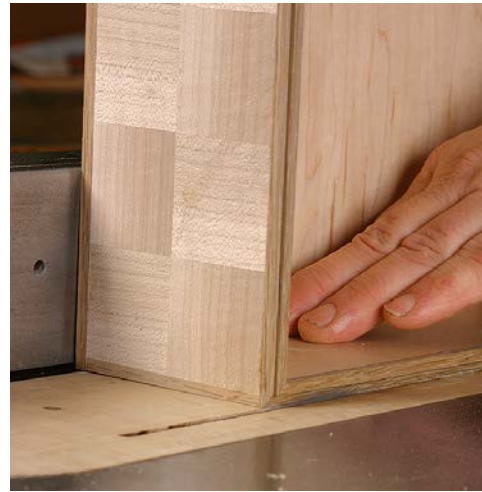
A rabbet meets its mate. Banding, mitered and glued to the lip of the bottom section, will mate with similarly rabbeted banding on the top section. Make a series of light cuts to sneak up on a tight fit.
