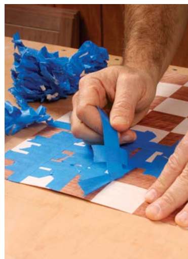
Veneer tape locks in the pattern. Peel off the small pieces of blue tape from the show face. Then use veneer tape on the entire surface (above), overlapping the pieces slightly and trimming away the excess. Draw the tape across a wet sponge to dampen it. After the veneer tape has dried, remove the blue tape from the opposite face (left).
