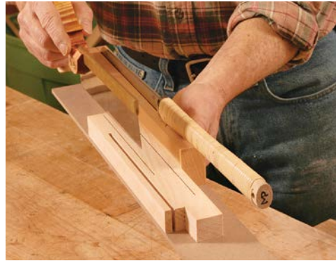
Simple storage for saws. Pekovich cut kerfs in pine blocks to secure his handsaws, scrapers, and combo square. The blocks are glued to a medium-density fiberboard (MDF) base and installed as a single unit.
