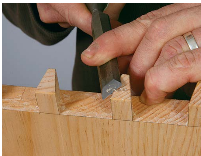
Tiny chamfers are a big help. Chamfered edges give the proud dovetails a distinctive look and also make assembly go more smoothly.
