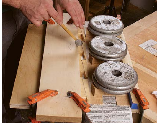
An ingenious clamp. Scrap blocks and weights keep veneer sheets from buckling. Wedges tapped in place between the veneer and fence provide clamping pressure.
