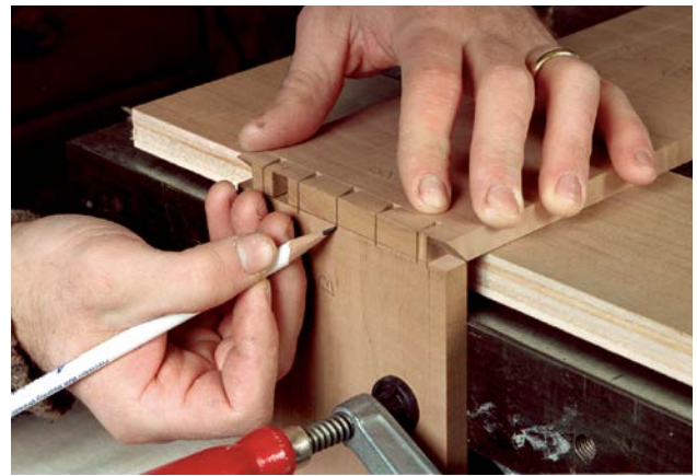
Mark the pin boards from the tail boards. A clamp is worth as much as a steady hand when transferring the locations of pins.
