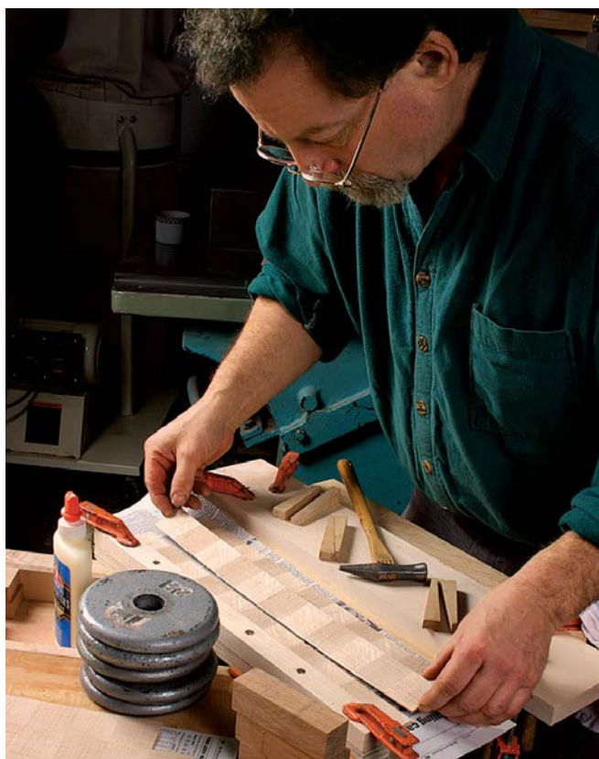
The second glue-up. Veneer strips are edge-glued a few at a time. Old newspaper keeps veneers from sticking to the gluing jig. The strips are staggered to create the checkerboard pattern.
