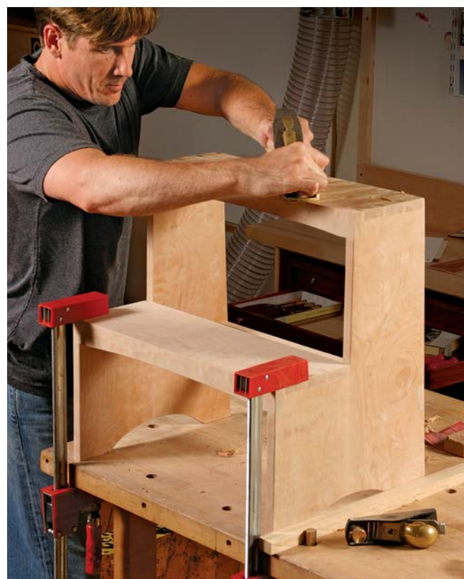
Sharp plane eases awkward work. Prepping the outside surfaces isn't simple, but clamping the stool down tight to the bench and using a very sharp plane to take light shavings makes the job manageable.
