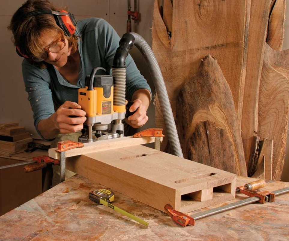
Rout shelf dados while columns are clamped together. Clamp a straightedge to the columns to guide the router (left). Use a chisel to square up the front edge of the dados by hand (above).
