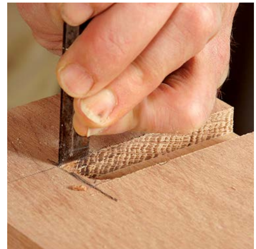
Rout shelf dados while columns are clamped together. Clamp a straightedge to the columns to guide the router (left). Use a chisel to square up the front edge of the dados by hand (above).
