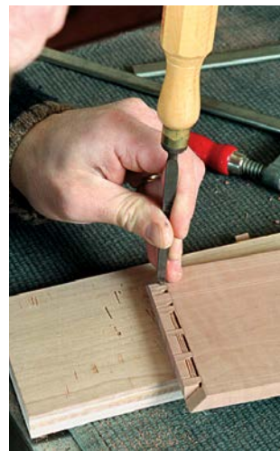
Mark the pin boards from the tail boards. A clamp is worth as much as a steady hand when transferring the locations of pins.
