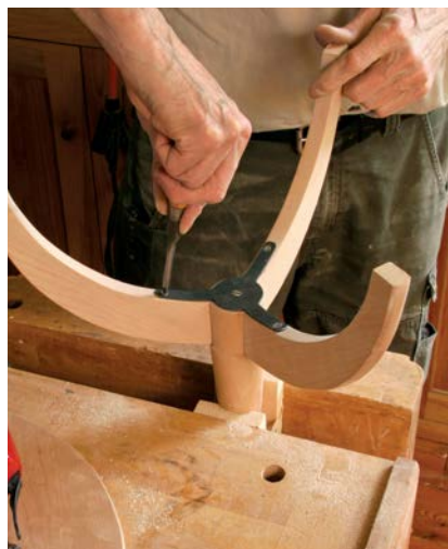
Bottom needs support. Screwing in a metal brace, or spider, reinforces the sliding dovetails. Becksvoort bought his spider and modified it, cutting several inches off each of its legs.
