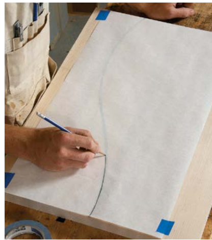
Thin strips make sweet curves. Lewis uses sandwiches of 1/8-in.-thick strips to create the S-curved stripes that pass through the entire board.
