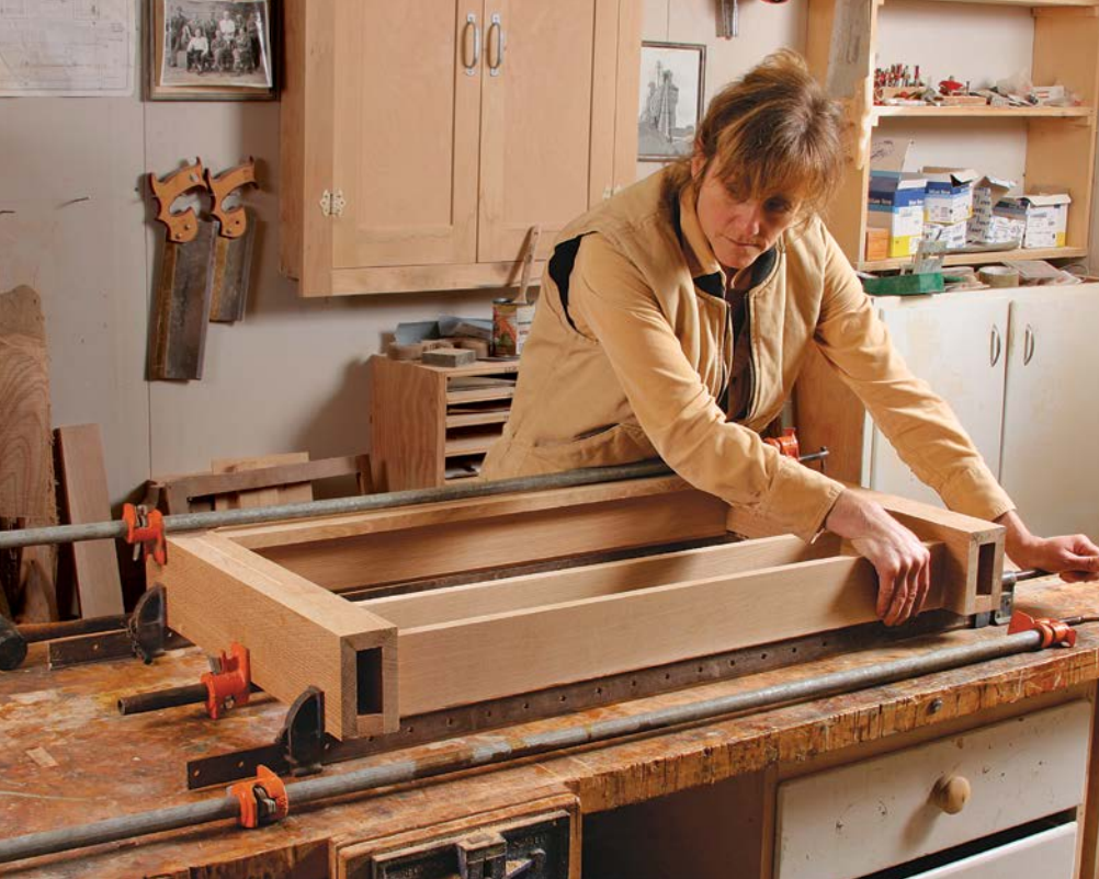
Clamping the case. Use enough pressure to pull the shelves into their housings, but avoid excessive strain on the hollow columns (left). Apply finish to the parts before screwing the back boards in place (above).
