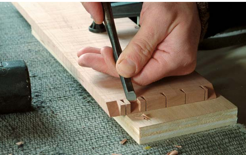
Rough-cut the outside miters with a saw. Then pare them to your pencil line with a chisel.
