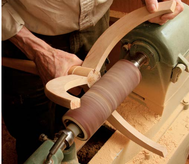
Joint cleanup. After the glue cures, smooth the bottom of the post with a drum sander.
