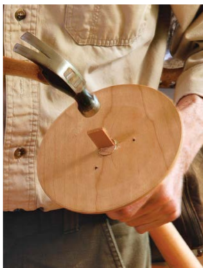
Crosswise wedge. To avoid splitting the subtop, orient the wedge perpendicular to the grain. After the glue cures, saw off the wedge and chisel the tenon flush. Then attach the top with screws through the subtop.
