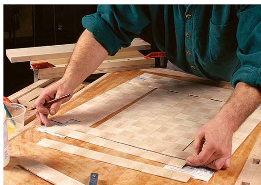
Spreading the sheets. Once the parquet panels have dried, lay them out and arrange side panels to match the grain pattern with the top panel.
