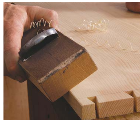
Final touches before assembly. With all the joinery cut, Hunter creates a glassy finished surface with light passes of a Japanese smoothing plane (left) and chamfers all exposed edges (right).
