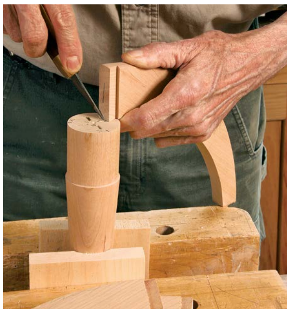
Socket layout. With the post inverted in the vise, scribe around the dovetail key. Pine cushion blocks hold the post steady.
