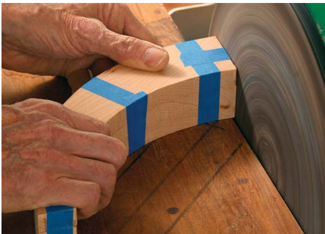
Strapped in for sanding. After cutting the legs, tape them in a stack and smooth the ends and the outside curve at the disk sander (left). Sand right through the tape. Retape the stack, then fair the inside curve with a drum sander (above).
