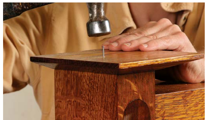
Attach the end caps. Countersink the finish nails and fill the holes with matching wood putty.
