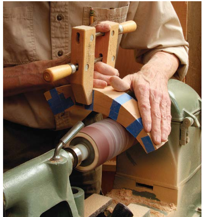
Strapped in for sanding. After cutting the legs, tape them in a stack and smooth the ends and the outside curve at the disk sander (left). Sand right through the tape. Retape the stack, then fair the inside curve with a drum sander (above).
