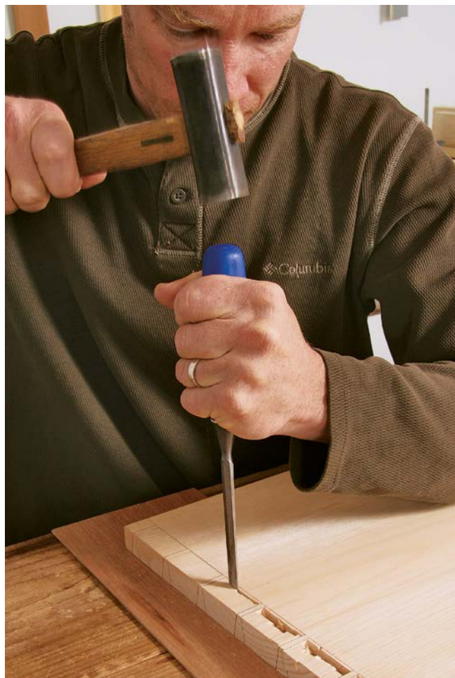
Rip the pins. Hunter saws just shy of his layout line, then pares right to it, leaving the line for reference.
