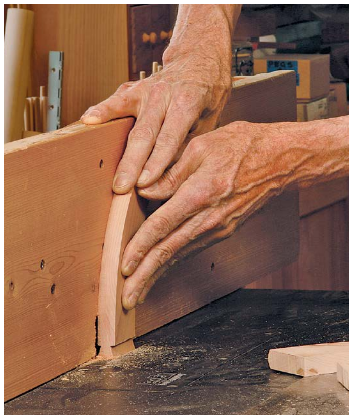
Standing dovetail. Cut the sliding dovetail keys at the router table, using a dovetail bit and a tall fence.
