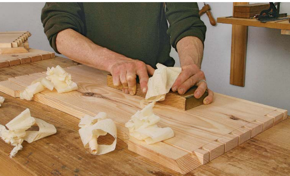
Final touches before assembly. With all the joinery cut, Hunter creates a glassy finished surface with light passes of a Japanese smoothing plane (left) and chamfers all exposed edges (right).
