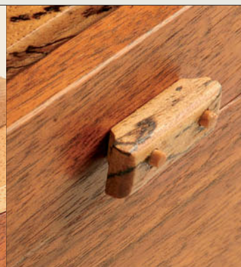
Front-mounted. Mounted to the front of a hinged lid, the pull serves as a lifting point.
