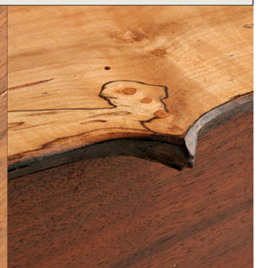
Live-edge. The natural curve of a live edge works perfectly as a lift for some boxes.
