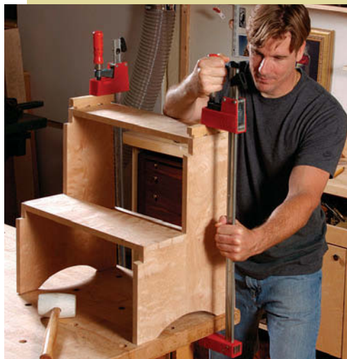
One step at a time. Clamping is easier if you do each step in turn. Dry-fit the rear stretcher to keep things square as the glue dries.
