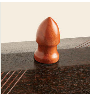
Turned. Small lathe turnings make wonderful pulls. A single brass screw holds each one in place.
