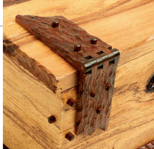
Wood. Shopmade hinges add to the handmade appeal. The flat version (above) is screwed from the bottom. Wood pins secure an L-shaped hinge (right).
