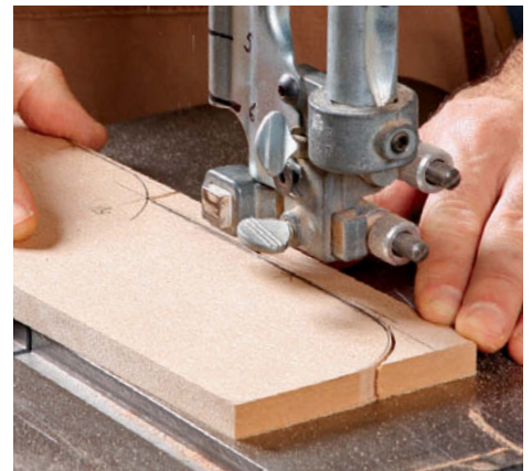
Bandsaw the profiles. Stay close to the line.
