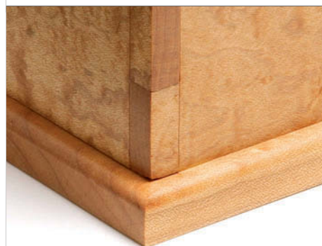
Oversize flat bottom. An oversize flat base creates the look of a molding around the bottom of the box.
