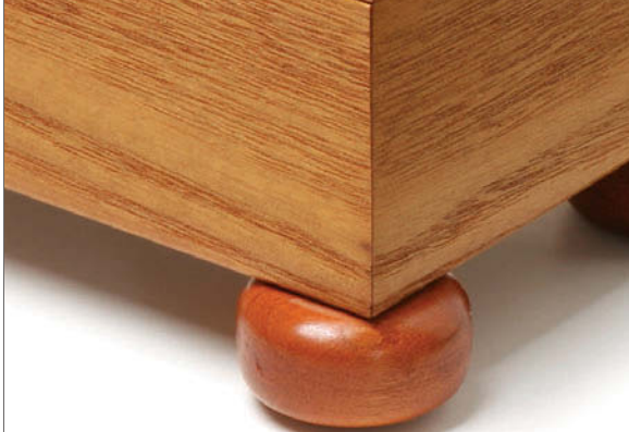
Rounded disk. A single countersunk screw driven through the bottom of the disk secures it to the corner of the box.
