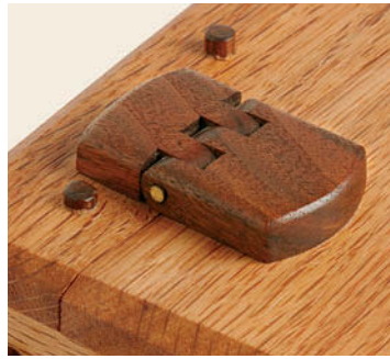
Wood. Shopmade hinges add to the handmade appeal. The flat version (above) is screwed from the bottom. Wood pins secure an L-shaped hinge (right).
