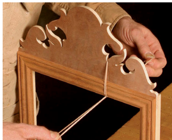
Glue on the first attachments. Apply a thin film of glue to the straight side of the top crest, place it on the poplar subframe, and begin clamping with rubber bands. Use two rubber bands knotted together to stretch around the frame, securing the ends over projections on the crests. Because the attachments do not touch each other, if you work carefully it is possible to apply all six at one time.
