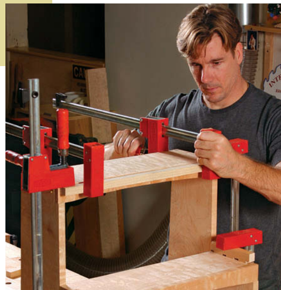
One stretcher at a time. Use two clamps to hold the stretcher against the step and two more to pull it down into its socket.
