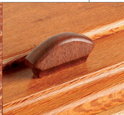
Fan-shaped. Rounded and softened edges give this pull a delicate look that works nicely with lightweight lids.
