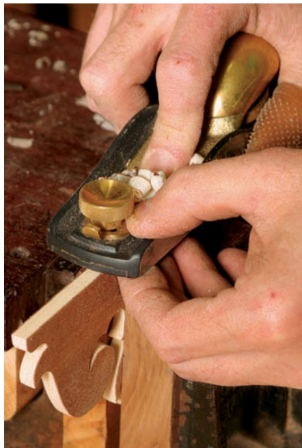
A good contact surface. Joint and square the straight edges of the attachments with a block plane so that they will have good glue contact with the frame.
