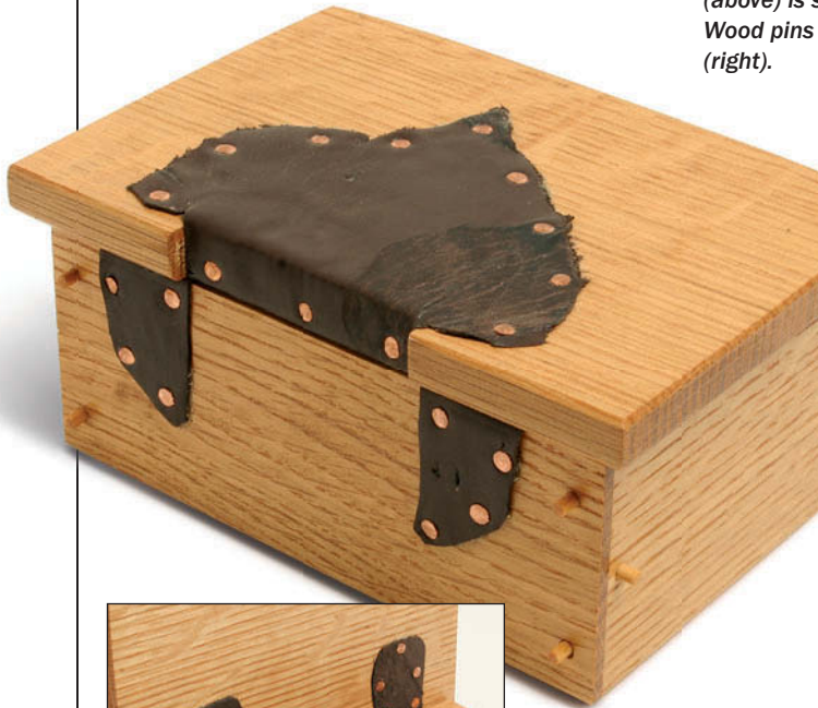
Leather. Three pieces of leather—two end pieces and a center piece—are secured with brass tacks to create a unique hinge.
