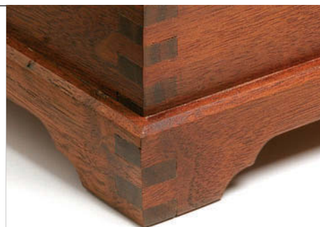
Cutaway base frame. Cutting away the bottom edge of a base frame also produces feet.
