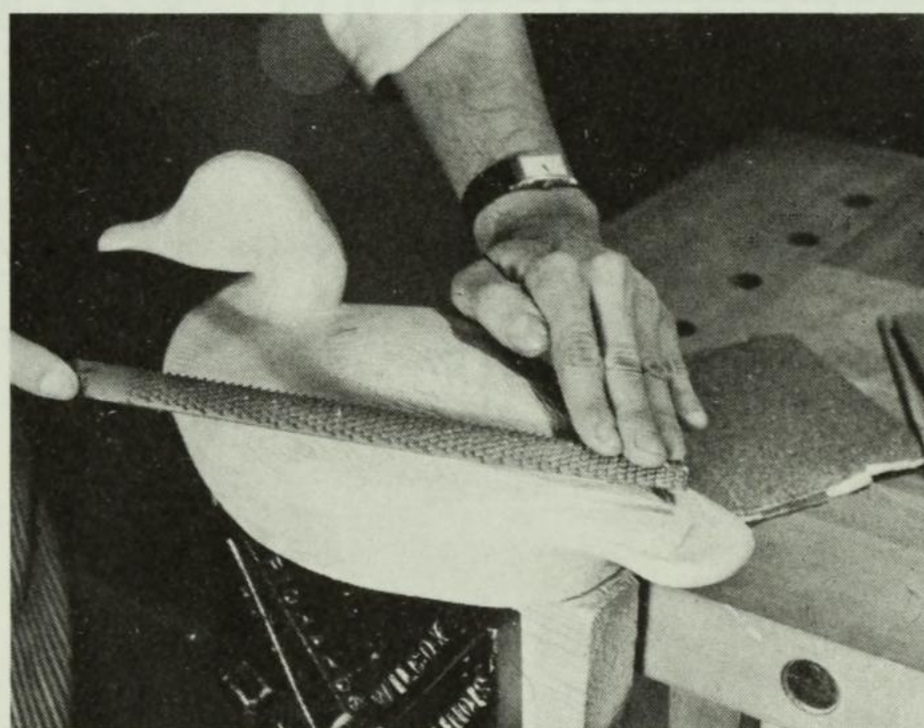
Photo 6. The final roughing effect which is essential to a good decoy is accomplished with a bastard file or wood rasp.
