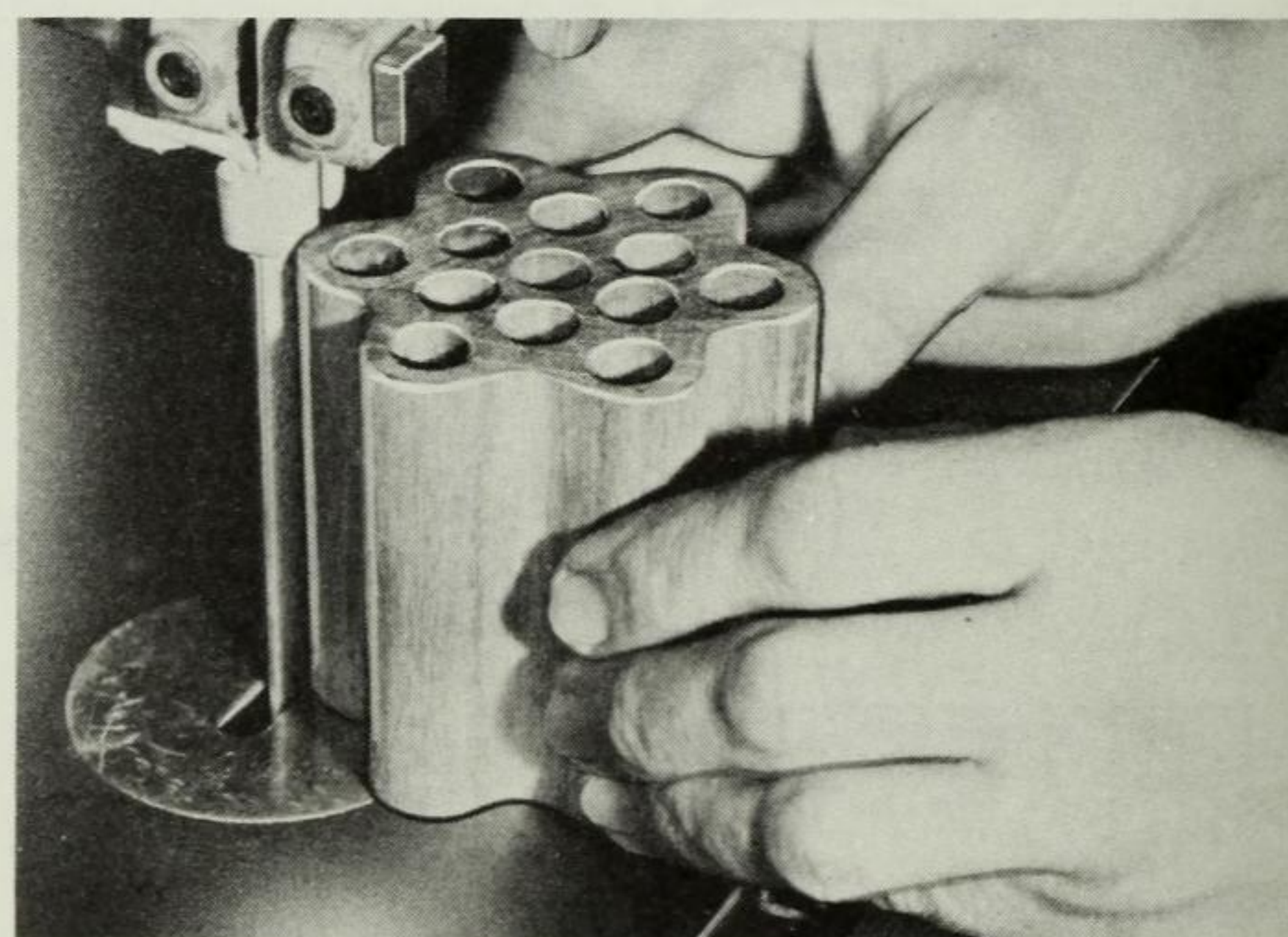
Photo 2: To sand the outside curves use the belt sanding attachment with a fine belt on the band saw.
