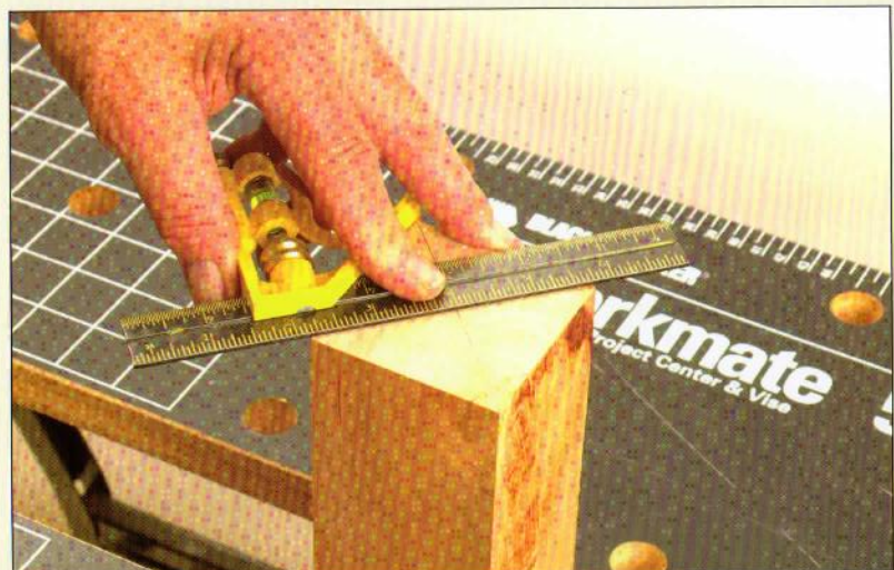
Figure 1.25. By connecting the corners, a combination square finds the center of a turning blank. A small square like this is a very useful measuring and layout tool.
