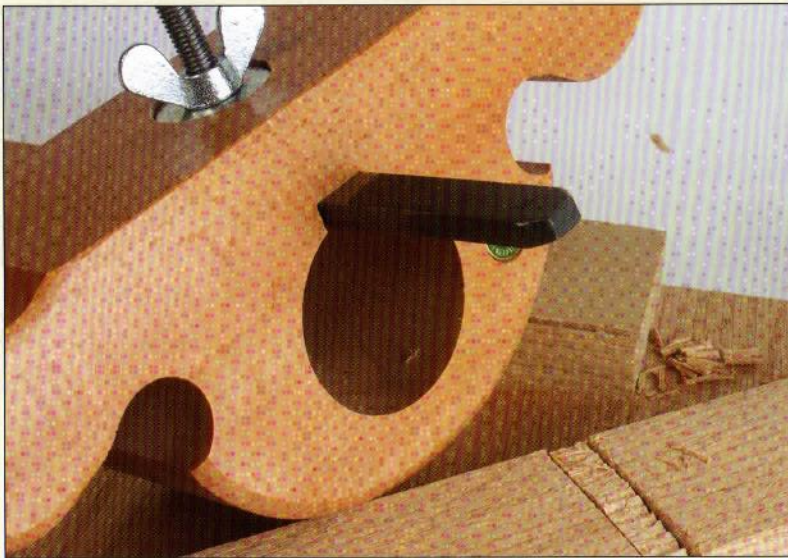
Figure 1.30. Router planes flatten the bottom of recessed areas or can clean up machine-routed areas. This particular plane has a nice wooden body.
