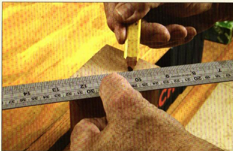
Figure 1.22. Aluminum straightedges are accurate and easy to handle, making them a good choice for in-shop measuring. A rule may also be used to find centers.
