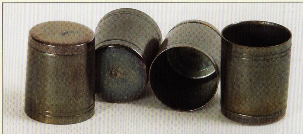
Figure 1.9. Metal can caps make great cane tips. They slip on and may be epoxied in place. A brad or small screw may also be driven into the stick's end grain to secure them.
