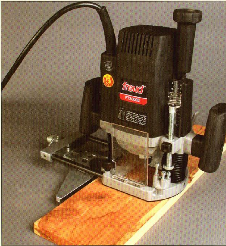
Figure 1.41. A plunge router with an edge guide can do a lot of the work on canes and staffs.
