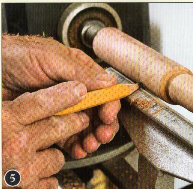
5 Darken the marks —Use a very sharp carpenter's pencil to run the marks all the way around the cylinder.
