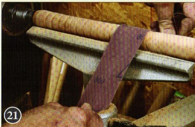
21 Sand and finish —Do finish smoothing of both spindles while they are on the lathe, using cloth-backed sanding strips. I also applied the Liberon wax finish at this point.
