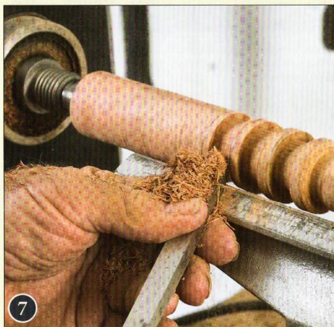
7 Reduce the diameter —Continue removing waste wood from between the future beads until these spaces all reach the same depth.
