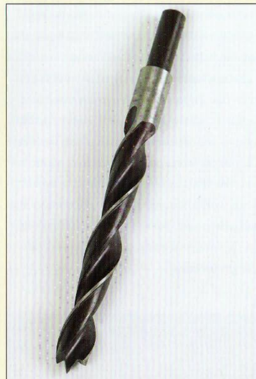
Figure 1.34. A brad point drill bit will start without an initial center punch and makes a clean hole.
