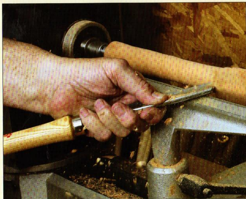
Figure 1.37. The lathe allows you to remove wood quickly and accurately to form round stock for your stick, cane, and staff projects.
