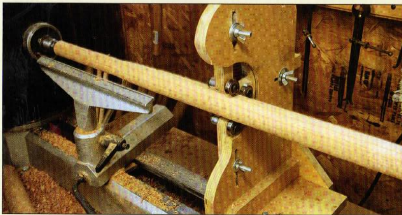
Figure 1.40. Spindle turning on the lathe is aided by a steady rest. There are several on the market. This one is homemade.
