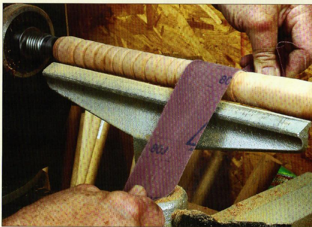
Figure 1.51. Sanding is an essential preparation for every type of finish on wood. On-lathe sanding saves a great deal of time and works better than trying to hand sand or power sand with the shaft off the lathe.
