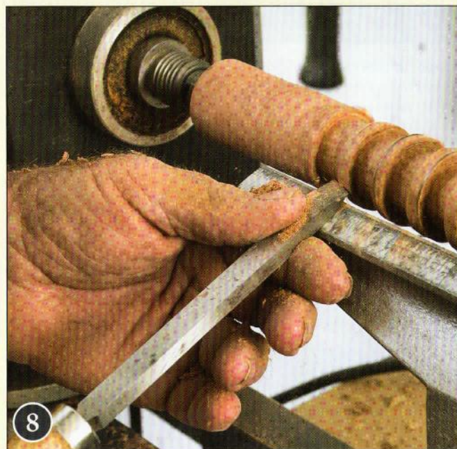
8 Round the beads —Use the skew chisel to round over the beads, but don't undercut them.
