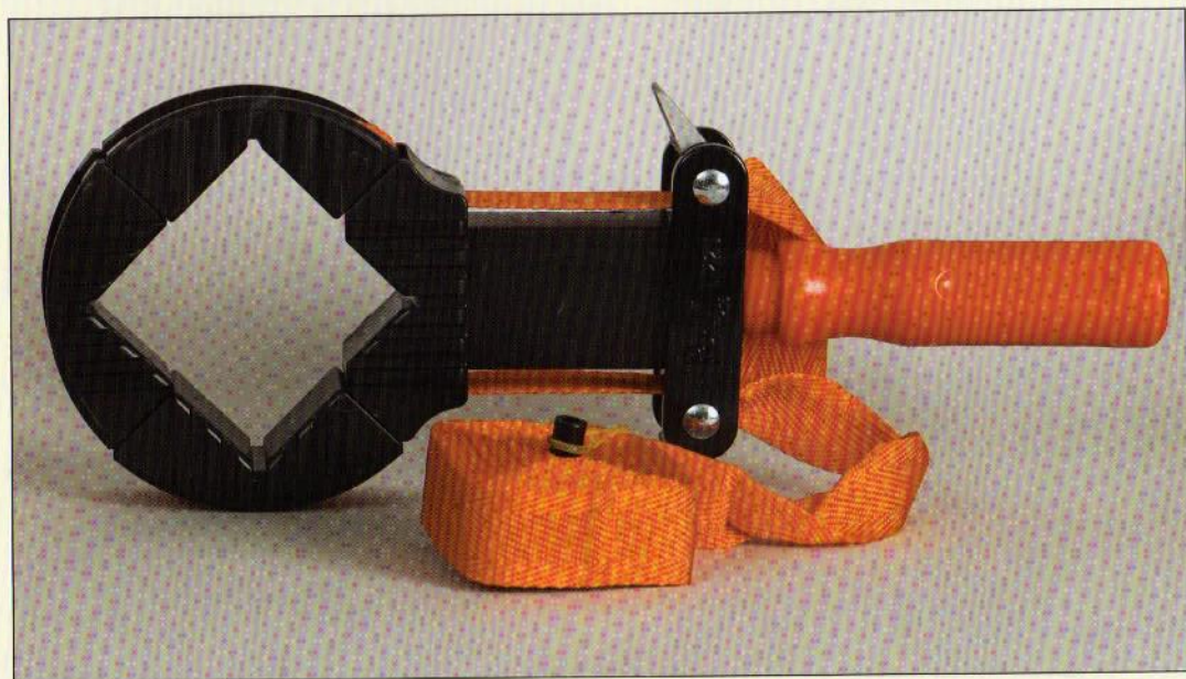
Figure 1.8. Band clamps are especially useful for round, octagonal, or similar shapes and range from light-duty to heavy-duty types. This band clamp is made for light tasks.
