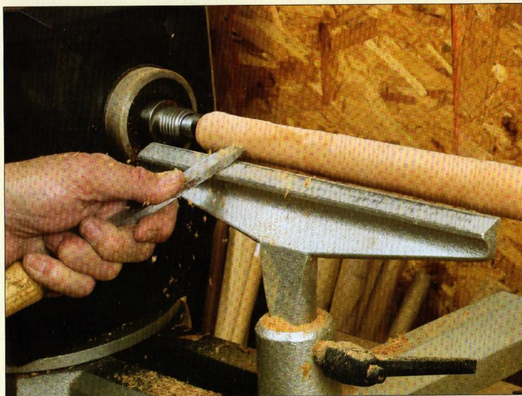
Figure 1.38. The lathe also makes it easier to smooth out the shafts of sticks, canes, and staffs. Here, the skew chisel makes a planing cut and leaves a very smooth surface.
