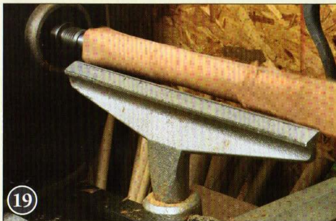
19 Turn the shafts —Make the same preparations—marking the centers, cutting the kerfs, drilling the holes—for the two longer spindles. Start with the thicker of the two pieces for the top, and turn the blank cylindrical on the lathe.
