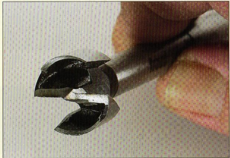
Figure 1.35. Forstner bits make clean, flat-bottomed holes.
