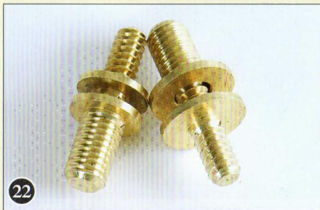
22 Install the brass joins —To fit the two-piece threaded joins, simply drill the top of the bottom section for one piece, and the bottom of the top section for the other piece. Epoxy in place and screw the two pieces together.
