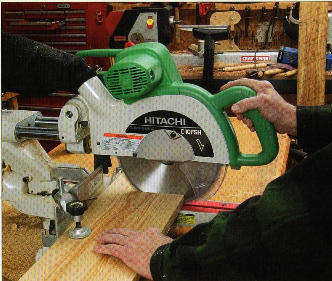
Figure 1.42. Here, a 10" slide compound miter saw is squaring a board end.
