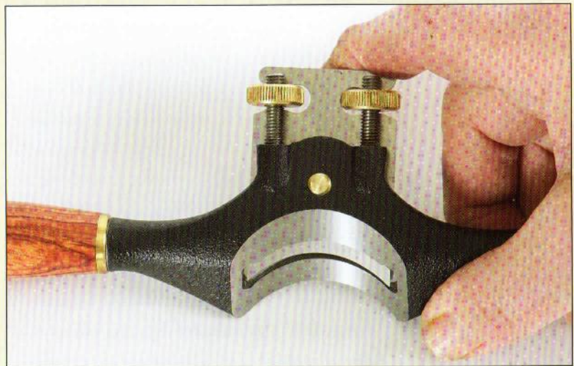
Figure 1.31. This is a convex surface spokeshave, used to form round surfaces.
