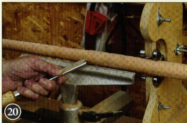
20 Continue turning —Continue shaping the shaft. Steady rests are a big help with long, thin spindles.
