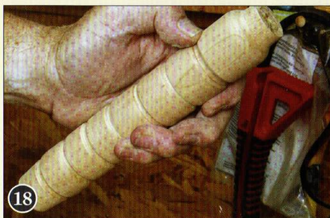
18 Wax the wood —I applied a Liberon hard wax finish while the handle was spinning at moderate speed on the lathe.
