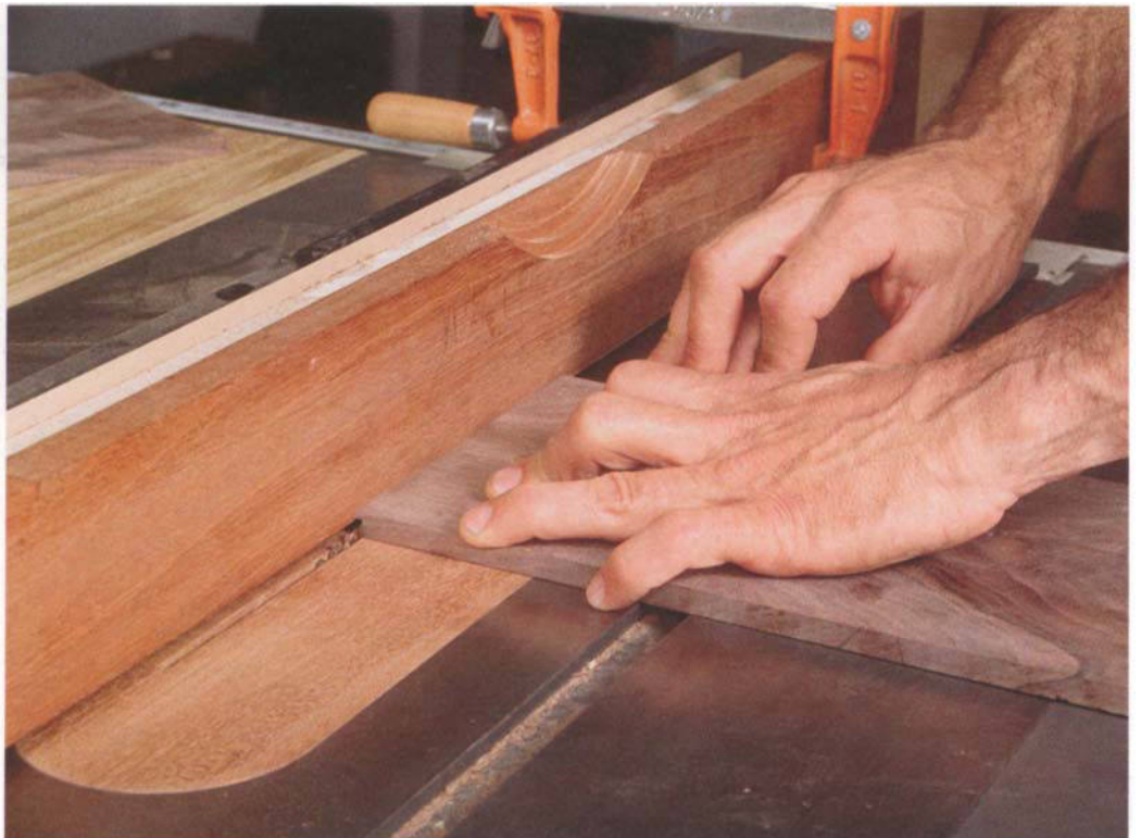
PHOTO C: Cut the shoulder of the rabbet using a board clamped to the rip fence above the rabbet to prevent the cutoff from jamming between the blade and fence.
