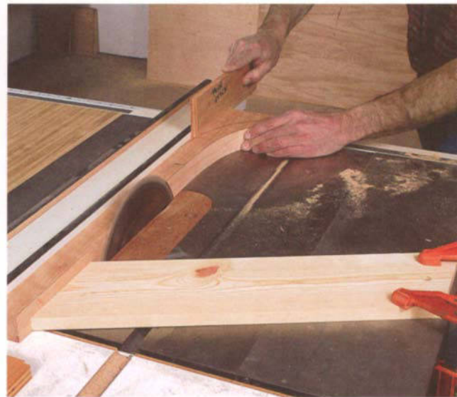
PHOTO A: Set up a featherboard to press the leg to the rip fence. Use a block to stop the cut after 18½ in.
