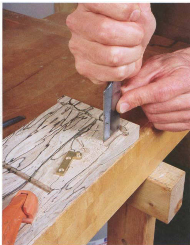
PHOTO C: Using a sharp chisel, gradually pare to the layout lines, until the hinge leaf fits very snugly.
