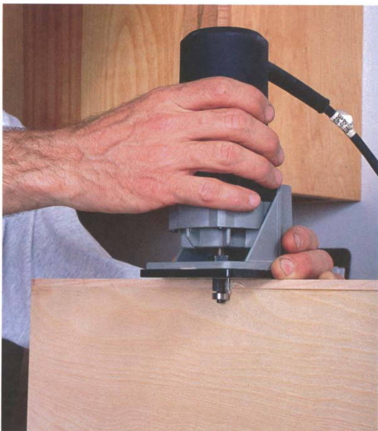
PHOTO D: A laminate trimmer with a flush-trimming bit quickly routs the edging flush to the plywood panel. Afterward, smooth the joint with a block plane set for a very fine cut.
