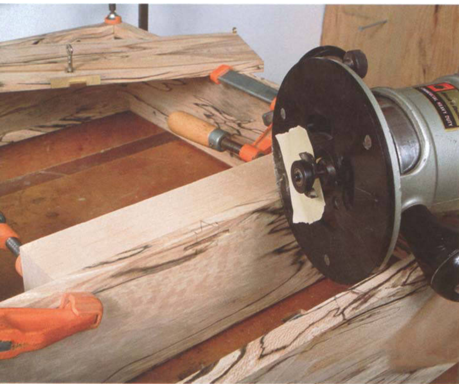
PHOTO G: Use a slot-cutting bit to rout the mortise for the lock bolt. Clamp square scrap to the divider to steady the router. (The masking tape here simply provides a better view of the bit.)
