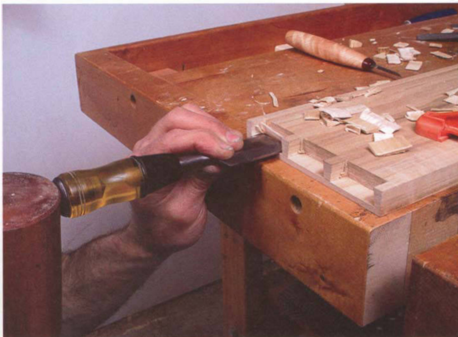
PHOTO J: After chiseling out the bulk of the waste, use a wide flat chisel to pare down to the layout lines.
