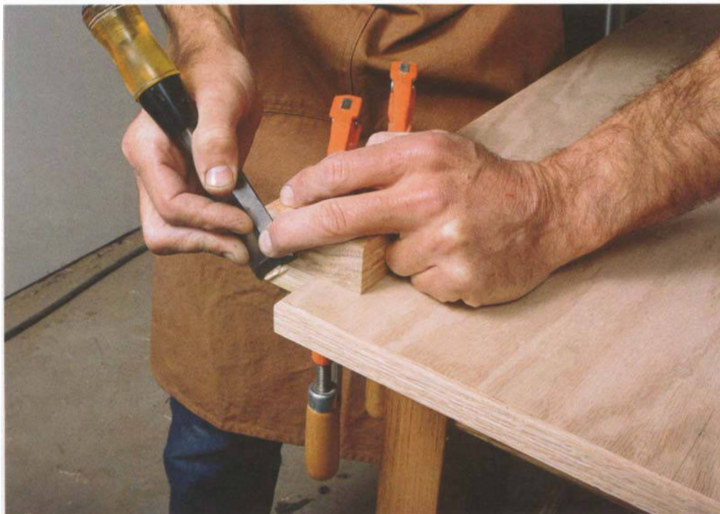
PHOTO D: After jigsawing the platform notches just a hair small, pare them to final size, guiding a chisel against a square wooden block.
