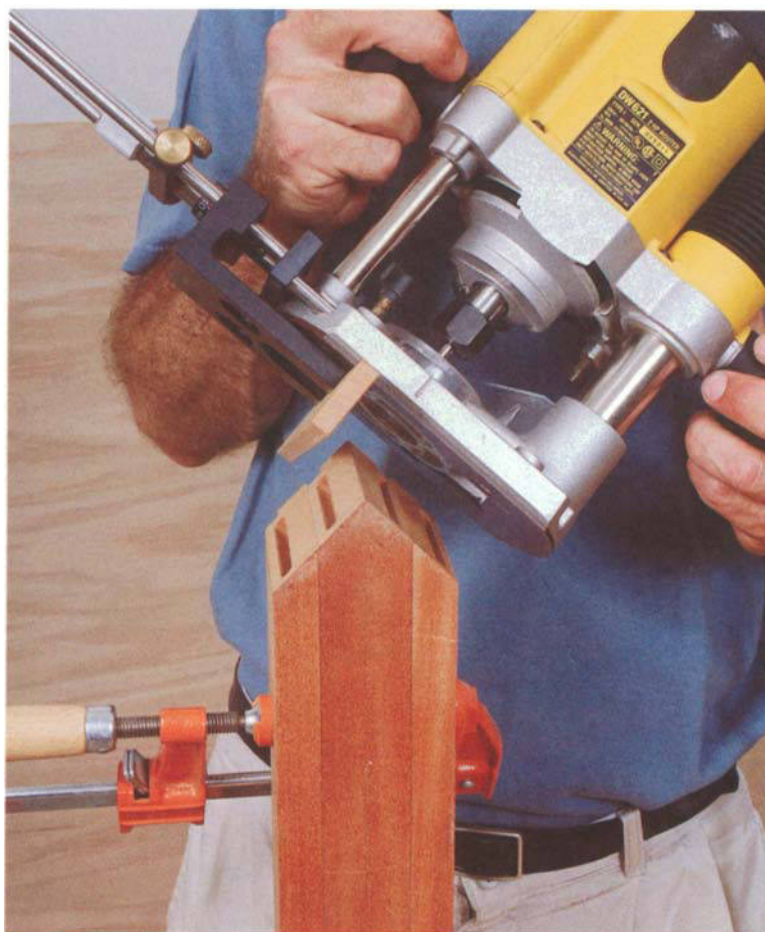
PHOTO A: A shopmade T-square clamped to the case side guides the router when cutting the shelf dados.
