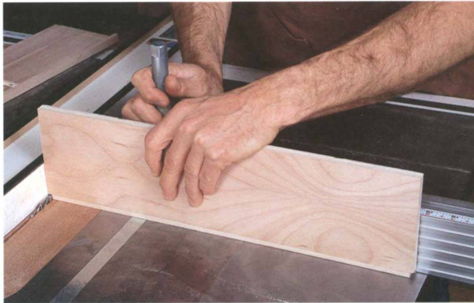
PHOTO B: After gluing on the slightly long shelf edging, nip it off ¼ in. from the end. Use the rip fence as a stop.
