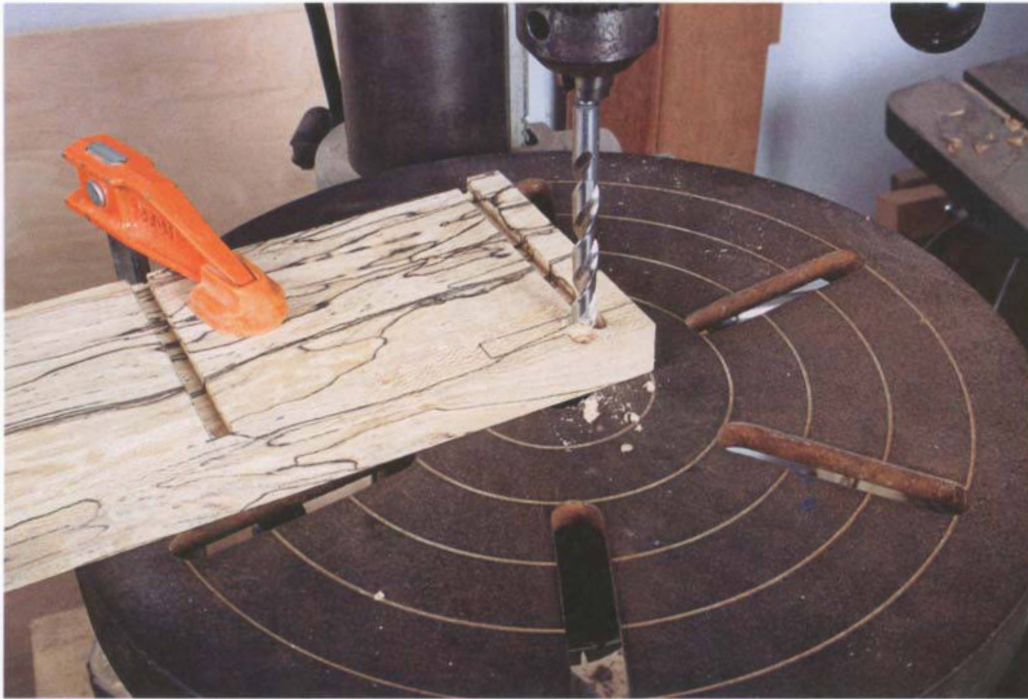
PHOTO A: Bore a hole to accept the knife hinge knuckle. Make the hole as deep as the hinge leaf is thick.
