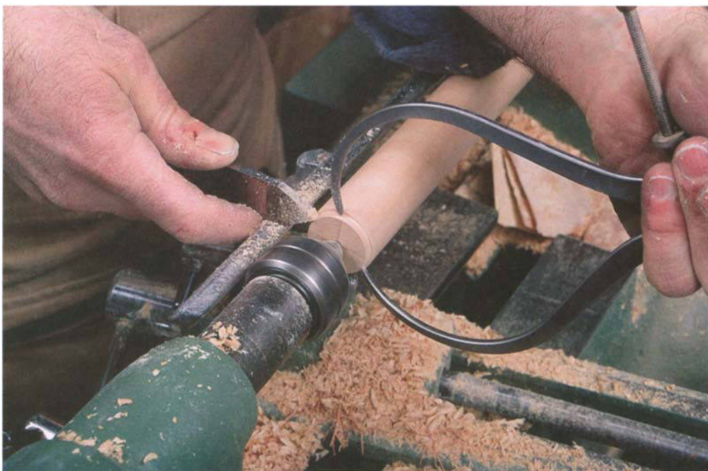
PHOTO N: Use a parting tool to turn the tenon on each end of the arm rail.
