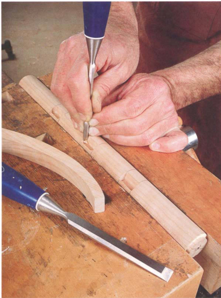
PHOTO P: Cut away only the corners on the thin-walled edge; then enlarge the mortise bit by bit on the opposing edge until it accepts the slat.
