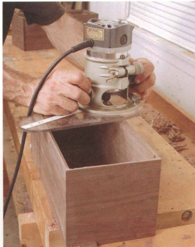
PHOTO E: To prevent tearout on the interior rabbet shoulder, first make a shallow "climb cut," carefully moving the router in a counterclockwise direction. Finish up by routing in a clockwise direction, as shown here.
