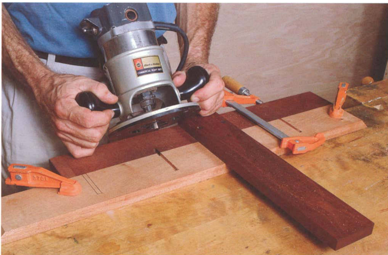
PHOTO A: A shopmade T-square clamped to the case side guides the router when cutting the shelf dados.
