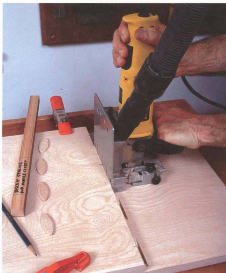
PHOTO G: Set the biscuit joiner for a #10 slot, align the center index line on the bottom of the joiner with the biscuit location mark, and plunge into the divider.
