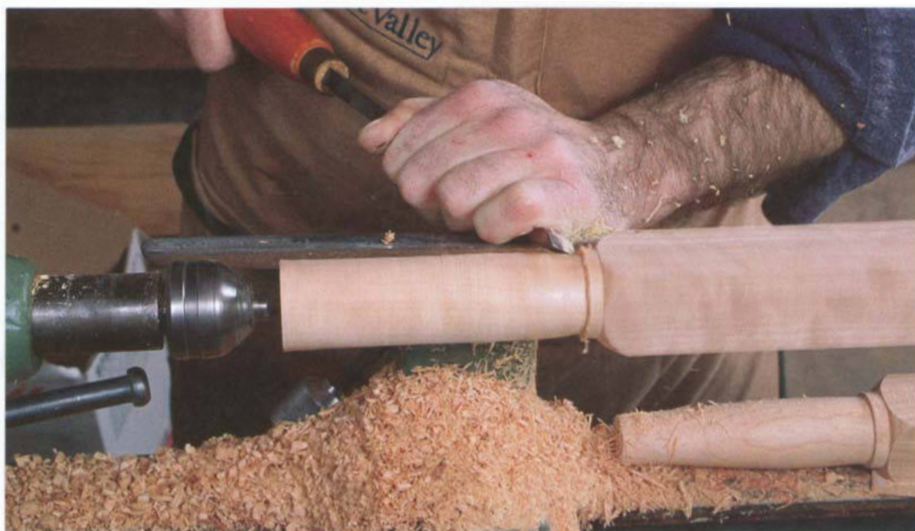
PHOTO D: Use a skew to shape the top of the curve, creating the ring above.
