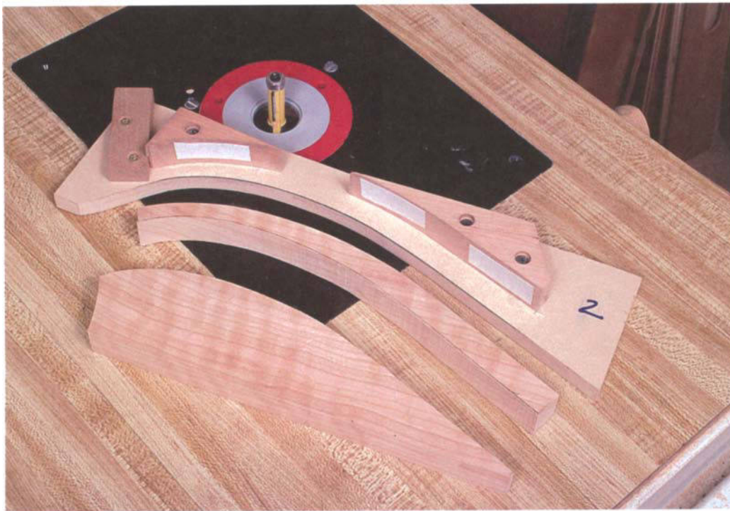
PHOTO L: After bandsawing just outside of the pencil line, the slat is ready to be mounted in template jig 2 for routing the concave edge.
