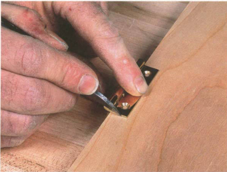
PHOTO B: Hold the hinge down firmly and scribe around the perimeter of the leaf with a sharp knife. Make your first pass a light one to prevent shoving the hinge. Deepen the outline on the second pass.
