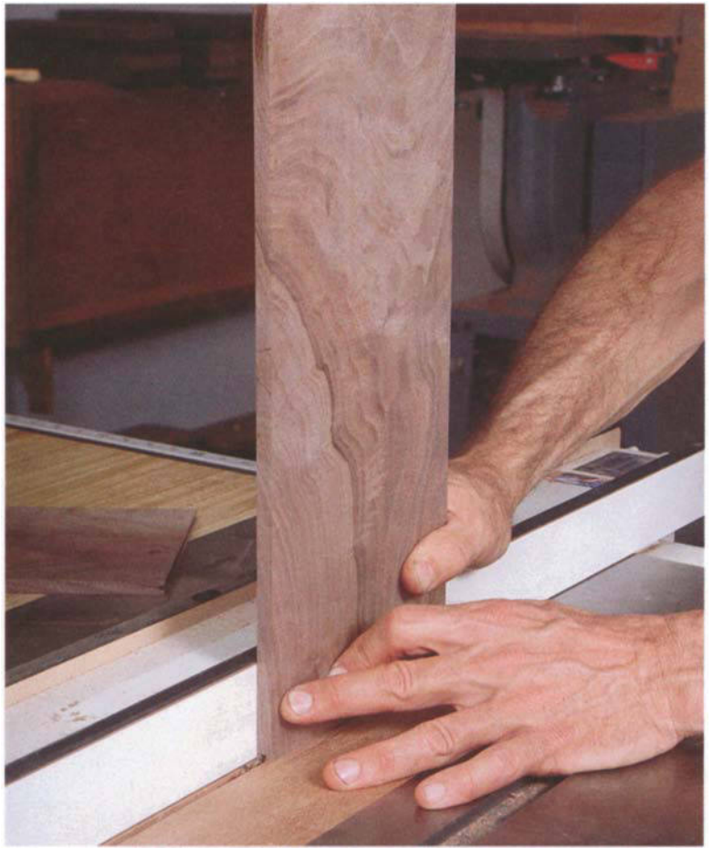
PHOTO B: To make the rabbets on the box tops and bottoms, first cut each tongue to thickness, sliding it firmly against the table-saw rip fence.
