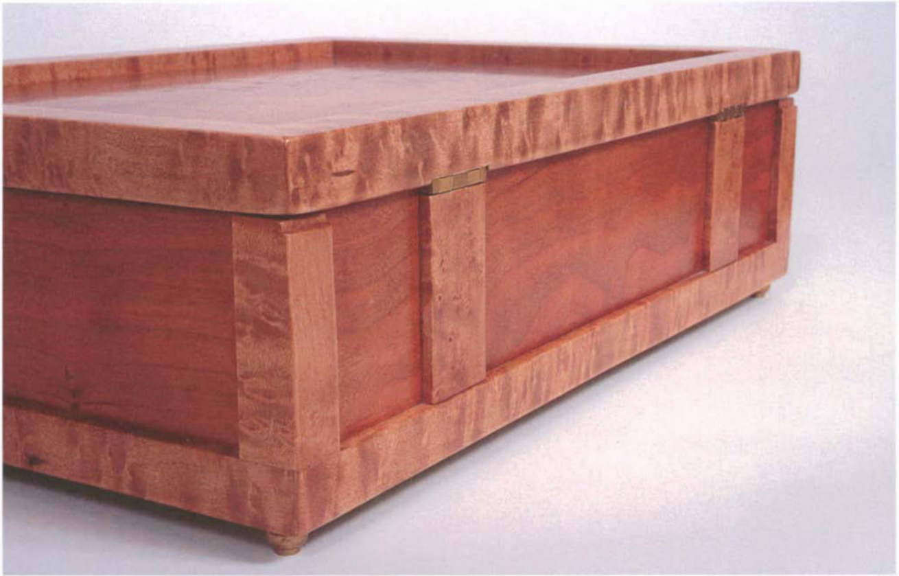
PHOTO C: Cut a small notch in the upper ends of the rear trim pieces to accommodate the swing of the lid. The rear vertical trim pieces fill in the hinge overhang.
