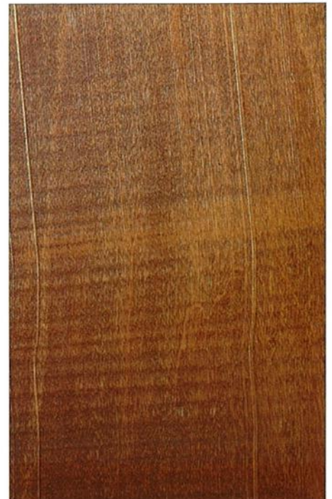
All power cutting and shaping tools leave marks in the wood that must be sanded out. The "washboarding" shown here is caused by a jointer or planer.
