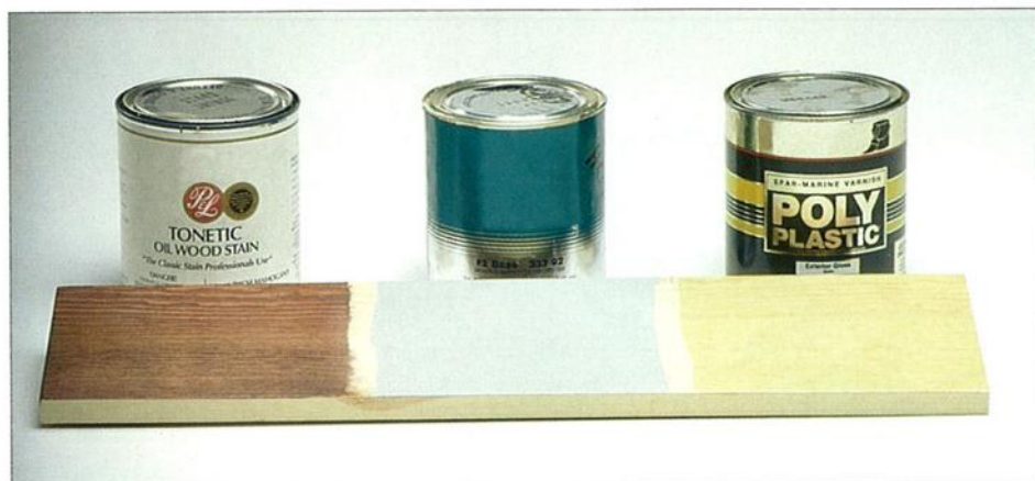
Stains, paints, and finishes (from left) are each made with only three main ingredients. Stains and paints are colorant (usually pigment), binder, and solvent or thinner. Finishes are simply binder, with a solvent or thinner usually added.
