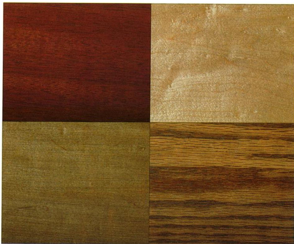
The same stain looks different on different woods. Here the same stain was applied to mahogany (top left), maple (top right), poplar (bottom left), and oak (bottom right). The stain looks very red on mahogany because mahogany is red to begin with. The stain has only a slight effect on maple because maple is a dense, tight-grained wood that absorbs little stain. The stain darkens poplar because poplar is porous. The stain darkens and highlights the grain of oak because oak is porous with a pronounced grain.
