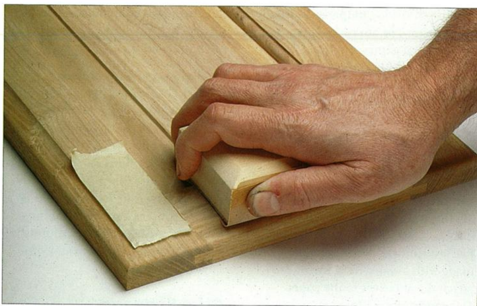
Use masking tape to protect a stile from cross-grain scratching while you sand the rail.
