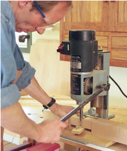
NOTCH IT. After cutting the mortises for the rail tenons, the author uses a hollow-chisel mortiser to notch the posts where they accept the corners of the cabinet top and cabinet bottom.
