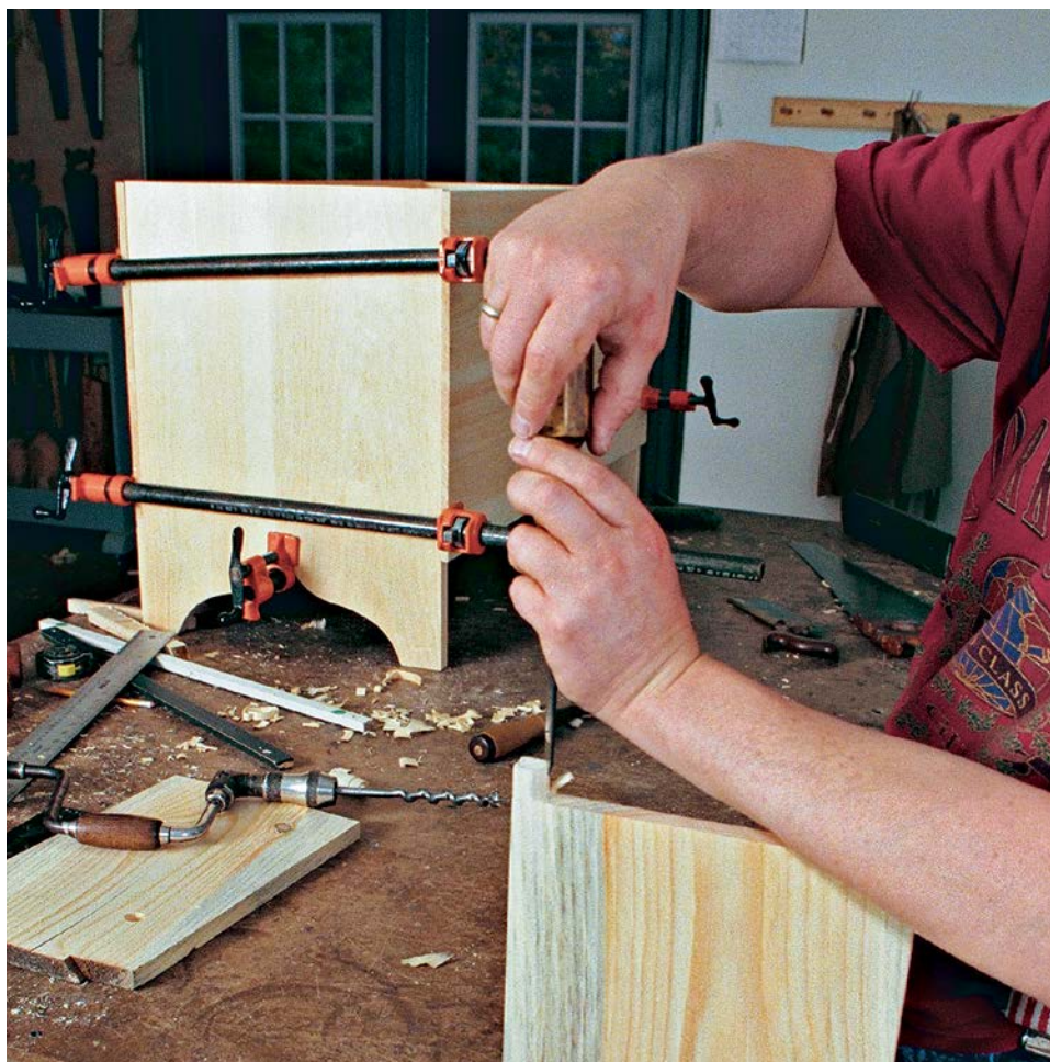
WOOD HINGE FOR THE TILL. After clamping the chest together for a test fit, mark the dados for the till. The till's lid hinges on lugs, small round tenons made by removing a strip of wood from each end of the lid and rounding off the remaining stub with a chisel.
