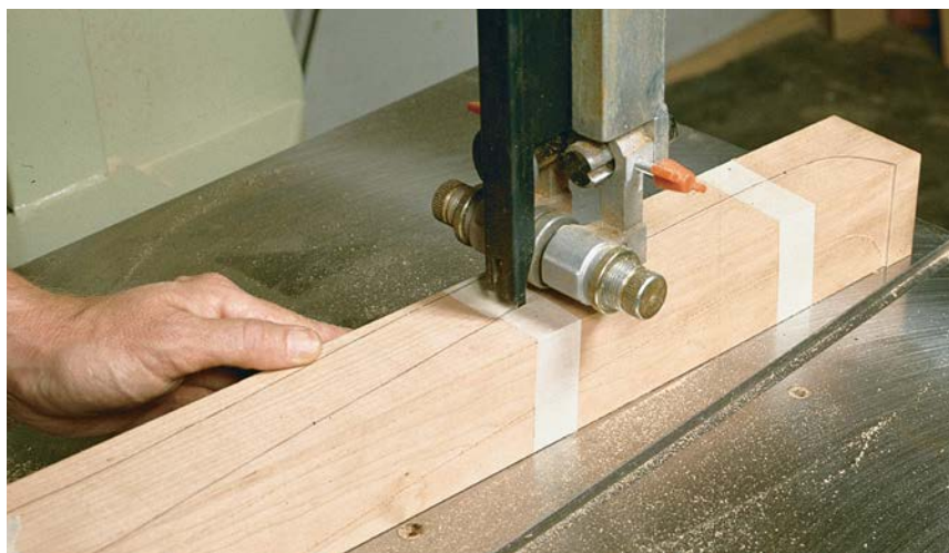
BILLET REBUILT. With the blade guide lowered to just above the stock, bandsaw along the layout lines. Tape the cabriole cutoffs back in place, and turn the billet 90^\circ to make the second pair of cuts. After turning the foot, clean up the bandsawn curves with a spokeshave.
