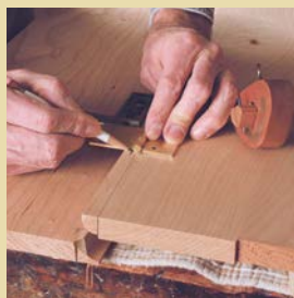
LOCATE THE HINGE BARREL. Square a line up from the quirk.
