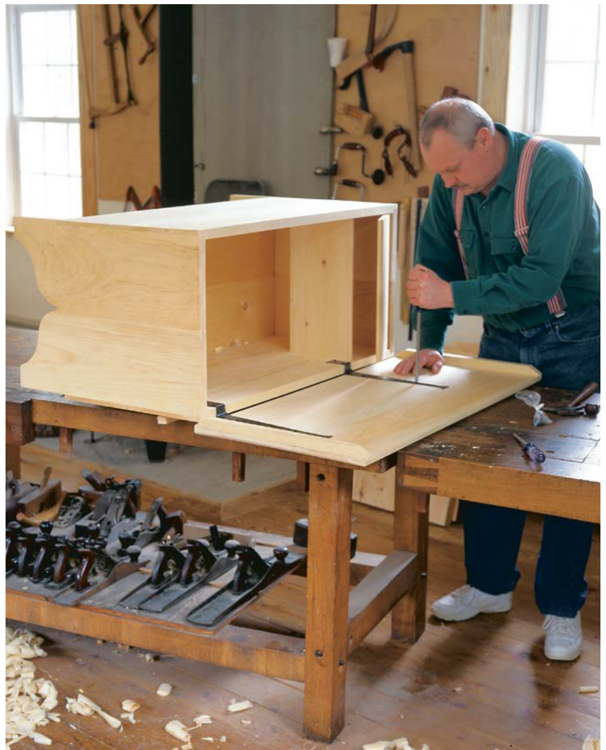
WHITE PINE CHEST MADE THE OLD WAY. Using sharp hand tools, the author made a blanket chest in a few afternoons. The till—a box within the box—is used to hold small items.
