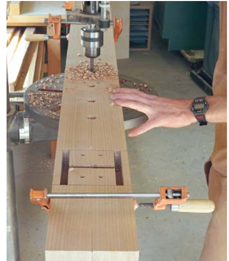
DOUBLE DRILLING. Pairing up the posts makes it easy to cut the half-round notches for the shelf-support bars. It also ensures the notches will correspond exactly in height.
