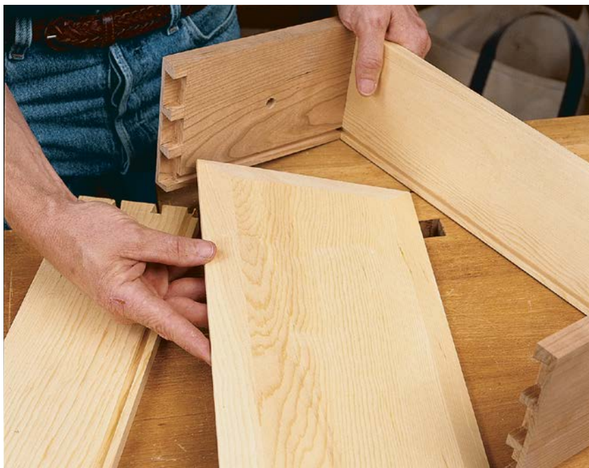
ASSEMBLE THE DRAWER WITH THE BEVEL DOWN. The pine bottom floats in grooves in the pine sides and in the cherry drawer fronts.
