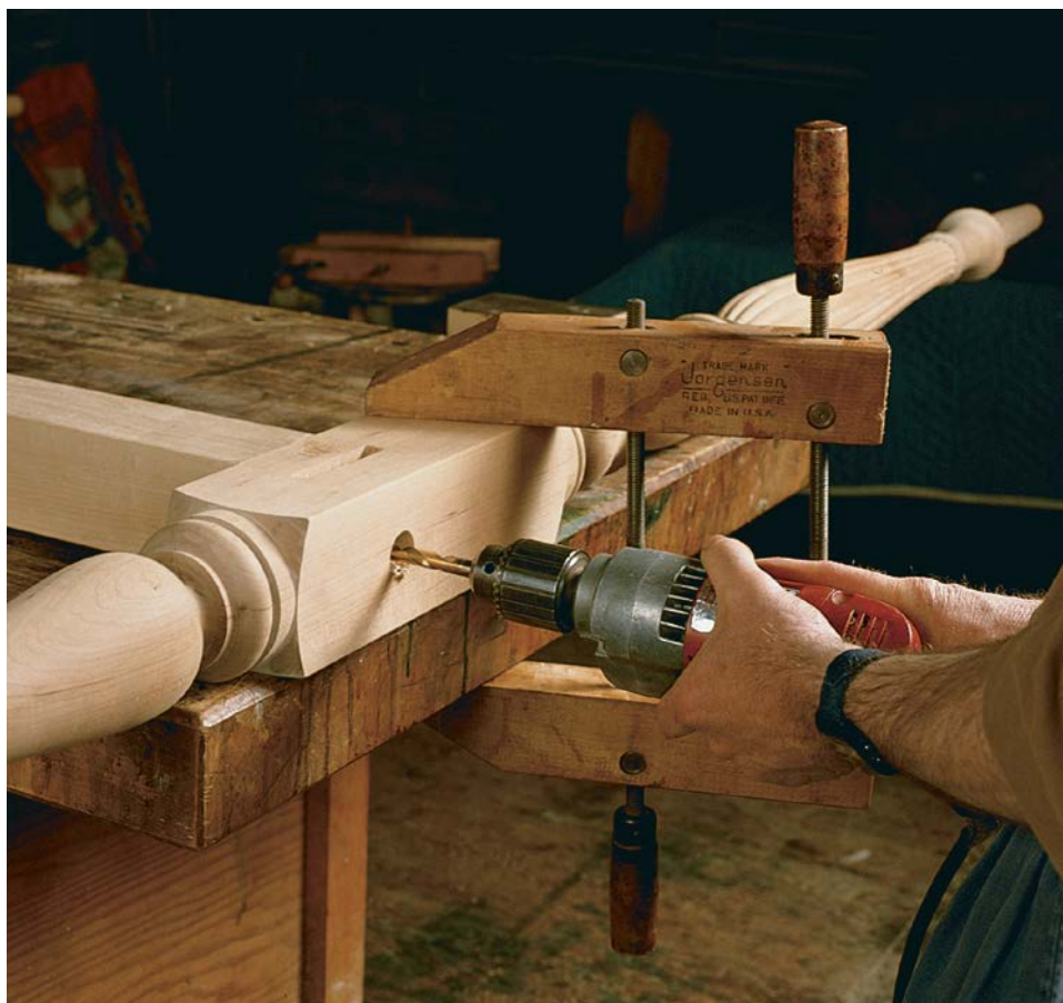
DRILLING HOLES FOR BED BOLTS. Holes bored through the bedposts serve as guides when drilling rails for the bed bolts. The nut is hidden in a mortise in the side of the rail.
