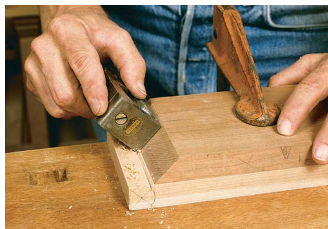
RUN A RABBET PLANE ALONG A GUIDE BLOCK to cut the chamfer that limits the swing of the knuckle joint hinge.
