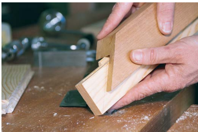
FOR CLEAN MITERS, USE A GUIDE. Rabbets on door stiles and rails meet in a miter at inside corners. For tight-fitting joints, the author pares pieces with the help of a guide block cut to a 45° angle.
