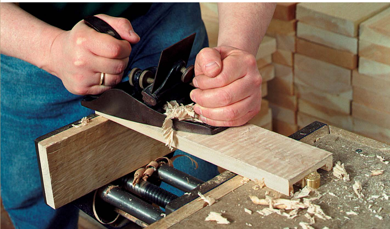
SCRAPER PLANE FOR DRAWER VENEER. After cutting the veneer flush with the drawer front, use a scraper plane to finish the veneer.
