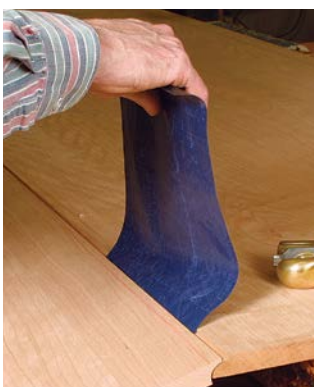
CARBON PAPER STILL HAS A USE. Becksvoort holds carbon paper between the joint as he opens and closes the leaf. Black marks are left where the joint is too tight. Those spots are trimmed with sandpaper or a block plane.
