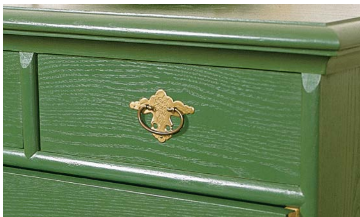
PAINT PRONOUNCES THE TEXTURE. On a coarse-textured wood like ash, an opaque finish brings out the grain while hiding the color. The author left the ash case and drawer fronts unprimed to keep from filling the pores. He used painter's tape to mask the drawer sides and drawer openings. The interior finish is shellac.
