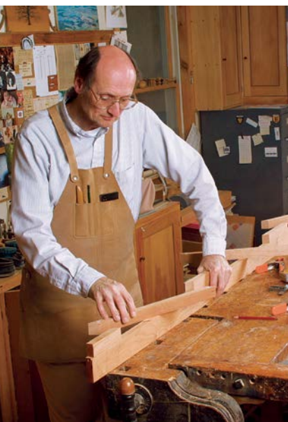
LET IT SPIN ON A NAIL. Becksvoort uses nails to act as pivot pins, because they are stronger than brass and can be let into a smaller hole.
