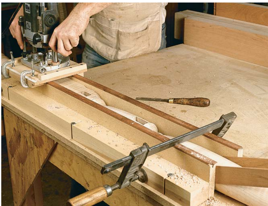
ROUTING BED-POST MORTISES. With a post wedged in this jig, you can easily rout mortises for the rail tenons whether the post is turned or shaped. Then, just use a chisel to square the mortises' corners. For adjustability, the router base slides in tracks in the carriage, and one of the jig's rails has slots for its mounting screws.
