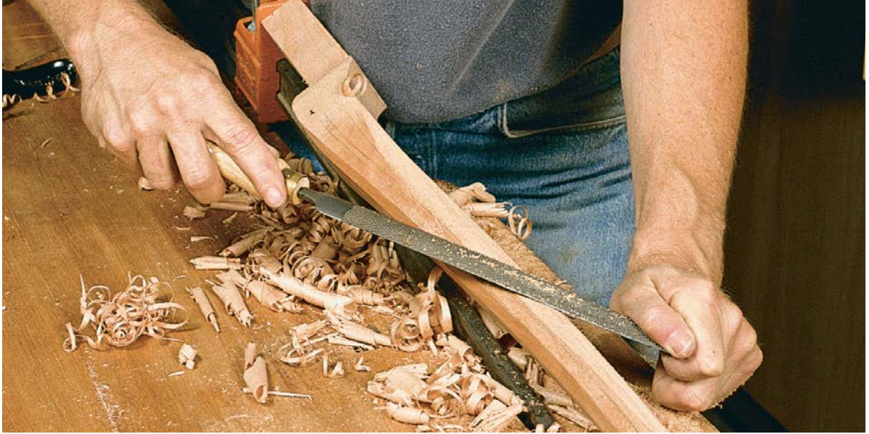
SHAPING THE FOOT. Only the lower part of the foot and the pad are shaped on the lathe. To provide good purchase for the live center, leave the leg full-sized above the knee until after turning.
