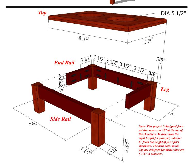
Use the figure above and the Cutting Diagram on Page 2 as guides to cut the parts to size and shape and to drill pocket holes. Set your Kreg Jig and drill bit for 3/4" stock.
