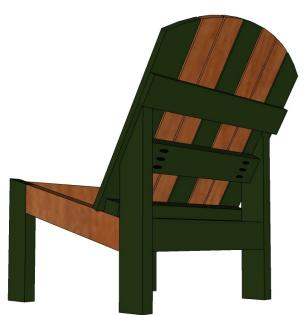
Position the Back Assembly so the Bottom Back Support is flush with the short side of the 30-degree miter on the Back Legs, and the bottom of the End Back Slats rest against the Side Rails and Base Support assembly.
