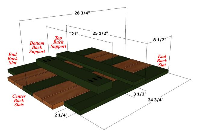
Position the End Back Slats and Center Back Slats 1/4" apart and flush at one end. Use 1/4" stock for spacers. Clamp the Slats in place on your work surface. Position the Top Back Support as shown, and attach using glue and 1 1/4" deck screws (use at least two screws for each Back Slat).
