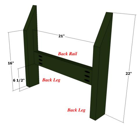
Drill three pocket holes on each end of the Back Rail - one centered and two 3/4" from each side.
