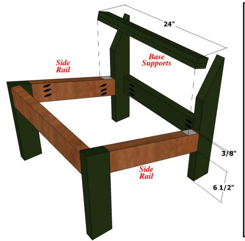
Cut the Side Rails to length with parallel 15-degree miters on each end. Use the illustration for marking the location for three pocket holes on each end.
