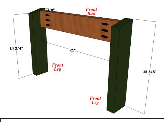
Drill three pocket holes on each end of the Front Rail - one centered and two 3/4" from each side.
