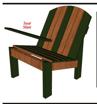
Use a router or sander to create a roundover on the edges of the face that will be positioned up on the Seat Slats. In this illustration, the Seat Slats have been finished in two tones. It's best to do this prior to attaching them to the chair base. Be sure to not apply a finish on any area that will have glue applied.
