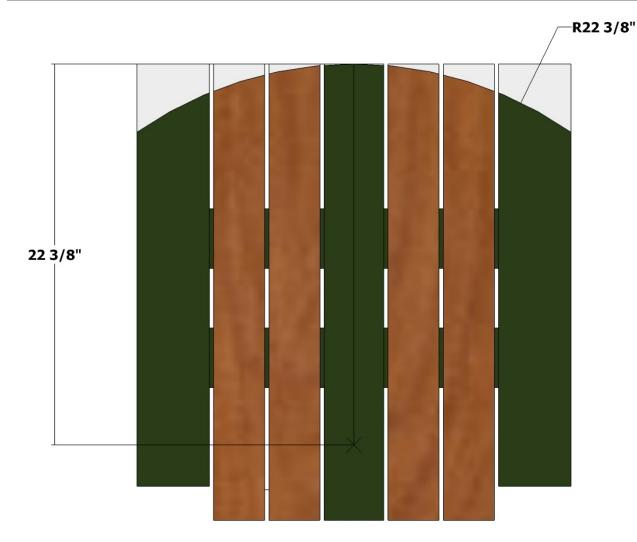
Flip over the Back Assembly and mark a point on a centerline 22 3/8" from the top end of the middle Center Back Slat as shown. Use a bar compass or a string and pencil to mark a 22 3/8" radius across the Back Assembly. Cut away the marked portion to create the back shape.
