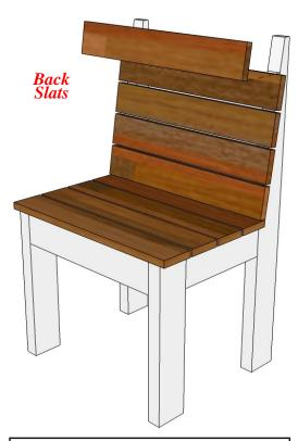
Position the first Back Slat flush against the back Seat Slat and equally spaced across the assembly. Attach using glue and 1 1/4" (DS). Position the remaining Back Slats 1/8" apart and attach using the same method.
