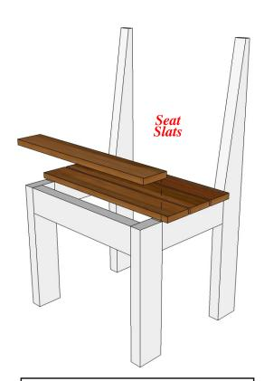
Position the first Seat Slat flush against the back legs and equally spaced across the assembly. Attach using glue and 1 1/4" deck screws (DS). Position the remaining Seat Slats 1/8" apart and attach using the same method.
