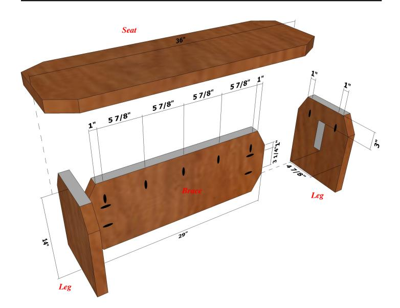
Use the figure above and the Cutting Diagram on Page 2 as guides to cut the parts to size and shape and to drill pocket holes. Set your Kreg Jig and drill bit for 1 1/2" stock.
