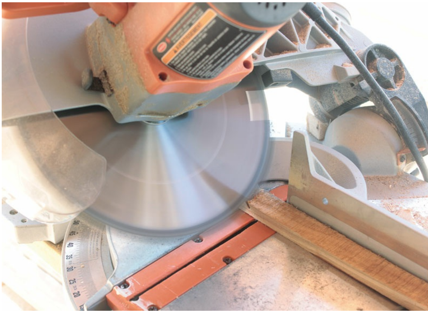
mitering a 45° angle on the edge side
