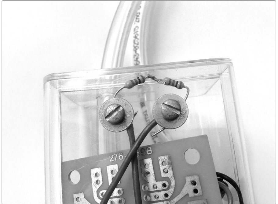
FIGURE 6-21: A set of bridging resistors connect the body contacts, making it easier for my callused old hands to play the Droid Voicebox (the resistors are mounted inside the transparent case, with their leads sandwiched between the washers and nuts).
