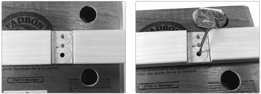
FIGURE 10-15: The hole for my pickup's leads aligns with one of the spade bit's guide holes from Step 11. You can see that more clearly with the pickup wires installed (right).
