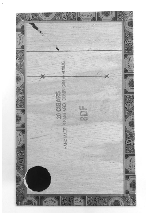
FIGURE 11-7: Placement of the sound hole
