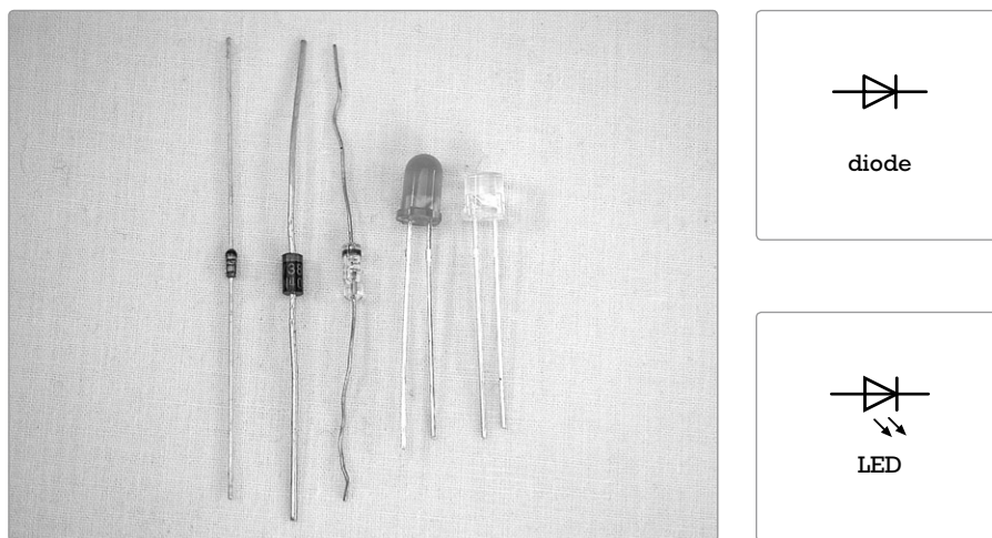
FIGURE A-7: Diodes and LEDs (left), and their symbols (right)
