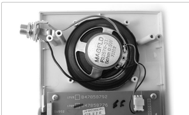
FIGURE 7-6: A “jumped” auxiliary output jack
