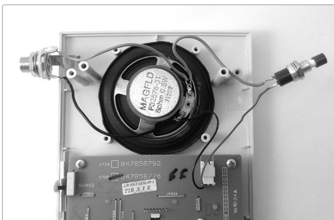
FIGURE 7-7: An auxiliary output with a momentary mute
