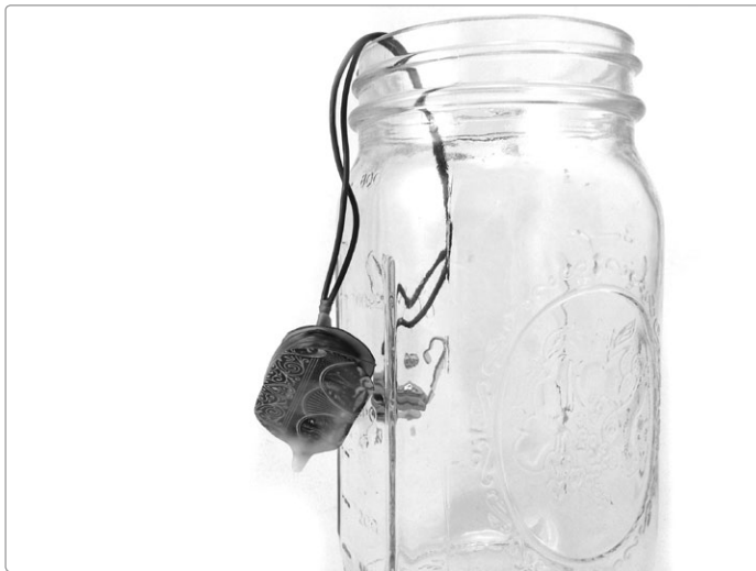
FIGURE 9-8: Drip-drying the potted pickup
