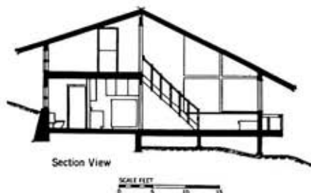
KITCHEN, INGLENOOK tuck under sleeping balcony to help create cozy sense in a one-room house.
