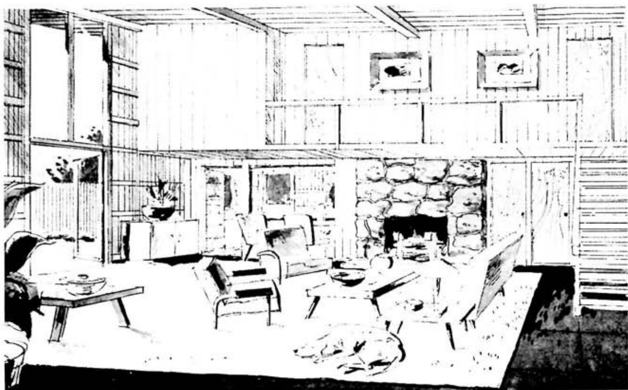
INTERIOR at the final stage, with cabin complete. Balcony which serves as entrance hall to the bedrooms also diminishes the height of inside wall to the scale of the fireplace and hearth. Room size is 15 by 27 feet.
