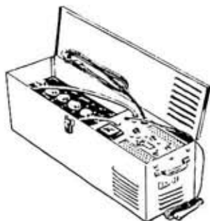
CONVERTER-CHARGER with power of 500 watts good for emergency.
