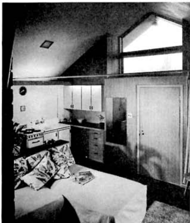
LOW COUNTER separates living and kitchen areas. Interior walls are combed plywood; ceiling is fiberboard.
