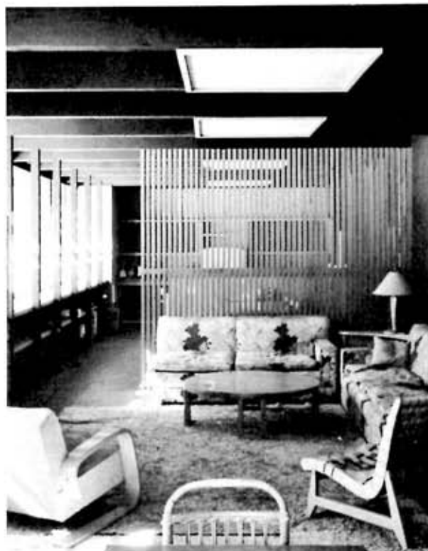
SCREEN of 2 by 4's separates living room from dining room. Perforated wallboard panels close off bedrooms.
