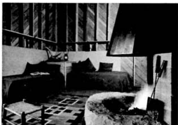
BEDS SWING out to be made. Circle around fireplace is volcanic stone. Back and sides are of firebrick.
