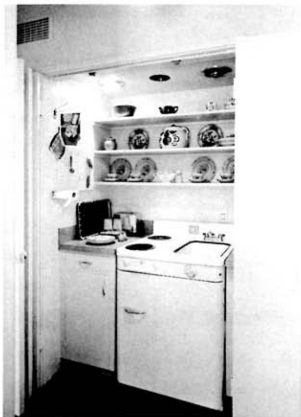
KITCHEN in a closet has combination sink, range, refrigerator plus counter. Design: Burde-Shaw-Kearns.
