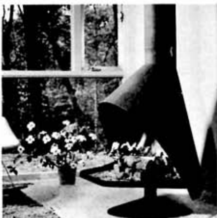
LEFT: Economical hood-type fireplace has 12 square feet of reflecting surface. Design: Wendell Lovett. CENTER: Buoy-shaped metal fireplace, in center of room, radiates heat on all sides. RIGHT: Brick-base fireplace with copper hood and wide metal chimney warms entire room. Design by William F. Hempel.
