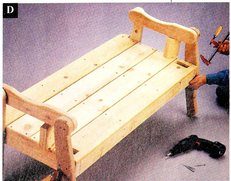
Carefully clamp the leg frames to the seat, and attach them with glue and counterbored screws.
