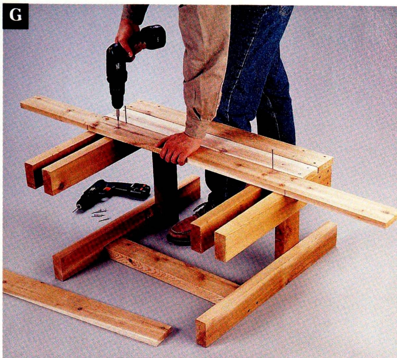
The longer face boards attached to the tall benches overhang the doubled posts so they cover the sides of the short benches when the tree surround is assembled.
