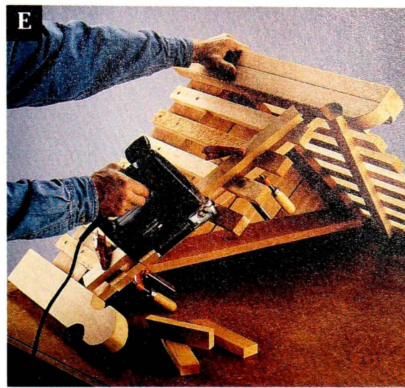
Use a cutting guide to trim the tops of the slats so they are flush with the tops of the stringers.
