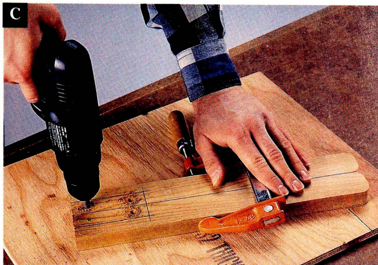
Drill countersunk pilot holes through the posts before you attach them to the handle.
