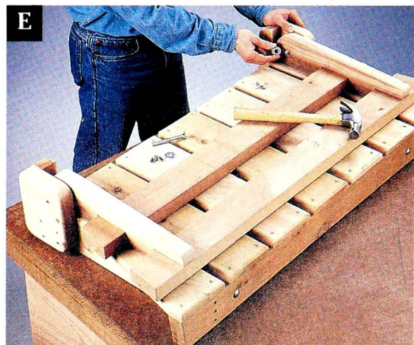
E Attach the backrest to the seat frame with carriage bolts and wing nuts.
