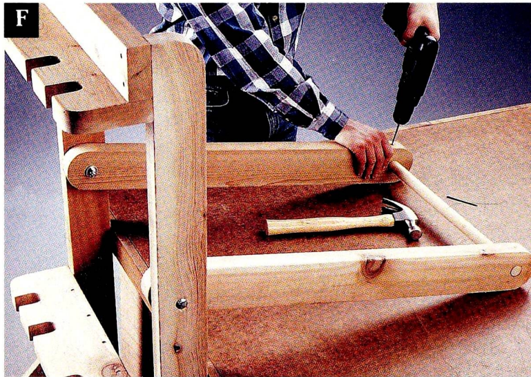
Drill a pilot hole through each arm and into the ends of the handle, then drive a 4d finish nail into the hole to secure the handle.
