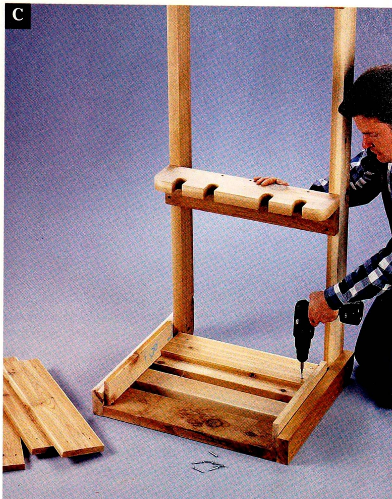
Attach the bin slats to the front supports, leaving a \frac{1}{8} "-wide gap at both ends of each slat.
