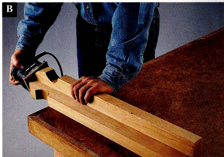
Sand the top of the corner post assembly so the joint is smooth.
