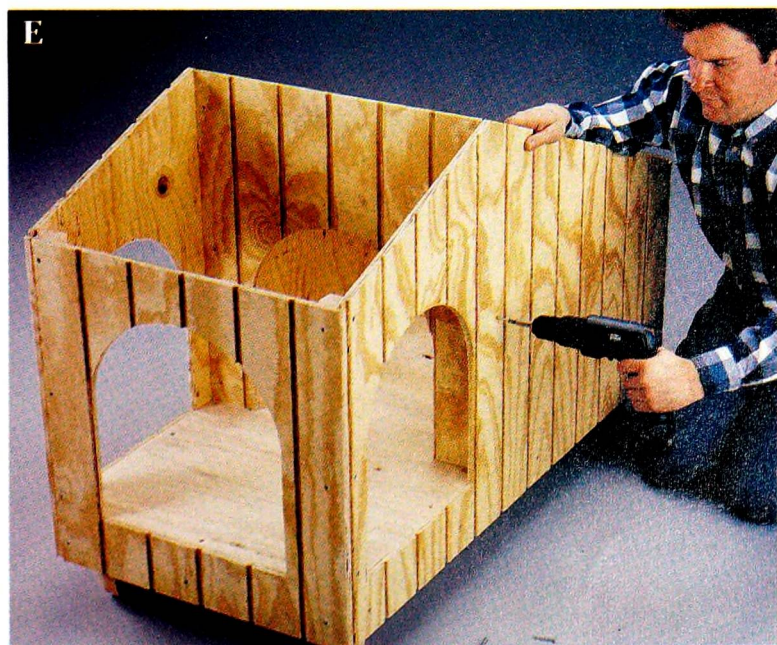
Fasten the center panel by driving screws through the side panels into the cleats. Use a combination square to keep the panel even.
