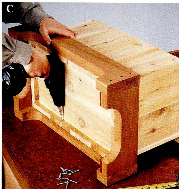
The recess beneath the bottom boards in the planter bin provides access for driving screws.
