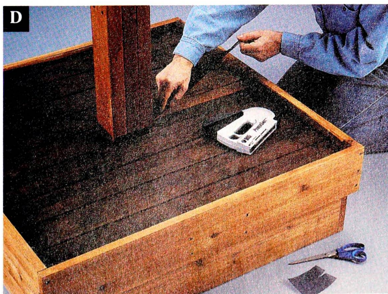
Staple window screening over the tops of the floor boards to keep bird food from falling through the gaps.
