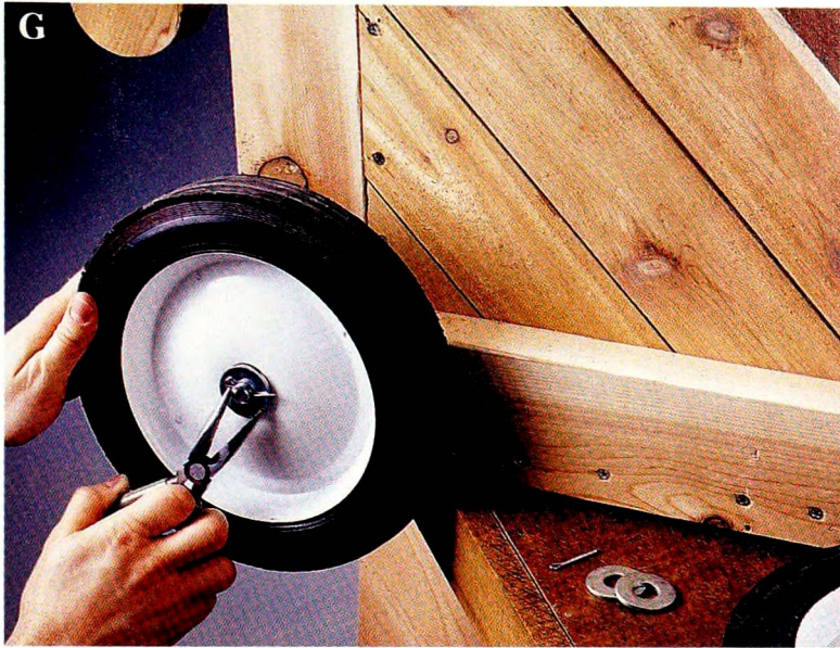
G Secure the wheels by inserting a cotter pin into a hole at the end of each axle, then bending down the arms of the pin with pliers.
