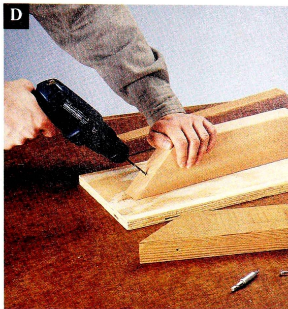
Before attaching the cap ends, drill pilot holes through the mitered ends of the cap front ends.
