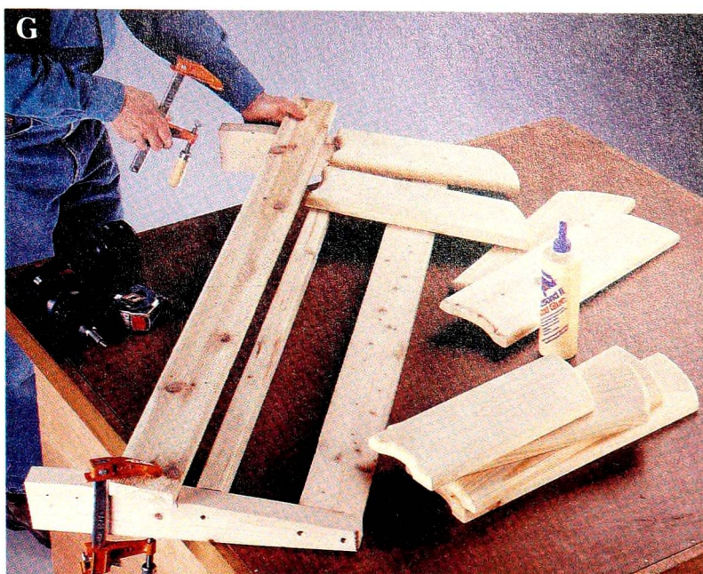
Clamp a straight board to the back frame to help keep the back slats aligned along their bottom edges as you install them.
