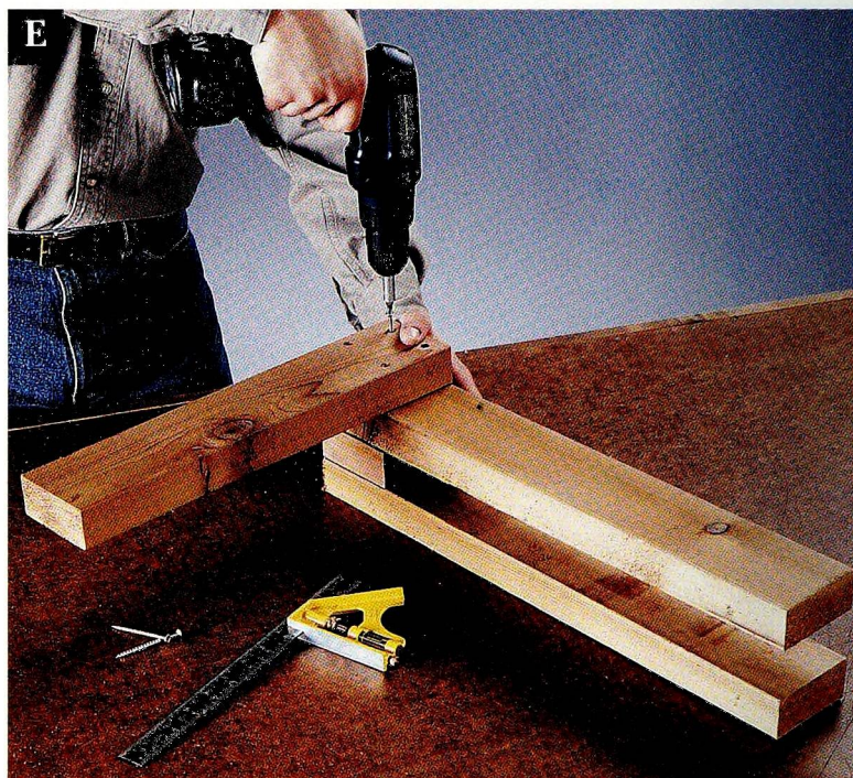
After making doubled posts for the tall benches, attach the seat rails.
