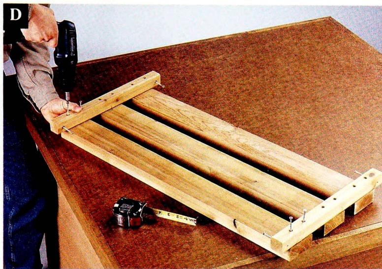
D Fasten the bottom cleats to the shelf slats, keeping the ends of the slats flush with the outside edges of the cleats.
