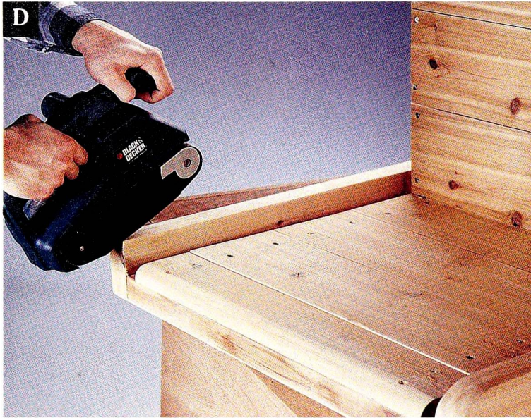
Round over the tips of the front supports and the front edge of the end slat, using a belt sander.
