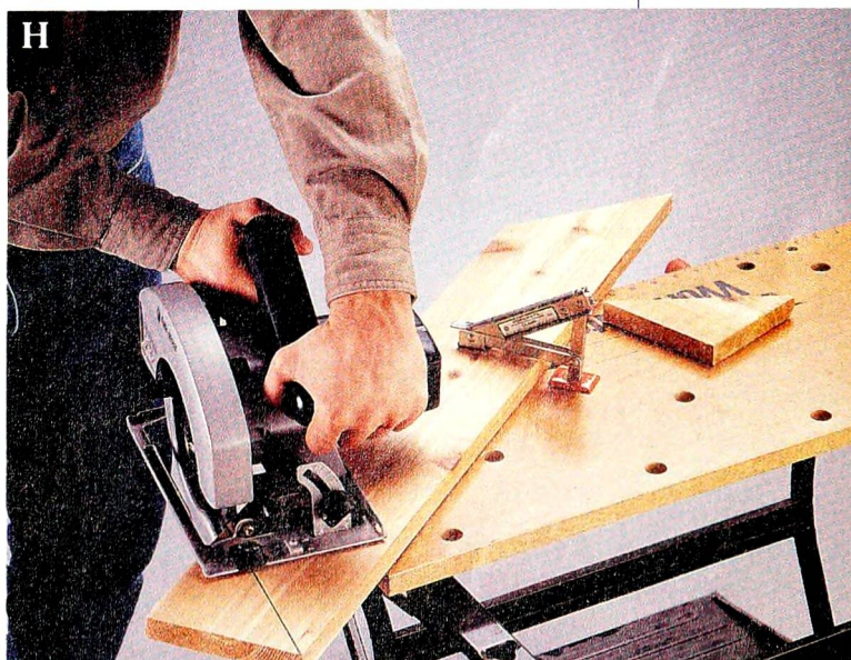
The 1 × 6 caps are mitered to make a square frame around the top of the tree surround after it is assembled around your tree.
