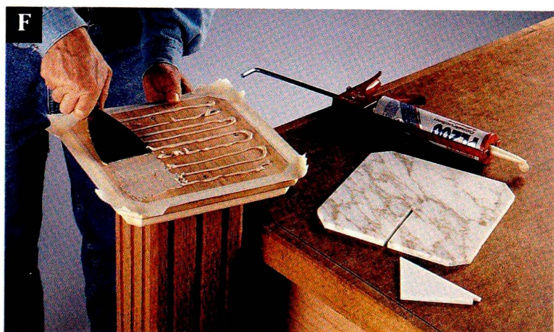
F Frame the top of the top outer plate with masking tape, then apply a layer of construction adhesive to attach the sundial face.
