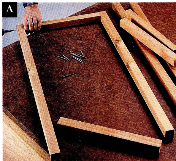
A Fasten the cleats between the rails to construct the panel frames.
