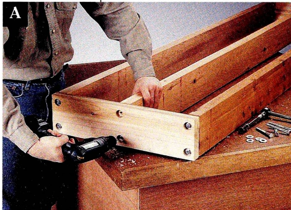
Use a smaller bit to extend the pilot holes for the lag screws into the ends of the bottom rails.
