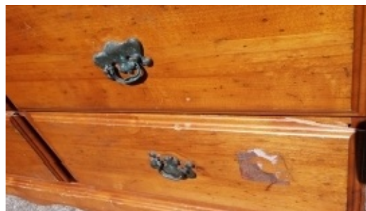
Image 3: Drawer Issues: You can see where the drawer front broke off. It had to be fixed. Find out how.
