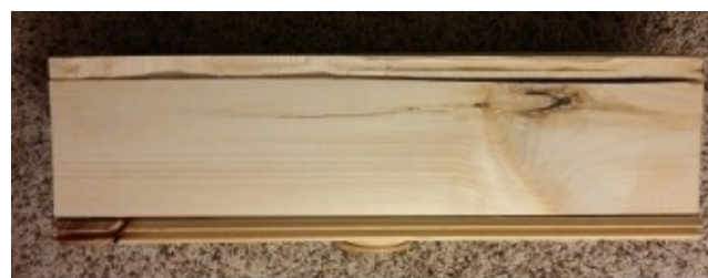
Bottom of the drawer Note the bottom piece fits between the front and back.
