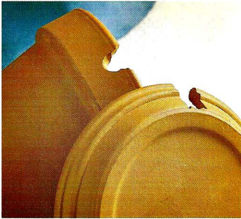
Cutting mouse holes for water flow and the electrical cord in terra cotta pots and underliners is a simple process with a multi-purpose drill bit.
