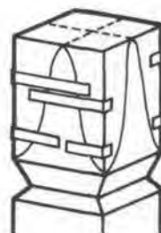
Tape the waste back on to make remaining cuts
