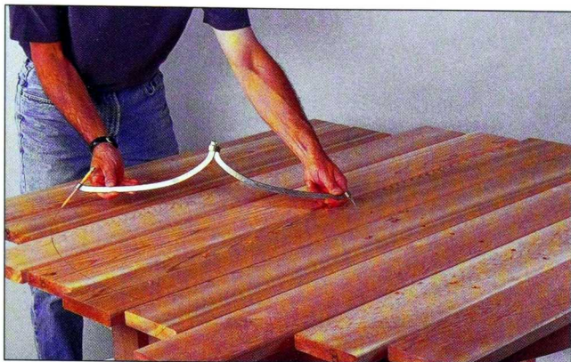
Fig. 11 Space the boards equally, and screw them to the crossrail. Draw the outline of the top on the boards so that you can cut the diameter with a sabre saw.
