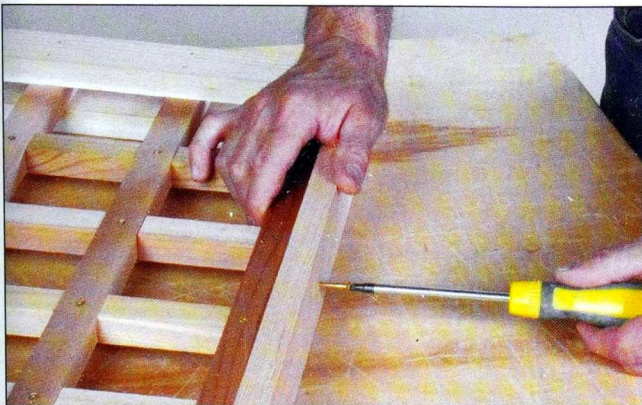
Fig. 5 Nail the vertical end strips to the top and bottom rails, and add screws between the horizontal lattice members.
