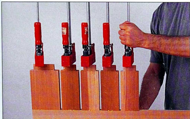
Fig. 14 The first stage in assembling a benchtop is to glue and clamp slats to one stile. Use one clamp in the center of each slat.
