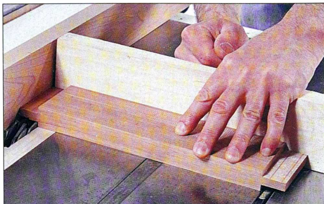
Fig. 7 Use a dado blade setup in the table saw to cut the tenons on the apron pieces. Butt each apron to the fence, and make the cut.
