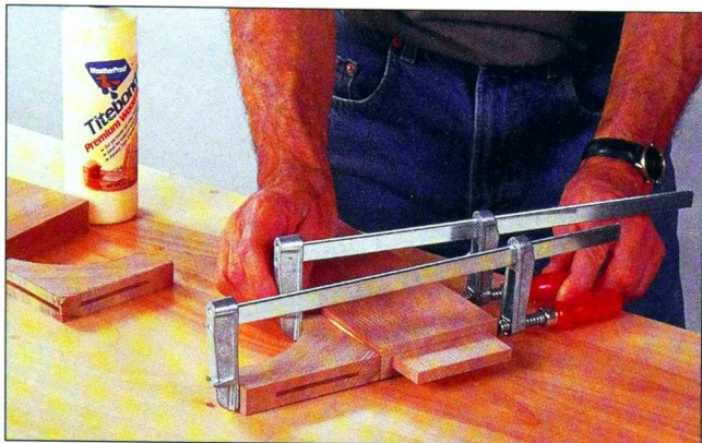
Fig. 4 Apply glue to the joining-plate slots and the plates, and join each bracket to a leg. Clamp until the glue sets.
