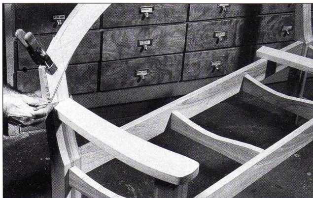
Fig. 14 Dry assemble the bench with the arched rail clamped in place. Lay the armrest on the front leg and trace the position on the rear leg.
