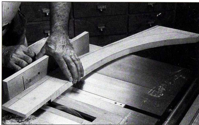
Fig. 10 On each half of the arched rail, first cut the inside curve. Make a flat edge tangent to the curve, then cut the half-lap.
