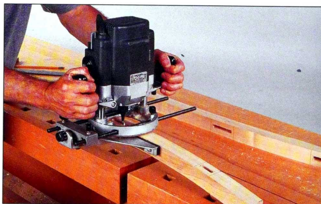
Fig. 14 Use a plunge router with its fence positioned on the leg's straight face. Cut the side rail and stretcher mortises.
