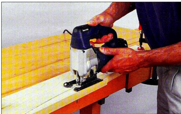
Fig. 2 Clamp the workpiece to the bench, and saw the chair sides to shape using a sabre saw held to the waste side of the line.
