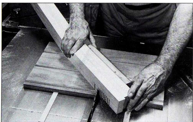
Fig. 5 Hold the legs on a sliding platform and make repeated deep kerf cuts to form the angled half-lap for the arched back rail.
