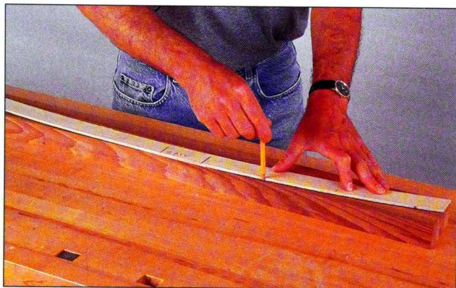
Fig. 12 The first step in building each cedar chair is to make a precise template for the rear leg, and trace the shape on the leg blanks.
