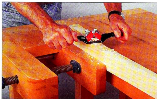
Fig. 3 Clamp the seat supports and the back supports in a sturdy vise, and smooth out the sawn surfaces using a spokeshave.
