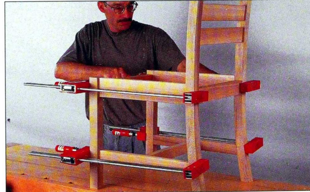
Fig. 19 Glue and clamp together the rear leg subassembly, the front legs, and the stretcher subassembly.
