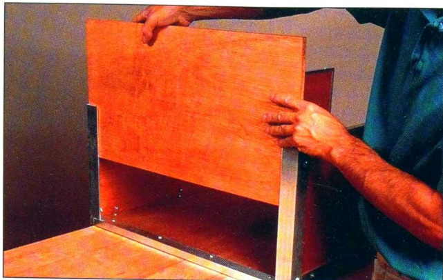
Fig. 12 Test fit the sliding plywood panel. If it sticks a little, apply lubricant such as Teflon spray to the panel edges and to the channels.
