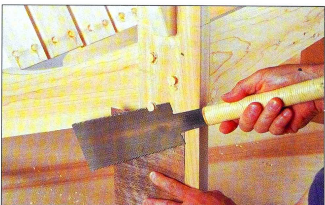
Fig. 16 Place a veneer shim under a fine-cutting pull-stroke saw, and cut the plug nearly flush with the workpiece surface.
