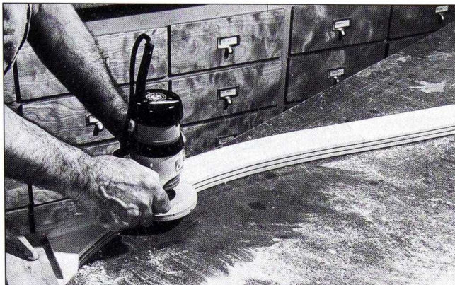
Fig. 13 Cut the groove in the arched rail using a slotting cutter and router in a series of passes. Clamp the stop block to the rail.
