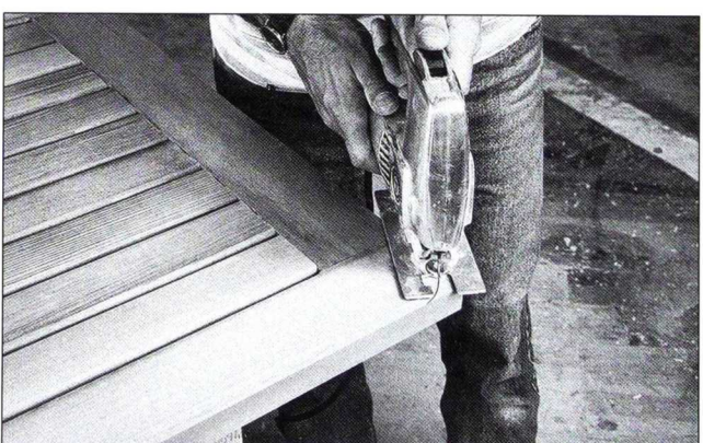
Fig. 17 Carefully cut the radius on each top corner of the table using a sabre saw and staying just to the waste side of the line.
