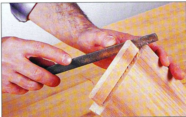
Fig. 9 Round off a tenon with a rasp. The tenon's radius matches the radius left by the spiral up-cutting bit used to cut the mortise.
