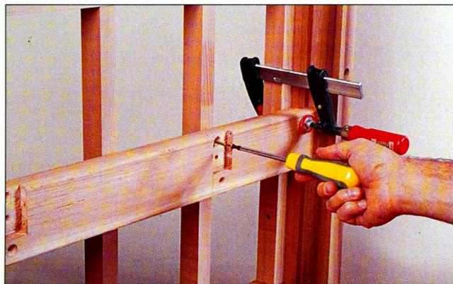
Fig. 14 Turn the trellis upright to install the seat frame parts. Then disassemble the trellis and take it to the site for installation.
