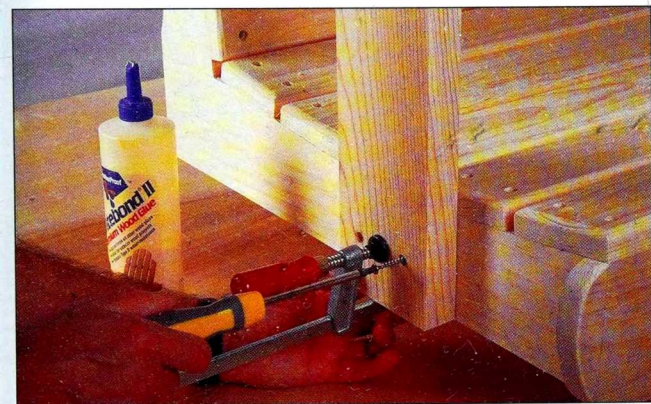
Fig. 12 Clamp each arm support in place, and bore pilot holes through it. Next, fasten the workpiece with galvanized screws.
