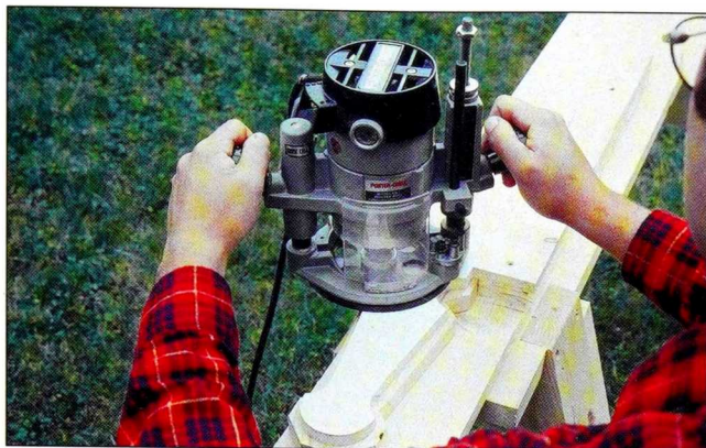
Fig. 3 Use a router with a 1/2-in. bit, 1-in. guide bushing, and a picket jig to trim the rough pickets to the finished shape.
