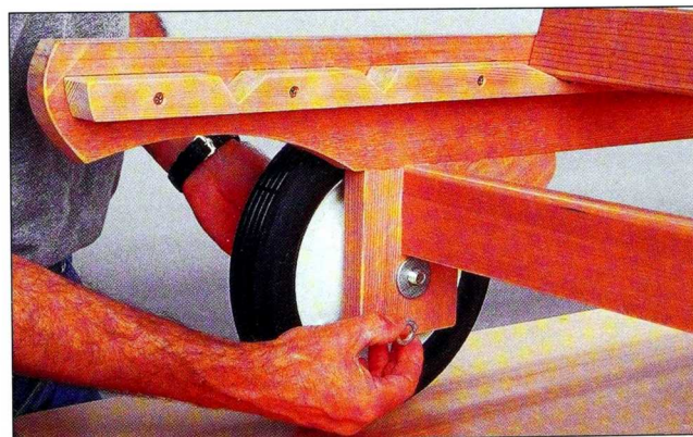
Fig. 12 After filing away the square shoulder on 1/2-in. carriage bolts, use the bolts as axles to support the wheels.
