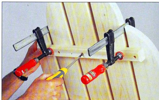
Fig. 12 After all the back slats are installed, clamp the back support in place, and attach it to the back slats with screws.
