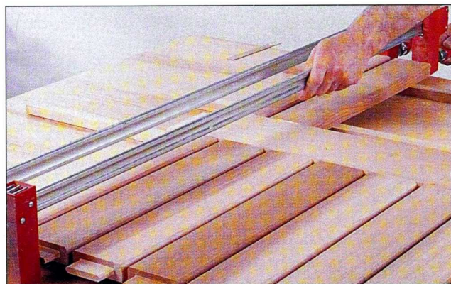
Fig. 16 A second set of slats is glued and clamped to the center rail. Again, use one clamp in the center of each slat.
