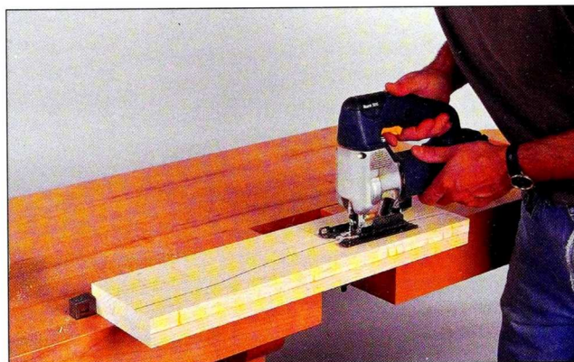
Fig. 2 Clamp a seat support blank in a vise and cut the curved edge using a sabre saw. Keep the saw just to the outside of the line.
