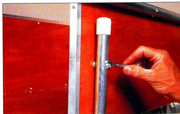
Fig. 20 Cover tubing ends with furniture caps. Use three washers between the leg and the sides. Cut off the excess screw shaft, and file it smooth.
