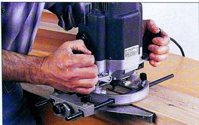
Fig. 6 Using a spiral up-cutting bit in a plunge router, cut the table leg mortises. Two legs clamped together provide a stable base.
