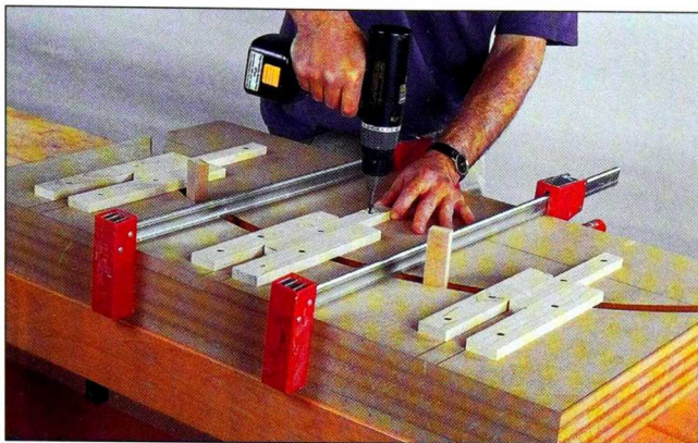
Fig. 3 Use 3/4-in.-thick spacers between the bending form pieces. Clamp the form pieces together and fasten the alignment strips.
