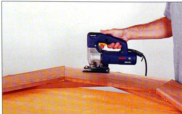
Fig. 12 Use a sabre saw to cut out the arch. Cut on the waste side of the line and smooth the arch with 100-grit sandpaper.
