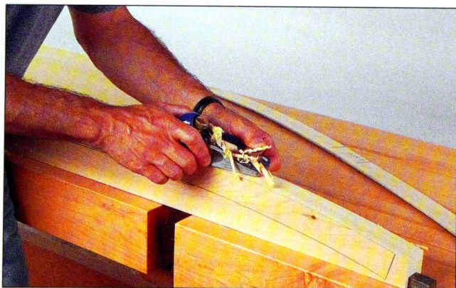
Fig. 13 Cut the outside curve on the leg. Then securely clamp it to the bench, and smooth the curve with a block plane.
