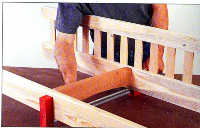
Fig. 16 Use a bar clamp to securely pull the front rail and back rail assembly tight to the center seat-support rail.
