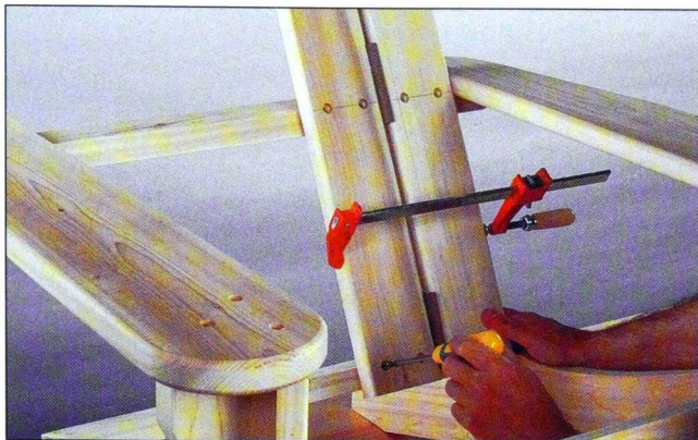
Fig. 11 Fasten the first back slat with screws. Place spacers between it and the next slat. Clamp them, and screw securely in place.
