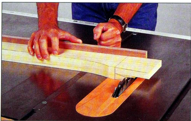
Fig. 4 Install an auxiliary fence on the miter gauge and hold each workpiece to it. Make several passes to cut the half-lap.
