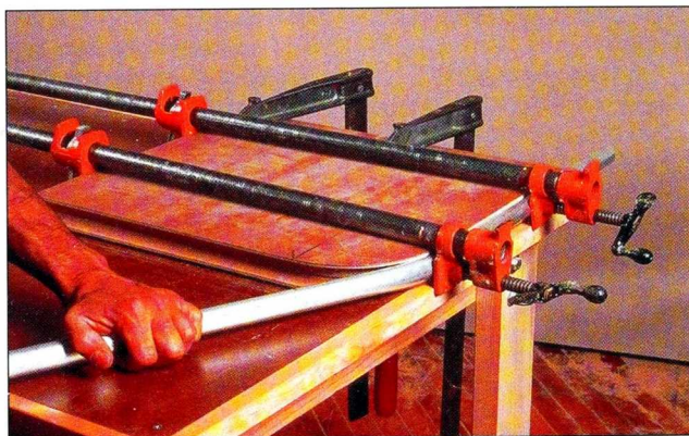
Fig. 19 Align the marks on the tubing with those on the jig, and clamp the bending jig securely to the workbench.
