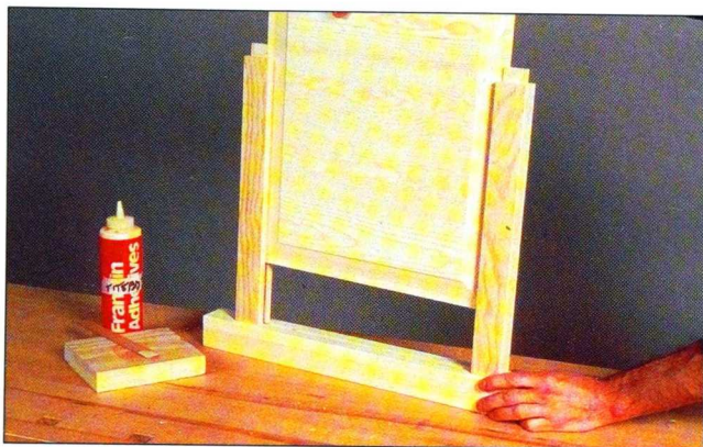
Fig. 6 Begin assembly by gluing two rails to one post. Then slide the panel into the grooves, add the opposite post, and clamp the joints tight.
