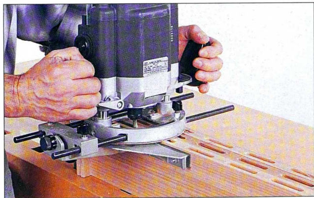
Fig. 10 To cut the long row of mortises in each stile and rail, clamp three of the workpieces together to support the router.
