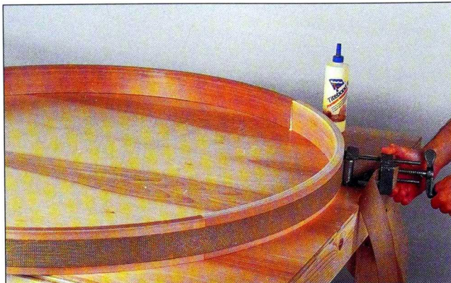
Fig. 8 Glue and clamp the apron sections together using a strap clamp. Check its diameter at several points to ensure true round.
