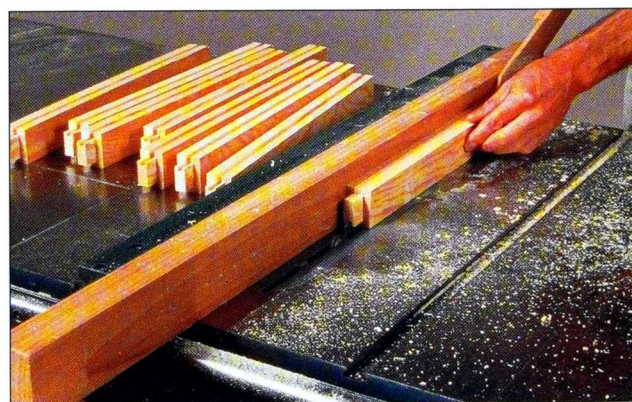
Fig. 3 Reset the dado blade and make the \frac{1}{4} -in.-wide x \frac{1}{2} -in.-deep grooves in each rail. Use a pushstick to move the work safely.
