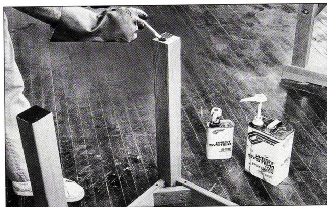
Fig. 19 To prevent water penetration and the resulting staining, apply two coats of epoxy on the bottom of each leg.
