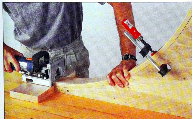
Fig. 7 Transfer the cradle to a sturdy bench, and use the cradle to hold the apron section in place while cutting the biscuit slots.
