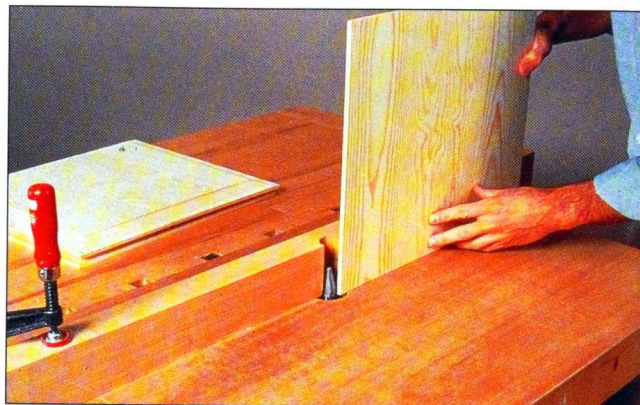
Fig. 5 After trimming the panel to exact size, cut the raised panel profile on a router table with a vertical panel-raising bit.
