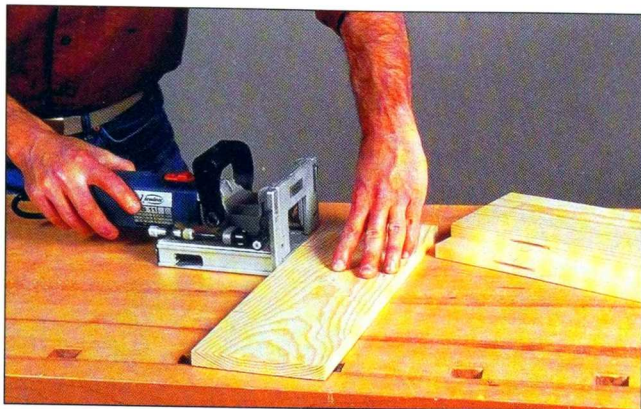
Fig. 4 Make the side panels by gluing the narrower stock pieces together. Use a plate joiner to ensure good alignment of the pieces.
