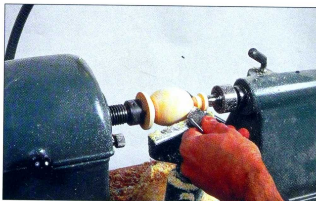
Fig. 9 Use a template as a guide to shape the finials. Leave a stub at the top end and sand while it's in the lathe. Then sand the stub smooth.
