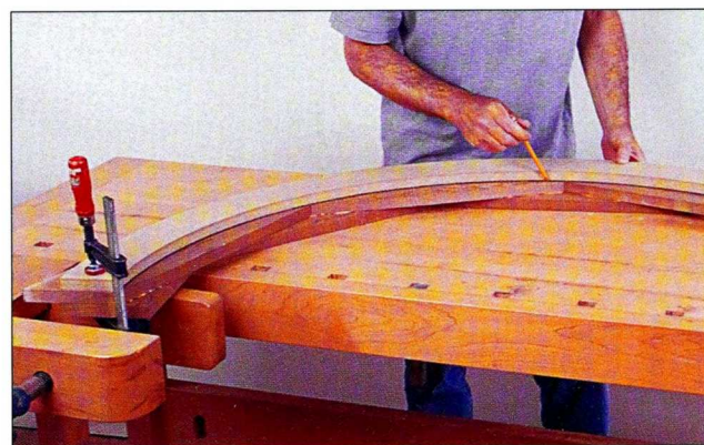
Fig. 11 Clamp the arch pattern to a glued-up blank and trace the shape. Next, mark the straight cuts on the arch ends.
