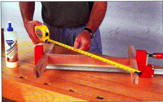
Fig. 17 Glue and clamp together two side stretchers with a cross stretcher. Measure diagonally to check the assembly for square.
