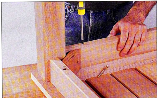
Fig. 20 Attach the tabletop to the base with several screws. Drive each screw into its matching counterbored hole in the apron.
