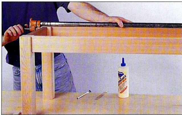
Fig. 13 Join two leg-apron subassemblies spanned by a long pair of aprons. Glue and clamp this to complete a bench base.
