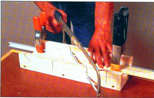
Fig. 5 Cut miters on the ends of the channel stock using a miter box and hacksaw. Support the channel walls with a scrap block.
