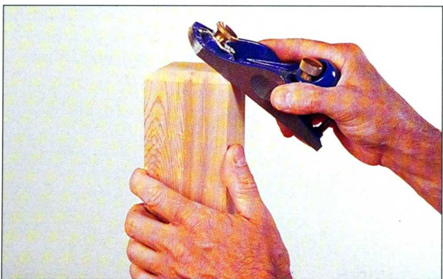
Fig. 7 Crosscut the leg top so that it's square to the angled face of the leg. Use a chisel or block plane to chamfer the end.
