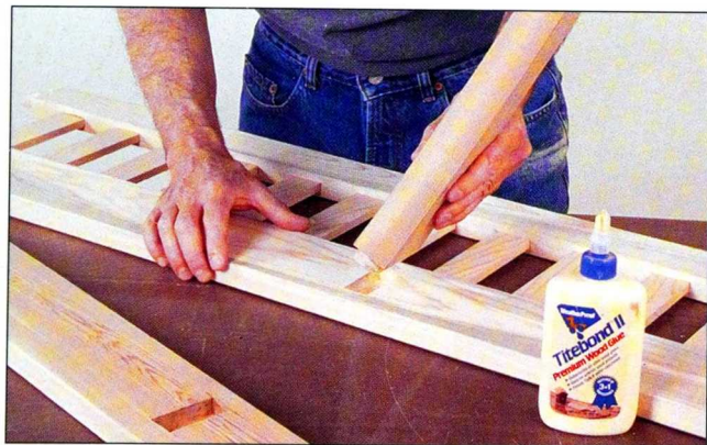
Fig. 15 Spread glue in the shallow center rail mortises and on the seat-support rail tenons. Then go ahead and join the parts.
