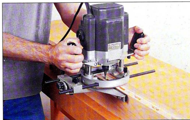
Fig. 10 Rout the slat mortises in the bench rails. Clamp a second board to the workpiece to help support the router base.
