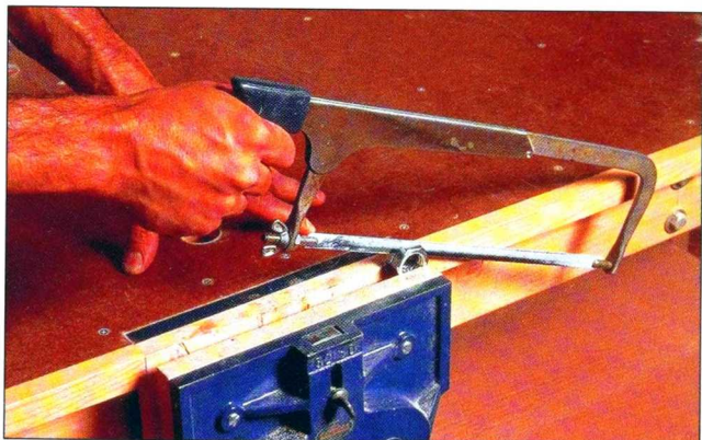
Fig. 15 Clamp the nut in a vise and then slowly saw it in half. Clean up the saw marks with a fine file or a sanding block.
