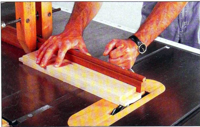
Fig. 16 Clamp a stop to the miter gauge fence. Use a dado blade to cut the tenons on the rails, stretchers, and back slats.
