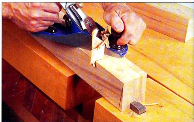
Fig. 4 Use a sharp plane to smooth the sawn surfaces. Switch to sandpaper, spokeshave, or a scraper at the back inside corner.
