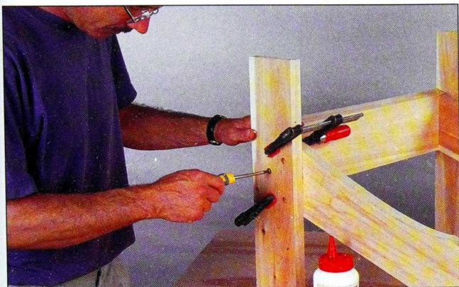
Fig. 7 Spread glue on the joint between the front leg and the chair sides. Hold the parts with a clamp, and drive the screws.
