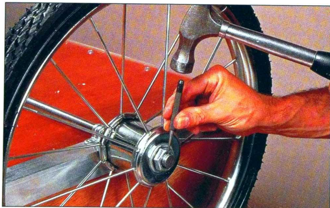
Fig. 16 Temporarily install the wheels and nuts. Dimple the axle using a centerpunch to mark the location of the cotter pin hole.
