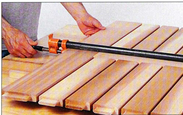
Fig. 17 Carefully glue and clamp a side rail to the center rail. One clamp, precisely centered, should provide enough force.
