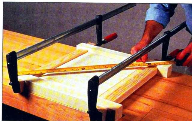
Fig. 7 Check that the assembly is square by measuring opposite diagonals. If necessary, loosen the clamps and adjust the entire piece to square.
