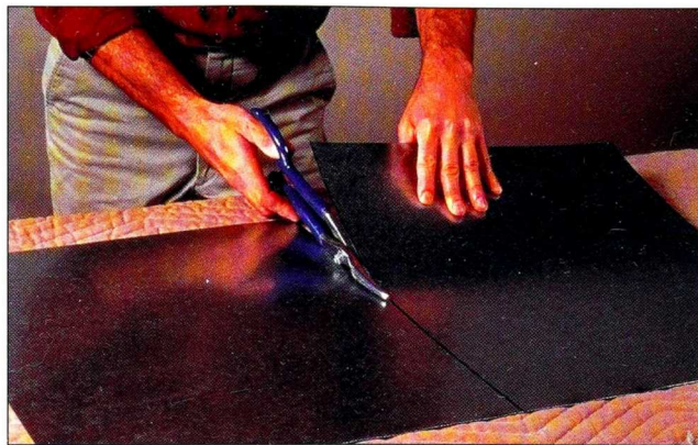
Fig. 10 Use a felt marker and straightedge to lay out, cut, and bend lines on the sheet metal. Make the cuts with heavy-duty shears.
