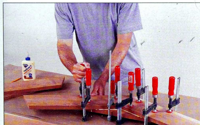
Fig. 9 Carefully glue together the staggered layers that make up each arch blank. Assemble each of these blanks in stages.
