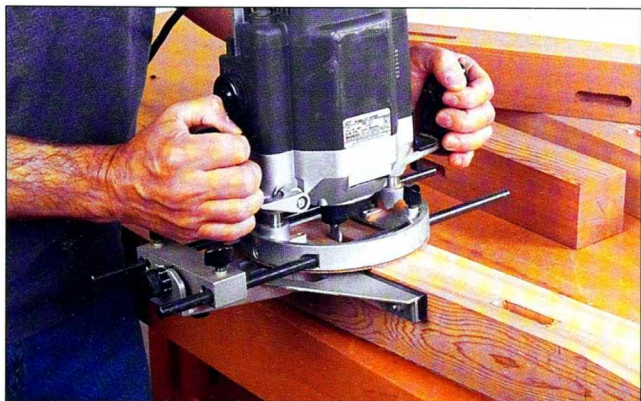
Fig. 5 Mark the mortise locations on the front and rear legs, and use a plunge router and edge guide to make the cuts.
