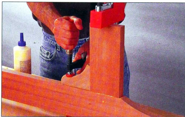
Fig. 5 When the leg/bracket assemblies are finished, join them to the rails. Apply glue to the plate and mortise-and-tenon joints, then clamp.
