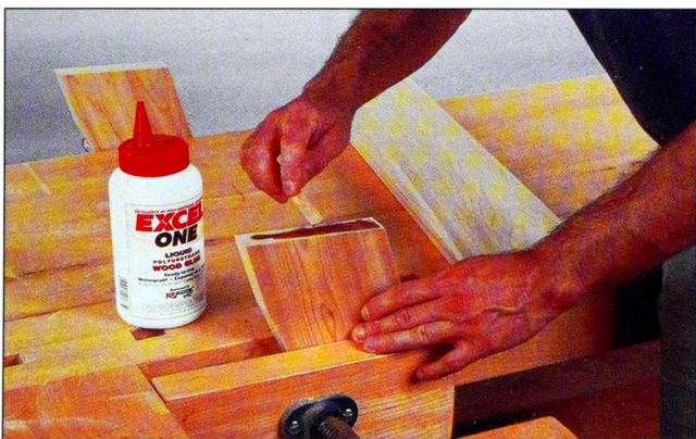
Fig. 5 In two stages, apply polyurethane glue to the end of the leg. Allow some glue to be absorbed, and then apply more.
