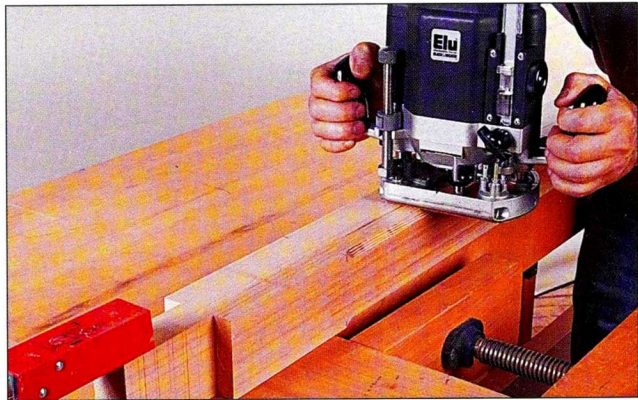
Fig. 2 Mark the stopped-chamfer end points on the cedar posts, and then rout the corners using a chamfer bit in the router.
