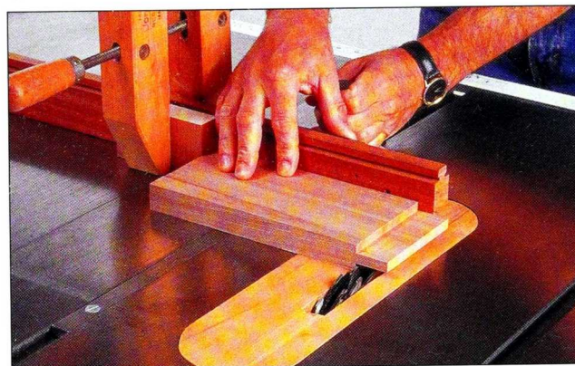
Fig. 2 Cut the leg tenons with a dado blade and table saw. A stop block clamped to the miter gauge ensures consistent tenon lengths.
