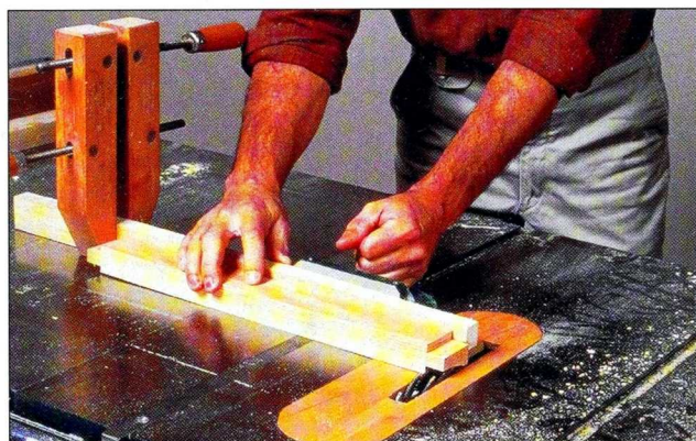
Fig. 2 Cut the rail tenons with a dado blade. A stop block clamped to a miter gauge extension ensures accurate repetitive cuts.
