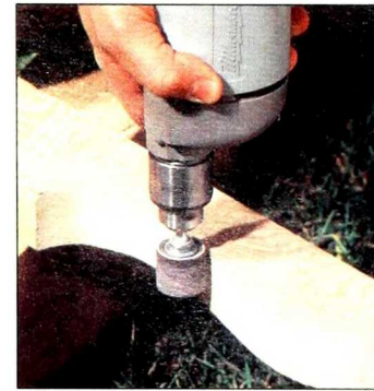
Figure 4: A sanding drum chucked in an electric drill speeds sanding.
