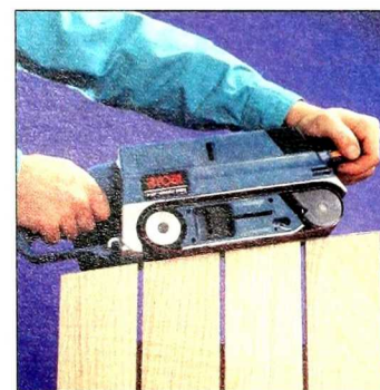
Figure 7: Sand the sawn edges of the back slats with a belt sander. Hold the sander firmly to keep the curve smooth.
