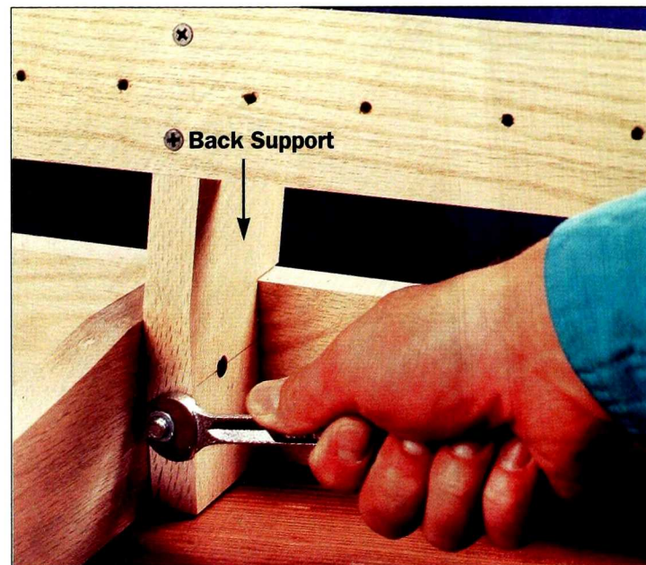
Figure 4: The back supports are screwed to the seat supports, then bolted to the rear seat rails to make a strong joint.
