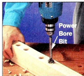
Figure 2: A power bore bit or spade bit makes the flat-bottom holes that you need to countersink the eye bolts and carriage bolts.
