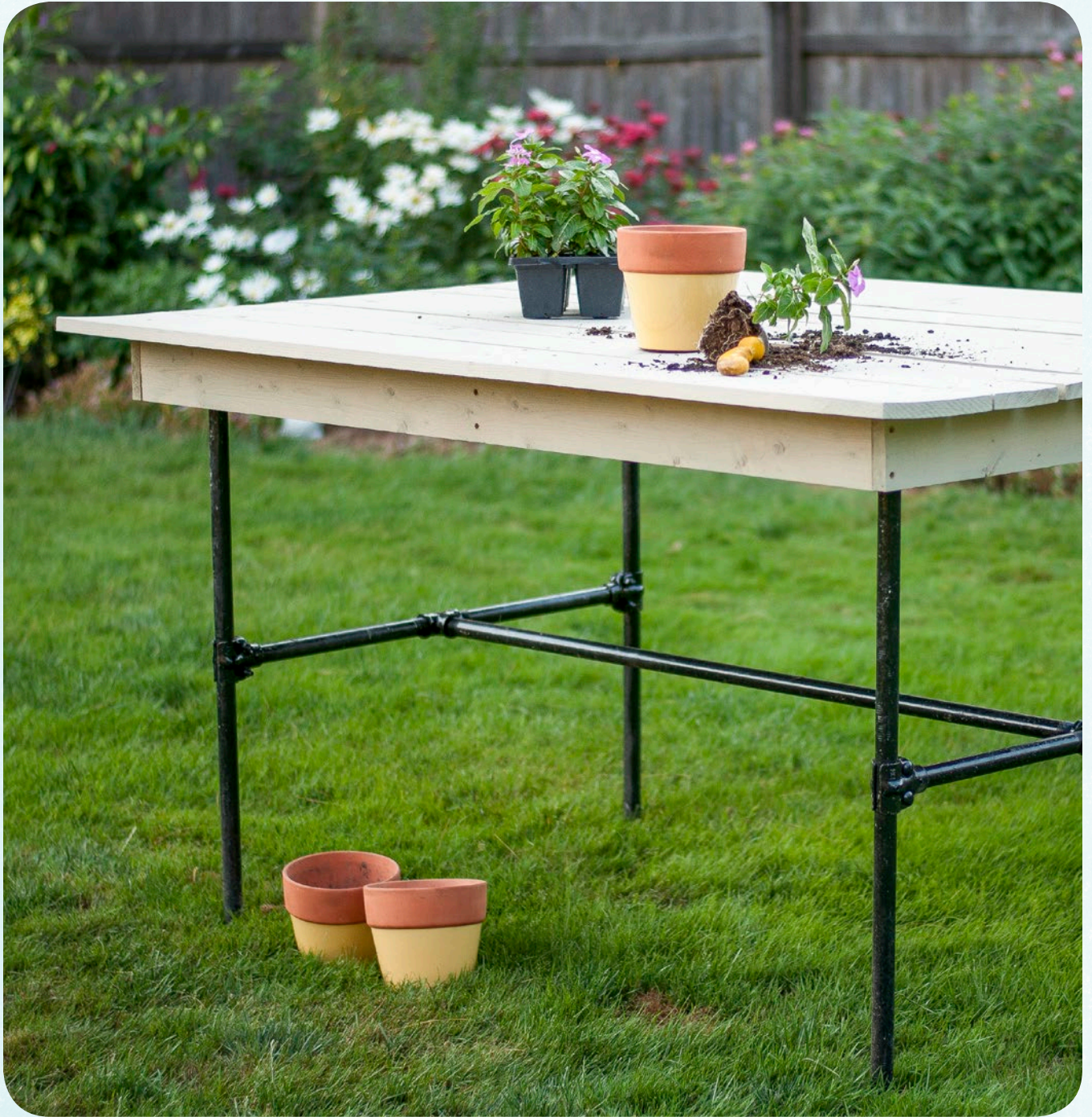
▲ The finished potting bench, ready to be put to work. The tabletop is stained with gray and the legs are painted with black enamel paint. The space between each tabletop board was created using a dowel as a spacer instead of measuring the distance between each board—this method saves time and is more accurate.
