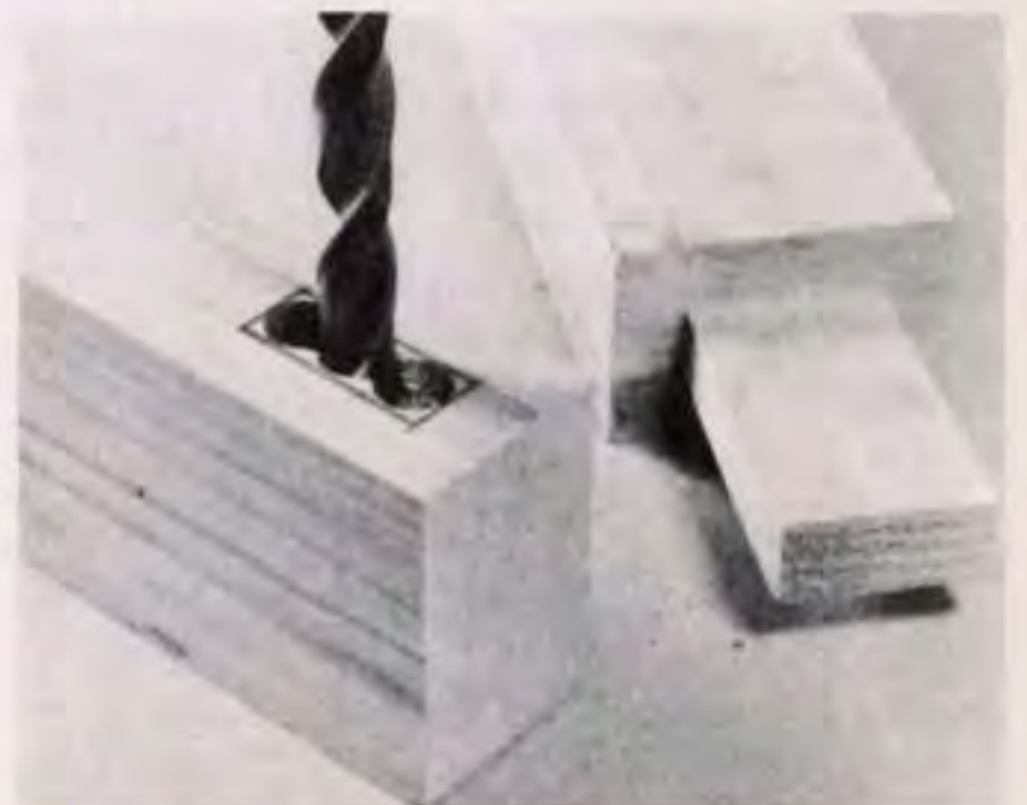
Measure and mark mortise; clear waste with brace and bit, corners with chisel
