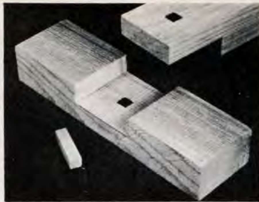
Tee half-lap is used for stretcher or any other spot where wood is joined other than at corners. Square peg adds strength
