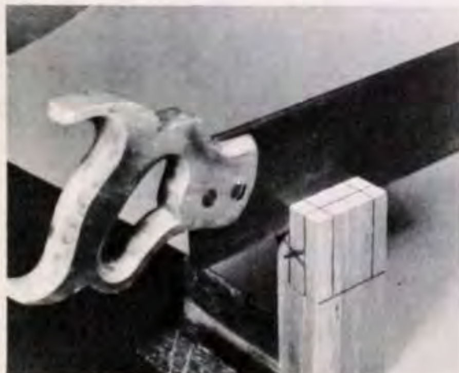
Next, cut cheeks of tenon with panel or back saw. Saw on "waste" side of lines
