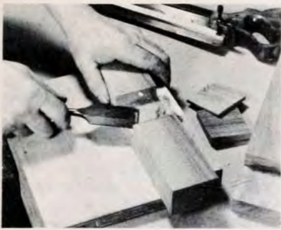
Use sharp chisel to remove waste to the depth of half-lap between saw cuts. Work from both sides to prevent splintering
