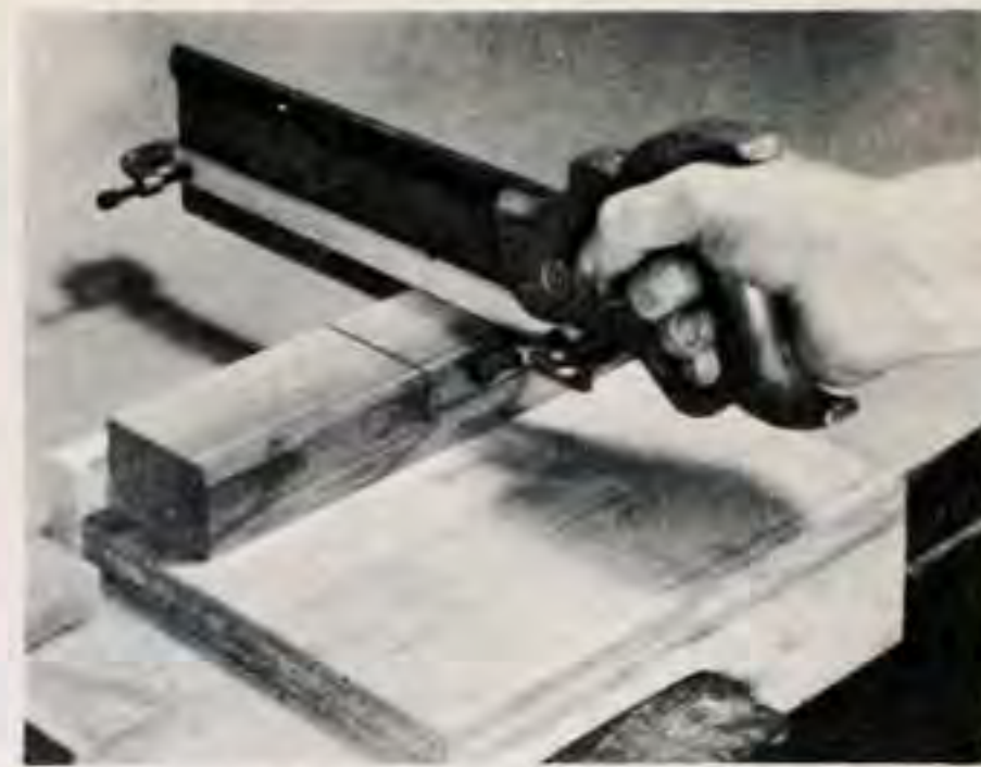
Making half-lap joint by hand. Mark carefully and saw with panel or back saw. Strips clamped to saw limit depth of cut
