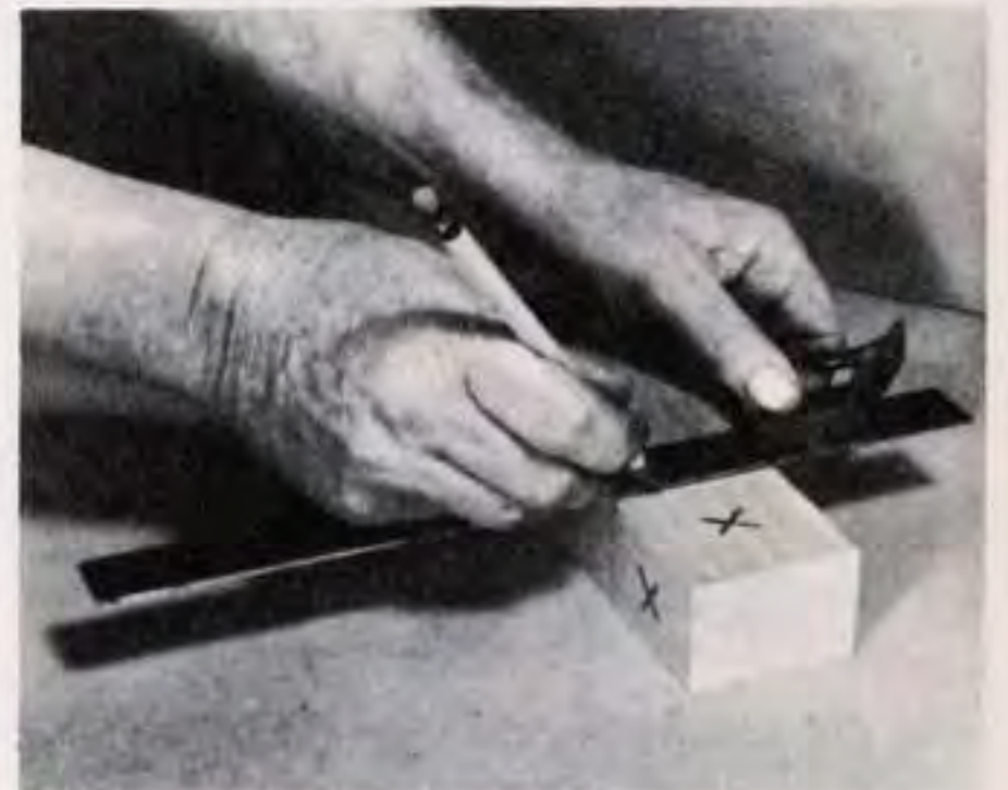
When making mortise and tenon joints by hand, first step is careful marking of square shoulders with try-square, pencil
