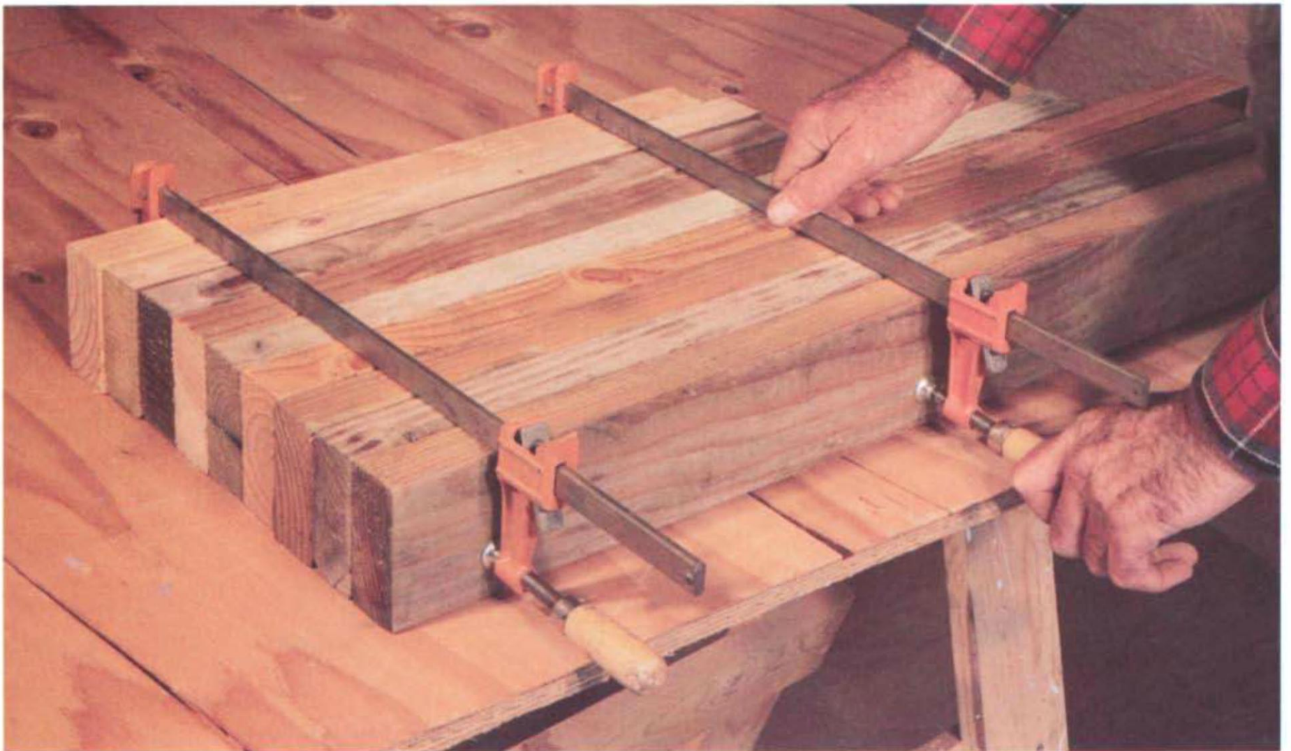
Bar clamps (bottom) and pipe clamps (top) can hold wood securely during glue-up.
