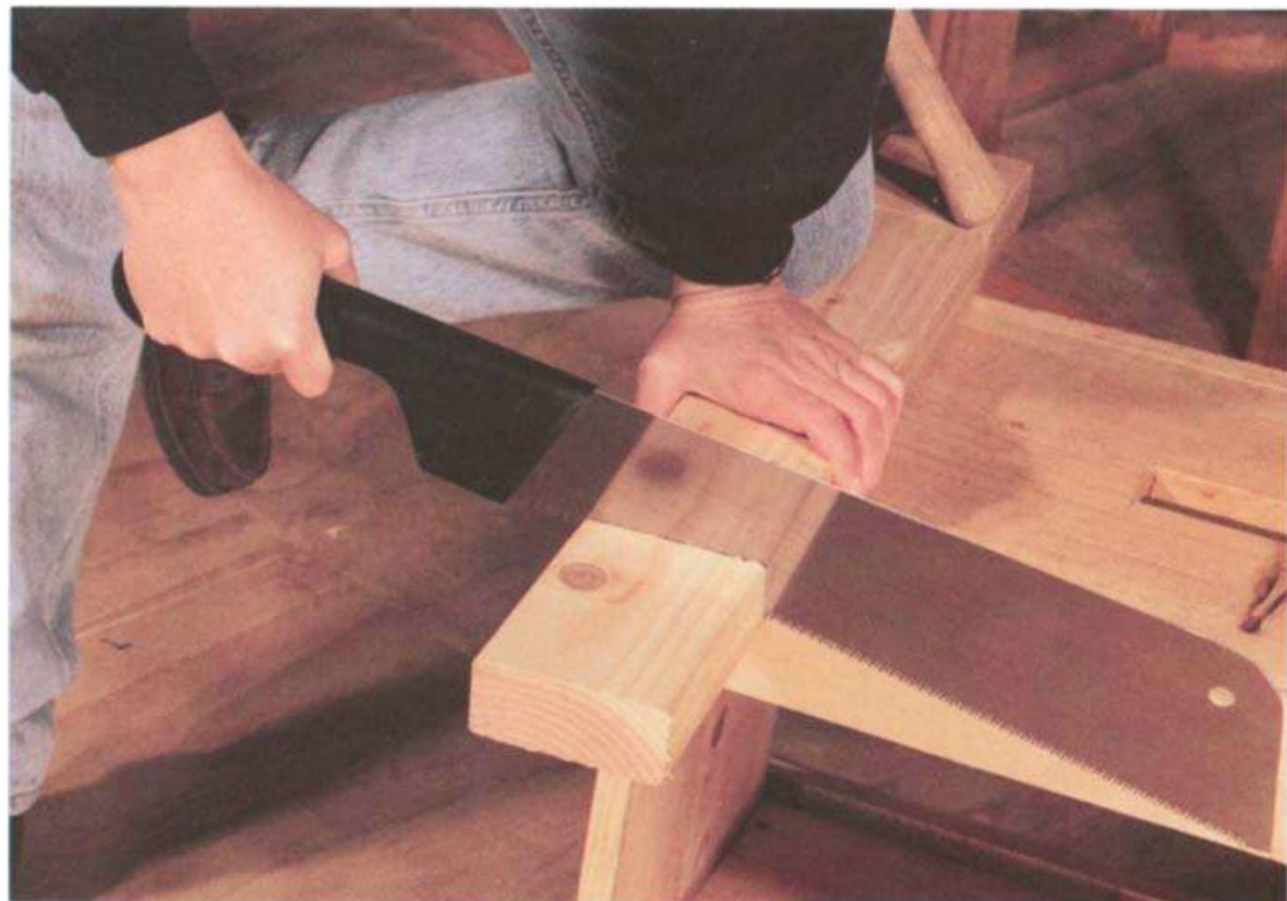
Japanese handsaws cut on the pull stroke rather than on the push stroke. For best cutting, keep the saw at a 10° angle.
