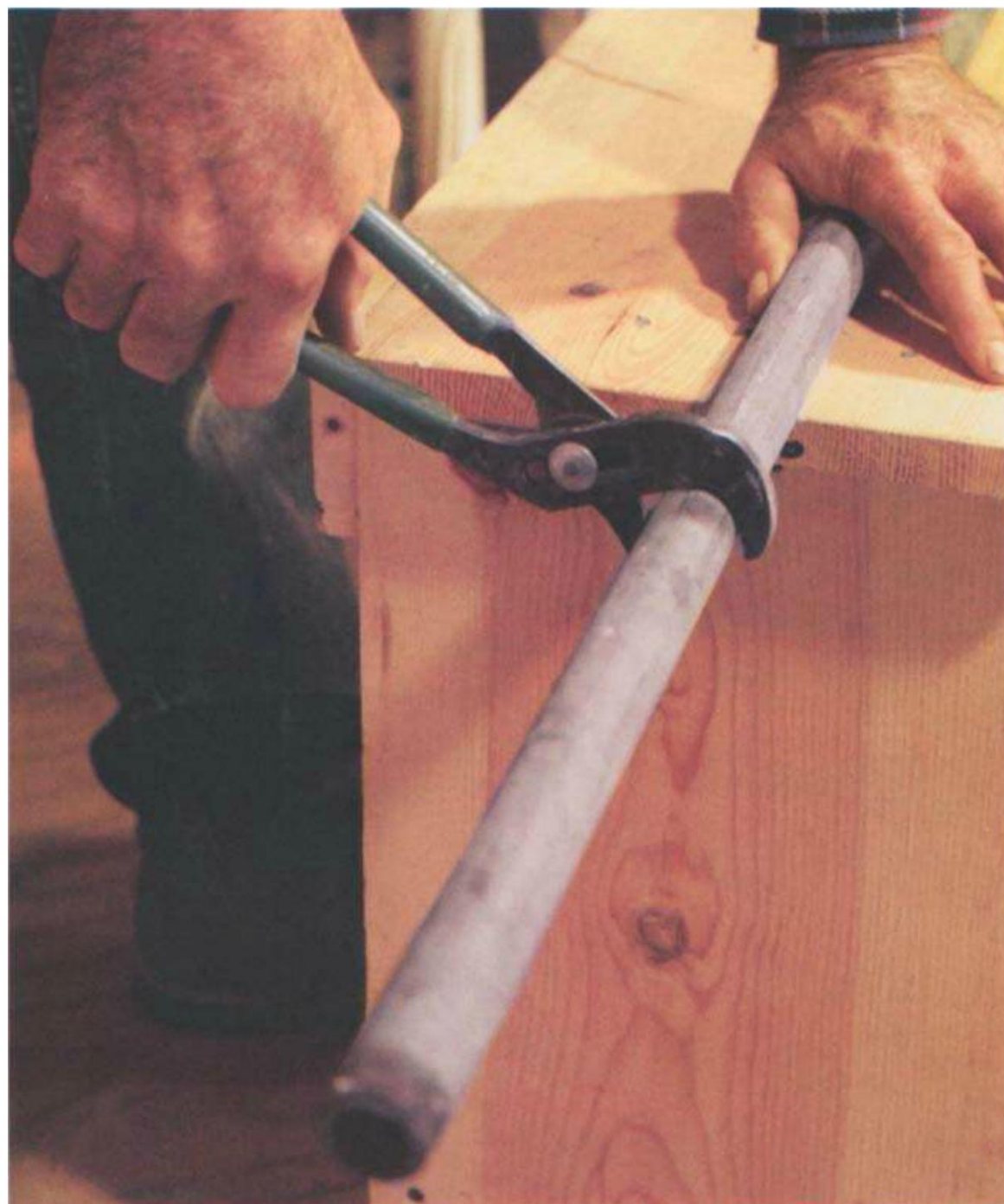
Channel-lock pliers can be adjusted like a wrench to grip pipes and other large objects.
