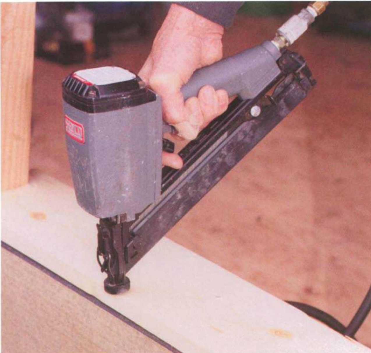
A finish nailer works well for trimwork, such as nailing in the stool for a window. (Photo by Roe A. Osborn.)
