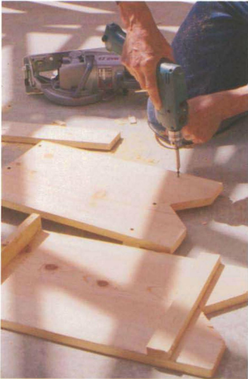
Attach the bottom cleats to the sides using 1 1/4-in. drywall screws.
