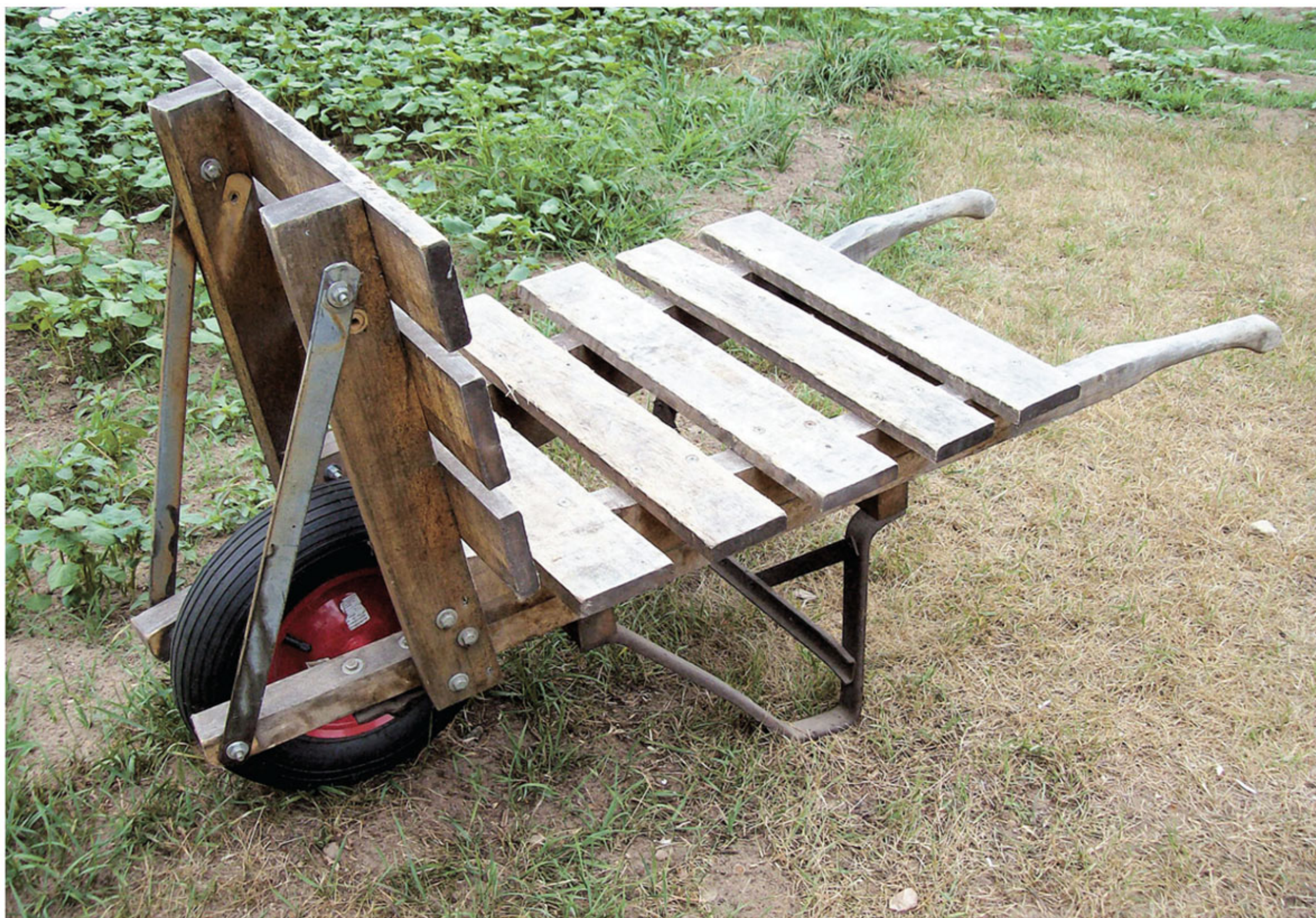
Using the wooden wheelbarrow his dad used for some 50 years, Jack McGee updated it by carving new handles and building a slatted bed, leaving the sides open for hauling long lengths of firewood for his outdoor stove.
