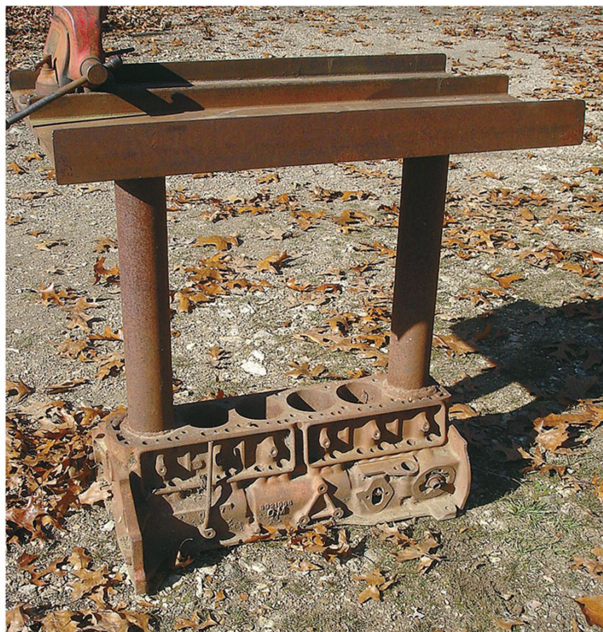
Lengths of pipe inserted in engine block support the tabletop.
