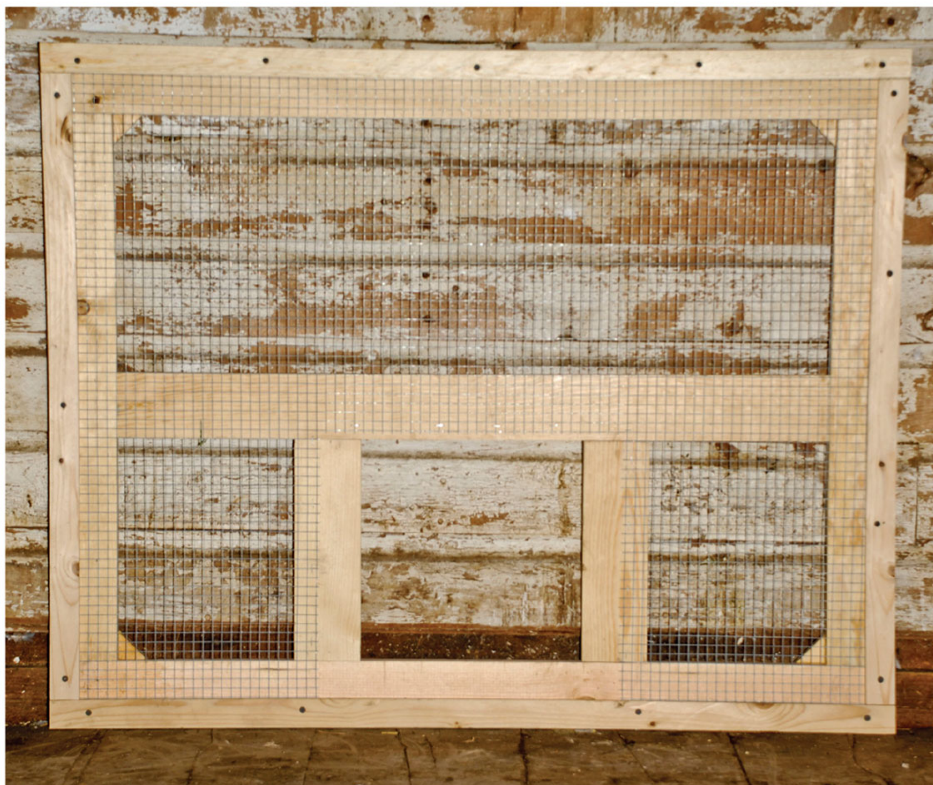
Outside of door panel (not shown in illustration on Page 60): Two (S) pieces are at the top of the door frame, and two vertical (N) pieces on the sides.
