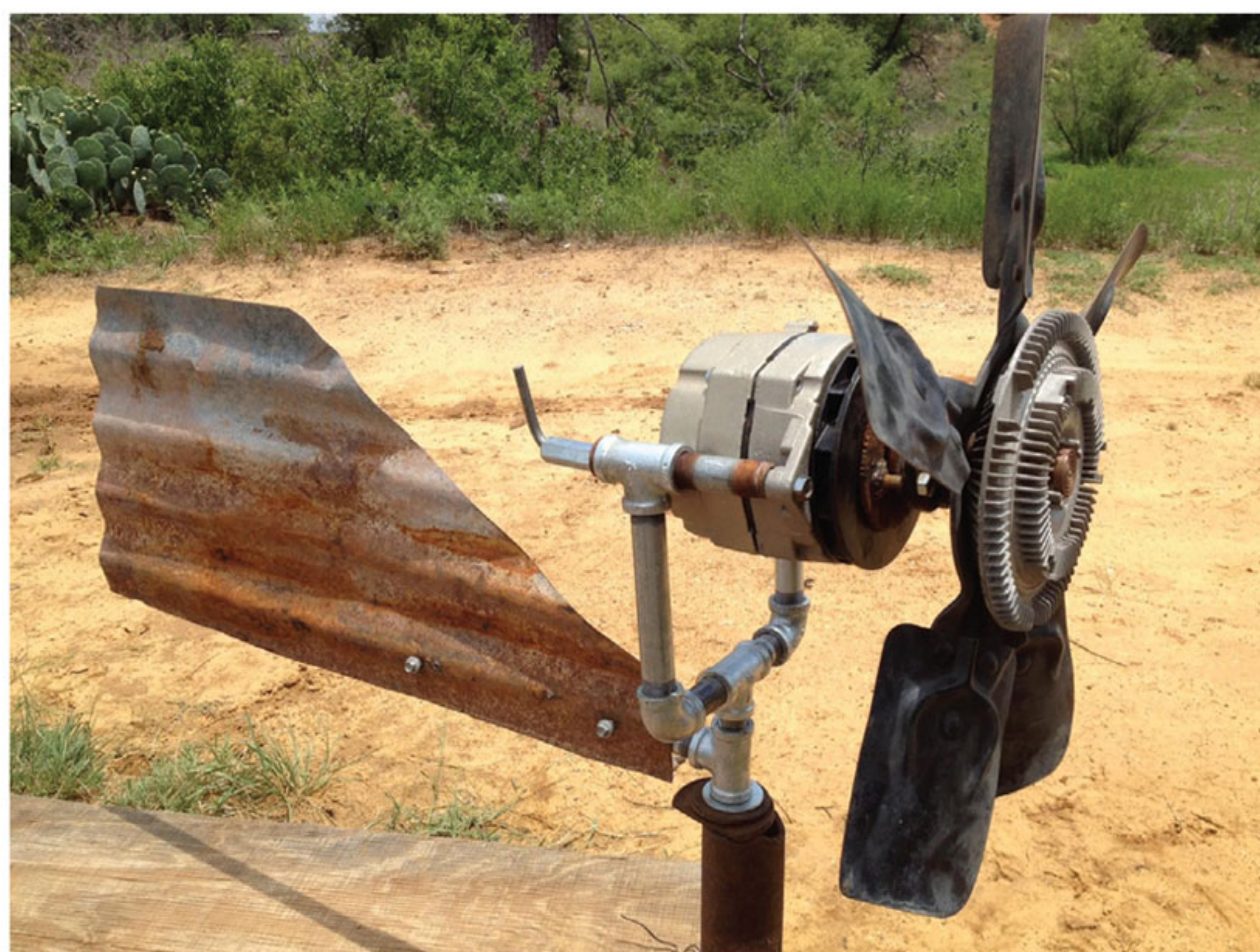
CLOCKWISE FROM TOP LEFT: Use self-tapping screws to affix the tail to the nipple; a lock washer needs to be added for each bolt in the assembly for the alternator shaft; a car/truck fan clutch assembly is needed for the generator; along with a car/truck alternator; the completed wind generator; and a view of the assembly from the back, before the tail has been added. OPPOSITE: The completed wind generator in place on the tower.
