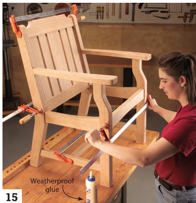
15 Glue the frame together. To ensure even clamping pressure on all the joints, center your clamps, keep them level and tighten them sequentially, one twist at a time.
