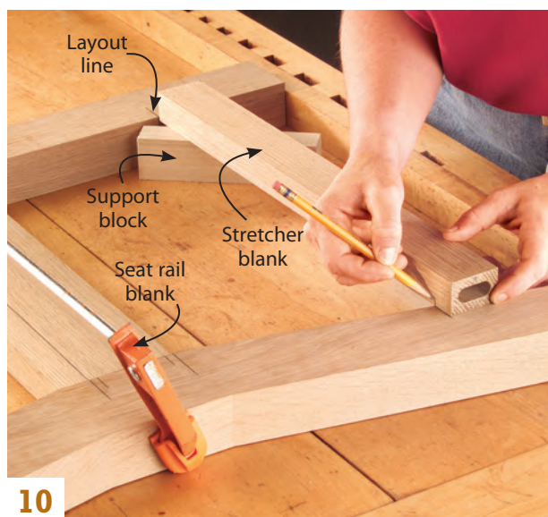
10 Cut the stretchers to fit after dry-assembling the legs and seat rail blank. Align the stretcher with the layout lines, butt its front end against the leg and mark the back end.
