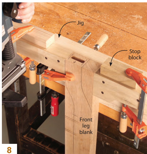
8 Rout mortises for the arms in the tops of the front leg blanks using a shop-made jig to support the router (Fig. C).
