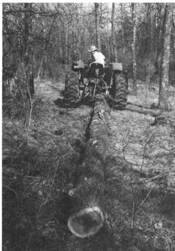
A small- to medium-size tractor can be used for skidding. Smaller logs can be skidded out with a four-wheel-drive vehicle. Below: Once your logs are cut to length, you must skid them out. Commercial loggers use heavy equipment. You may want to hire a logger to do the job. (Photo courtesy Caterpillar Tractor Co.)
