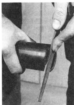
Remove burrs on the end of pipe with a file or knife, or with sandpaper. Lightly touch up the outside edge.
