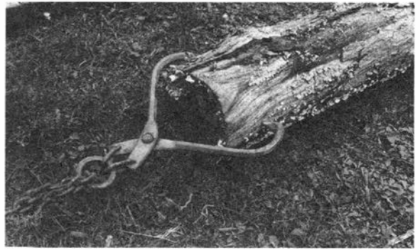
Skidding tongs grip the log so you can pull it out.
