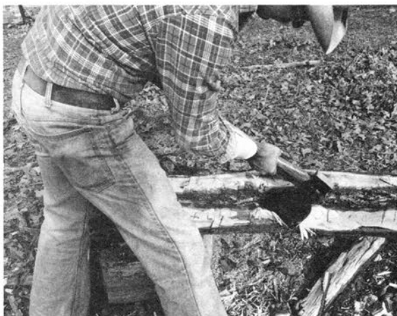
The hard work of hewing comes in removing the wood between the scored lines. Some hewers prefer to stand on the opposite side of the hewed line (photo above), behind the log to protect their legs. Others (middle photo) stand on the same side. Straddling the log (bottom) is especially dangerous. Work with safety in mind and use slow, controlled chopping strokes.
