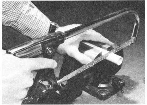
Plastic pipe is easy to cut. Almost any fine-toothed saw can be used. (Photo courtesy Genova, Inc.)
