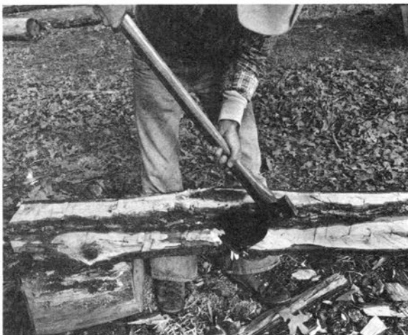
The hard work of hewing comes in removing the wood between the scored lines. Some hewers prefer to stand on the opposite side of the hewed line (photo above), behind the log to protect their legs. Others (middle photo) stand on the same side. Straddling the log (bottom) is especially dangerous. Work with safety in mind and use slow, controlled chopping strokes.
