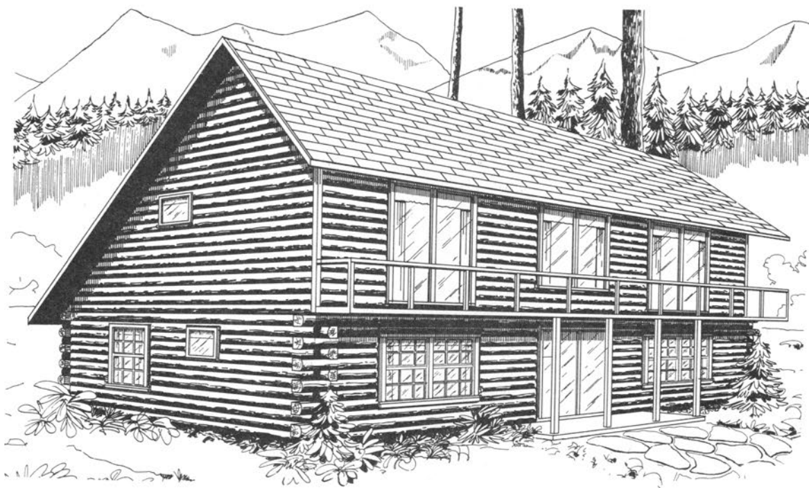
This is a typical passive solar style. Large windows face south, and a steep roof with few windows face north. (Photo courtesy Lincoln Logs Ltd.)
