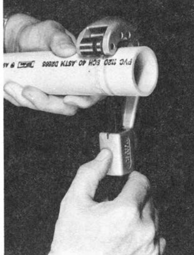
Rigid plastic pipes may be cut with a large plastic-cutting wheel in an ordinary pipe cutter. (Photo courtesy Genova, Inc.)
