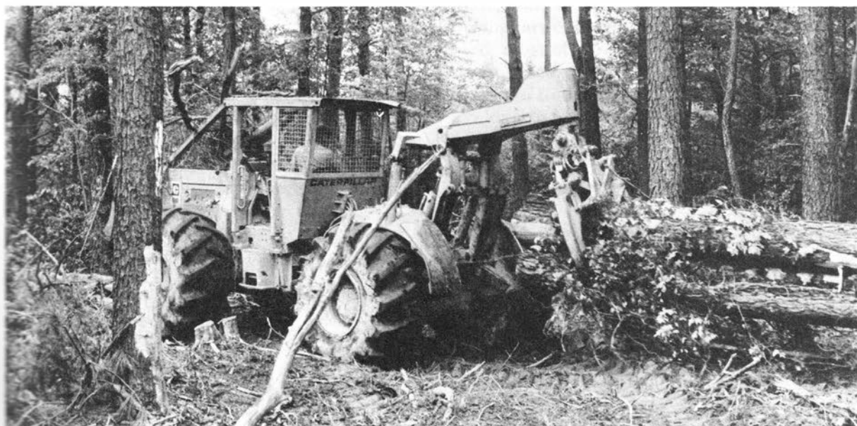
A small- to medium-size tractor can be used for skidding. Smaller logs can be skidded out with a four-wheel-drive vehicle. Below: Once your logs are cut to length, you must skid them out. Commercial loggers use heavy equipment. You may want to hire a logger to do the job. (Photo courtesy Caterpillar Tractor Co.)
