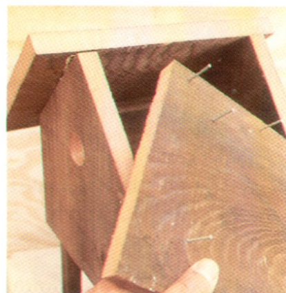
ABOVE: Redwood (shown here) and cedar offer natural resistance to decay, which makes them ideal for outdoor birdhouses.
