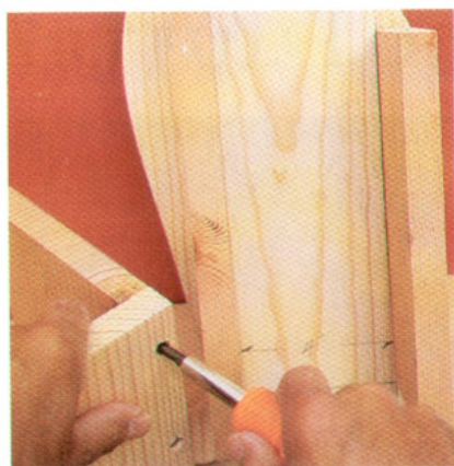
Fasten the roof pieces together with outdoor screws set in counterbored holes.
