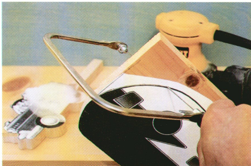
Cut out the car and trailer along the pattern lines, bypassing areas the blade won't easily reach.
