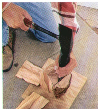
Split the log so that each side piece is at least 4 inches thick at its widest point.
