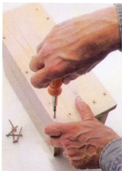
Attach one side to the backing board, then the floor, the other side, and the roof.
