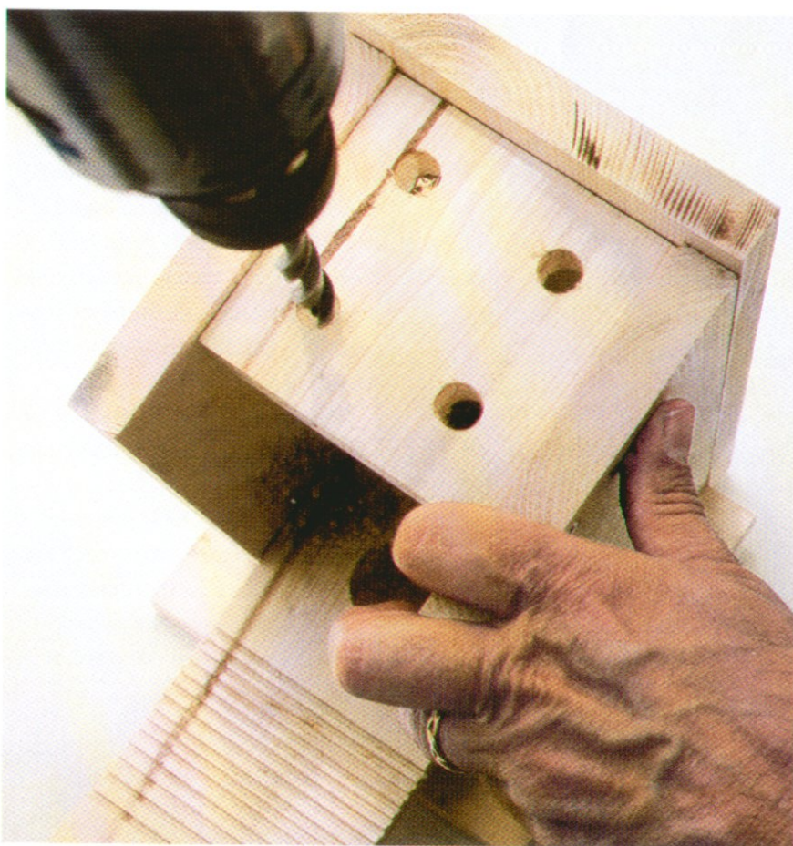
Drill four 3/8-inch holes in the floor to provide for adequate drainage.
