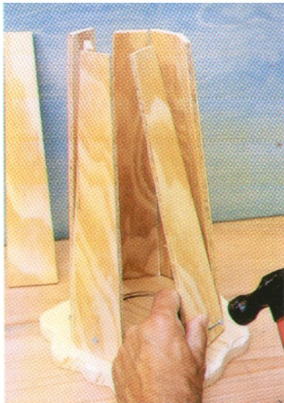
Glue and toenail the staves to the octagon facets after octagon C is affixed to the base.
