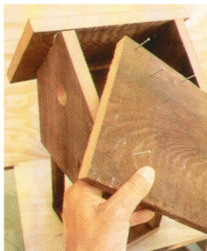
Nail the short side of the roof in place, then the overlapping side.
