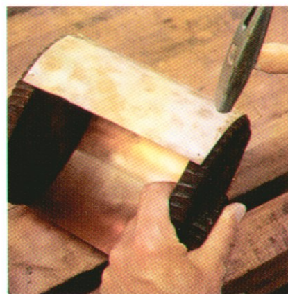
Attach the copper flashing to the end pieces with escutcheon pins along the edge.
