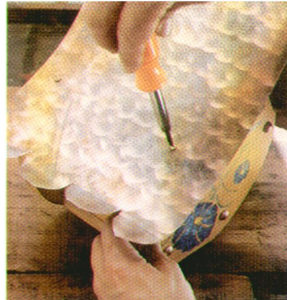
Fasten the roof with brass screws at the deepest part of the roof's curves.
