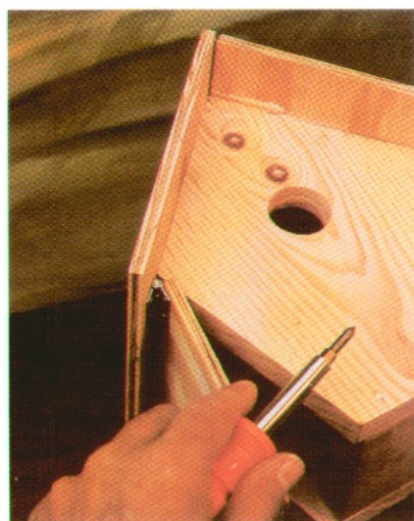
Screw the hinges to the roof with their barrels about 2 inches from the gable ends.
