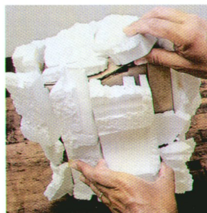
Break up foam blocks and butt them together to create a highly uneven surface.
