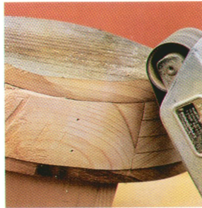
Though not essential, a belt or random-orbit sander comes in handy for projects requiring considerable sanding.
