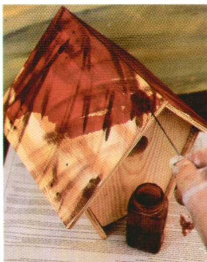
Using the applicator that comes with it, apply a flood coat of red leather dye to the roof.
