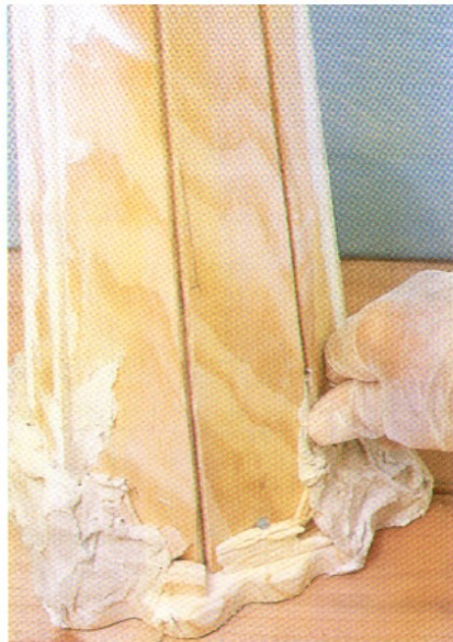
Plaster between the staves and the base, the base surface, and the scrap wood.
