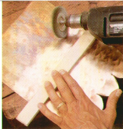
Texture the copper roof with a wire-wheel brush. Hold it firmly with a wood scrap.
