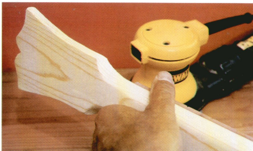
Using a rasp and sander, shape the peghead so it is thinner than the neck and slopes back from it.
