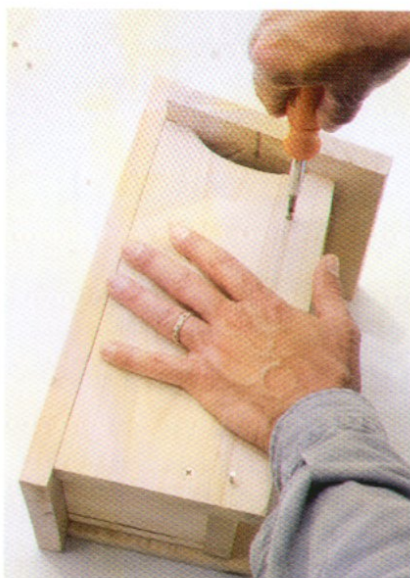
Attach the door with two screws driven about 1 3/4 inches down from the top.
