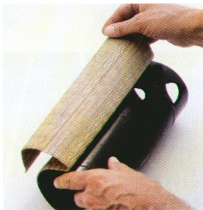
After applying three or four lines of hot-melt glue around the pipe, attach the placemat.
