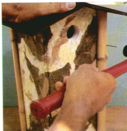
Drill two 1/8-inch pilot holes in each corner post, then fasten with 3d finishing nails.
