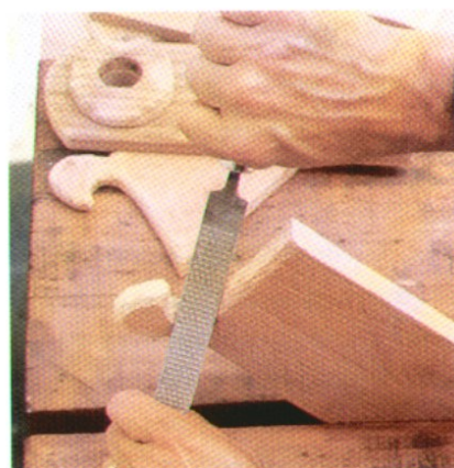
Chamfer and distress the exposed edges of the wooden parts, using a coarse wood rasp.
