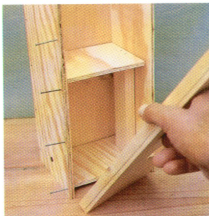
Fasten the sides to the gable ends, check the fit of the floors, then assemble.
