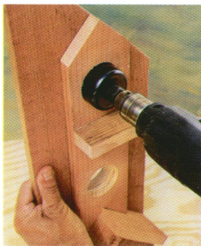
Mark the entry holes, drill pilot holes, then cut them with a 2-inch or 2½-inch hole saw.
