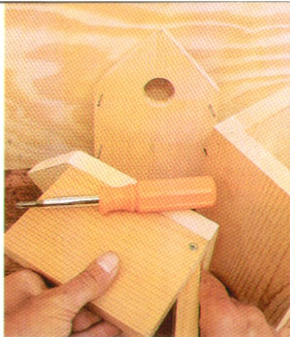
Attach the floor with outdoor screws; it is beveled at the back to permit it to pivot freely.
