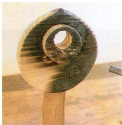
Using a propane torch, char the surfaces of the wood ends and the security panel.
