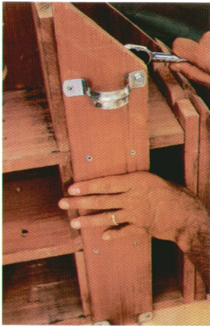
To add the upper pipe strap, screw the left side through B2 into divider J, then bolt it.
