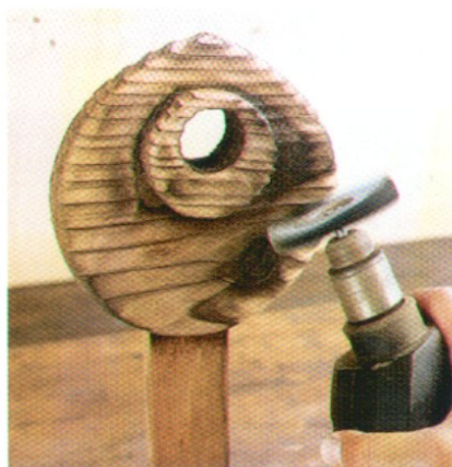
Brush away the charred wood using a wire wheel mounted in an electric drill.
