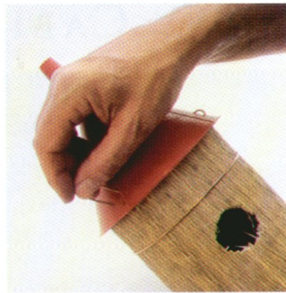
Attach the funnel with 3-inch lengths of copper wire bent into the shape of a staple.
