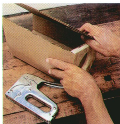
Using hot glue and staples, attach the corrugated cardboard panels to the plywood base.
