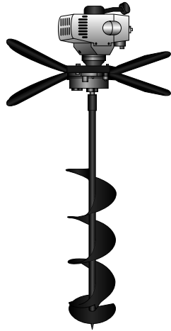
Figure 3-7: A power auger brings horsepower to a hole- digging party.
