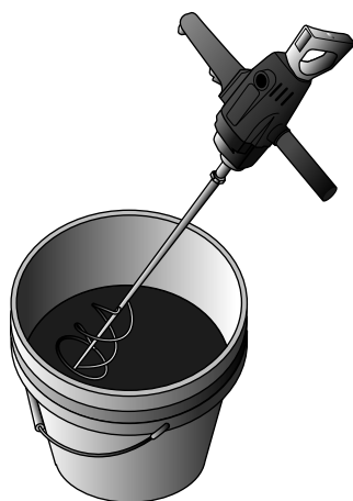
Figure 6-5: A drill mixer can whip up a batch of concrete if you don’t mind the mess.
