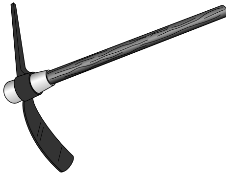
Figure 3-1: A mattock makes short work of stubborn tree roots and shallow rock.
