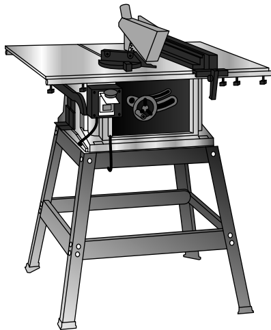
Figure 3-5: A table saw is tops for cutting sheet goods like plywood.
