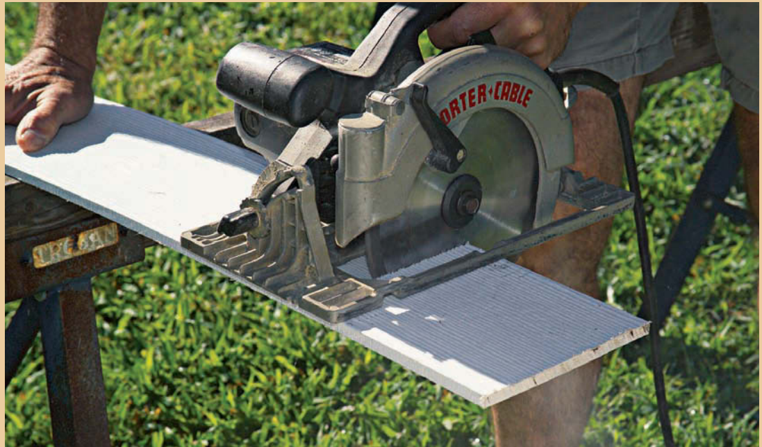
Portable circular saw equipped with a carbide-tipped blade.
