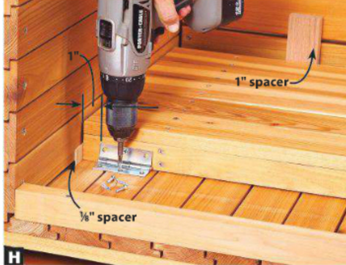
Position the folding shelf in the base with 1/8" spacers at the sides and 1" spacers at the bottom. Screw the hinges in place.
