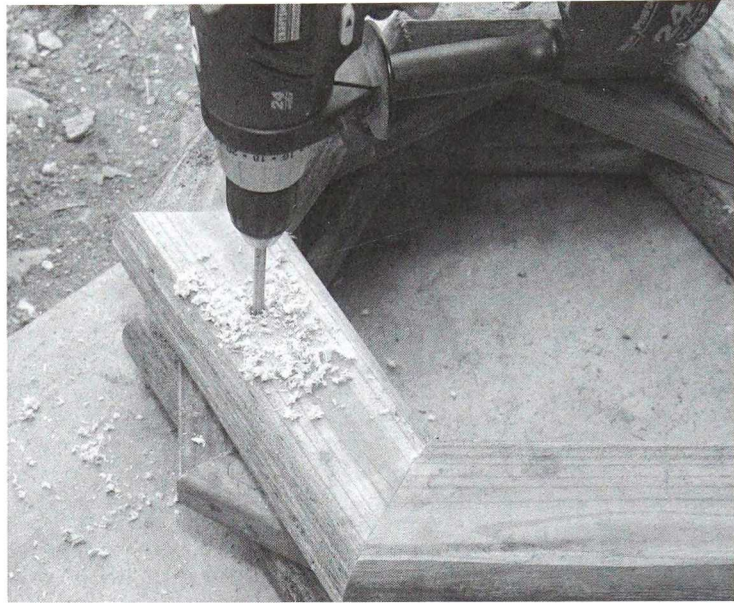
The planter is assembled upside-down. Holes are counterbored for screws.
