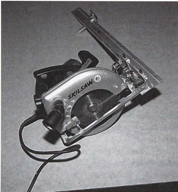
Large panels are easily ripped using the Craftsman Accu-Rip accessory guide.
