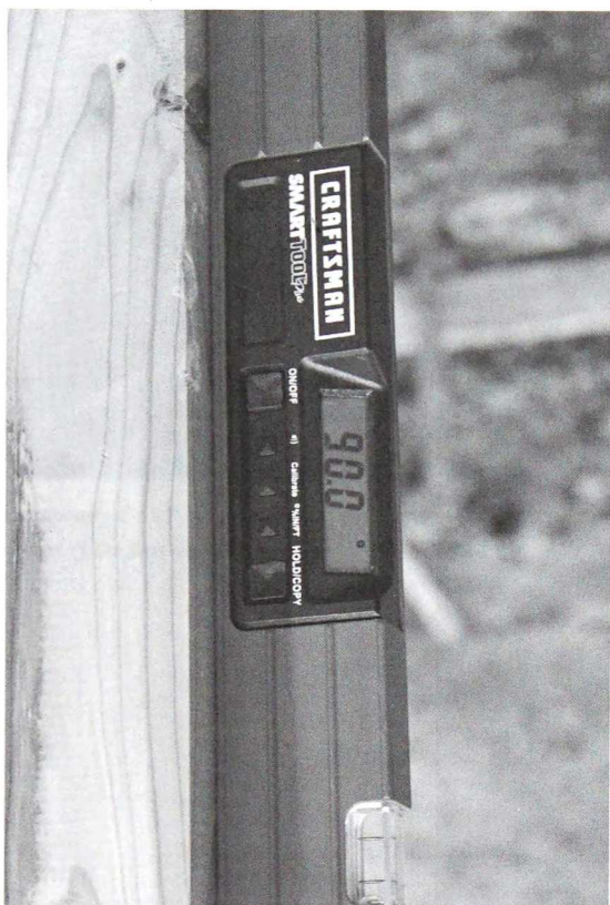
The Craftsman Smart Tool Plus Level makes an easy job of leveling and plumbing all portions of the project.
