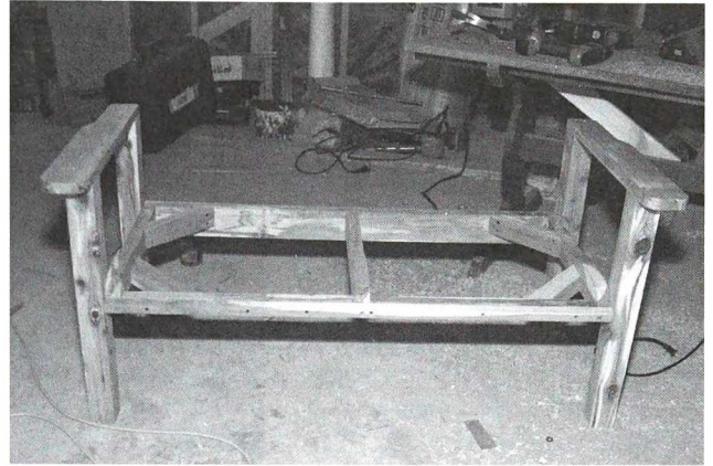
Shown is the basic bench seat frame
