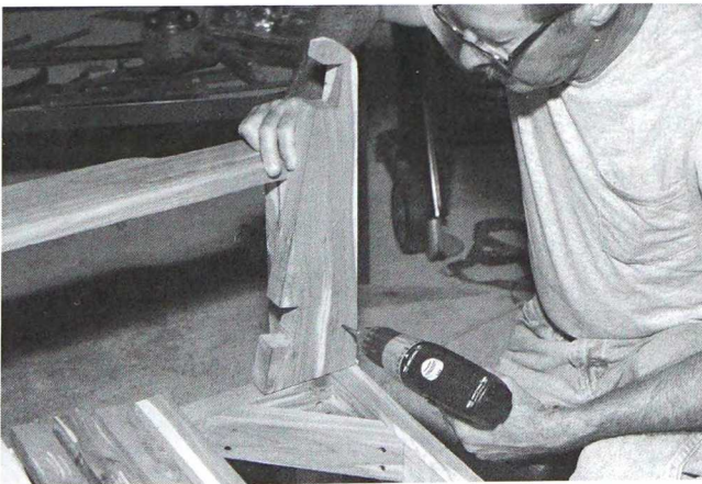
The backrests are fastened to the upper ends of the legs.
