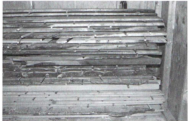
In most cases, sawn woods should first be air-dried before using for construction.
