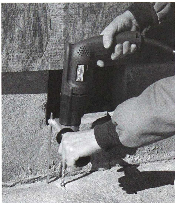
An impact driver is best for heavier driving chores. It can be used with screws or to drive lag screws. Corded hammer drills can be used for boring in concrete and other extremely heavy-duty chores.
