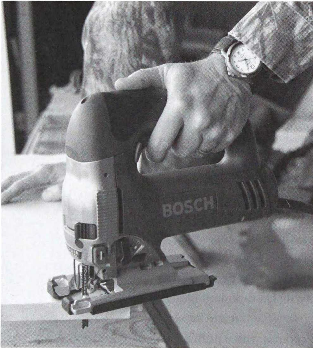
Saber or jigsaws are useful for many chores, such as cutting holes in siding for windows and doors.
