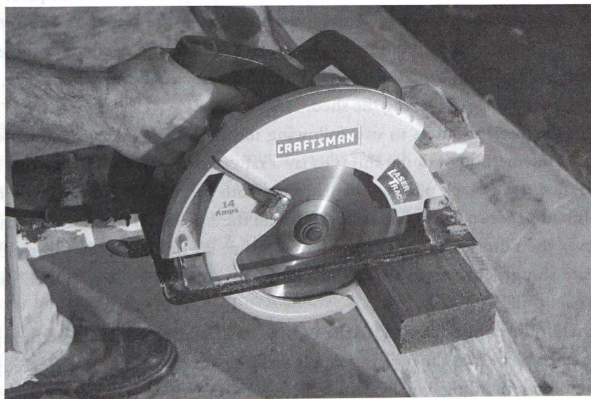
A portable circular saw makes it quick and easy to cut 2 \times 4s to length.
