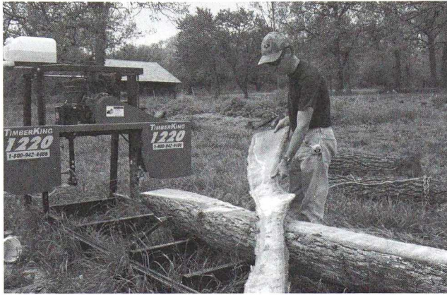
Slabs, or the waste from sawmills, are used to create the bench.
