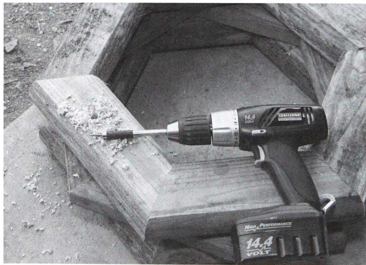
Brass screws are used to assemble the hexagon rings.
