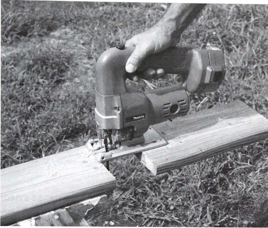
A cordless jigsaw is extremely handy for notching deck boards around posts and other chores.
