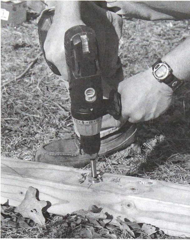
Forstner bits can also be used for this chore. Make sure the workpiece is backed up to prevent splintering out the back.
