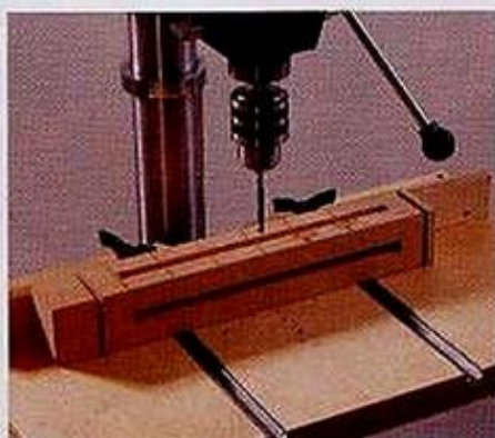
Drill \frac{3}{4} " holes where marked on each leg for the shelf pins. A fence on your drill press ensures alignment.
