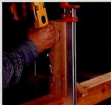
A handscrew and a bar clamp help hold the rail (B) in position when attaching it to the post (A).
