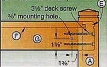
BENCH DETAIL (END SECTION VIEW)
