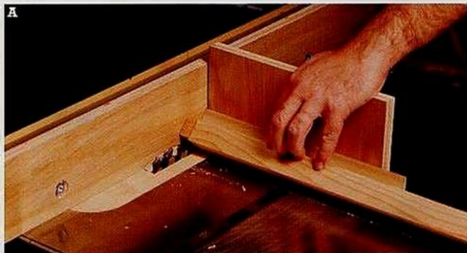
Using a 45°-angled support secured to your miter-gauge extension, trim the corners off the square-cut tenons to fit into the 1" holes in the rails.
