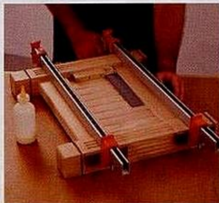
When assembling the planter endframes, be sure to square them as you tighten the clamps. The slats float in the frame.
