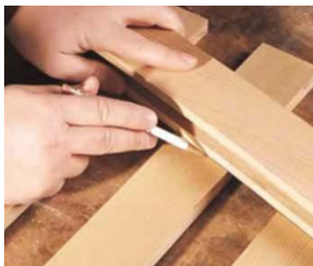
Holding the arched top rail steady was the most difficult part of routing the top groove for the slats. Remember to make the cut in two passes on each side. In this photo you can see that the rail hasn't been cut for length yet, allowing extra support for the router at the beginning and end of the cut (at left).
