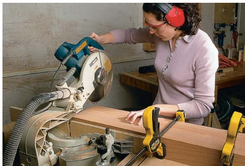
We used a miter saw to cut our pieces to length. Here you can see that we clamped all the top boards together and “gang cut” them to length simultaneously.
