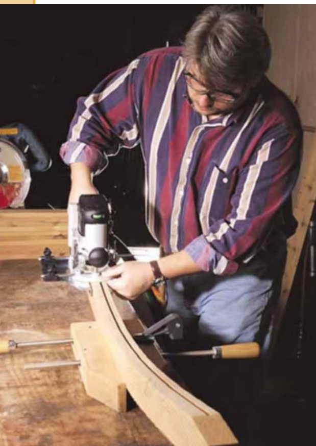
Holding the arched top rail steady was the most difficult part of routing the top groove for the slats. Remember to make the cut in two passes on each side. In this photo you can see that the rail hasn't been cut for length yet, allowing extra support for the router at the beginning and end of the cut (at left).
