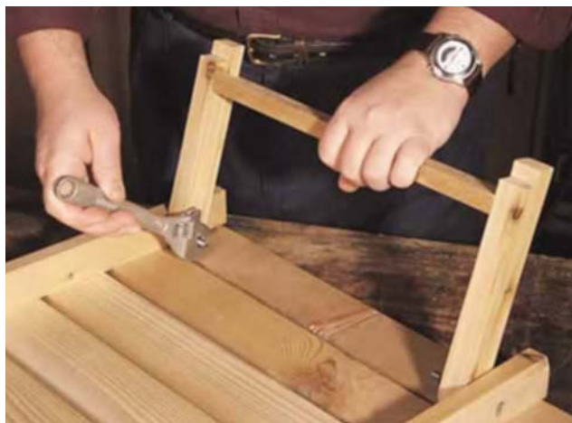
Last, but not least, bolt the table legs in place to the table battens. Note the notches on the ends of the legs which drop into the previously cut notches to stabilize the table.
