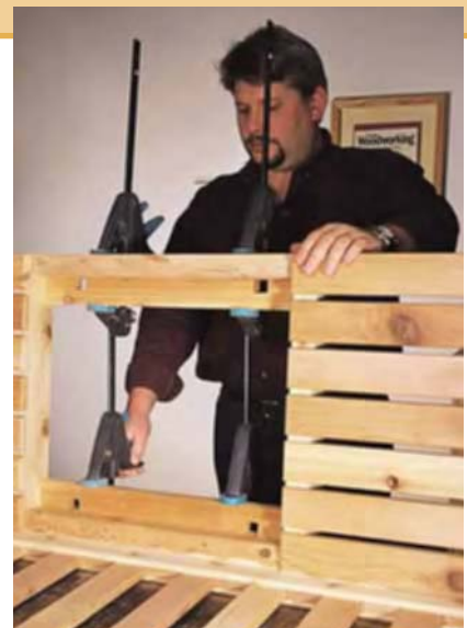
With the notches cut in the support cleats, the two pieces can be glued in place in the seat frame.
