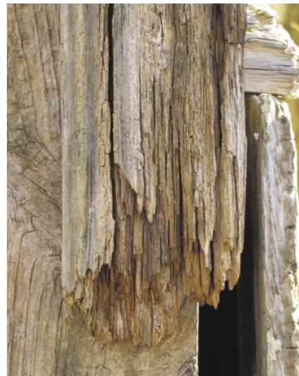
Rot is very destructive to wood, as is obvious in this photo. Pressure-treated wood and the heartwood of redwood, cedar and a number of exotic woods including teak, mahogany and ipe resist rot. A wood preservative that is not pressure-injected is fairly ineffective at preventing rot on non-rot-resistant woods.
