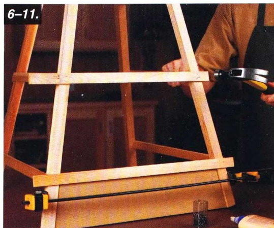
6-11. Clamp the spacer between the assemblies' legs at one end. Attach the rail blanks, aligning them with the adjoining rails.
