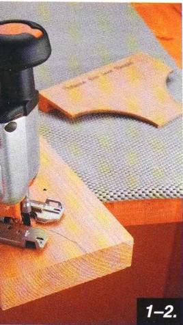
Left: A portable jigsaw comes in handy for scrolling details. Right: Circular saws can produce the cuts needed on dimensional lumber.
