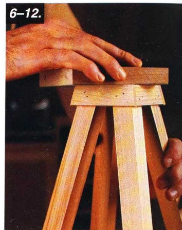
6-12. Using a sanding block with 80-grit sandpaper, flatten the top edges of the rails (C) to receive the top assembly.
