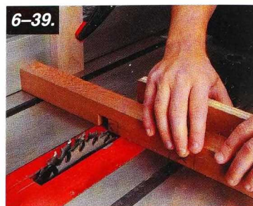
6-39. For the second pass, butt the workpiece against the fence. This doubles the dado width without changing the setup.
