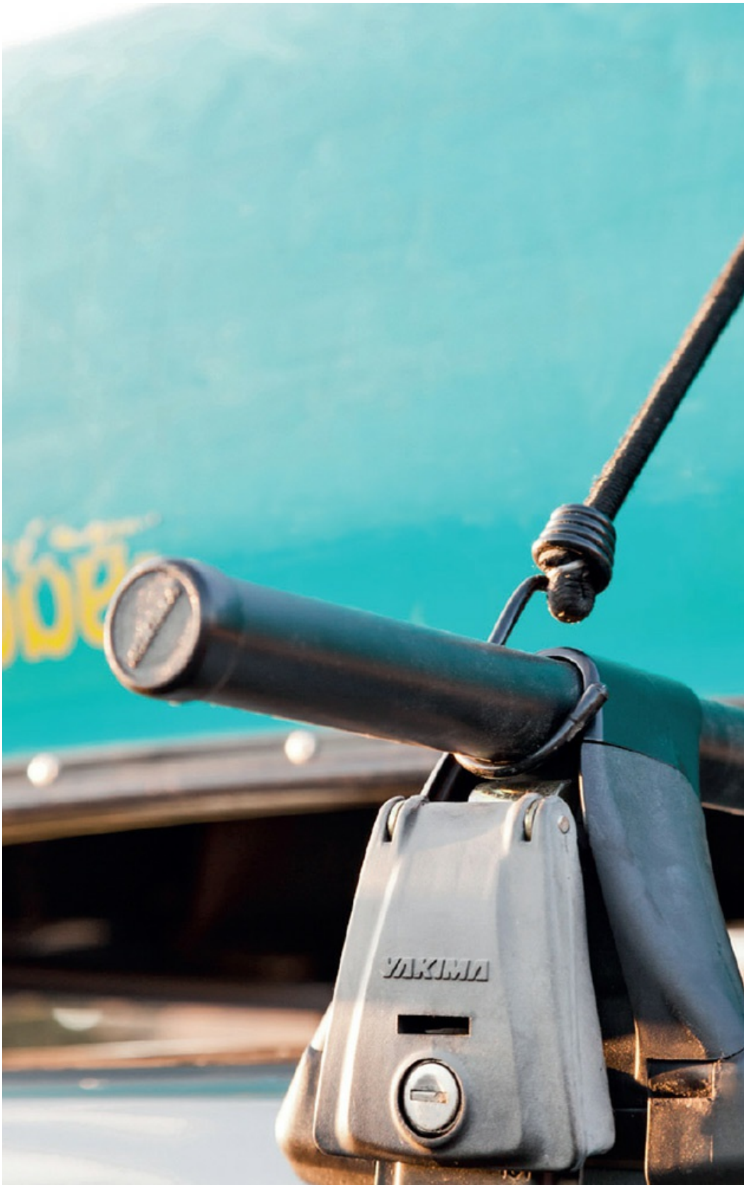
Never use bungee cords to secure loads to a car's roof rack
