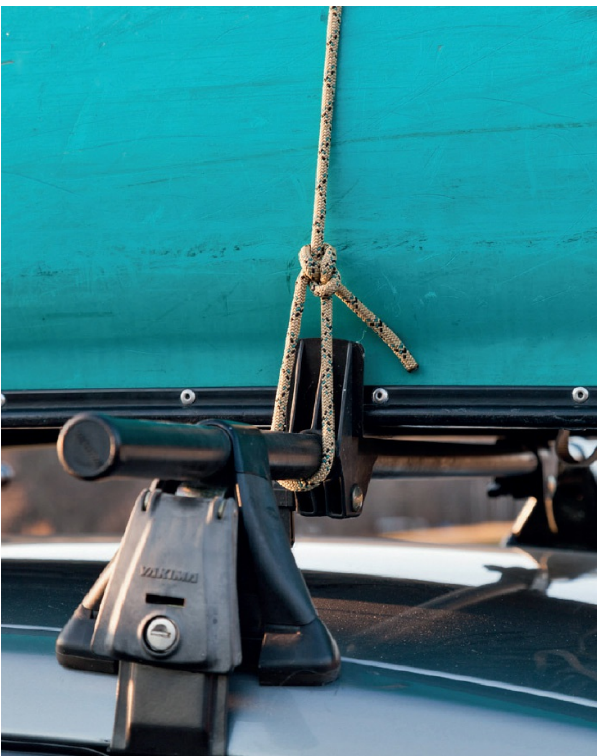
A Bowline (shown) is a good knot to begin the tie-down process. A Slip Knot Trucker's Hitch secures the canoe to the roof rack crossbar on the other side of the car. Similar knot combinations should be used on both crossbars, and from the bow and stern of the canoe to the front and rear bumpers or tow hooks on the vehicle.
