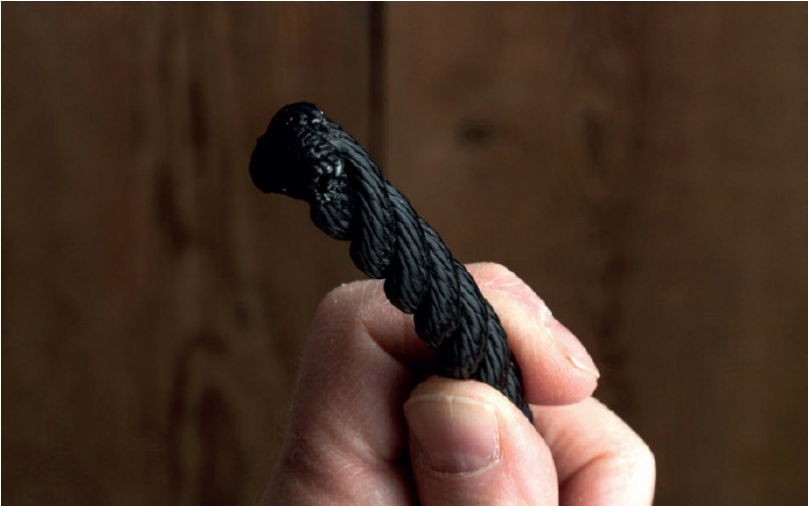
Melting a rope's end is not pretty, but it's an effective way to prevent fraying
