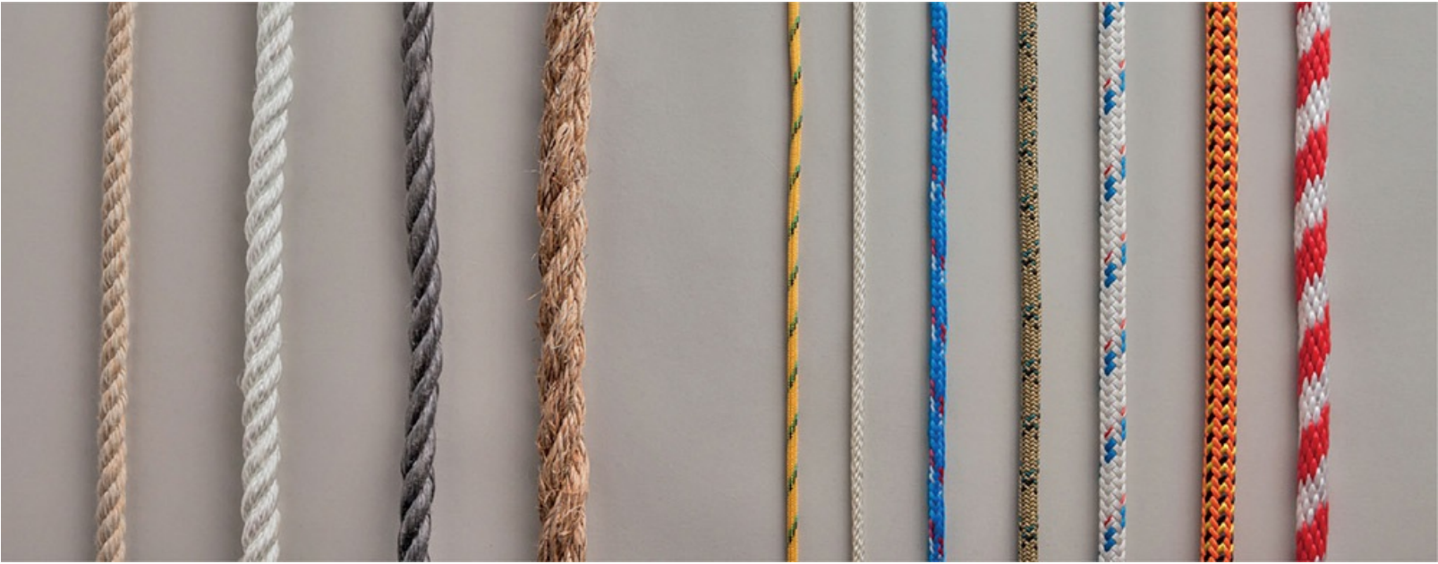
A selection of twisted (left) and braided (right) ropes
