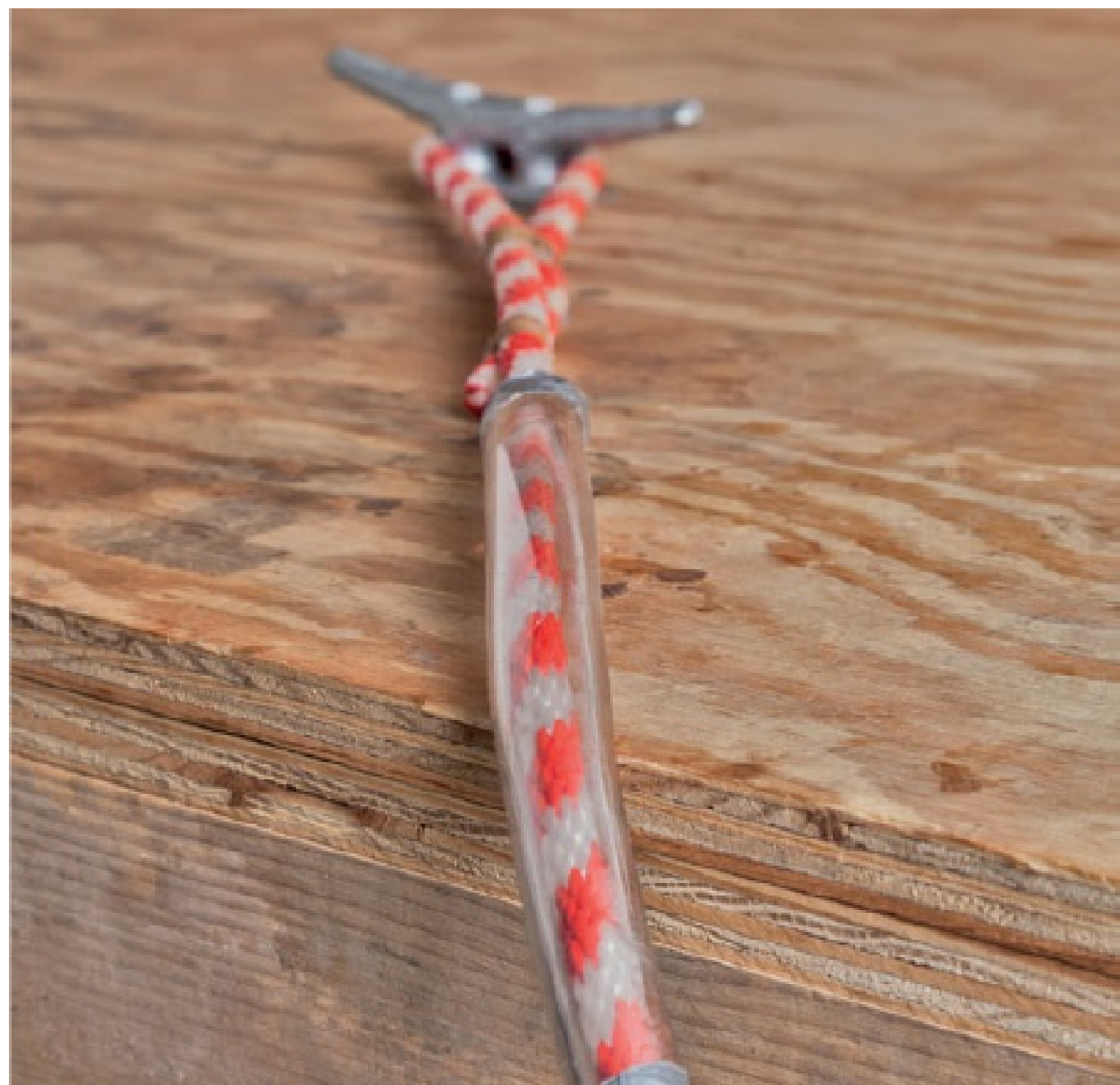
Plastic hose may be applied to a section of rope that will be frequently subject to abrasion
