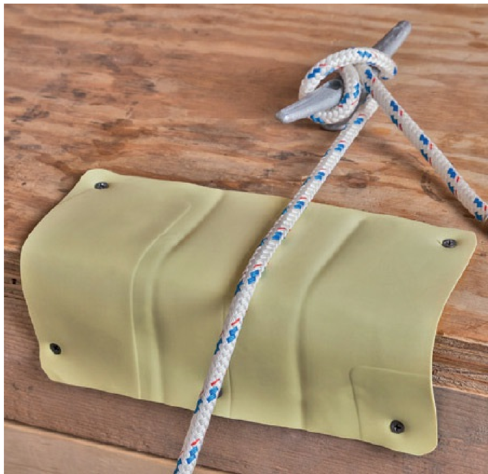
Alternately, a hard edge can be protected with a sheet of plastic, metal, or leather to prevent chafe
