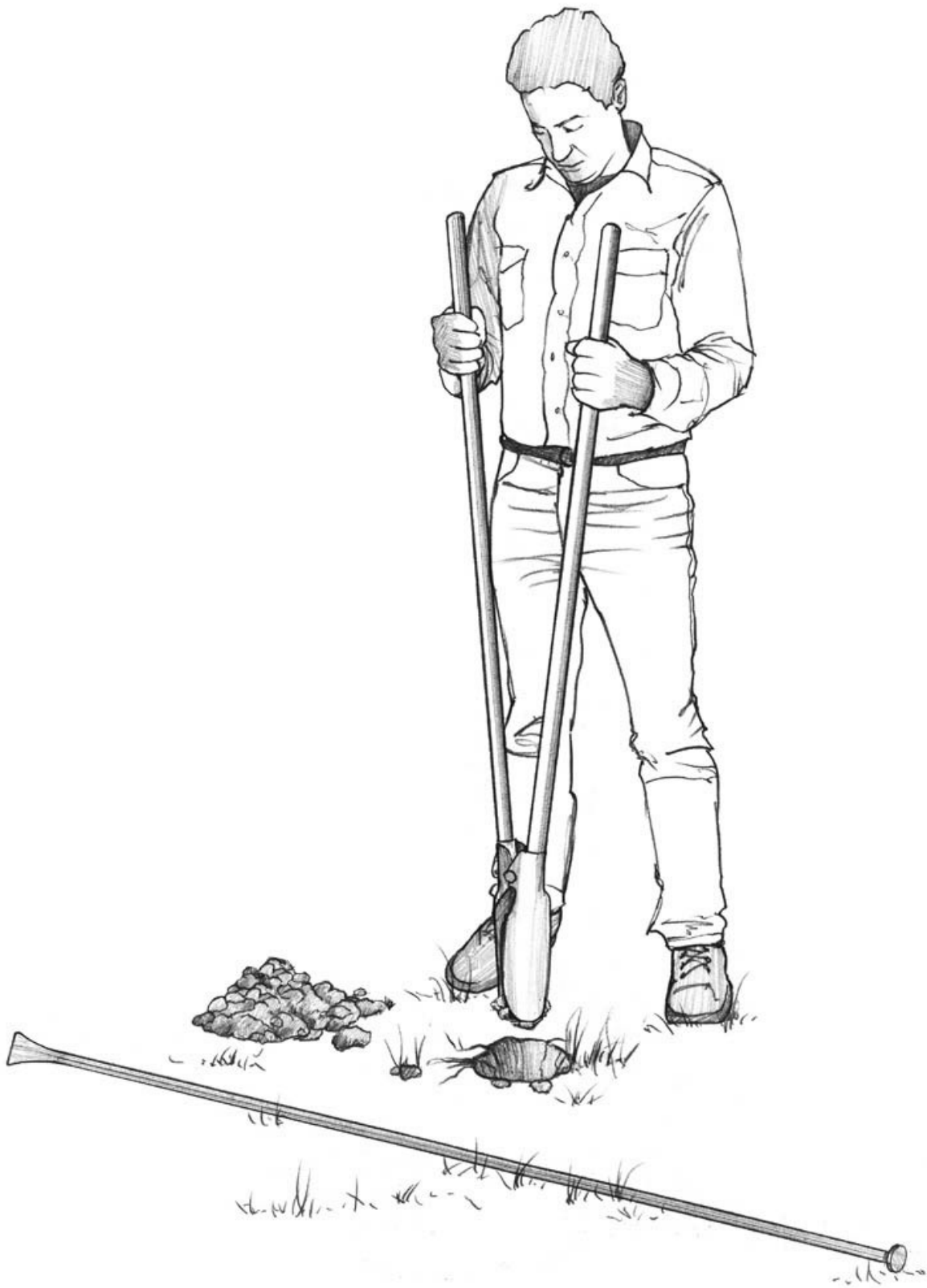
ABOVE: using a clamshell digger
