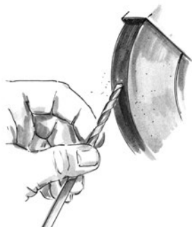
Sharpening a drill bit tip with a bench grinder
