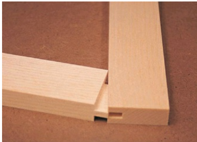
A typical mortise-and-tenon joint.
