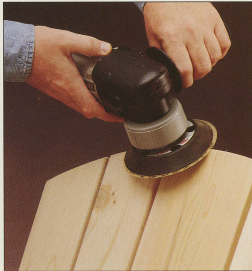
After evening out any slight irregularities in the ends of an Adirondack chair with a belt sander, you can use a random-orbit sander for final smoothing.
