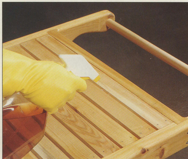
Tung oil is applied to the surface of a serving trolley. Using a squirt bottle as shown above is a quick and easy way to spread this finish. After being allowed to penetrate the wood for about 15 minutes, the excess oil is wiped from the surface with a rag.
