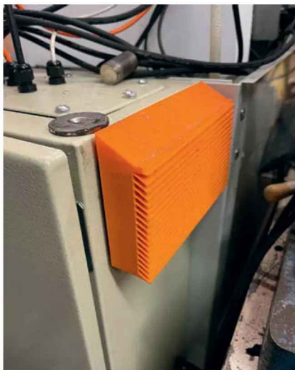
Photo 10: 3D printed fan housing and baffle.
