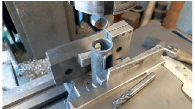
Photo 33: Chamfering end of trunk guide.
