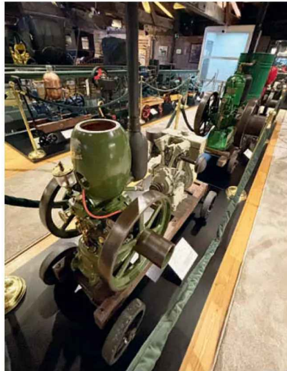
Photo 10: Petters Limited, Yeovil, England (circa 1930); stationary engine (petrol or oil-fuelled), 1.5HP, 750 rpm. Application: water pump, generator or light industrial drive. This 1.5HP engine is renowned for its durability and reliability. It has been commonly used from the early to middle of the 20th century.
