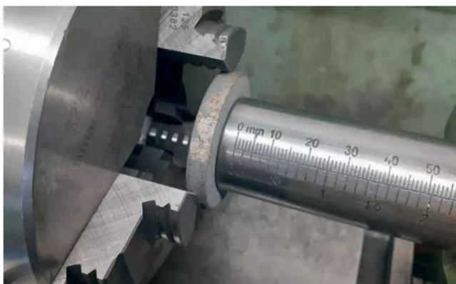
Photo 34: Positioning end cover with aid of tailstock.
