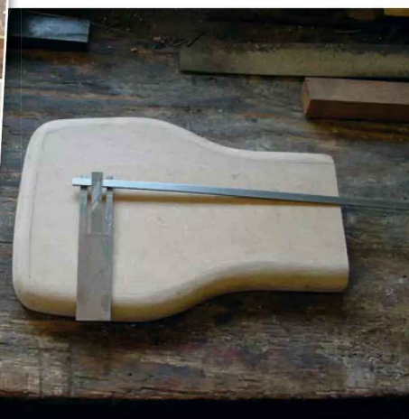
Photo 262: The little jig I made for putting the double bends in the crinolines.
