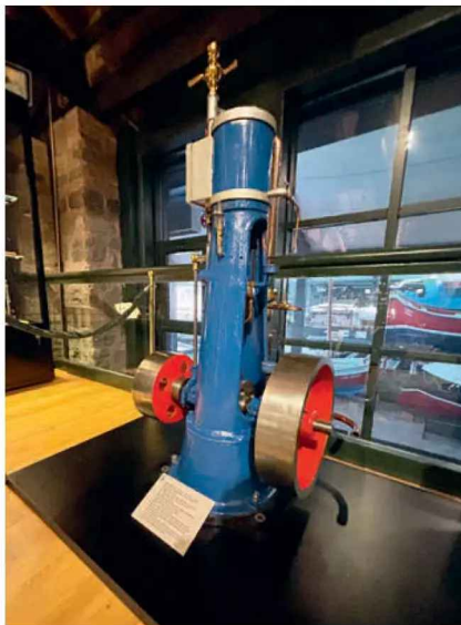
Photo 8: Robey & Co., Lincoln, England (circa 1920). Output: 3-4HP, 200 rpm, weight: 600 kg. Robey's 'Globe Works' was said to be the first factory in the UK lit by electricity and an electrical plant supplied by Robey lit Lincoln Cathedral to celebrate both the Golden and Diamond Jubilees of Queen Victoria.
