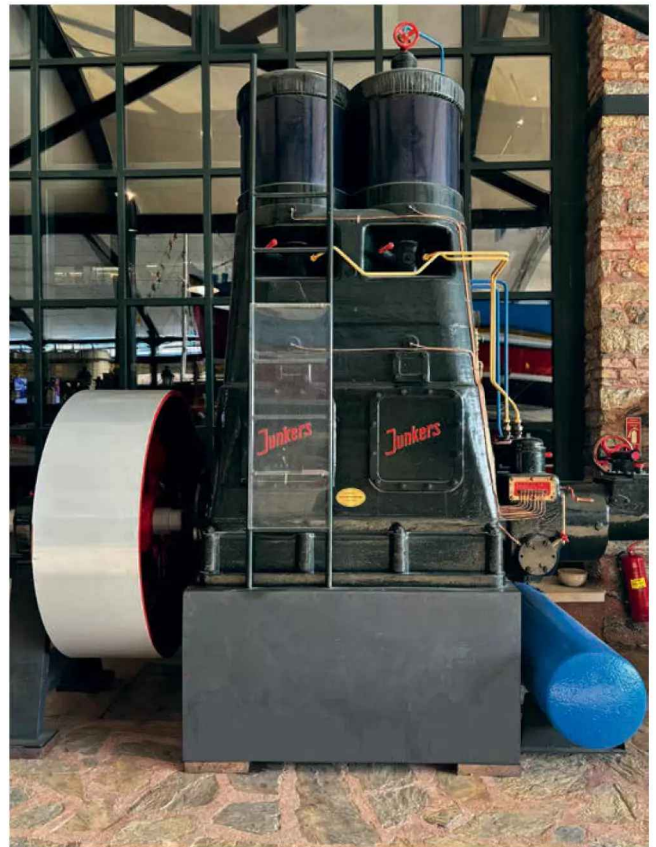
Photo 16: 2 HK 2002-Stroke-Cycle, 2-Cylinder, Opposed- Piston Diesel Engine manufactured by Junkers Motorenbau GMBH, Dessau, Germany (1928). 185HP, 4300 cc, 300 rpm.
