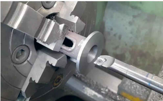
Photo 32: Flange faced and trunk guide bored.
