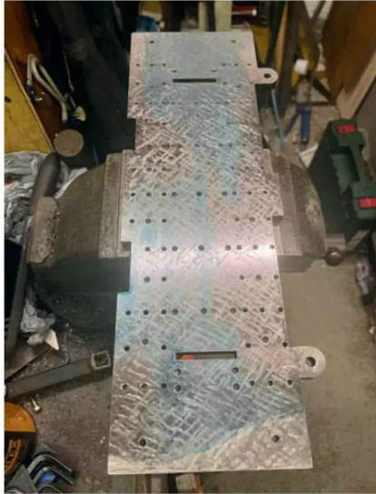
Photo 13: Gantry plate with blue showing the warp.
