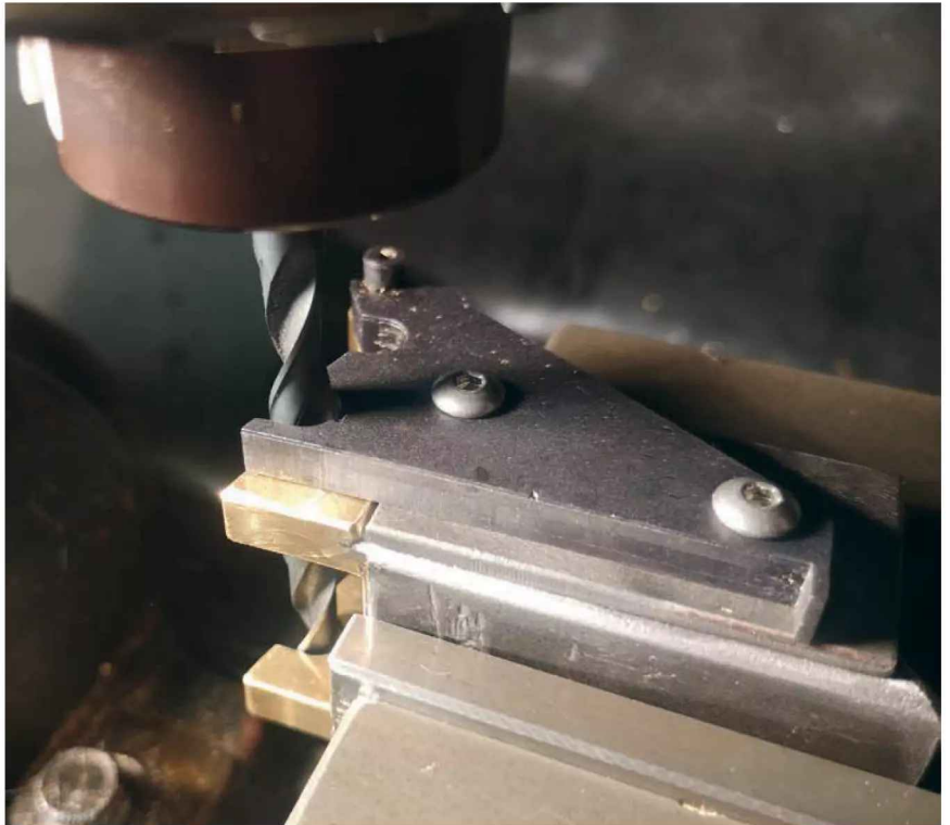
Photo 5: Drilling the 8 mm slots.
