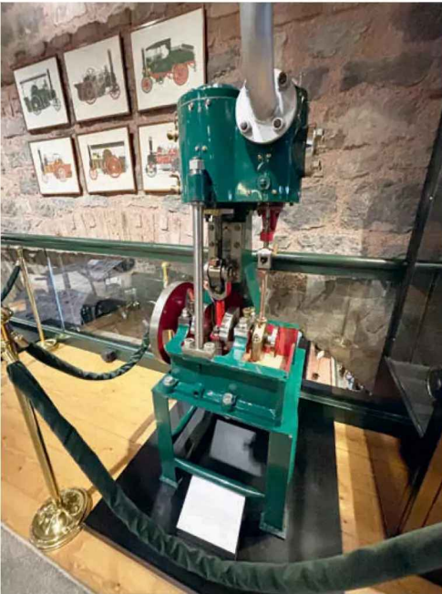
Photo 9: Single cylinder steam engine manufactured in Holland between 1970-1980. It was produced to demonstrate the working principles of single-cylinder steam engines.
