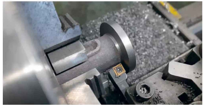
Photo 31: Left hand tool used to clean up surface for nuts.
