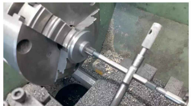
Photo 35: Cover turned, drilled and gland being tapped.
