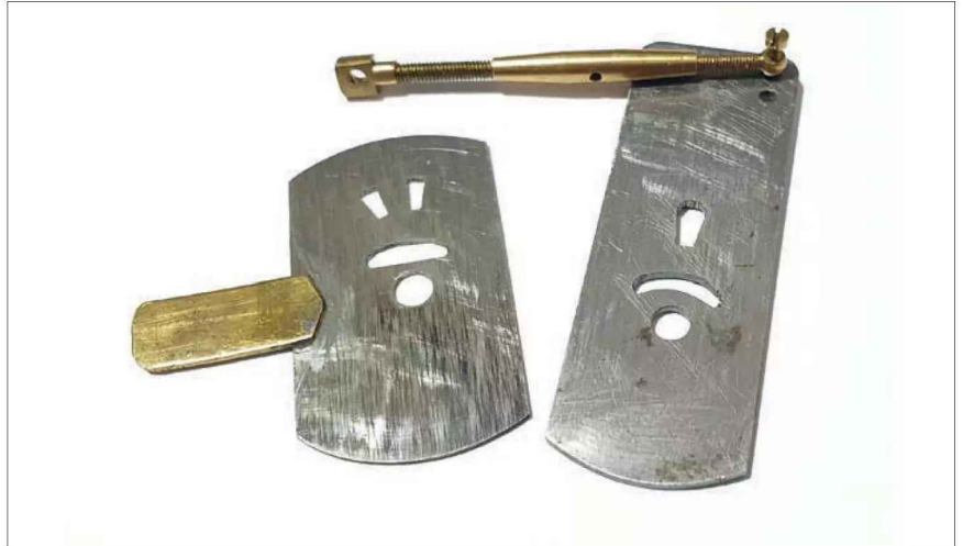
Photo 3: Types of moveable port plates. The right plate (with one aperture) was for two-way running with an earlier design of port block. The plate on the left is for one-way running to establish optimum port positions.
