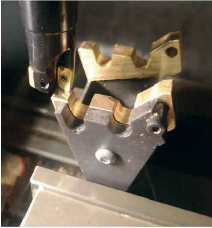
Photo 6: Machining across to break into the drillings and form the slots.
