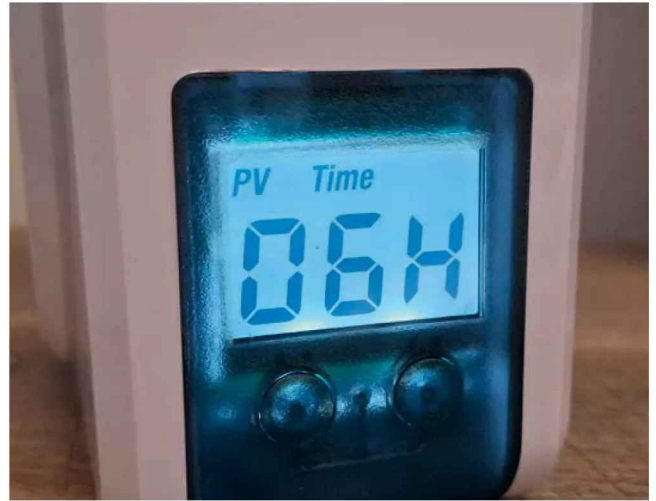
Photo 4: Two buttons access the various functions. An assortment of single, multiple long and short presses takes a little getting used to.
