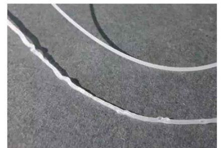
Photo 1: Test extrusions (0.4mm diameter) with Nylon 66, before (below) and after drying.
