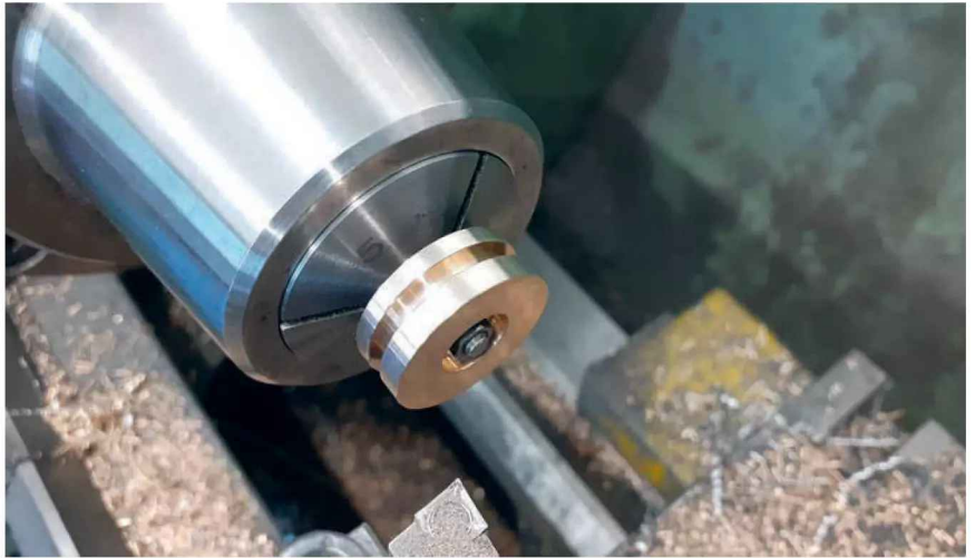
Photo 39: Turning piston to final size on its rod.
