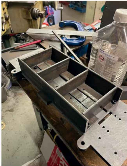
Photo 7: Gantry stiffening weldment.
