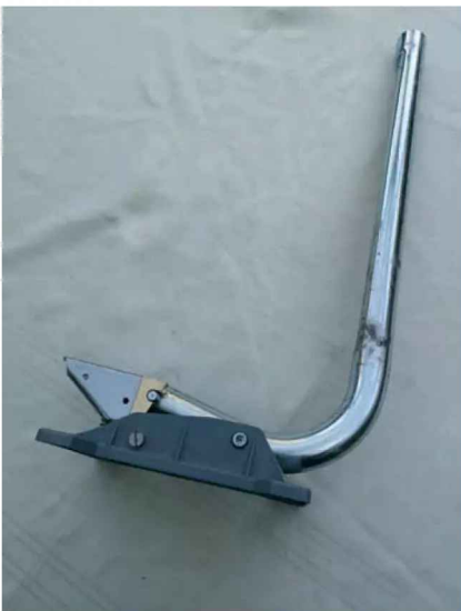
Photo 7: Pivot block angle clearance incorporated.
