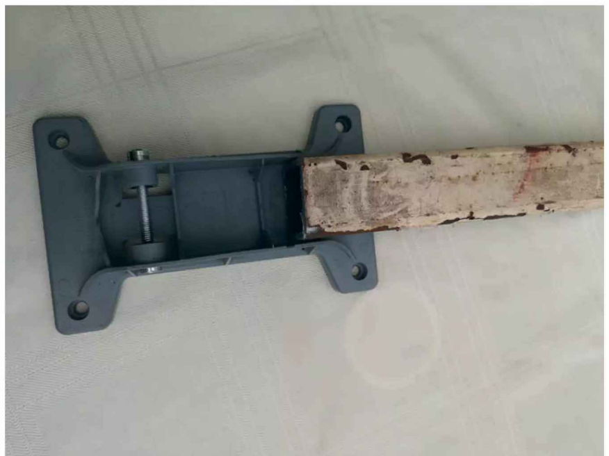
Photo 2: Steel section doesn't quite fit.
