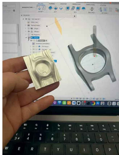
Photo 17: Watch case and CAD design.
