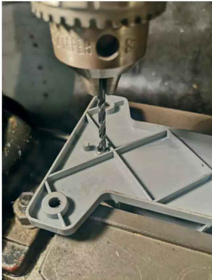
Photo 10: Drilling the channel flange for the spring pin.
