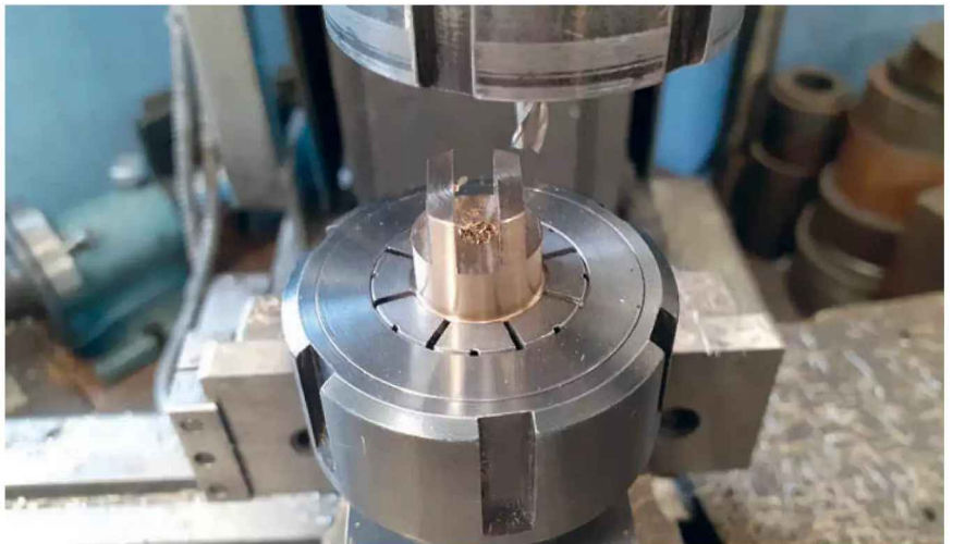
Photo 40: Milling crosshead slot and sides.
