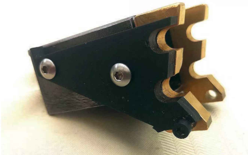
Photo 4: Pivot block with plastic slot plate attached.
