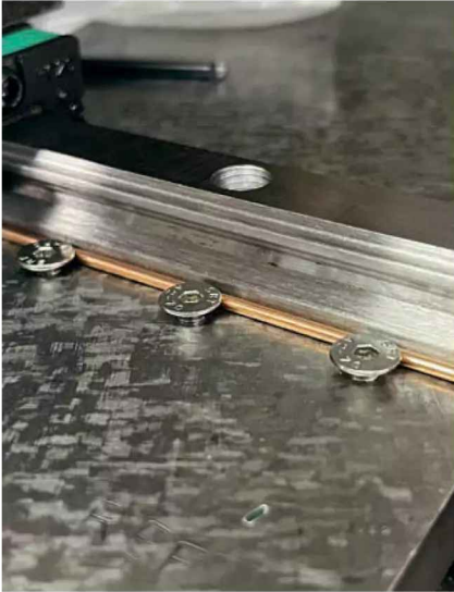
Photo 12: Alignment method for initial Y rail.
