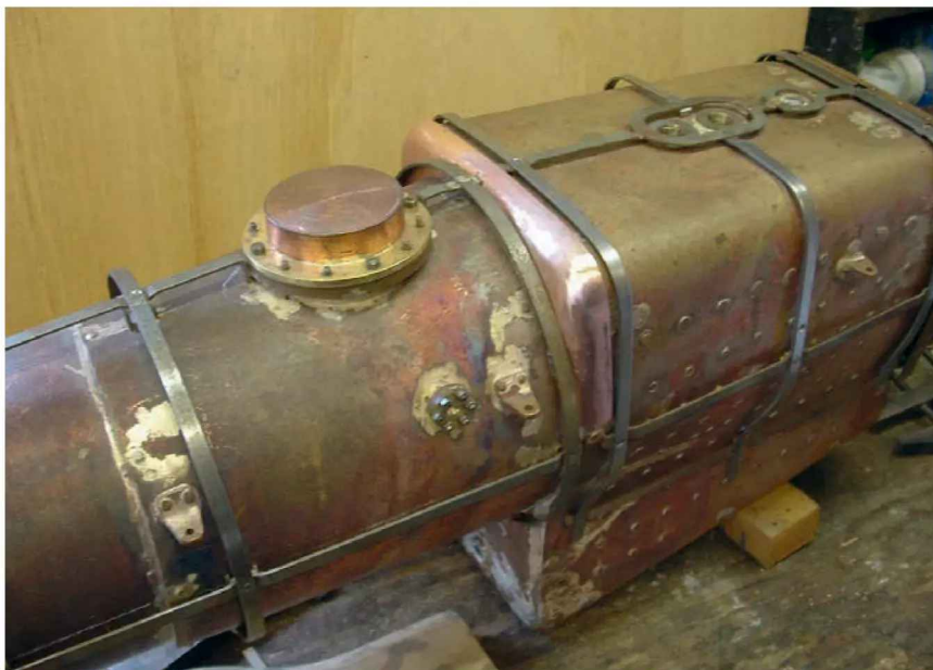
Photo 265: The oval which I made to fit around the safety valves which I silver soldered to the strips fore and aft and also the plate which I formed using the MDF block seen in photo 262.
