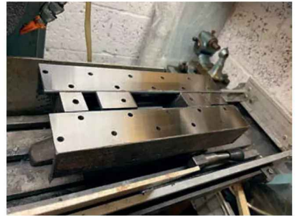
Photo 8: Surface ground weldment.
