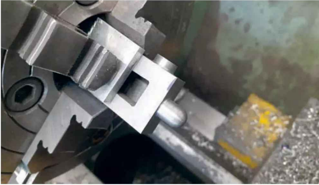
Photo 28: Turning domed end of valve chest.
