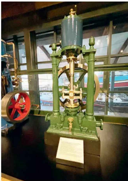
Photo 7: Single cylinder steam pump with Scotch Crank (circa 1920).
