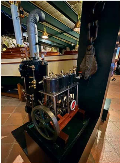
Photo 5: Three-cylinder steam engine & vertical steam boiler, manufactured in Holland circa 1970-80.
