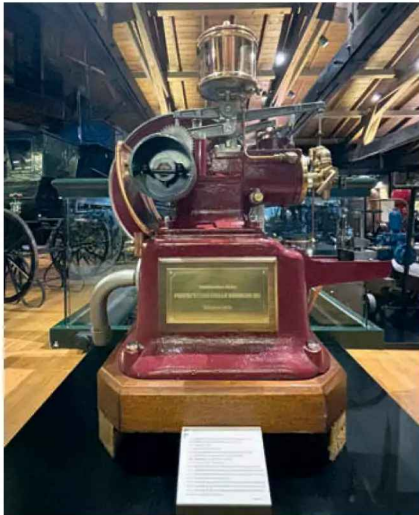
Photo 13: Langensiepen & Co., Magdeburg, Germany (circa 1898) Diesel engine. During the day this machine powered a mill in a factory, and when the factory closed in the evening, the flat drive belt was placed around the pulley of a generator to illuminate the houses next to the factory itself.
