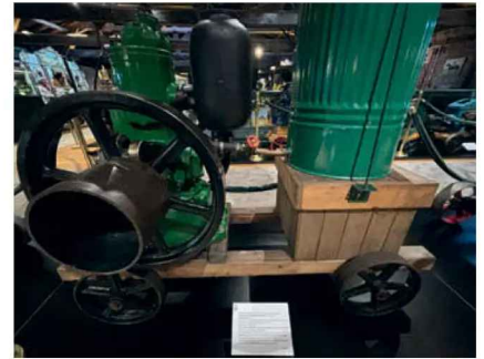
Photo 11: 2-Stroke 'M' type stationary engine (petrol or oil-fuelled) by Petters Limited, Yeovil (circa 1936), 5HP, 600 rpm.
