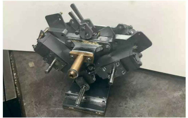
Photo 2: The original Fourrunner (end plate removed) incorporated a rudimentary reversing mechanism.
