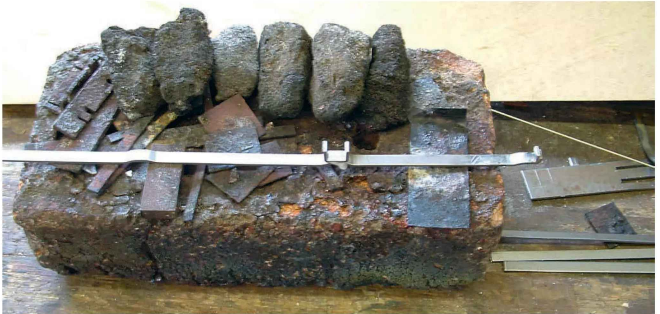
Photo 264: Another thing which I had to do was to silver solder a square of the same material on to the strip.
