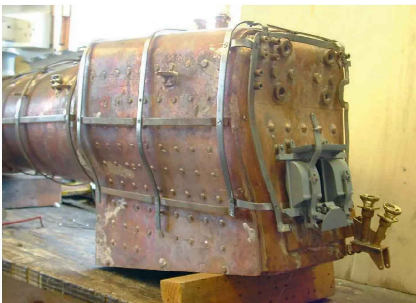
Photo 266: The crinolines now completed with a few more bits added including the base for adding the backplate cleading later.
