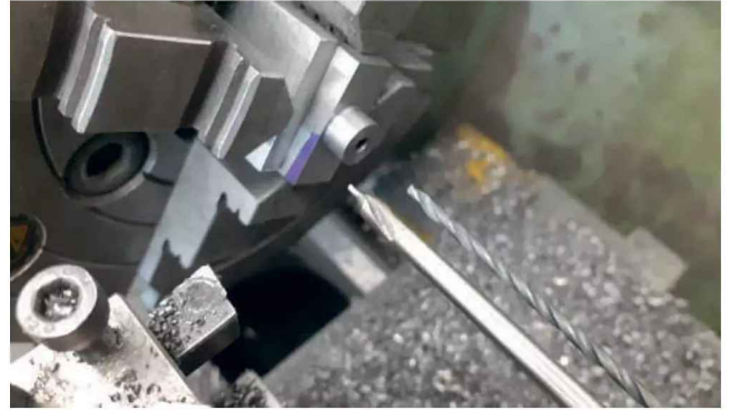
Photo 29: Long centre and 2.5mm drills for guide hole.
