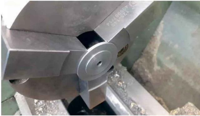
Photo 36: Shallow spigot turned on reverse side.
