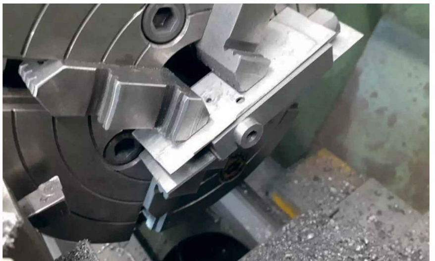
Photo 27: Machining top edge of valve chest.
