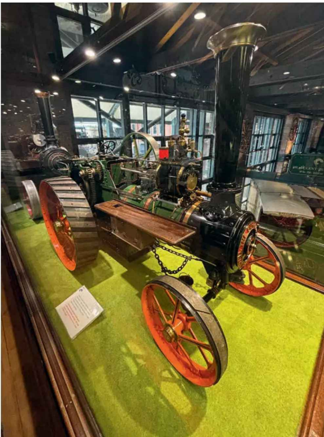
Photo 3: A wood and glass case containing, from right to left: ¼ full size working scale model of a 6HP general purpose agricultural traction engine built in 1901 by the company Charles Burrell & Sons at St. Nicholas Works in Thetford, England; ¼ full size working scale model of the last 7HP general purpose traction engine built by W.M. Allchin Ltd. Globe Works in 1922, Northampton, England.
