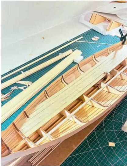
Installing the deck planks.
