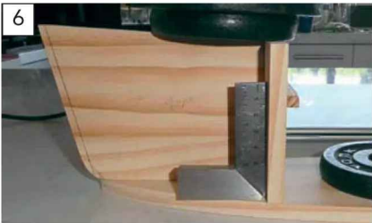
6 7 The pine frame bulkheads glued to the hull bottom and middle deck with exterior-use PVA, checked for squareness and then clamped/weighted overnight to cure.
