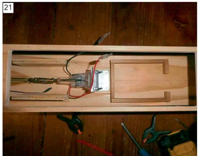
21 6mm square spruce battery position frame glued in front of the motor mount (as close as possible to 'guesstimated' CoG position), with scrap plywood mounts either side of the coupling/shaft to support the RX/ESC mounting plate.
