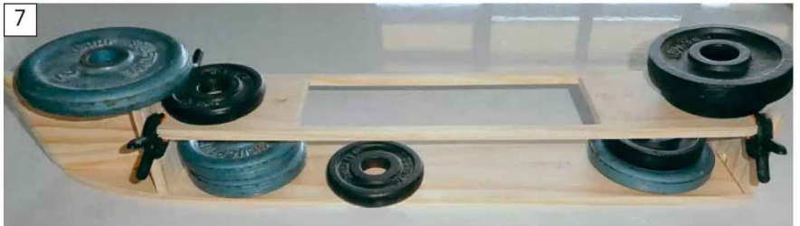
6 7 The pine frame bulkheads glued to the hull bottom and middle deck with exterior-use PVA, checked for squareness and then clamped/weighted overnight to cure.
