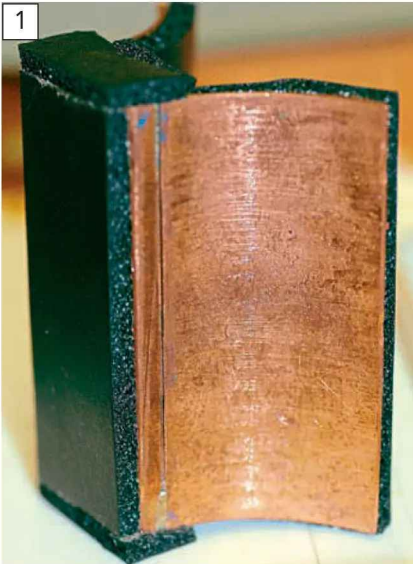
A copper saddle made from a chunk of electrical bus bar soft soldered to two pieces of copper pipe. All external surfaces have been insulated to prevent heat loss and get the most to transfer from the separator to the gas tank.
