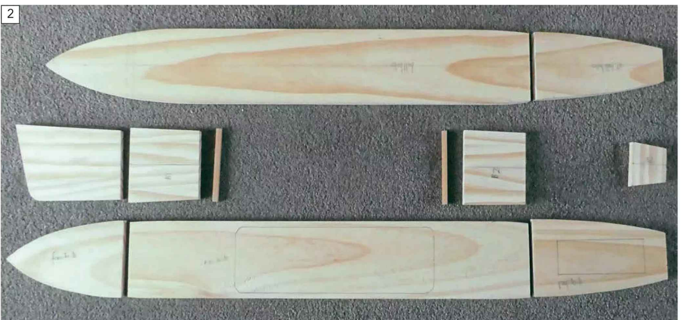
Hull frame pieces traced onto 12mm and 10mm pine and cut out (Nick used the pin-thru-plan method)
