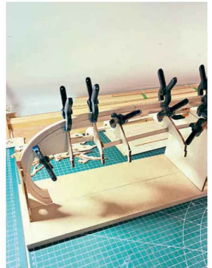
The first plank being laid.
