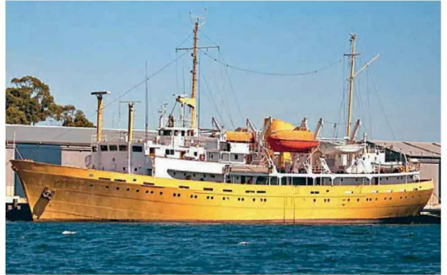
Wyuna at Inspection Head, Tasmania, showing the additional bridge modification to suit use by the Australian Maritime College.
