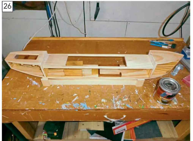
All R/C equipment removed, and the hull's internal surfaces sealed with polyurethane varnish for the waterproofing of otherwise inaccessible areas/places prior to side sheeting (with care taken not to avoid any surfaces where glue is later to be applied). Note, this was done in the shed, not on the dining room table!
