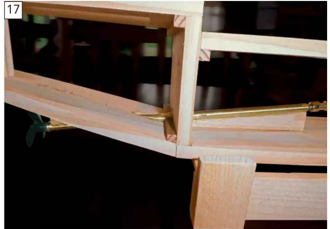
17 200mm x 4mm brass prop tube epoxied into position while connected to motor via solid coupling to ensure correct alignment.
