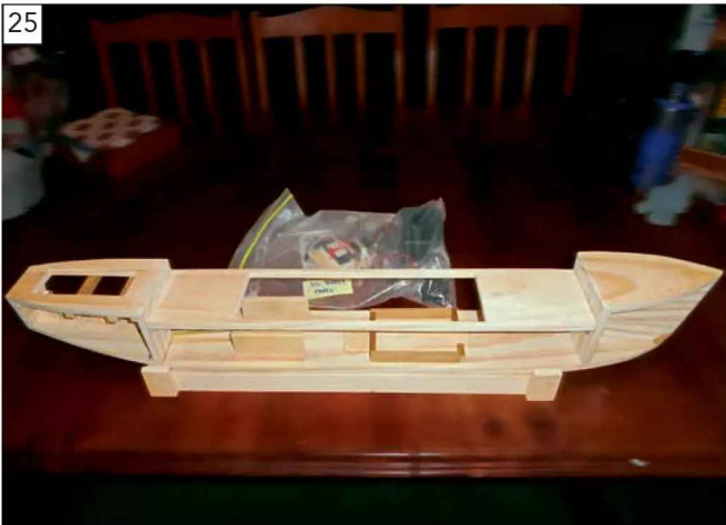
All R/C equipment removed, and the hull's internal surfaces sealed with polyurethane varnish for the waterproofing of otherwise inaccessible areas/places prior to side sheeting (with care taken not to avoid any surfaces where glue is later to be applied). Note, this was done in the shed, not on the dining room table!
