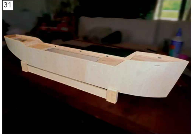
31 The hull sides trimmed to intended gunwale line, screw-holes filled and sides rough-sanded to remove any unevenness between hull side sheets. The freeing ports will be drilled and filed around the gunwales as suggested by plan and then the hull sanded smooth (240-400 grit paper) in preparation for sealing/painting.
