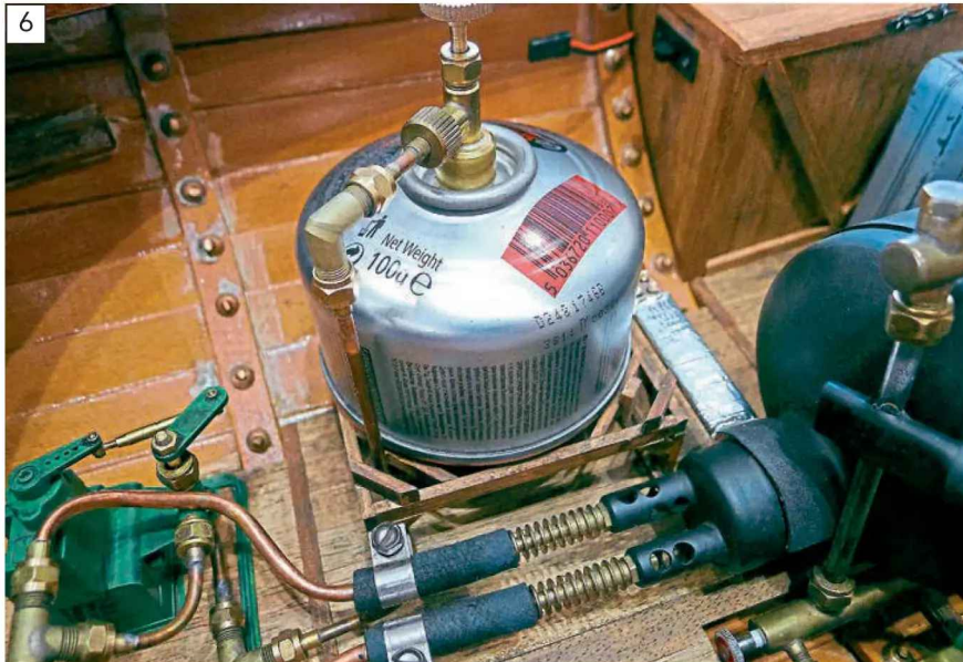
The gas tank sits on the warming plate. Richard admits to being quite surprised at how warm the plate actually gets, doing a good job of slowing down cooling of the disposable tank until such time as it can be replaced by a fresh one.
