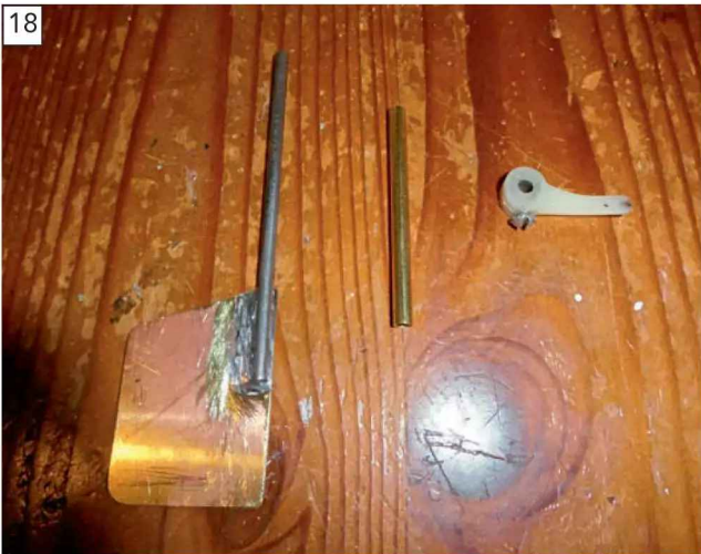
18 The 0.5mm brass sheet rudder cut out, filed, cleaned with rubbing alcohol and soldered to flat-filed end of a 4mm piano wire shaft – this having been cut to length and another flat filed on the opposite end to fit the repurposed aircraft nose wheel steering arm with grub screw. Also shown is the brass rudder tube of 4mm internal diameter cut to length.
