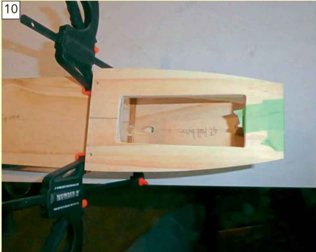
The stern pieces of carcass placed together and clamped, without glue, so the prop tube hole can be marked, drilled, alignment checked, then filed out.
