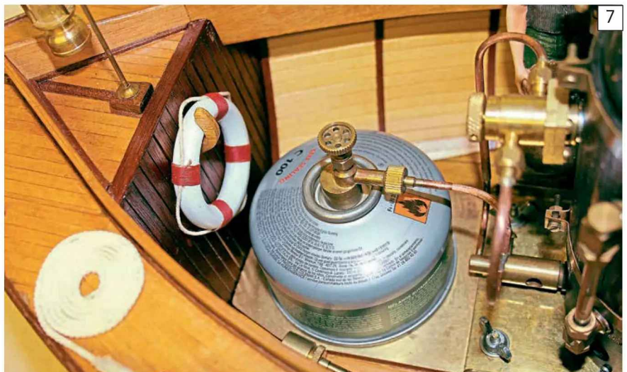
Sitting the gas tank on a brass base common with the boiler is an excellent way of using some waste heat to warm the tank. Keeping the tank close to the boiler also helps. Both, again, being things that need to be considered during the design of the plant layout.
