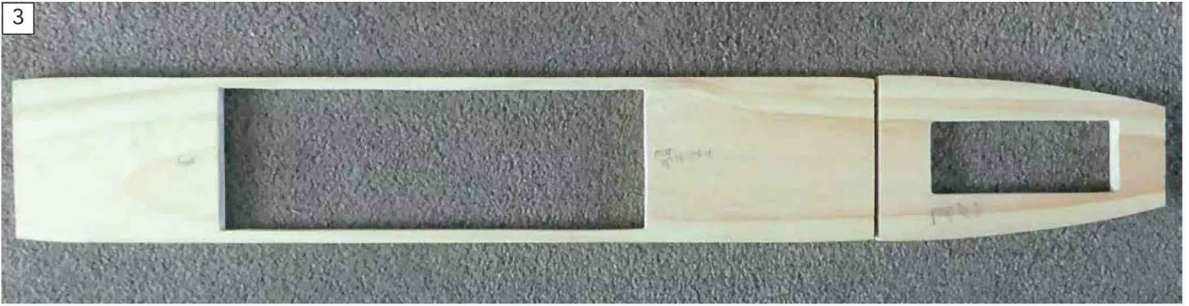
3 The hatch openings cut out using jigsaw/file and grit paper.
