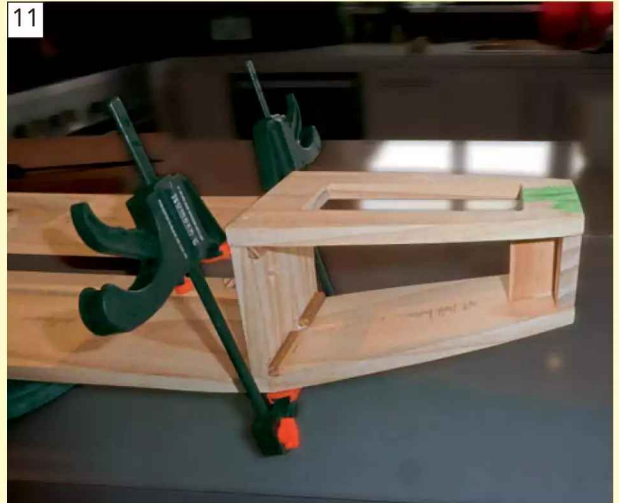
The stern pieces of carcass placed together and clamped, without glue, so the prop tube hole can be marked, drilled, alignment checked, then filed out.
