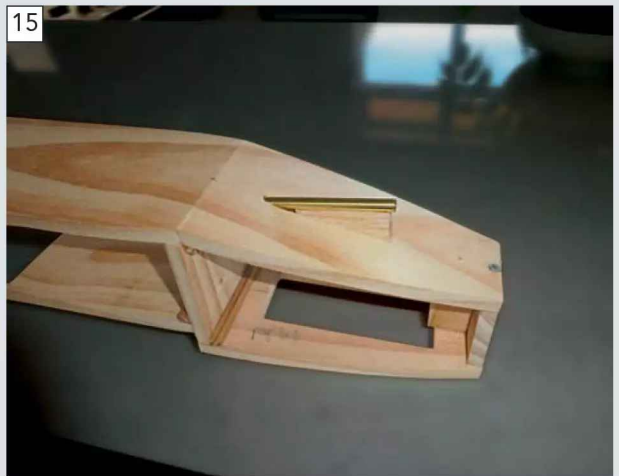
Stern section now glued together, alignment re-checked, 'pinned' with small screws and left to cure. Note the slight slope of the rear deck piece.
