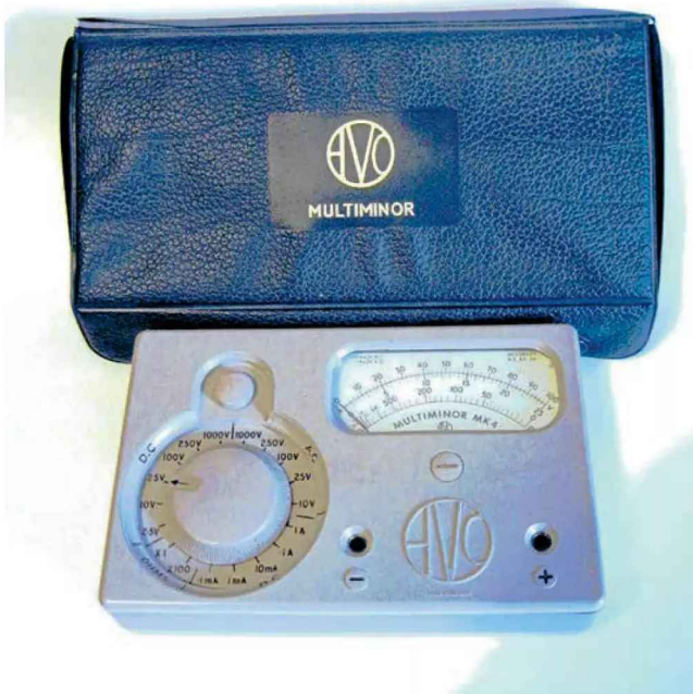
The little 'Avo-minor' was the junior instrument in AVO's range of professional measuring instruments.
