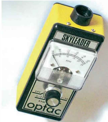
A more modern rpm meter/optical tachometer made by Skyleader of Croydon.
