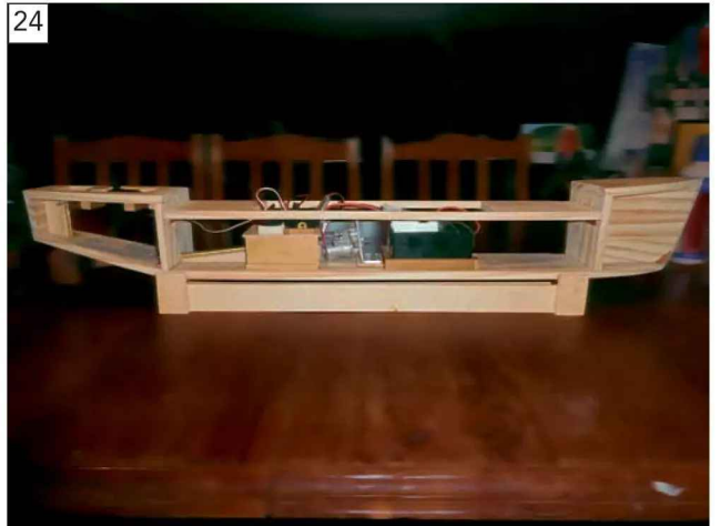
With the rubber tube now epoxied in position, the complete radio-control motor and steering set up is now installed and ready for testing - again, highly recommended, since it's much easier to make adjustments before the hull has been sheeted.
