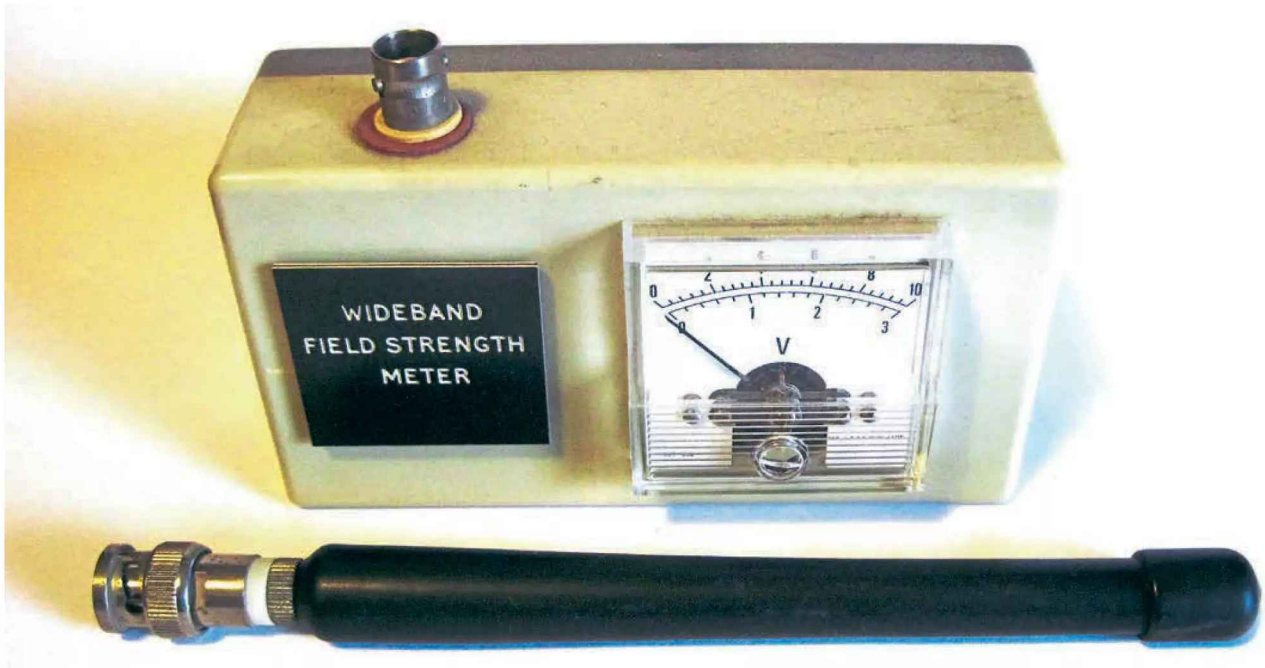
This home-built signal strength meter has been invaluable to Dave since about 1970.
