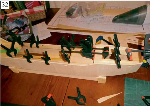
32 Hatch coamings from 1/16in basswood glued and clamped. The inside corners of the coaming will later be reinforced with scrap 6mm square spruce.
