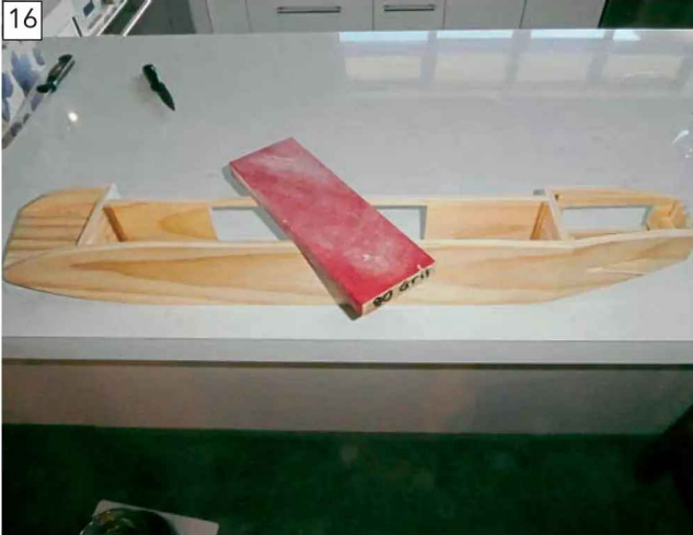
16 Carcass sides course-sanded/shaped to ensure good fit of side sheeting.
