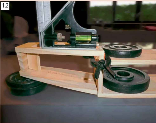
Stern section now glued together, alignment re-checked, 'pinned' with small screws and left to cure. Note the slight slope of the rear deck piece.
