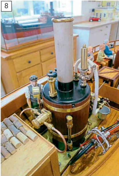
A mechanical attenuator valve, like this one from Forest Classics, maintains a constant boiler pressure. This means that the burner is only providing the heat that the engine needs so minimizes gas consumption and hence the cooling effect on the tank.
