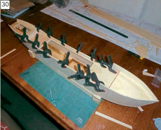
30 The gunwales reinforced with 1/16in bass strip, with the grain at 90-degrees to that of the side sheets, ensuring better strength around the freeing ports.
