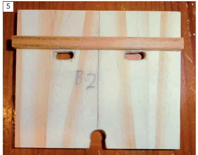
5 Holes drilled and filed out for prop shaft and servo connections.
