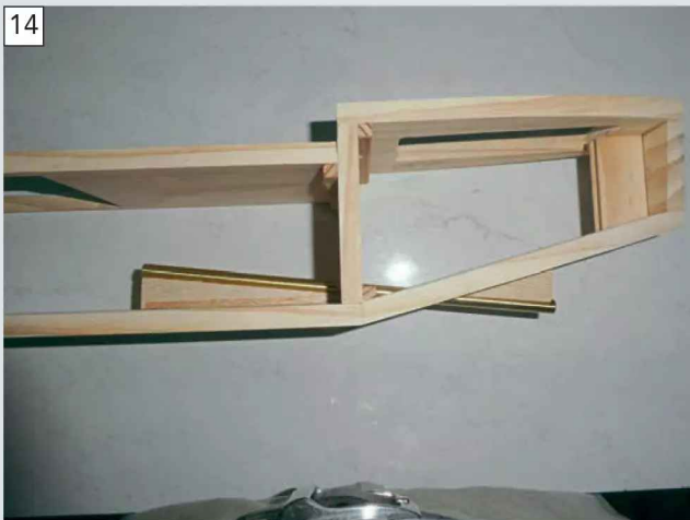
The prop tube inserted and internal support & skeg cut/filed to shape before gluing.
