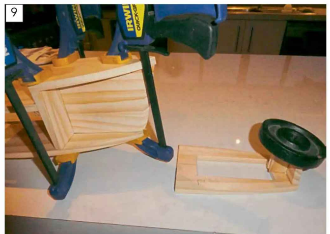
9 The foredeck glued to stem, and rudder tube support glued to rear deck piece.
