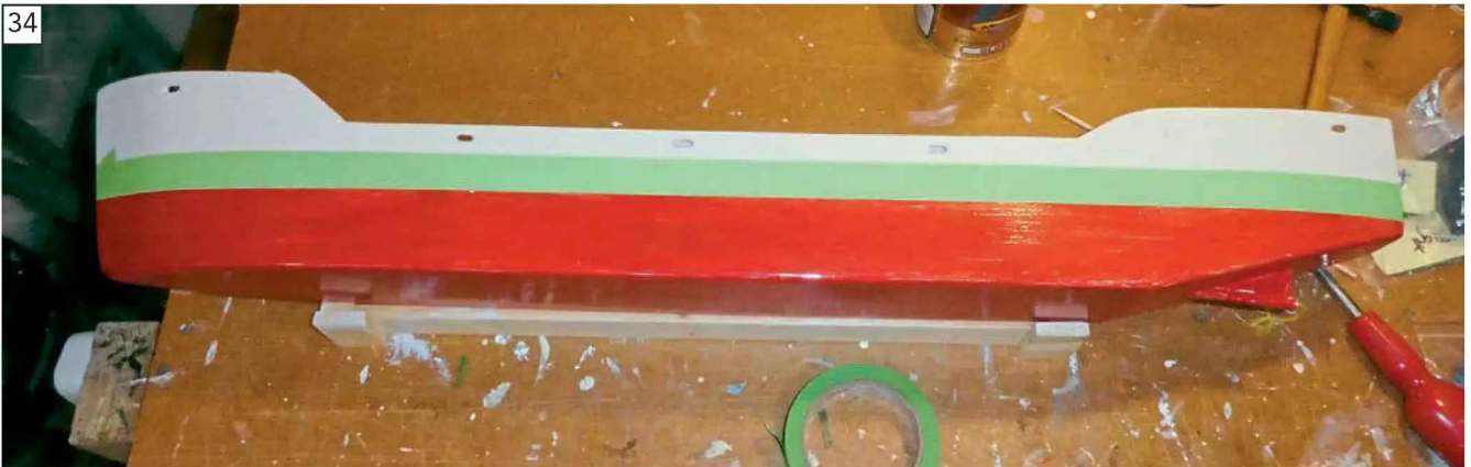
34 The hull now sealed with two coats of oil-based undercoat, sanded back, and oil-based enamels applied. Using the waterline suggested on the plan, gloss black enamel was used for the upper hull and gloss red for the lower. During this process, each individual coat was given a minimum of 24 hours drying time, with a light sanding to create a key before the next layer of paint was applied.
