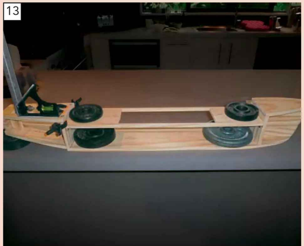
Stern section now glued together, alignment re-checked, 'pinned' with small screws and left to cure. Note the slight slope of the rear deck piece.
