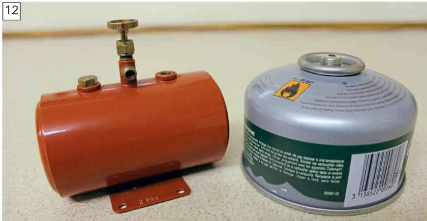
Using disposable gas tanks gives you a lot of flexibility in terms of operation and minimising the effects of gas cooling. The disadvantage is the cost of the 100g gas tanks.
