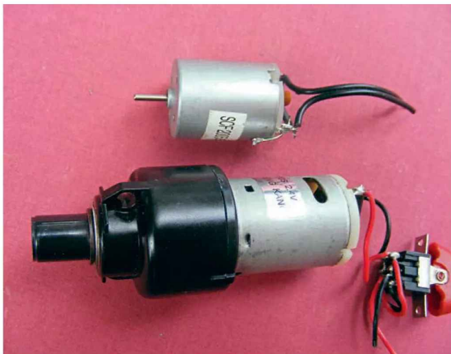
The motor and gearbox Glynn retrieved from a discarded electric screwdriver, sitting alongside an old chair motor also fit for repurposing.
