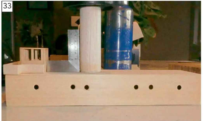
33 The superstructure, made from a combination of 3mm/1.5mm bass and 1/32in ply. Having been checked for 'squareness', the funnel, built up from 3mm scrap balsa strips around circular formers is now glued to the superstructure. The portholes have been carefully drilled/ filed out to avoid splitting the wood.
