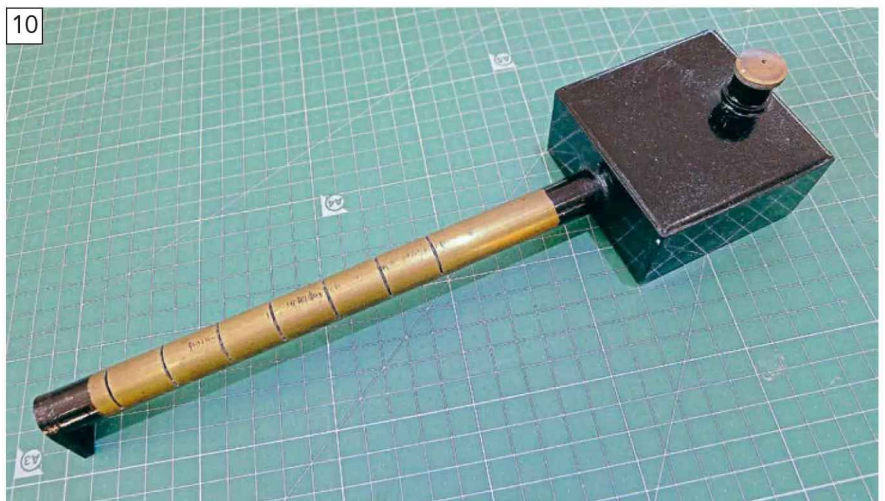
A traditional methylated spirit burner, as used on all Stuart Turner boilers for many years. The liquid fuel evaporates at the wick, so there's no variation in flame. Sometimes the old ways still have advantages!
