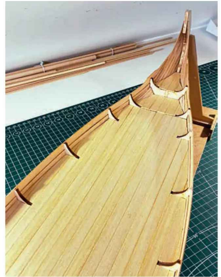
Deck planks fitted to the hull.
